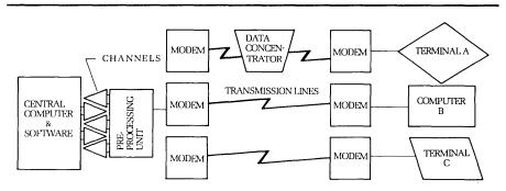
Figure 1. Typical Data Communications Network
