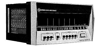
incredible job too. Because the general purpose 620/i has a bigger instruction set than any other computer in its class. 1.8  $\mu$ sec. cycle time. 16/18 bit words. 4-32K memory. Easy interfacing capability. Multi-level priority interrupts. Field-proven software. 10½ inches of rack space.
