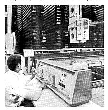
ized materials handling system controls the cranes by feeding punched cards into a central computer console as shown in the picture above.
