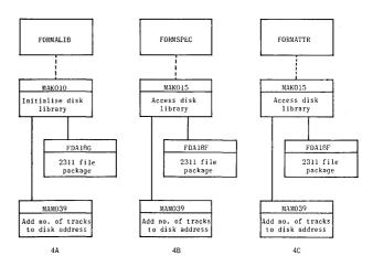
Figure 4. An example of reusing procedures in different parts of a software package.
