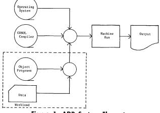
Figure 1. ADP System Elements
