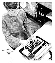
The new devices prepare computer-ready half-inch magnetic tape compatible with all Honeywell Series 200 computer systems, from the new small-scale H-110 (see New Products, Digital) through the large-scale H-8200, and with most computer systems of other manufacturers.
