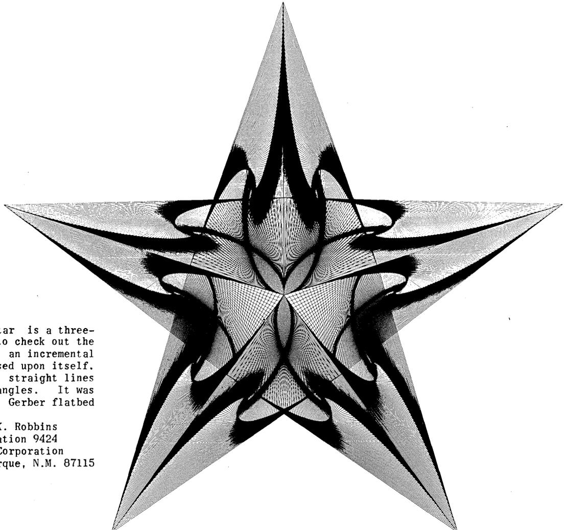
This five-pointed star is a three-pointed star, used to check out the incremental step on an incremental plotter, superimposed upon itself. The design has many straight lines at many different angles. It was produced on a large Gerber flatbed plotter.
