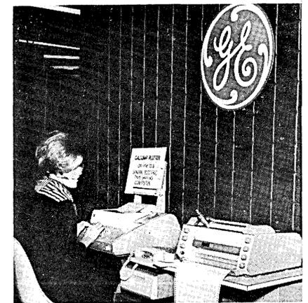
the stand under the plotter is a CalComp Model 210 controller which monitors all incoming data from the
