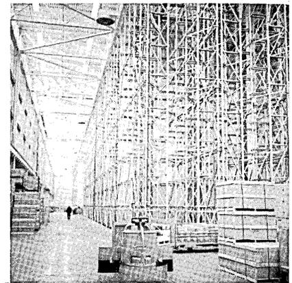
— Driverless tractor follows a cable buried in the floor to a programmed "stop" location
