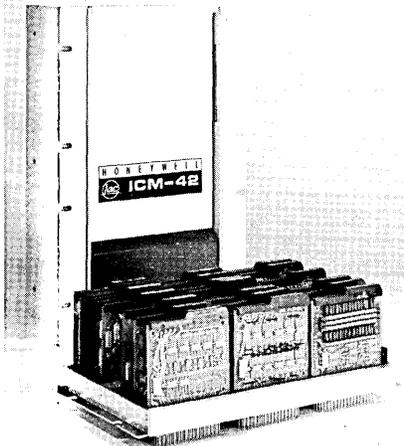
or as a separately-housed, self-contained memory unit designed for rack mounting (rear of photo). The pluggable core stack and other circuitry are accessible from the front of both units. (For more information, designate #45 on the Readers Service Card.)
