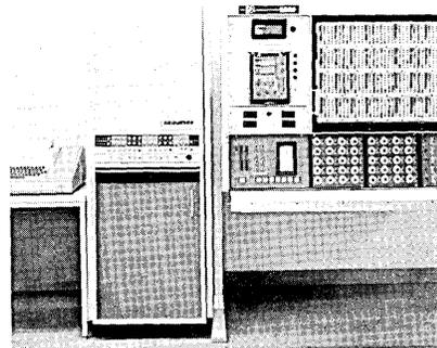
The GPS 200T is claimed to differ from other compact computers in that it is designed for greater expansion and for highest possible performance in real time and repetitive modes. Although furnished in a compact, desk top size cabinet, the GPS 200T is expandable to a complement of approximately eighty computing elements.
