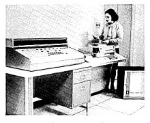
standard 100-word-per-minute teletype unit for each station and central control monitoring, and an ULTRONIC<sup>®</sup> Local Control Unit for installation at each station location (the Central Control Unit at the main office is the same in appearance and size). Not shown are the DATA PUMPS<sup>①</sup> (about the size of a telephone) which would be installed at each station.
