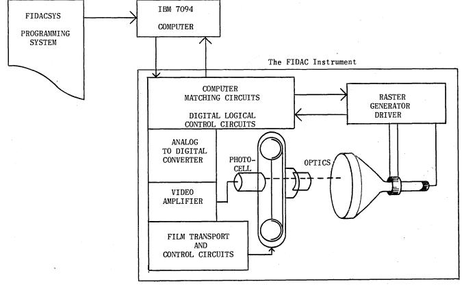
Figure 1b. Block Diagram of FIDAC System
