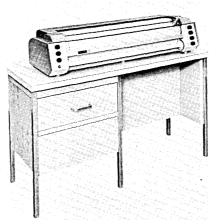
900 steps-per-second in .005 inch step size and 450 steps-per-second in the .01 inch step size. Model 663, with a 30-inch drum, operates at corresponding speeds of 700 and 350 steps-per-second. (For more information, designate #58 on the Readers Service Card.)
