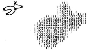
Figure 2. At the right is the representation in the computer's memory of a scanned chromosome. At the left are the plotted results of the computer analysis: the crosses represent the locations determined by the computer for the ends of the arms; the central line represents the location of the centromere as determined by the computer.
