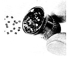
Approximately 8,000 are contained in this tiny thimble. Each has the equivalent of up to 57 components such as transistors, resistors and diodes. The circuits, produced by Sylvania's Semiconductor Division, are used in computers, missiles, space vehicles, satellites and aircraft guidance systems.
