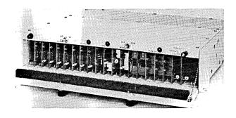
MAGNETICALLY CONTROLLED CORE MEMORY DI/AN Controls, Inc. Boston 25, Mass.
