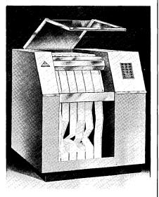
soundproofed cabinet houses the entire system which includes six 24column listers, control electronics and buffers. Solid-state electronics are used throughout this system. It will operate in any environment where other data processing equipment is normally located.
