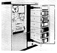
which have been mechanically modified for slide mounting in a van. The entire computer slides in and out of its rack as one assembly. Also, the paper tape punch, spooler, reader, and the power supply are mounted on slides. The machine may have extra long cables (some as long as 40 ft.) in order that the paper tape equipment, typewriter a and control panel may be physically removed from the computer itself when mounted in a van.
