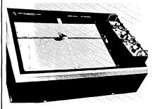
The HR-97 has interchangeable plug-in control modules. All of the plug-in modules have precision ten-turn input attenuators, full-scale zero adjustments and automatic pen-lift controls. A load-operate switch automatically picks up the pen and positions it away from the chart area for easy loading of paper.
