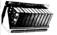
device transmits the total or net amount of these impulses to any one or a combination of the following: computer, data logger, telemetering equipment, printing demand meter, or other totalizer.
