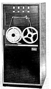
Model 3031 receives and punches into 8-channel tape information transmitted from the various points of origin. It contains tape handling mechanisms, control logic, and provides its own power and that of all transmitters on the same cable line.
