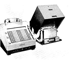
This machine translates information into machine language for computer use. The NCR tape-punching adding machine is programmed to operate the punched tape recorder automatically. An amount entered in the keyboard, adds into the machine total, prints on the adding machine tape, and is punched into the paper tape in code. An operator needs only to read printed tape to know what was recorded on punched tape. Corrections can be made before punched tape is sent off for processing.
