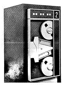
This magnetic tape device is suited to applications on small and medium scale computers and off-line systems where there are non-technical personnel and where long term continuous operation and low maintenance are required. The D 2020 is IBM compatible for tape formats of 200 and 556 bits per inch and has a 30 inches per second bidirectional drive with a 5 ms start and 1.5 ms stop. The series includes the transport, low and dual density signal electronics, and a complete group of options.
