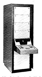
**CI-70** Precision Potentiometer Positioning System provides fully automatic tape or card set-up for coefficient potentiometers, diode function generators and UNE's. Programming time is reduced by a factor of 5. Potentiometers are set in less than 2 seconds each, with error no more than 10 millivolts. Other features are automatic scan, automatic check-out, and automatic error indication.
