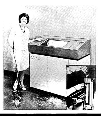
A new model of the H2O7 medium-speed line printer has a print ribbon claimed to have three times former life. When 64 characters are printed, line speed is 300 lines per minute. Interchangeable print drums (see photo insert) allow increased speed when a large selection of characters is not needed. A swing-up drum arm permits easy forms loading. A printer control, cabinet, and buffer for character serial input are optional with the print head.
