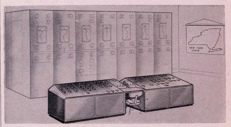
This new transistorized Economic Dispatch Computer, developed by G-E's Computer Department for the Niagara-Mohawk Power Corp. and the New York State Electric & Gas Corp., represents a significant advancement in the field of dispatch computers.
