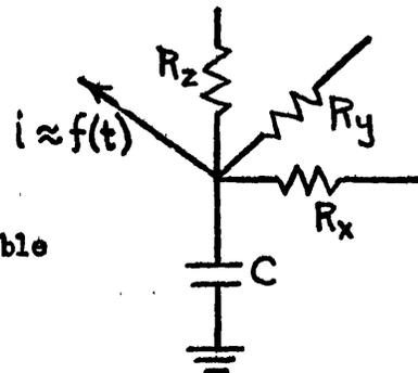
Figure 3 -- Analogous Electrical Circuits for Three-Dimensional Thermal Elements
