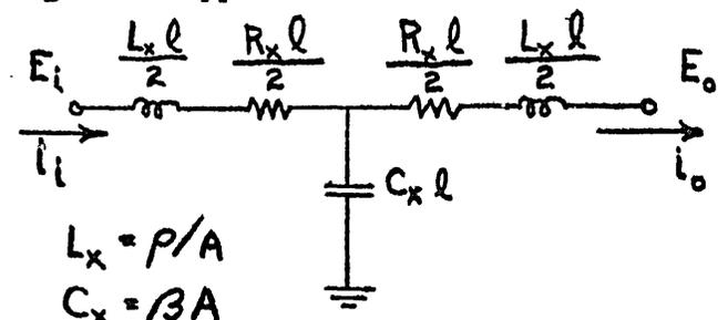
Figure 4 -- Electrical Analogies for Hydraulic Components
