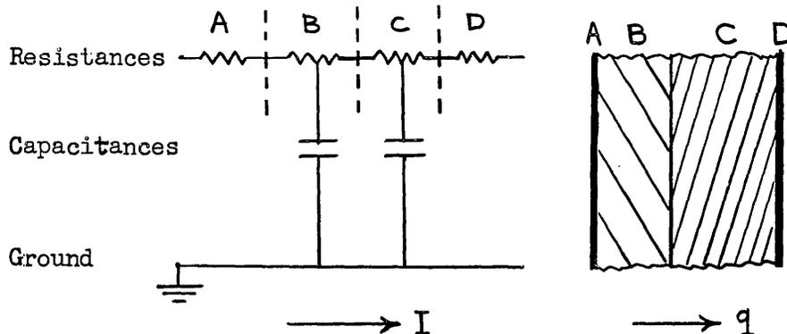
Figure 2 -- Comparison of Electrical and Thermal Relations
