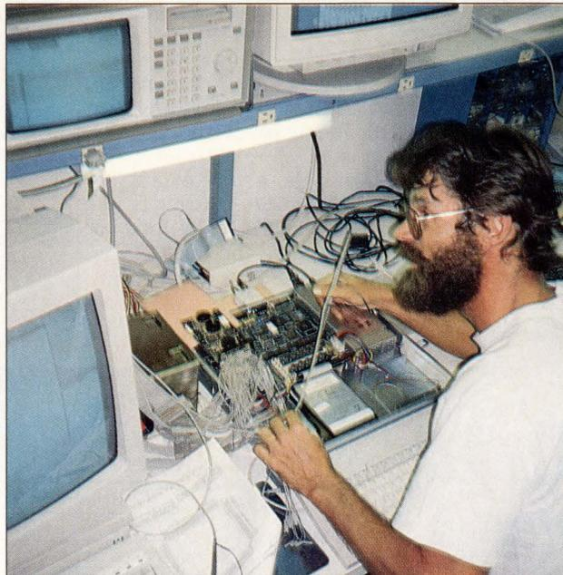
*James Warford, Nimbus Technology's manager of systems integration, says, "Using 'known-good' M bus processor modules is an advantage in wringing out a system. M bus timing is well-defined, and troubleshooting is relatively straightforward." Here Warford uses a header between a motherboard and processor board to put a logic analyzer on the M bus.*
