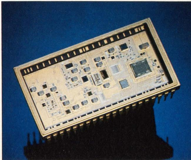
Hybrid A-D converters such as Comlinear's CLC935 still have a performance advantage over monolithic parts. This 12-bit, 15-Msample/s part maintains a 77-dB spurious-free dynamic range at 7.22 MHz. Signal-to-noise ratio is 66 dB out to Nyquist rates (7.5 MHz).
