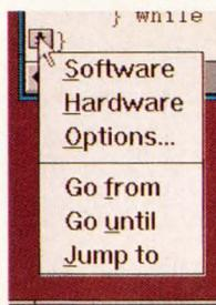
Breakpoint buttons appear on eligible lines. Set, delete, or switch between hardware and software breakpoints with one click.
