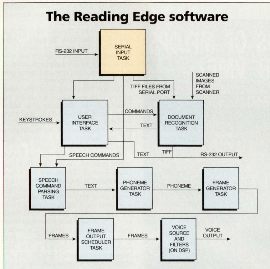
*Much of the processing in The Reading Edge machine is done in software. Images are received from the scanner, converted to text and broken down into phonemes. These phonemes are divided into discrete time segments called frames. The frames are sent to the DSP, where they modify filters that control the speaker output.*
