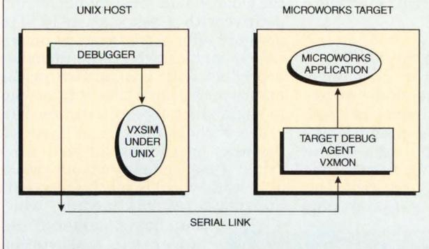
software runs as a UNIX process using the Sunos lightweight process mechanism to manage context switching. "You're writing C source and debugging with VxGDB, whether you do it on the host or target," Barbagallo says. "When the hardware comes in, you just recompile and download."
