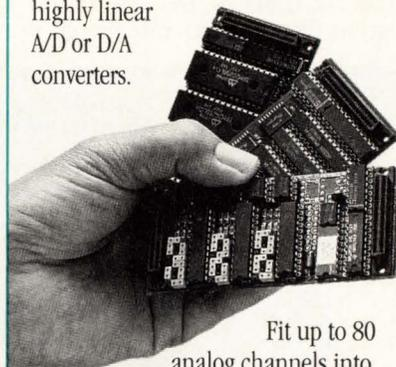
Fit up to 80 analog channels into one VMEbus or ATbus slot — up to 40 per Nubus slot. Directly connect most sensors including thermocouples and current loops. Programmable gain and low drift guarantee precision data.
