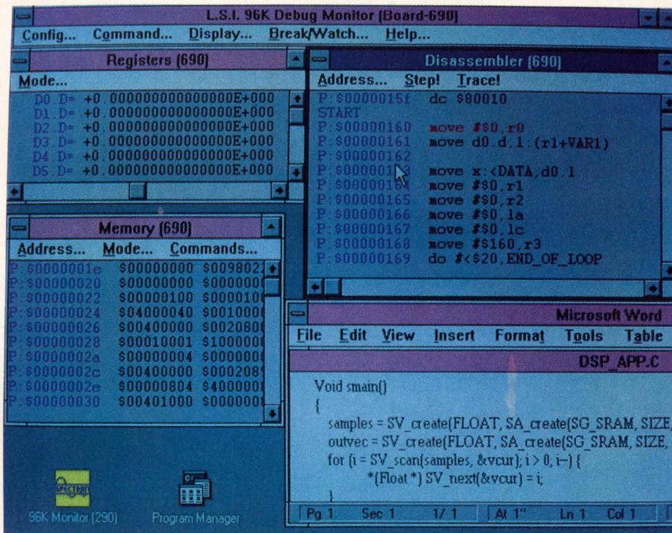
You can view registers, data memory and disassembled program memory simultaneously.
