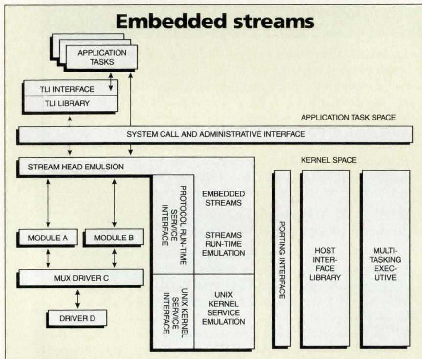
*Embedded Streams resides alongside a real-time kernel to which it's adapted via the host interface library. Streams can be constructed by interfacing modules and drivers to the embedded stream head (left). User tasks can access the stream head directly or via a TLI library that offers an OSI Layer 4 programming interface that's common to a number of different communication protocols.*
