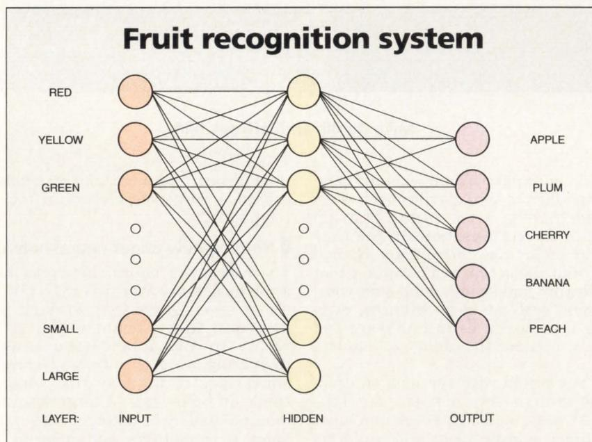
*In this simple neural network, a layer of inputs lists the various characteristics of fruit. When the network gets a stimulus from one or more of these inputs, it responds with an output. If the network guesses incorrectly, it adjusts the correlation of the internal connections or synaptic weights until it gets a correct answer.*
