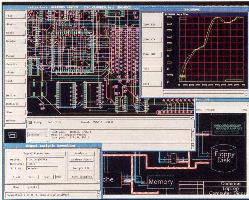
Cadence's System Workbench lets you adhere to electrical, physical and timing constraints during the entire design process. In this photo, Allegro's SigNoise (left window) is used to ensure the signal integrity of a trace in the layout (blue and white line at bottom of left window). The graphic display of the noise analysis is shown in the Etwave tool (right window).
