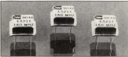
Connor-Winfield Corp. introduces its new 8-pin DIP ECL clock oscillators. The E500 Series is available in frequencies from 24 MHz - 180 MHz. Options available include industrial temp range of -40C to +85C, complimentary output, enable/disable function, and surface mount header. Frequency stabilities are available to +/-25 ppm over temperature.
