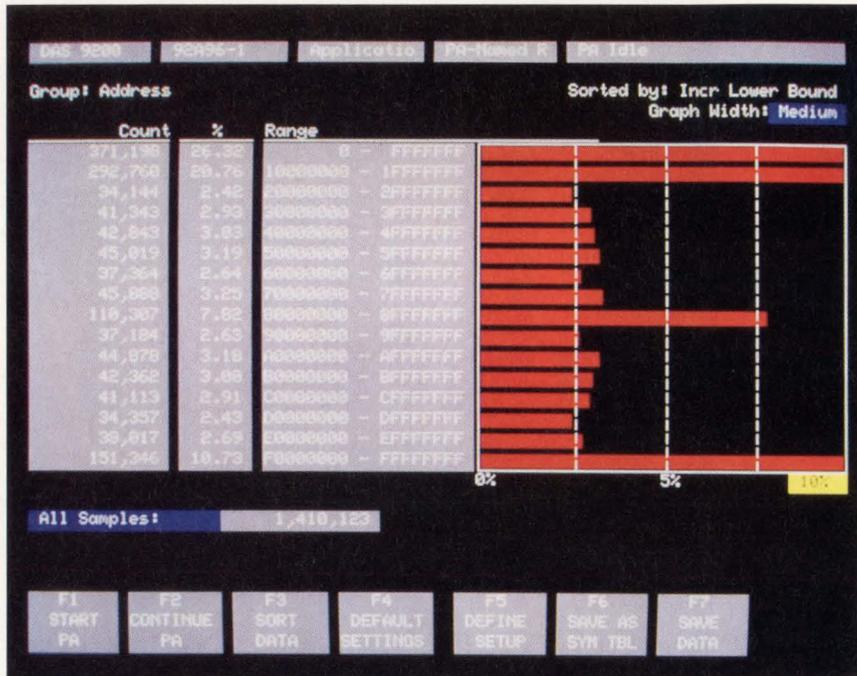
The Tektronix digital analysis system (DAS) gives insight into how well code is running at a structural and architectural level. One of its capabilities is code profiling, in which the display is divided into address ranges which show a statistical sample of what percentage of the CPU's time is being spent in which parts of the program. This lets developers home in on performance bottlenecks that might not be apparent from the level of bytes and registers.
