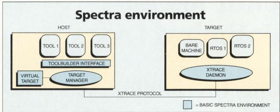
Ready Systems' Spectra environment supplies a common interface for development and debugging tools on the host system. Tools communicate with the real or a virtual target via the same interface. The shaded blocks identify the basic Spectra components.
