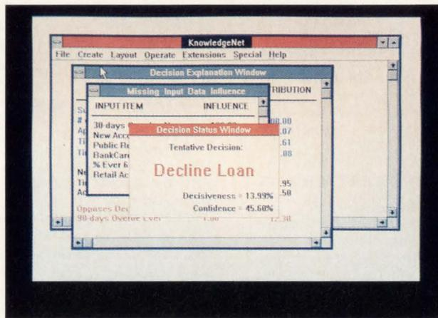
*Banks are using neural network software to verify a person's loan eligibility. In this application from HNC, variables such as an applicant's time at a fixed address, time at a particular job, previous loan delinquency, and savings account data are passed through the network for evaluation. The network builds a profile of the loan applicant and makes a recommendation to the financial institution.*
