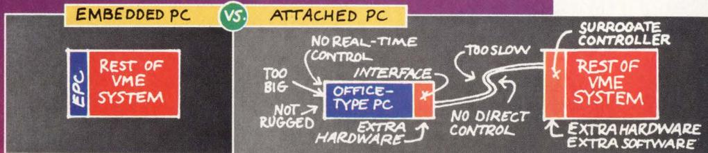
Integrating a PC with your VME system is a smart move. The "PC advantage" provides a superior human interface and access to the PC's huge base of system, application and development software.
