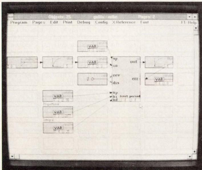
*The Gellix CASE tool lets users put control programs together by graphically linking precompiled routines in a hierarchical structure.*
