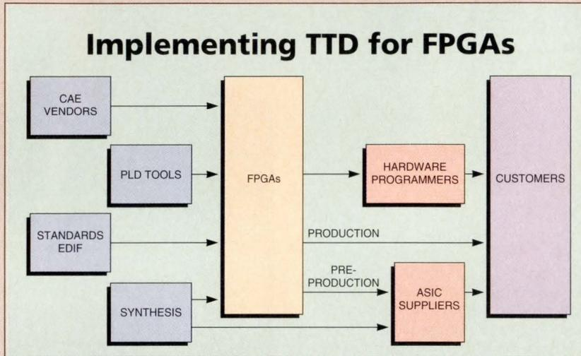
In FPGA applications, TTD would give designers access to CAE software, PLD systems, synthesis tools, hardware programmers and design platforms and a vendor-independent gate array migration path.
