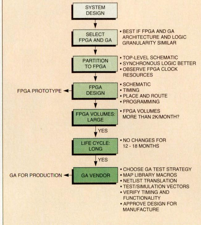
*The Actel design flow for migrating from an FPGA to a gate array makes clear that Actel emphasizes that designs turn out best when users early on try to match the FPGA to the gate array with regard to architecture and logic granularity.*
