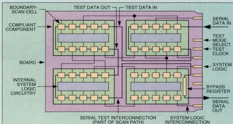
*The Bypass instruction, a mandatory requirement for IEEE 1149.1 compliance, selects the Bypass register so that the serial data path (bypassing all other test data registers) is as short as possible. Using this instruction for each component whose testability features are not being used, minimizes the scan path length across the board, saving time. The Bypass instruction makes the component behave as a single-stage shift register.*
