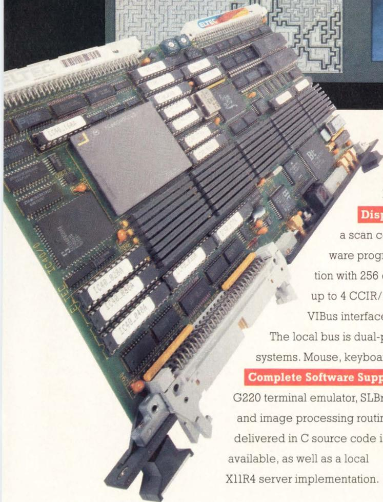
**Speed** Optimum throughput is achieved through the use of the MC68040, one of the most powerful CISC processors available, offering 20MIPS and 3.5MFLOPs combined with a local bus bandwidth of 40MB/sec. Picture acquisition occurs in video realtime.
