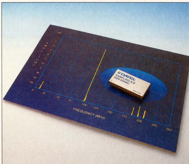
The ADS-930, a 16-bit, 500-kHz converter from Datal, offers several features geared toward signal processing applications. The device offers an SNR of 87 dB and -90 dB harmonics. An on-board FIFO provides smoother operation with DSP chips while reducing the number of DSP interrupt instruction cycles necessary.
