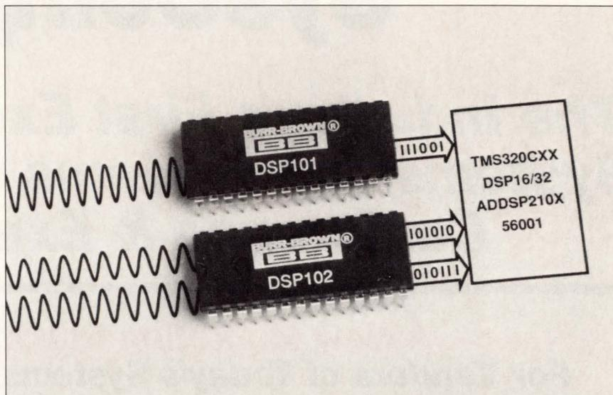
*Burr-Brown's DSP101 and DSP102 are both 200-kHz, 18-bit A-D converters specifically designed to interface with DSP chips. Instead of using an ASIC or programmable logic to implement the interface, designers can connect the DSP101/102 directly to a DSP. The parts interface with the serial ports on DSP chips from Analog Devices, AT&T, Motorola, and Texas Instruments.*
