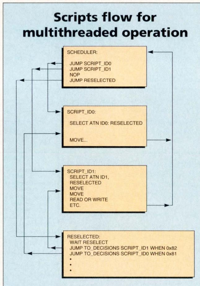
SCSI Scripts make it easy to have more than one task active at a time. The main driver running the host computer keeps track of I/O requests in a table or scheduler. Each time an application program requests a new I/O instruction, the main driver enters a Scripts Jump instruction into the scheduler. Each time an I/O is completed, the main driver replaces the I/O request with a NOP instruction.
