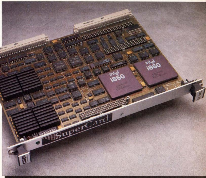
*CSPI has developed SuperCard, a i860-based vector processing subsystem for the DECstation 5000. The board interconnects with the DECstation via DEC's Turbochannel—or optionally via direct I/O ports. The DEC version of CSPI's SuperCard is finding use in a variety of applications, such as signal processing, sonar, radar, ASW, image research, medical imaging, and electronic publishing.*
