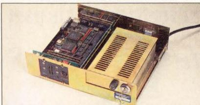
COMPLETE INDUSTRIAL PC WITH A PASSIVE BACKPLANE 286 OR 386 CPU WITH SSD AC OR DC INPUT POWER, RS232 & RS422/485 PORTS.
