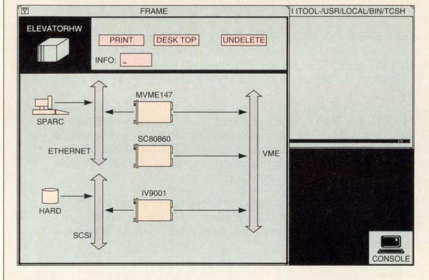
*Graphical hardware descriptions of the mixed multiprocessor architecture provide documentation and the necessary information for users to quickly build pSOS+/Unix or VMEexec applications. The transparent multiprocessing of the operating systems works with these descriptions to insure fast incremental enhancement without application changes or painful rebuilding.*
