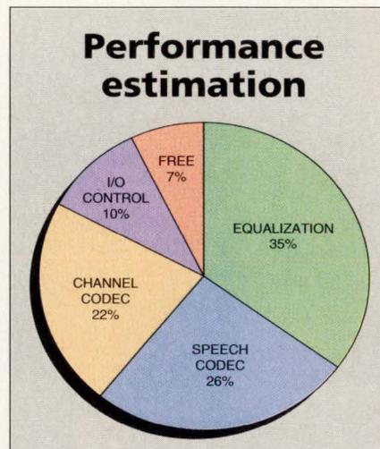
Philips/Signetics prepared a performance estimation illustrating the computational load on a digital signal processor inside a cellular phone. As can be seen, the equalization is most demanding on the DSP's time, followed by the speech and channel codec functions.
