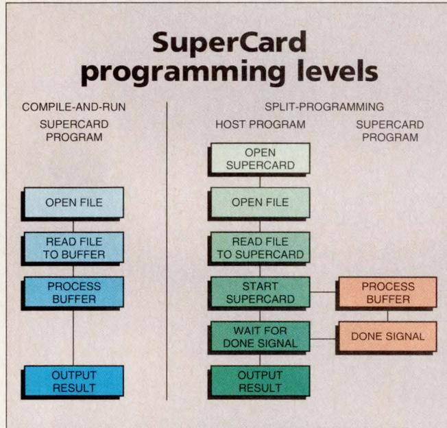
CSPI offers two levels of programming for its SuperCard, depending on the speed-up desired and the level of effort to be expended. The compile-and-run mode lets designers compile, link and run any C or Fortran program with few, if any, changes. For greater speed-up, it's possible to replace program loops with sub-routing calls to one of CSPI's libraries.
