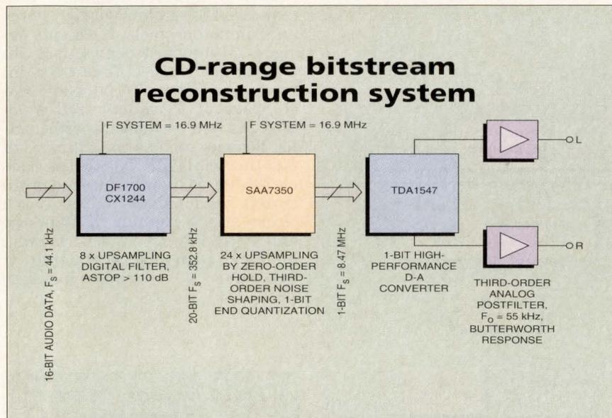
A 192 $\times$  oversampled bitstream CD system can be designed using the Signetics SAA7350 in conjunction with an 8 $\times$  oversampling filter, 1-bit D-A converter and third-order Butterworth filters.
