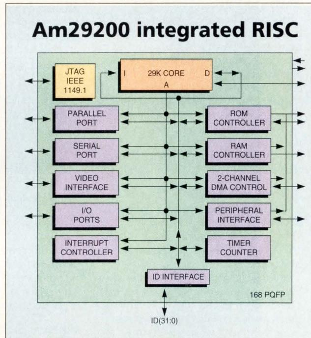
The newest member of AMD's 29000 family is the 29200 micro-processor. AMD has integrated most of the functions currently found on laser printer controller boards on a single chip in an effort to kick Motorola's 68000 out of low-cost machines.
