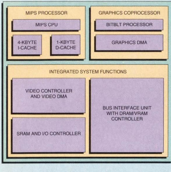
*X marks the spot where LSI Logic hopes to build terminals around the LR33020, the world's first RISC-based X windows terminal controller. LSI Logic has integrated most of the peripheral control circuitry needed to build X terminals onto the device.*
