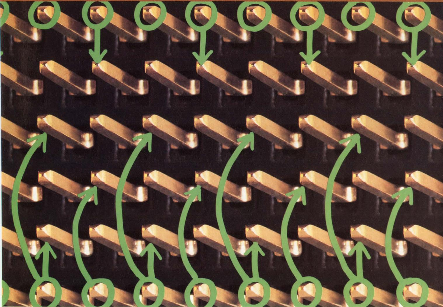
AMP TBC Plus connectors give you complete freedom in ground and signal assignment, so you can write your own 'ground rules' for outstanding electrical performance in high-speed, high-density backplane applications.
