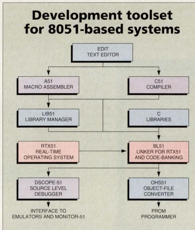
The complete set of Franklin development tools for 8051-based systems includes the RTX51 real-time executive and a simulator/debugger that lets designers simulate almost all derivatives in the 8051 family.
