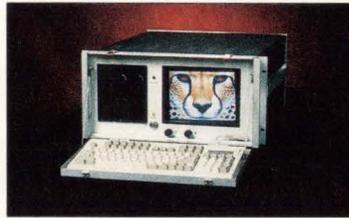
RUGGED AND HIGH PERFORMANCE COMPUTER SYSTEMS WITH FOLD DOWN KEYBOARD AND VGA MONITOR FOR RACK, BENCH OR PORTABLE APPLICATIONS
