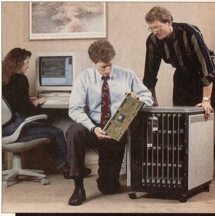
*Logic Modeling's family of hardware modelers let users on an Ethernet network access multiple devices simultaneously. "Memory in the system is dynamically allocated," says Pete Jaeger (standing), model development manager. "This lets multiple users sample a device's behavior and return to their simulation environment while others access the device."*
