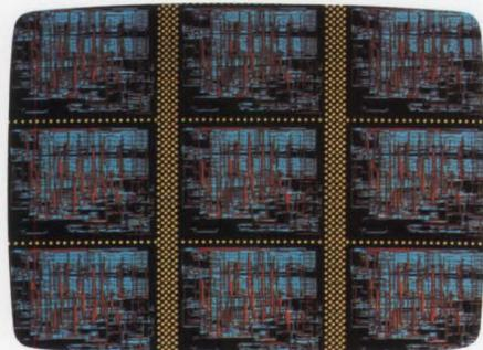
DAZIX CAM workstation contains a powerful set of features to panelize and prepare PCB designs for all manufacturing processes—photo tooling, fabrication, assembly and test to meet diverse data requirements.
