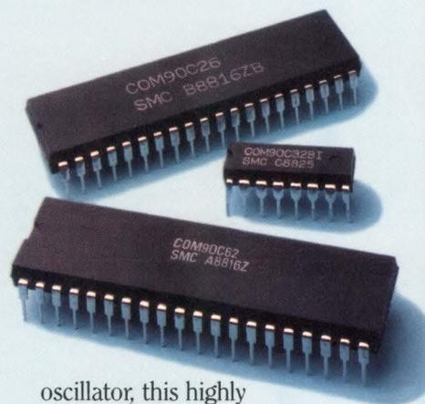
oscillator, this highly integrated IC contains all the logic necessary to control a token-passing ARCNET interface across standard coax, twisted pair or fiber optic cable. The COM90C62's high level of integration allows inclusion of a LAN interface directly on a PC mother board.
