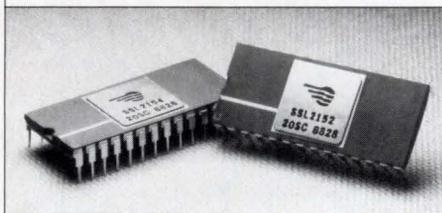
TTL-compatible inputs/outputs, are cascadable in memory depth and word width, and feature a ninth bit to handle parity checking. To accommodate different system requirements, the SSL2152 has totem-pole "Match" output, while the SSL2154 has open-drain "Match" output for OR-tying with an external pull-up resistor. Both parts feature on-chip parity-generation and -checking capability, parity-error output, and forced-parity-error input. Prices for both devices start at \$56.
