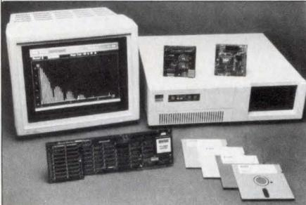
contains up to 96 kwords of zero-wait-state memory, interface circuitry for the I/O modules, and direct memory access capability for transfers to and from the PC's memory. A broad line of software is available for the DSPPro line. DSP Library Plus offers a large selection of software routines that are callable from programs running on the PC.
