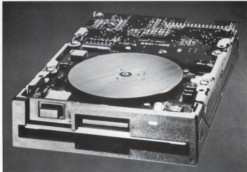
tion. The dual-mode (1- or 2-Mbyte) device uses phase-correction circuitry combined with a wide gap head for full compatibility with conventional 1-Mbyte drives.
