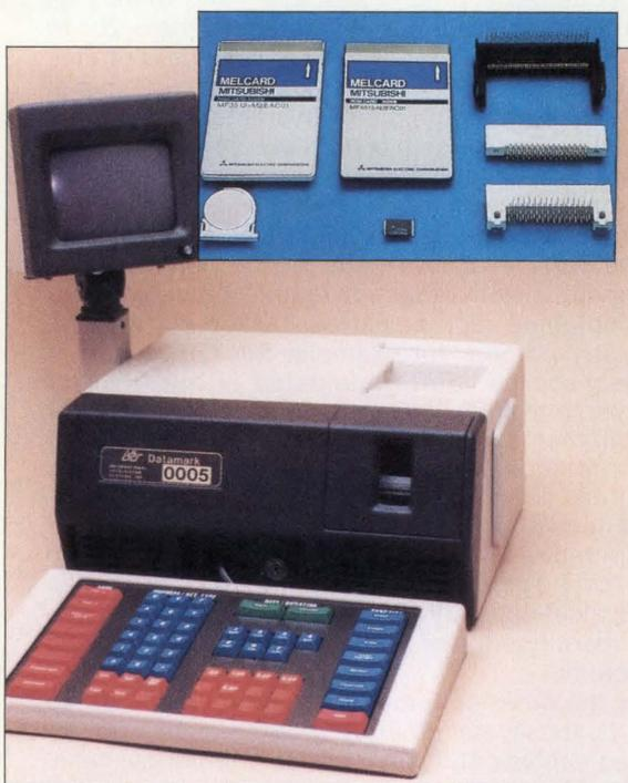
Melcard memory cards from Mitsubishi can store up to 512 kbytes of static RAM, one-time programmable ROM or masked ROM. Cards and connectors are available with 8- or 16-bit-wide data paths and with two styles of connector: pin or shielded edge connector. One system that uses the Melcards is a lottery terminal made by International Totalizer Systems. Data entered at a local store can be removed by means of the Melcards and taken to a central processing facility for each lottery drawing.
