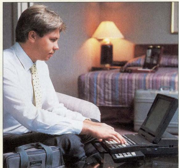
The addition of optional numeric keypads to laptop computers such as the Mitsubishi mp286L extends keyboard functionality to desktop levels. With the keyboard-keypad combination, compound actions on the base keyboard alone can be accessed with a single dedicated key.
