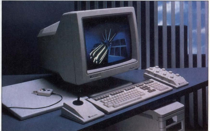
4,096 colors from a palette of 16.7 million. Shaded solids are rendered as flat or shaded surfaces using Phong or Gouraud shading algorithms. In addition, the 9300 supports rational cubic B-splines, which render curves according to their true mathematical definition, rather than as a series of vectors, and curved surfaces as true curves rather than a mosaic of polygons.
