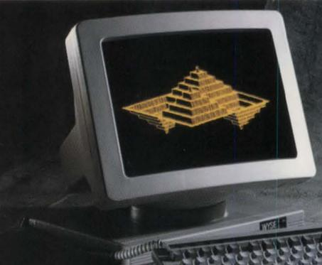
The WY-99GT terminal is shown with a screen displaying a 3D pyramid graphic and a keyboard in front of it.
