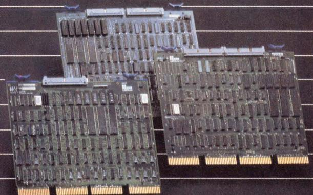
1/2" TAPE—CONTROLLER/COUPLER PERTEC I/O
