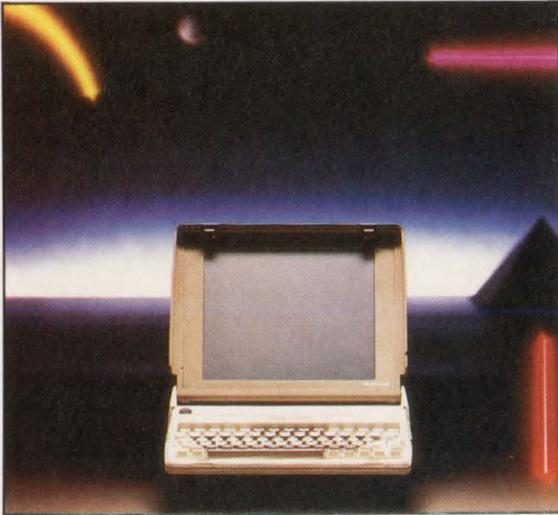
Smaller than a briefcase and weighing only 9.1 lb, Data General's One personal computer is operationally compatible with the IBM PC. It runs the MS-DOS and CP/M-86 operating systems using a 4-MHz 80C88 CMOS microprocessor. The unit's LCD shows a full 25 lines of 80 chars on a screen. Double 3½-in. disk drives located at the side of the keyboard/chassis, provide up to 737 Kbytes
