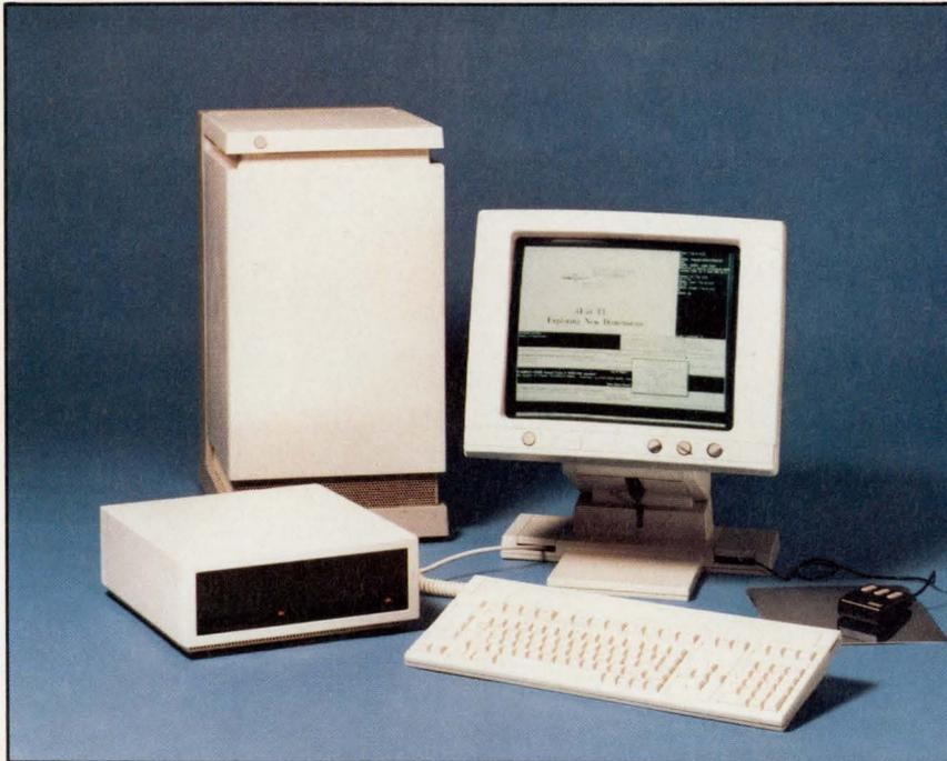
The smallest, dedicated symbolic processor presently available, TI's Explorer includes 5¼-in. Winchester disk drives, a high resolution monitor, and a keyboard that includes Lisp specific keys.
