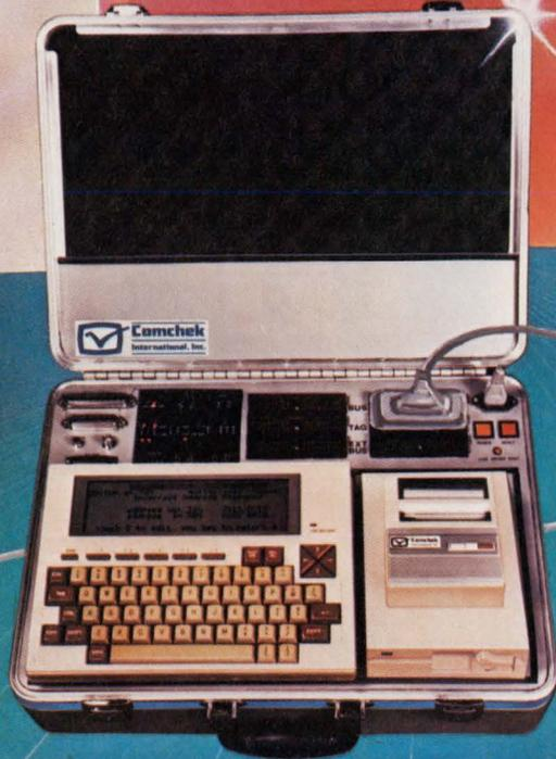
Comchek's Channel Simulator. The ideal tool for simulating the operation of the standard I/O channel on IBM® 360, 370, 4xx or 30xx computer systems from just one location.
