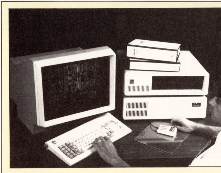
Enhanced graphics, achieved in the Daisy Personal Logician through the use of a graphics processor, a larger monochrome or color monitor, and an Ethernet link to the local area network, turn the IBM PC into a powerful workstation.
