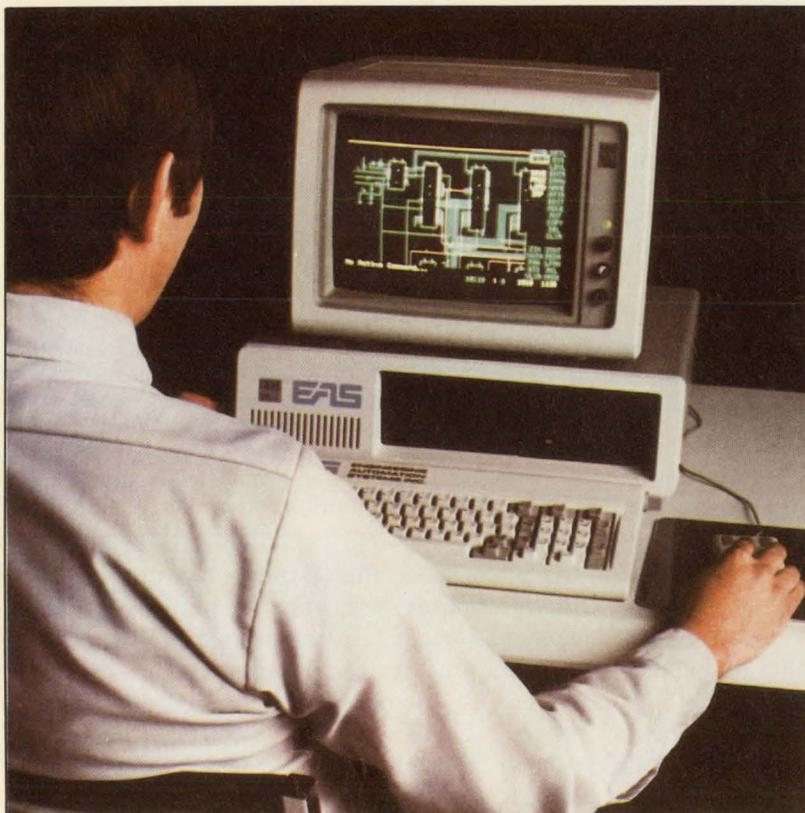
Automated checking of design rules and verification of system logic are typical of personal computer design systems. This system from EAS and P-CAD provides complete printed circuit board design, from the initial layout to the finished product.
