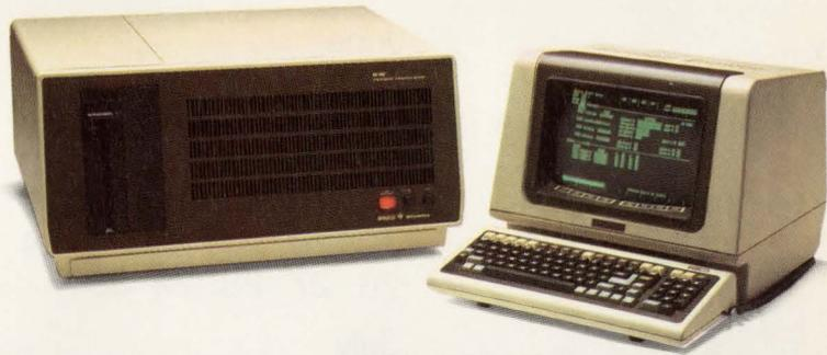
*The Gould 9516S Microsystem Integration System supports any combination of 68000, 8086, 8088, Z8001, Z8002, 68B09E, 8085A and Z80A microprocessors. It includes a 1 megabyte thinline double-density, double-sided floppy disk drive. Its RS-232-C port lets you interface with any minicomputer for fast, effective software development.*
