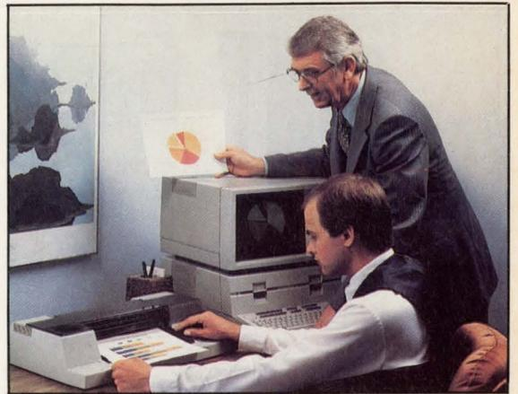
pen acceleration. Each velocity axis is programmable from 1 to 38 cm/s in 1-cm/s increments.
