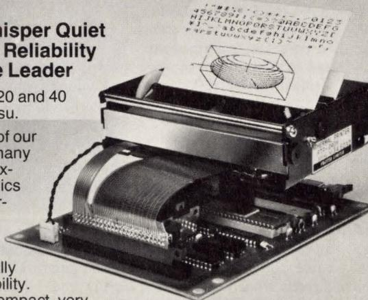
The result is a perfect printing component for applications such as in measurement and analysis equipment. In personal computers and P.O.S. terminals. And as an auxiliary printer.
