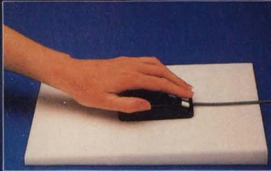
GTCO's patented digital electromagnetic scanning—with no mechanical parts—lends itself to operation in office and industrial environments that cripple an optical or mechanical mouse.
