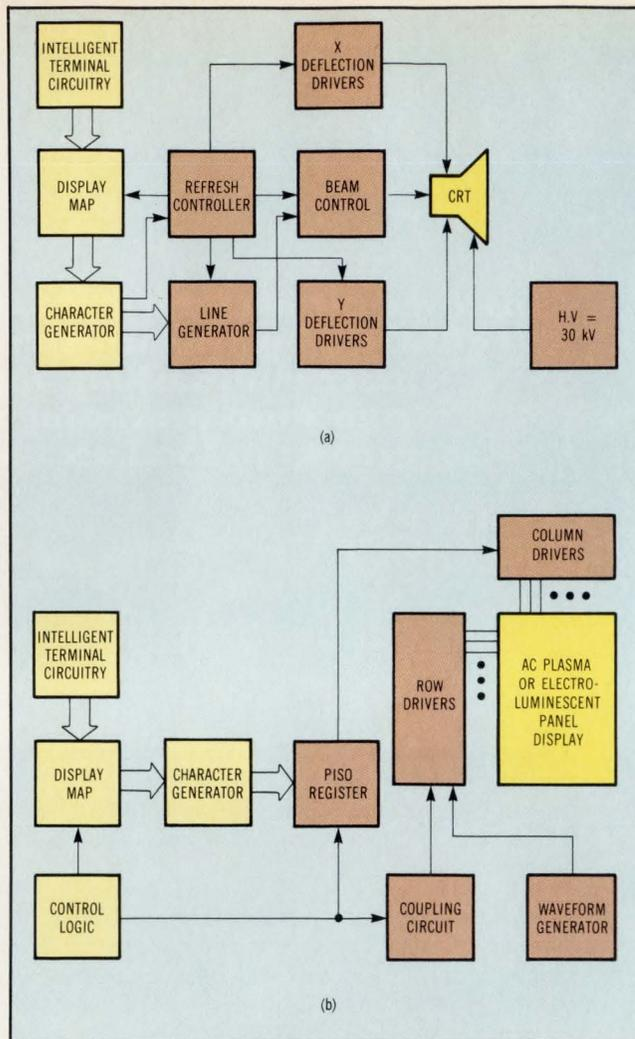
**Fig 3** Circuitry for CRT displays (a) differs significantly from that of ac plasma or electroluminescent displays. The required high voltage power supplies also add weight and bulk. The ac plasma and electroluminescent circuits (b) differ mainly in the types of row and column drivers used (SN75500 and SN75501 for the plasma display; SN75551, 2 and SN75553, 4 for electroluminescence), and in waveform generator voltages (100 V for plasma, and  $\pm 200$  V for electroluminescence).
