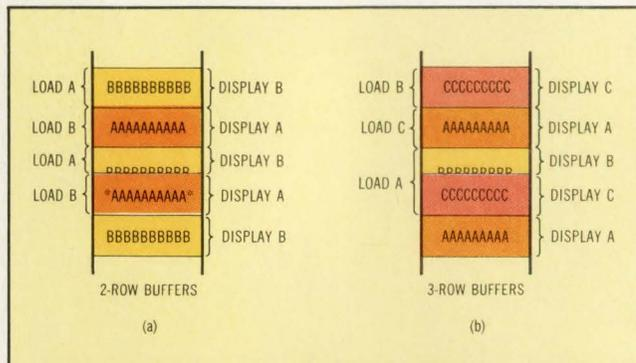
**Fig 3** For split-screen scrolling applications, a character row could be displayed for only a single scan line. With two row buffers (a), this does not leave enough time for the reloading of the alternate row buffer, which results in a flashing screen. With three row buffers operating in a rotating fill-display mode (b), any single row buffer can be displayed for one scan line without any danger of screen flashing.
