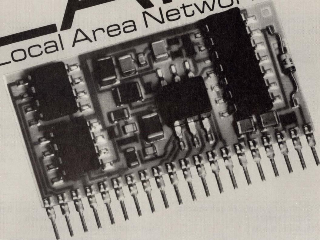
The Zenith LAND Hybrid (Local Area Network Driver) is a cost-effective, highly reliable interface for baseband LAN's including Datapoint's ARCNET<sup>™</sup>, and other compatible systems.
