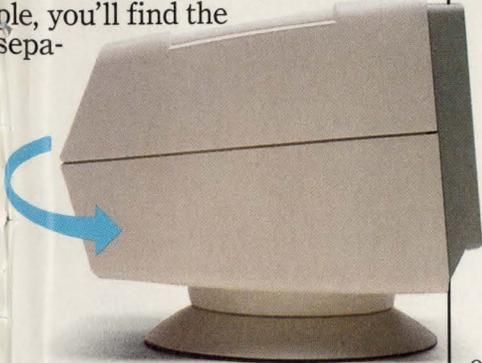
Monitor tilts and swivels to almost any position. Both models available with 12 or 14 inch screens.
