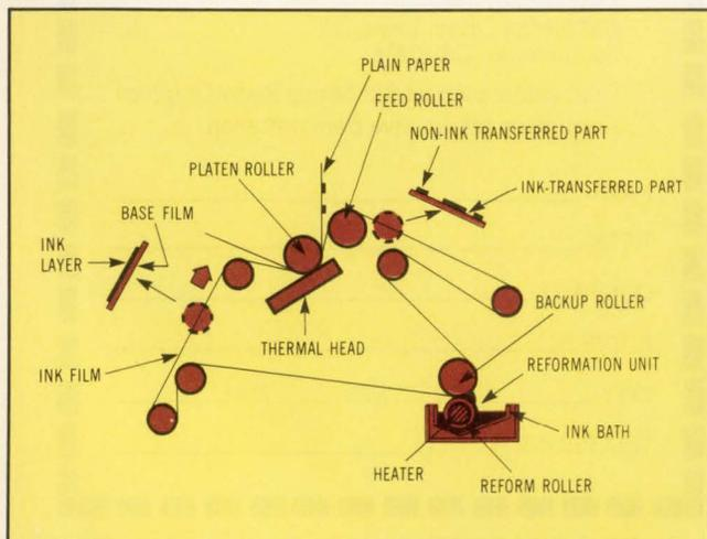
**Fig 7** Oki's plain-paper thermal transfer printer uses an ink film in an endless loop, while the ink is selectively melted by heat elements of the thermal head and transferred to the paper. Ink remaining on the film is remelted in the ink bath by the reform roller, which again supplies a uniformly thin 5- $\mu$ m ink layer on the film for the next cycle.
