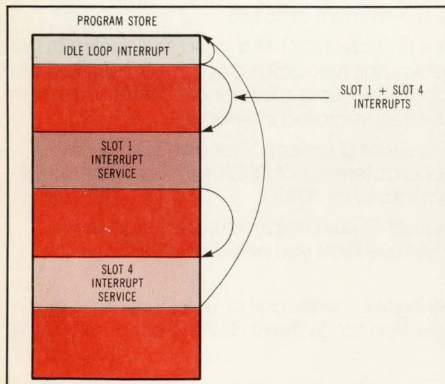
**Fig 4** Interrupt overhead is kept minimal by using low priority idle loop default. When higher priority interrupts occur (slot 1) they are serviced immediately. The last service routine instruction enables all interrupts and initiates processing of the next interrupt (slot 4).
