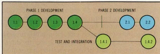
**Fig 5** Use of SCCS during development permits the original version (1.1) and the changes to be kept, rather than keeping copies of each version—a net disk space savings results. Only one user can access and change a file at any given time; all others must wait. SCCS also provides file management reports.
