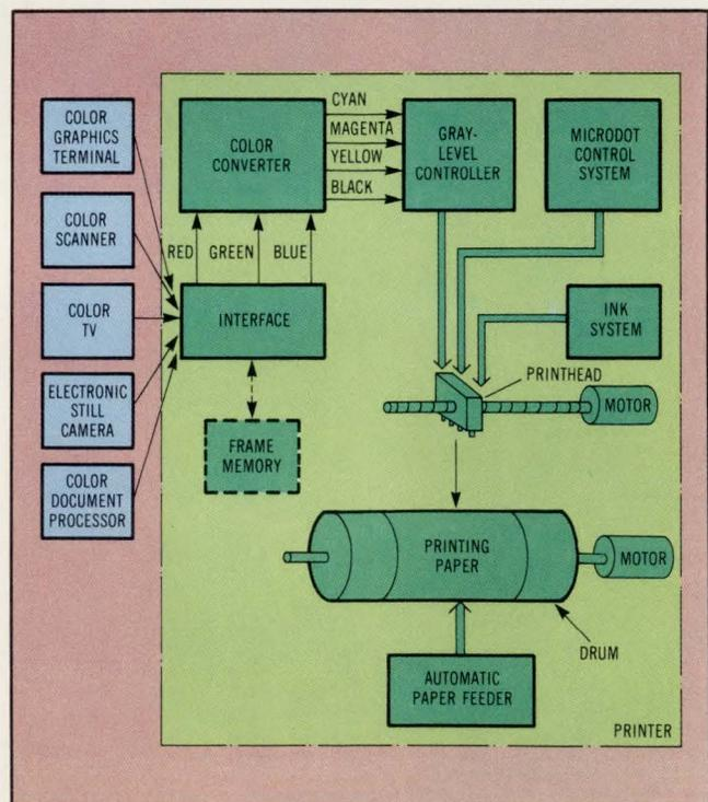
**Fig 3** Hitachi's full-color printing unit can accept color information from many different sources. A frame memory is used to retain data from a video source for reproduction. Four ink jets (cyan, magenta, yellow, and black) move horizontally across the paper as it rotates on the drum.
