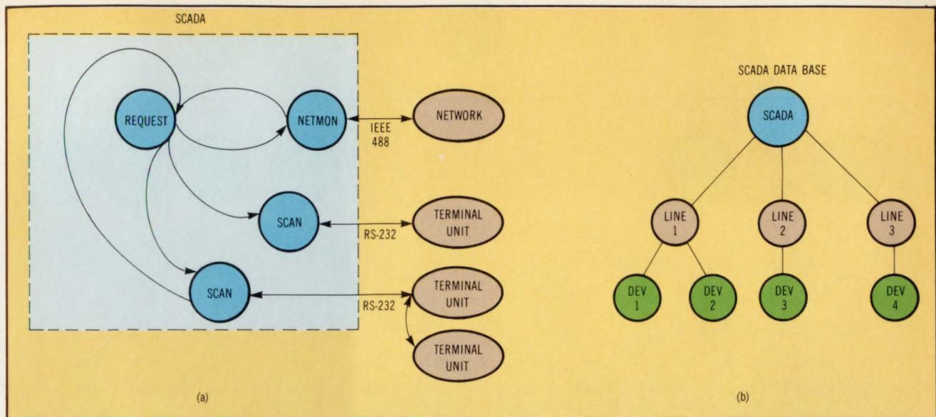
**Fig 2** The SCADA subsystem (a) manages interface devices and responds to status requests via the network. The various processes communicate through Unix pipes. SCADA, which serves as the main directory, has a subdirectory for each hardware communication line in the system (b). Each line, in turn, has subdirectories for each of the devices connected to it. These lowest level directories contain information about specific device parameters.
