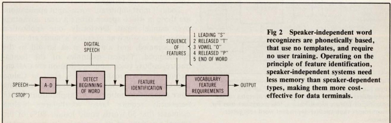
**Fig 2 Speaker-independent word recognizers are phonetically based, that use no templates, and require no user training. Operating on the principle of feature identification, speaker-independent systems need less memory than speaker-dependent types, making them more cost-effective for data terminals.**
