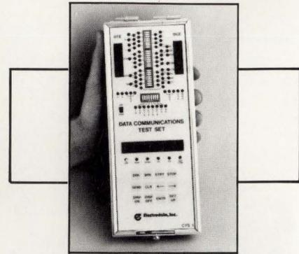
ing 1 of 8 patterns. The test set can count and display bit and block errors, blocks received, and sync faults. The CTS 1 is \$1495. **Electrodata, Inc.**, 23020 Miles Rd, Bedford Heights, OH 44128. **Circle 354**
