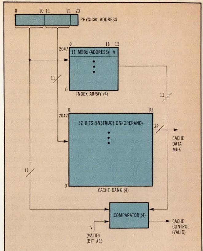
**Fig 2** The cache memory is divided into two 16K-byte banks. One bank shown consists of 2048 locations, each being 32 bits wide. The 11 most significant bits (MSBs) of a physical address are compared with 11 most significant bits from the index array to determine if a given operand or instruction is cache resident.
