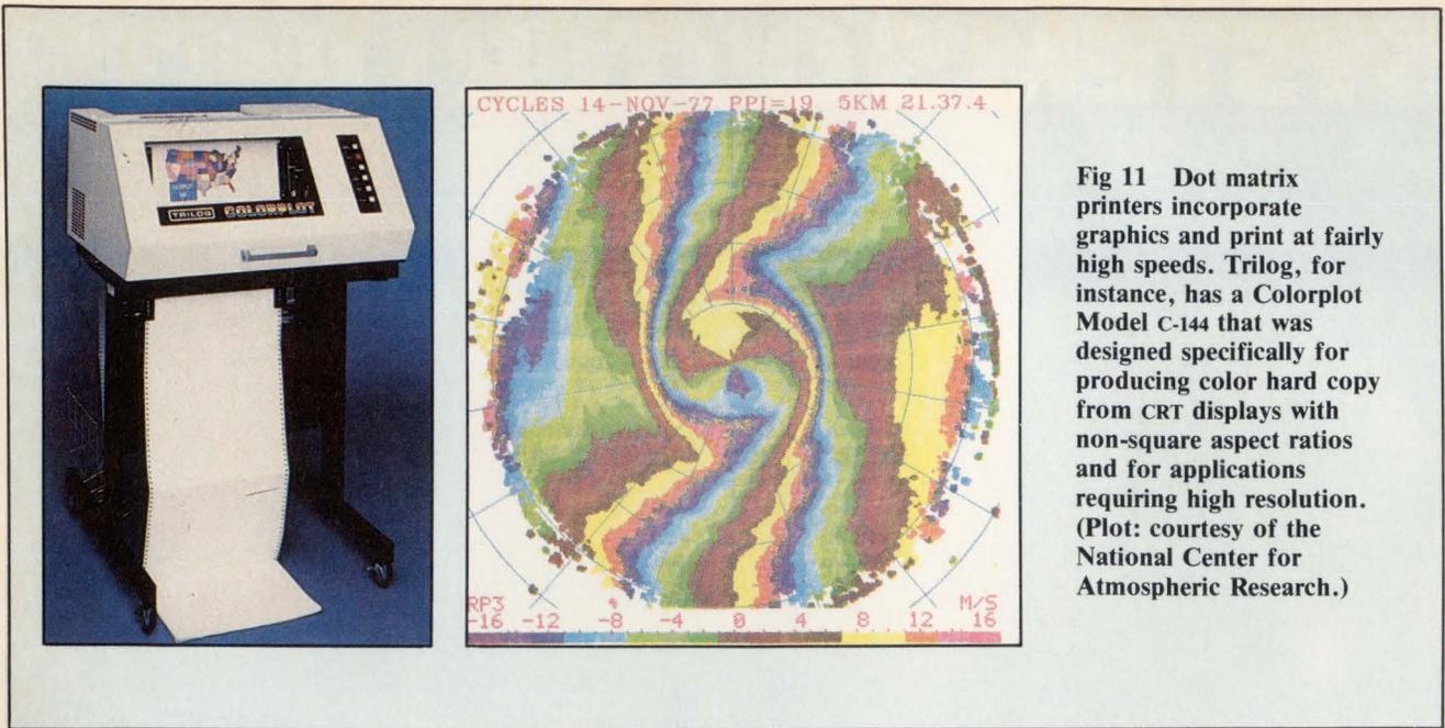
**Fig 11** Dot matrix printers incorporate graphics and print at fairly high speeds. Trilog, for instance, has a Colorplot Model C-144 that was designed specifically for producing color hard copy from CRT displays with non-square aspect ratios and for applications requiring high resolution. (Plot: courtesy of the National Center for Atmospheric Research.)
