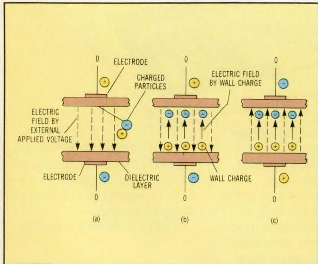
**Fig 5** To initially ionize the cell, a relatively higher voltage is required (a). Once ionized, however, ions in the panel adhere to the walls (b), creating a wall charge that makes it possible to sustain light emission at a lower voltage. Thus, the next discharge starts at a lower external voltage than the initial starting voltage (c).
