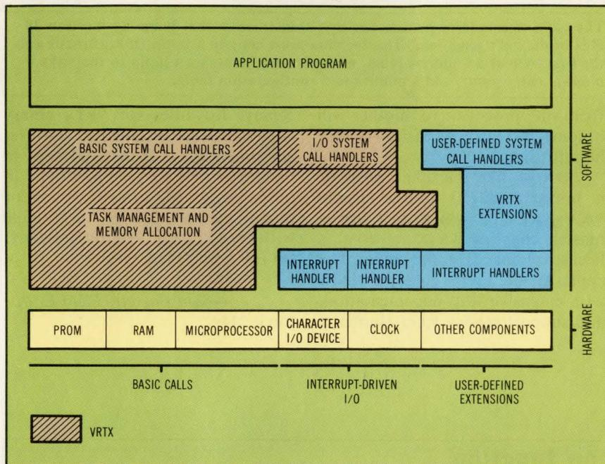
The basic VRTX system provides an interface between the application programs and the hardware on which they run. Software hooks provide the ability to build custom interrupt handlers and system call functions into the applications.
