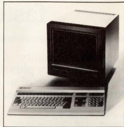
editing, memory and line lock, ASCII comm code, RS-232 interface, and transmission rates from 50 to 19.2k baud. The terminal is priced at \$1085. **Beehive International (UK) Ltd**, Index House, Ascot, Berkshire, SL5 7EU, England. **Circle 408**
