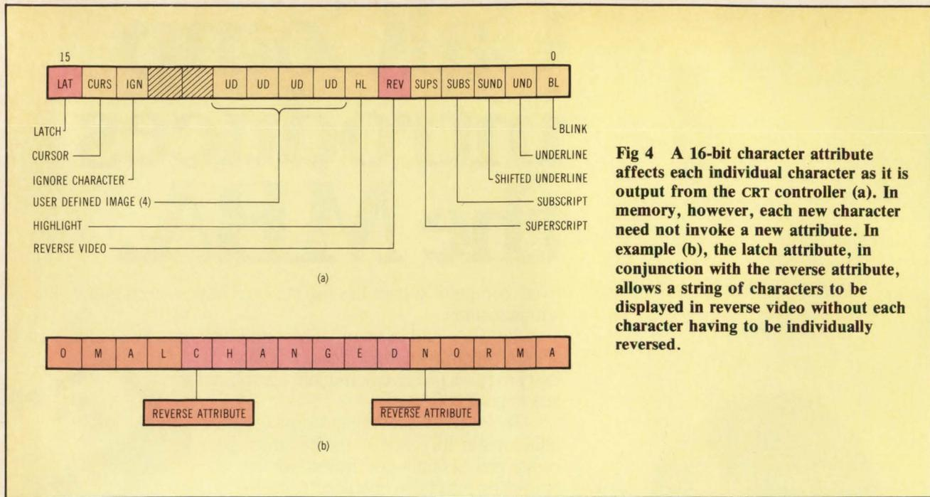
**Fig 4** A 16-bit character attribute affects each individual character as it is output from the CRT controller (a). In memory, however, each new character need not invoke a new attribute. In example (b), the latch attribute, in conjunction with the reverse attribute, allows a string of characters to be displayed in reverse video without each character having to be individually reversed.
