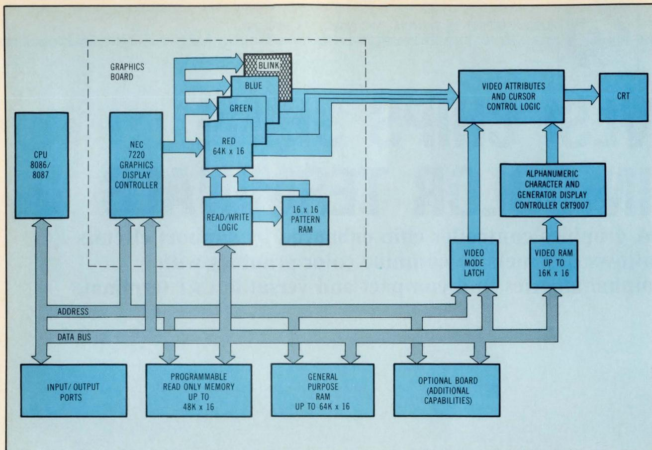
**Fig 1** Here, the CPU (an Intel 8086 with optional 8087 numeric processor) handles computation, input/output to the keyboard and other devices, and controls the video signal to the CRT. An NEC 7220 on the graphics board handles all graphical manipulations in the image planes.
