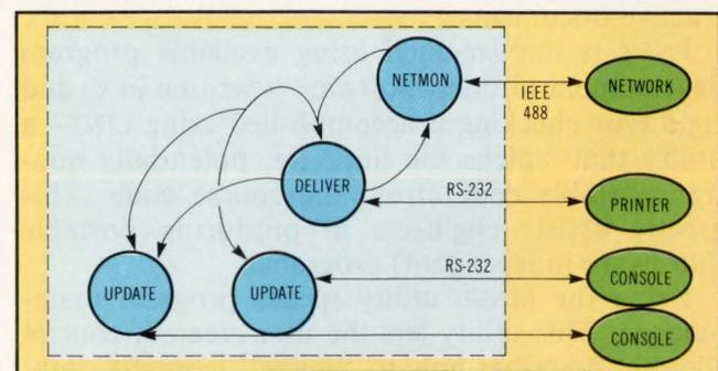
**Fig 3** MMI updates operators' consoles by issuing status requests to the network. The processes communicate through Unix pipes. Many update processes may be running, with each operator using a different display.
