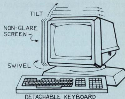
**Ergonomics:** MPC's terminals offer a non-glare screen, rotate 60° in either direction and compensate for height variations by tilting up to 20°. The detachable keyboard meets European DIN specifications.
