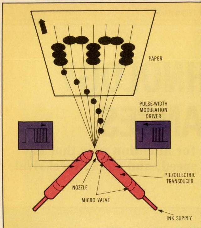
**Fig 1** A growing problem for ink-jet printer manufacturers has been the low reliability of the ink jets themselves. To increase reliability, jet number must be reduced. NEC's drop collision deflection technique uses only two jets to emit two simultaneous drops which, upon colliding, combine at a point adjacent to the nozzle orifices. Micro valves apply a constant pressure on the ink; pulse-width modulation drivers control the direction of the ink drops.
