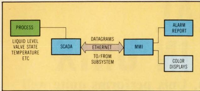
**Fig 1** The SCADA and MMI subsystems communicate via datagrams, which are sent by the 10M-bps Ethernet bus. SCADA monitors the sensors, computes measurements, responds to abnormal values, and answers queries from the network. MMI's main purpose is to interpolate the data from SCADA and update the operator's color CRT terminals.
