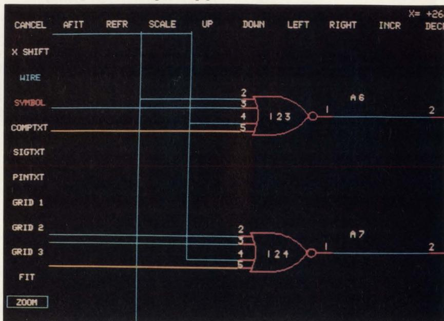
A portion of a logic diagram designed on the VIA series 100 is displayed with a portion of one signal net highlighted. When TRACE is activated, signals tied in a net are displayed in a special color.
