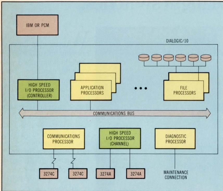
**Dialogic/One system's highly redundant architecture contains a diagnostic processor that allows dynamic redistribution of tasks if a component fails. Application processors supply local memory and processing for user operations; system processors handle system functions.**
