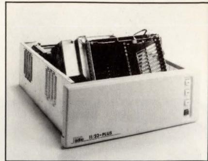
Design allows expansion of an additional 9 full-quad boards, or 19 half-quad boards, or any combination. The basic system is offered with a choice of 256K or 512K bytes of RAM. In one to nine quantity, prices range from \$4465 to \$5265. **ADAC Corp.**, 70 Tower Office Park, Woburn, MA 01801.
