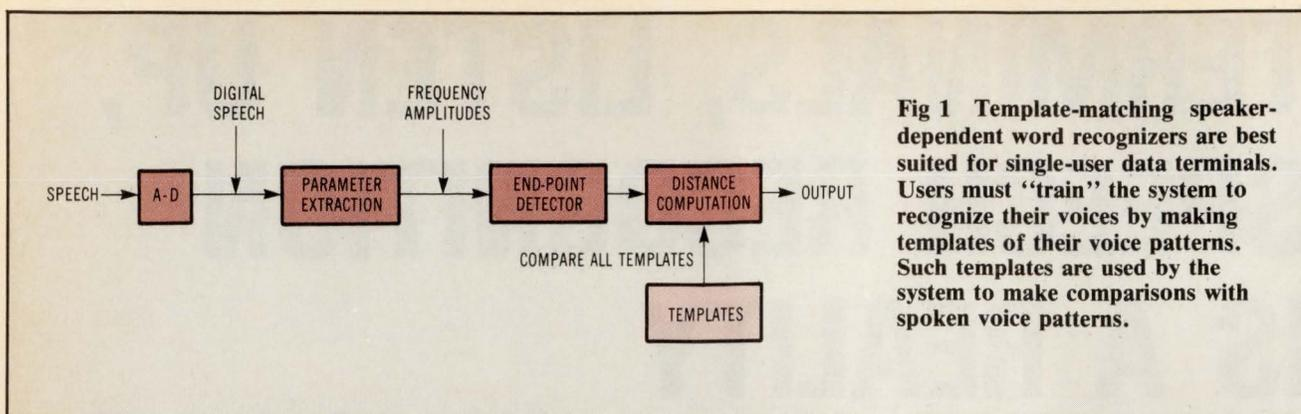
**Fig 1** Template-matching speaker-dependent word recognizers are best suited for single-user data terminals. Users must "train" the system to recognize their voices by making templates of their voice patterns. Such templates are used by the system to make comparisons with spoken voice patterns.
