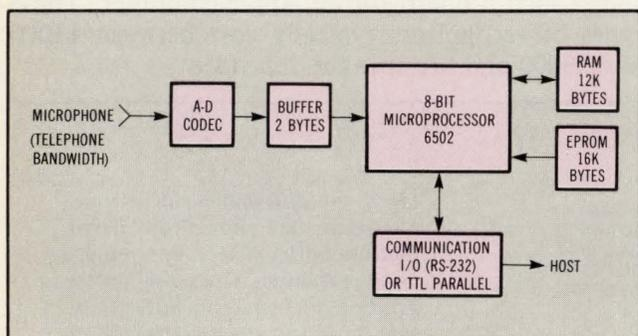
**Fig 4** An 8-bit microprocessor and a communications port form the core of Voice Control Systems' speaker-independent word recognizer. Because it operates on the principle of feature identification, this recognizer uses far less memory than speaker-dependent word-recognition systems.
