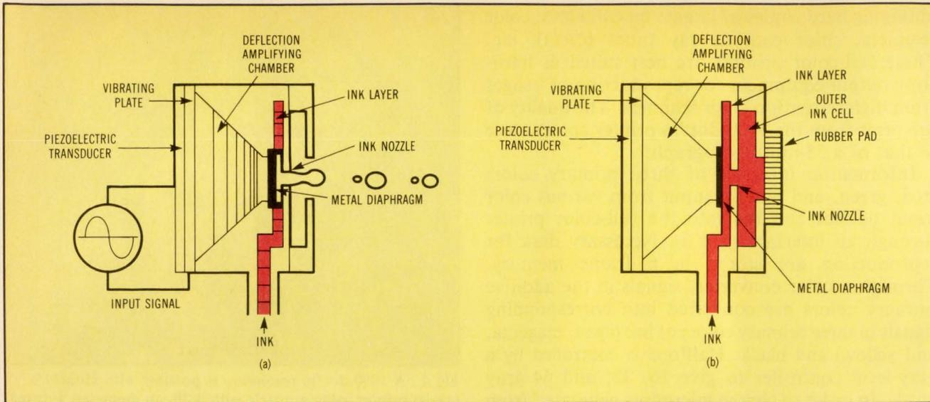
**Fig 5** A drop-on-demand printing system developed by Sanyo Electric uses a metal diaphragm to shield the outer ink cell, which is constantly filled with ink (a). This keeps the nozzle immersed in ink in the standby condition, thereby keeping the nozzle from clogging (b). When an input signal is applied, minute drops are generated that print a copy at 12 dots/mm.
