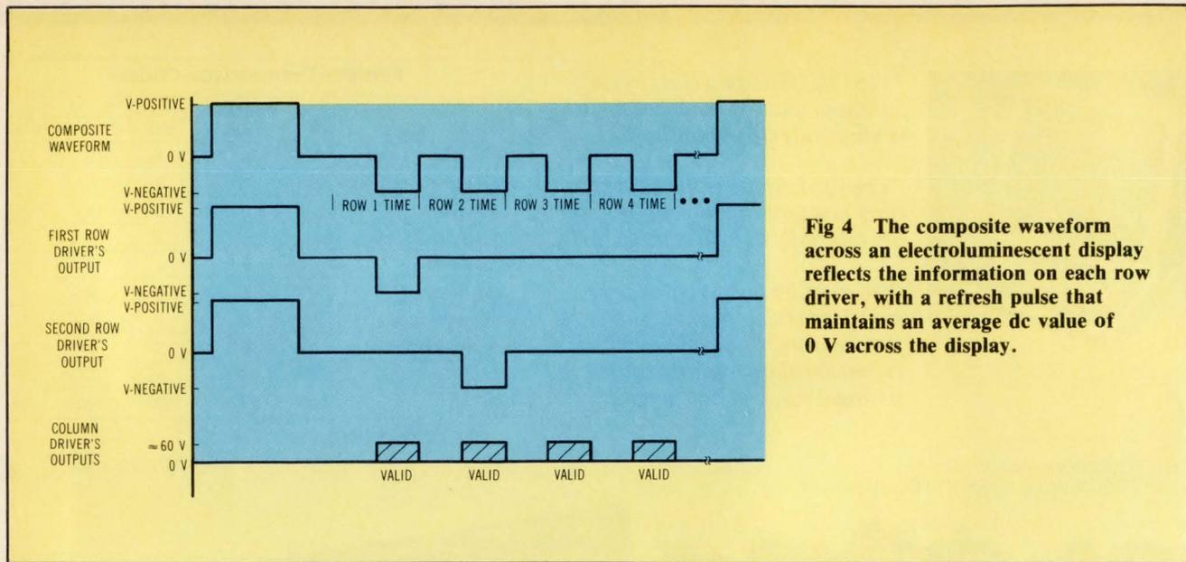
**Fig 4** The composite waveform across an electroluminescent display reflects the information on each row driver, with a refresh pulse that maintains an average dc value of 0 V across the display.
