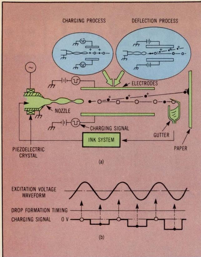
**Fig 2** Hitachi's microdot printing technique controls the dot's size and shape by having the ejected ink stream pass from the nozzle between two electrodes used as deflection plates (a). Dot size is controlled by applying a variable excitation voltage that stabilizes the formation of an optimal dot pattern (b). Microdots alternate with large drops, and charged microdots are deflected to the paper while uncharged drops fall into the gutter.
