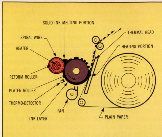
**Fig 6** A breakthrough in thermal transfer printers by Oki Electric in 1981 was to use a second roller with an internal heater to melt the ink, thereby applying a uniformly thin layer on the surface of the platen roller. A heat detector senses proper ink temperature, while a microcomputer adjusts for proper heat and airflow from the fan. The printer, however, requires specially treated paper.
