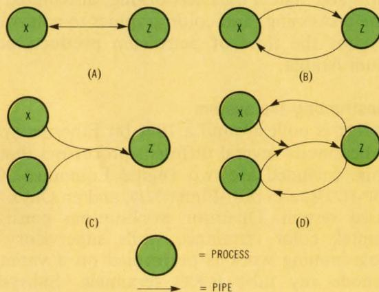
The first example (A) illustrates how one process uses a pipe to send data to another process (1-way communication). Example (B) depicts how the same two processes accomplish 2-way communication. A useful feature of pipes is that the write-end can be connected to many processes simultaneously. Unix thus guarantees that any message written by any one of those processes arrives at the read-end intact.
