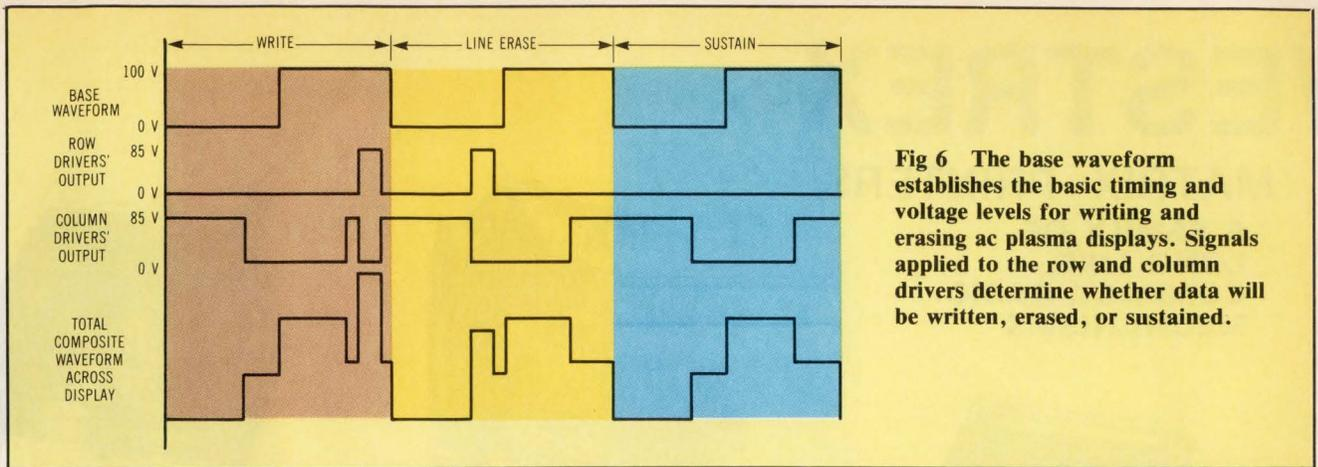
**Fig 6** The base waveform establishes the basic timing and voltage levels for writing and erasing ac plasma displays. Signals applied to the row and column drivers determine whether data will be written, erased, or sustained.
