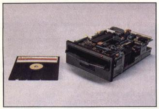
TC 500 Drivette accommodates smaller  $3\frac{1}{4}$ " form factor media. Low cost goals are met by manufacturing the drive of snap-fit parts and by using a traditional soft jacket on the diskette.
