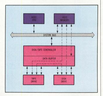
Fig 4 A combined intelligent disk/tape controller includes data buffers within its confines. Now, the host bus is only used for issuing commands to the controller. Thus, the host retains access to its program and memory before, during, and after all data transfers. Winchester disks, streaming cartridge drives provide users with a functional and flexible tool suitable for backup, archival storage, program and data transportation, and personal data security.
