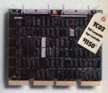
Coupler works with all NRZI, PE, GCR formatters at speeds from 12.5 to 125 ips.
