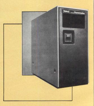
Typical backup times range from 6 to 35 min. Output ratings are 400 and 800 VA. Noise attenuation begins at 10 kHz and is 40 dB minimum over 100 kHz. Transfer time from power line to inverter is 4 ms typ, 10 ms max; for inverter to power line, 2 ms typ, 4 ms max. *Topaz, Inc, Electronics Div,* 3855 Ruffin Rd, San Diego, CA 92123. See at Booth N3539 Circle 209
