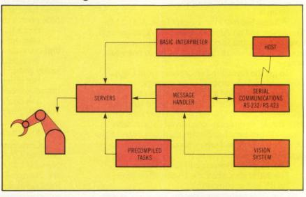
Robot servers, which control the Model 3030's manipulator, take their input from the BASIC interpreter, from precompiled tasks, or via a message handler. The message handler transmits commands from a host computer and also allows the vision system access to robot control.
