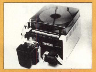
connect to a keyboard send/receive printer to provide automatic send/receive capabilities, or be used standalone. The unit punches and reads fanfold tape and senses low tape supply and tight tape. *Trend-DLC, Inc,* 280 Midland Ave, Saddle Brook, NJ 07662. See at Booth N4307 Circle 273
