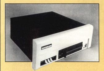
A22 systems contain an 8'' RX02 compatible floppy drive and a 10.4M-byte RL01/RL02 compatible 5<sup>1</sup>/<sub>4</sub>" Winchester drive. Software compatible with RT-11, RSX-11, RSX-11M, RSX-11 PLUS, UNIX, and TSX-PLUS, the 7" (17 cm) high microcomputer is supplied in either a rackmountable configuration or a desktop version. The chassis contains an 8-quad slot Q-bus card cage that accommodates standard DEC dual or quad boards.
