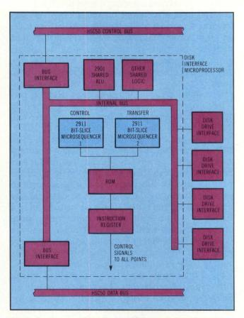
Fig 3 In the second level of parallel processing, the tasks of each disk interface microprocessor are divided between dual microsequencers. Microsequencer #1 handles the control functions involved in data transfers, and microsequencer #2 is dedicated to the actual realtime transfers.
