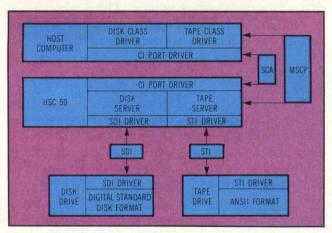
Fig 5 Layered software architecture offers maximum flexibility in connecting DSA disk and tape drives to CI buses. The software establishes a virtual circuit between the HSC50 node and the CPU node on the CI bus.
