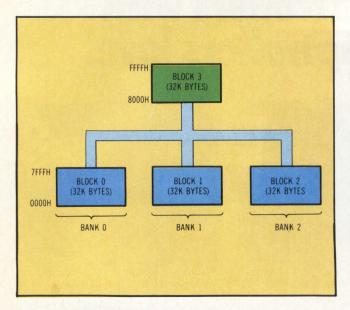
Fig 2 The CPU switches memory banks by selecting a 32K-byte block that fills low order addresses. The alwaysenabled common block contains routines to pass control and data between banks.
