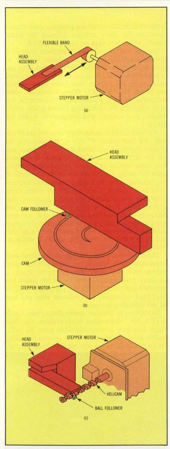
Head positioning mechanisms. Key to the accuracy needed for higher track density diskettes such as the sub-5" units, the flexible band positioner (a) claims to supply the fastest, most accurate positioning. Spiral cam (b) and lead screw (c) positioners are also commonly used.
