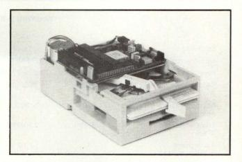
Varying the spindle speed as the recording head moves from inner to outer tracks lets IBM put data down at a constant 6865-bpi density. This method packs 358 bytes onto the single-sided 4" diskette's 46 tracks.
