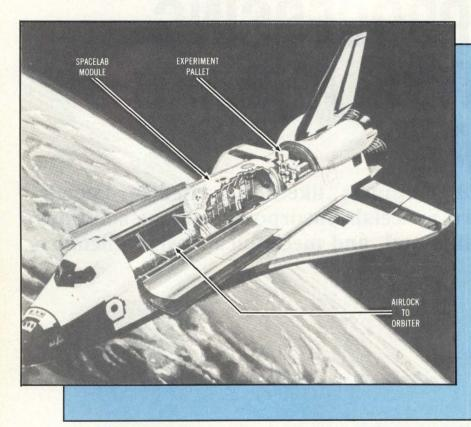
Photo 1 Spacelab, shown with long module and one experiment pallet installed in Orbiter cargo bay, can also be configured without a module. The SC-1 computer resides on the equipment pallet.
