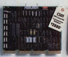
Handles 8-64 channels, 16-bit word transfers (DMA), 22-bit addressing. (16-channel price)
