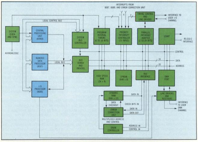
Fig 1 Block diagram of SC-1 computer shows arrangement of 8086, 8087, and 8089 VLSI processors on the local bus. The computer is equipped with 128K bytes of fault tolerant DRAM, up to 128K bytes of EPROM, timers, interrupt controllers, and ample 1/0.
