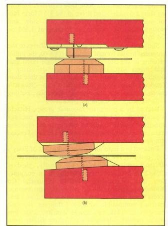
Double-sided recording heads. In a typical recording head (a), the top side is pressed against the medium by another directly opposing head on the bottom side. Drivetec's gumball head configuration (b) rounds the edges and offsets the heads to reduce media wear.
