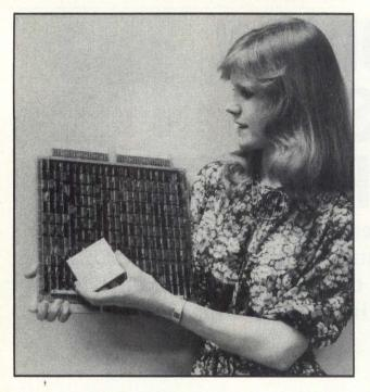
Photo 1 Compact micropackages containing Honeywell's current mode logic chips hold as much logic as all transistortransistor logic dual-inline packages on a large printed circuit board. The result is high concentrations of heat that must be quickly and efficiently dissipated.
