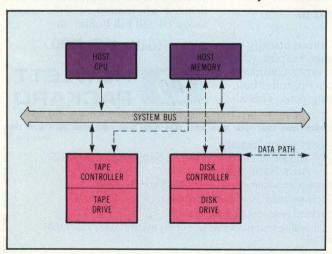
Fig 2 In a data buffer architecture using host memory, all communication takes place over the host bus. This may lead to serious contention problems, slowing overall throughput. Worse still, valuable host memory is usurped by buffer space.
