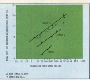
Fig 2 The graph shows radiation characteristics of various logic families, particularly the improvement in radiation resistance of newer devices. This improvement is attributed to thinner gate oxides and lower precise temperatures.
