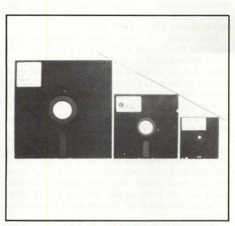
The  $3\frac{1}{4}$  " medium used in Tabor's Drivette is one-fourth the size of familiar 8" diskettes, yet holds half as much data using current technology. Capacity of the  $3\frac{1}{4}$  " medium is equivalent to that of  $5\frac{1}{4}$ " floppy media.
