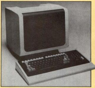
Standard equipment for the terminal includes the programmable function keys and 5 video attributes that can be used in any combination without a character space. Other features include a detached keyboard with LEDs, built-in tilt mechanism, and 2-speed smooth scroll. Characters are displayed in a 7 x 9 matrix with true descenders on a green, non-glare screen with screen saver. Amber phosphor is also available.
