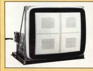
VR-1000 provides 100-lpi resolution in both vertical and horizontal dimensions with up to 8 levels of intensity. The raster scan monitor displays up to 1100 noninterlaced lines refreshed at 60 frames/s. The displays run at a pixel level of up to 100 MHz. A display of 1024 x 1024 is attained.
