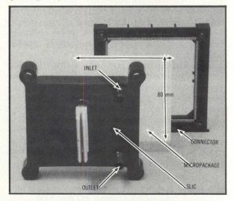
Photo 2 Shown are the basic elements of a silent liquid integral cooling assembly. SLIC provides efficient heat transfer from a micropackage to circulating water via a dry interface.
