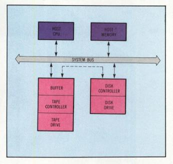
Fig 3 A buffer architecture that places data buffers in the tape controller eliminates problems involved in host memory buffer schemes. Data transfers still use the host bus, however, and contention problems remain.
