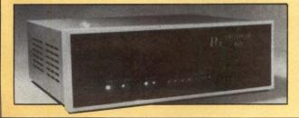
PCI 1076, an ASCII to 3270 SNA/SDLC protocol converter, lets personal computers, portables, microcomputers, and other devices including CRTs and printers communicate on a mainframe network. It connects to the host directly or by dial-up, allowing access to the host from virtually any location with a telephone. Up to 7 terminals can attach to one converter. *Protocol Computers, Inc*, 6150 Canoga Ave, Suite 100, Woodland Hills, CA 91367. See at Booth D2008 Circle 234
