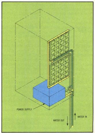
An example of a board and power supply arrangement within a main cabinet. A parallel flow scheme serves to equalize pressures within the cooling system.
