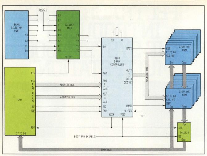
Fig 1 In a simple banked memory system, output port and multiplexer transform a 16-bit CPU address into 17 or more bits for extended memory array.
