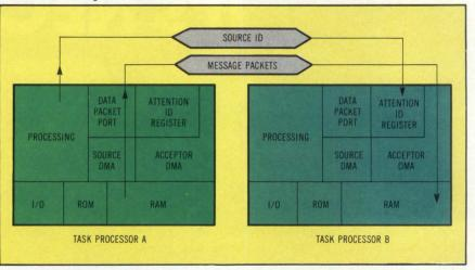
Rather than relying on shared memory, the Metacomp MPA-2000 transfers messages from the source memory (task processor A) to the acceptor memory (task processor B). The source initiates a transfer by passing the source ID number to the acceptor's Attention ID register, generating an interrupt in task processor B.
