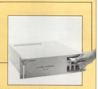
Model 8911 programmable IBM channel interface provides direct connection to an IBM mainframe as well as Ethernet hardware and software on the outboard side. Two versions of Ethernet drivers are currently available. The first implements Stop and Go Error Control Protocol. With the second protocol, data throughput rates of up to 200k bytes/s can be achieved if the receiving node supports expedient acknowledgment.
