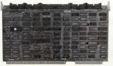
Xylogics 450 Multibus Disk Peripheral Controller.
