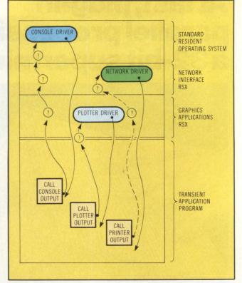
Fig 4 Resident system extensions modify OS functions. The left-most arrow traces control flow between modules for a standard function. Question marks represent decision points where either processing occurs or control is passed on. Dashed arrow illustrates the network RSX intercepting what would normally be a standard OS function call.
