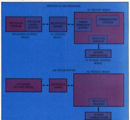
The modular architecture and common interfaces of the XNS approach limit the amount of modification needed to adapt to changing computers, operating systems, and LAN configurations.
