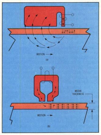
Vertical versus longitudinal recording. To squeeze more bits into a linear inch, vertically oriented media stand magnetic particles on end (a), whereas longitudinal methods lay them on the substrate's surface (b).
