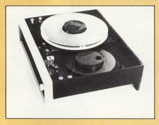
archival data storage. It accommodates both 81/2" (22-cm) and 7" (18-cm) diameter reels, as well as 10<sup>1</sup>/<sub>2</sub>" (27-cm) precision reels. An optional asynchronous interface is planned with internal data memory buffers for high speed DMA data transfers from host computer to drive. Standard Pertec/ Cipher interface compatibility will be offered.
