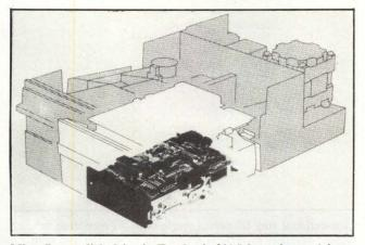
Microfloppy disk drive in Tandon's  $3\frac{1}{2}$ " form factor (photo inset) occupies one-eighth the volume of an 8" drive (shaded area), but stores more than one-half the quantity of data.
