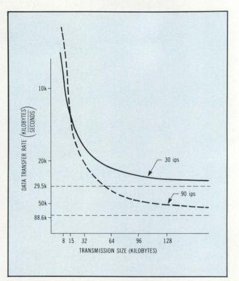
Fig 1 When streaming must be interrupted, large transmission blocks are essential for efficient 90-ips tape speed operation (dashed line). If data rates to the streaming cartridge fall below those required for continuous operation, the overhead associated with tape stopping and restarting could become prohibitive. In such cases, a slower, 30-ips speed streamer (solid line) exhibits higher throughput.
