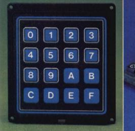
SERIES 83-84-86 Short stroke standard 3x4 and 4x4 keyboard configurations. Choice of 1/2 inch or 3/4 inch button centers and post or flange mounting. Standard coded outputseasily interfaces with logic circuitry. Excellent audible and tactile feedback
