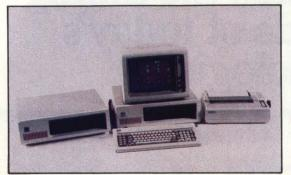
Greatly increased storage capacity, in both user memory and disk backup, is one of the advances in the IBM Personal Computer XT. A base system features 128K-byte memory, a dual-sided diskette drive with a 368,640-byte capacity, and a 10M-byte high performance fixed disk drive. Also included is an asynchronous communications adapter that enables the system to communicate with other IBM Personal Computers, larger IBM systems, and outside information sources.
