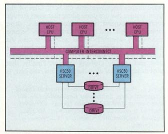
Fig 1 All CPUs linked to a CI bus have access to any magnetic disk or tape drive unit connected to a mass storage server. Two servers may access the same drives through their dual ports.
