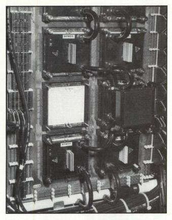
Photo 3 SLIC/micropackage assemblies are mounted in a 4 x 4 configuration on backplane boards. Flexible rubber hoses provide parallel flow paths and serve as hinges when the replacement of a micropackage is necessary.
