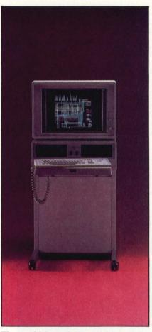
The 4115 high resolution color raster terminal incorporates a 1280 x 1024, 60-Hz noninterlaced display, a 32-bit coordinate space, and a 1M-byte/s DMA channel.
