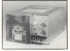
The 6010 series 750-W single-output 48-Vdc input power supply is housed in an industry std 5 " x 8 " x 11 " (13- x 20- x 28-cm) package. The supply provides output voltages ranging from 2 to 48 V with a 750-W max capability. Remote sense, thermal shutdown, foldback current limiting, and an MTBF greater than 50k hours are standard. The system is forced air-cooled and is rated at 60% efficiency. Qualidyne Systems, Inc. 2256 Main St, Chula Vista, CA 92011. Circle 400
