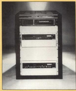
Defender verifies a user with both an ID code number and a physical location. After the system is called on any standard touchtone telephone, a digitized voice response asks for an ID code number. Once a number's validity is checked, the caller is instructed to either hang up or reenter the ID number. If the number is not successfully reentered in 3 attempts or 30 s, the system automatically disconnects and sends an alarm message to its printer.
