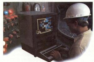
**Step 4** With the process under P.C. control, the operator may easily monitor and change process variables through the IDT display and keyboard.
