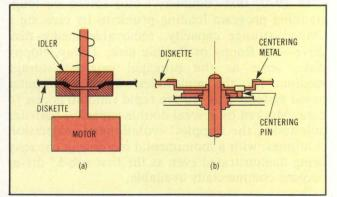
Diskette centering techniques. Typically the diskette's center hole is positioned over the spindle and is fixed into position by a mechanism that drops down on it (a). Sony's drive uses a metal hub on its diskette that contains a centering hole (b). This hole mates with a pin on the spindle to guarantee accurate centering.
