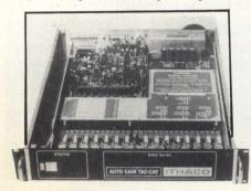
Self-calibrating features and V/F measurement technique yield 6-digit precision. Subsystem has Z80 processor and resident firmware for independent operation via attached CRT terminal. Continuous memory scanning allows immediate access to data and limit checking. **Ithaco, Inc, PO Box 6437, Ithaca,** NY 14850. **Circle 414**
