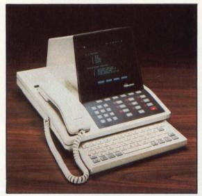
With the SL-1 Displayphone from Northern Telecom, authorized personnel have access to computerized information resources and electronic mail systems via video screen and keyboard. This integrated voice and data terminal is specifically designed to combine most of the voice and data features from earlier Displayphones with those of the SL-1 business communications system. The SL-1 can transmit asynchronous data at speeds up to 1200 bps.
