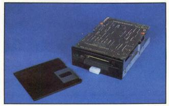
sA300, Shugart's initial microfloppy, stores 500k bytes using single-sided recording and handles data transfers at 250k bits/s. Both drive and medium conform to the Microfloppy Industry Committee's proposal.
