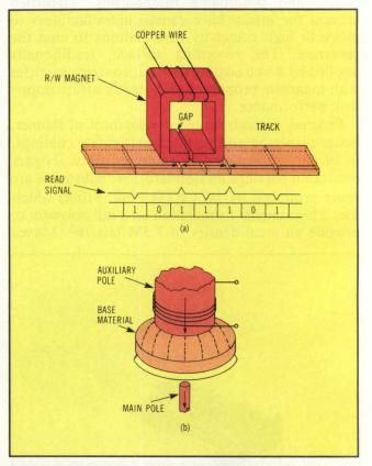
Conventional ring (a) versus single-pole (b) recording head. Higher densities in vertical media can be written and read using single-pole heads. Although capable of reading/writing vertical media, a conventional head cannot attain full potential of these media.
