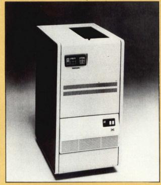
The Eagle is a Winchester-type drive that transfers data at 1.8M bytes/s. The Keystone operates at 25 ips in start/stop mode and at 25 ips and 100 ips in streaming mode.
