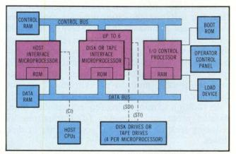
Fig 2 Parallel processing increases 1/0 throughput by dividing tasks among three types of processors. One manages 1/0, one oversees host CPU interface tasks, and one supervises a data channel to disk or tape drives. As many as four drives can connect to each of six data channels.
