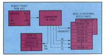
Fig 4 Execution of MSCP requests in the I/O control processor include assigning each new request ordered positions in the seek queue of the specified drive and in the rotational access table for the specified cylinder in that drive. I/O throughput is optimized by subsequent reduction of seek time and rotational latency.
