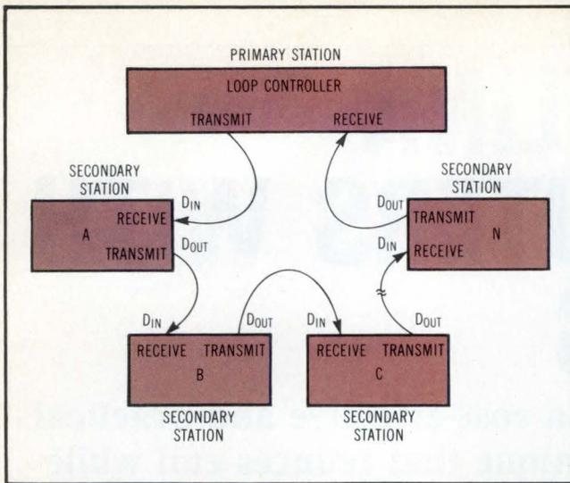
**Fig 1 Loop configuration. Loop controller on primary station repeats data, serially, to each secondary station.**
