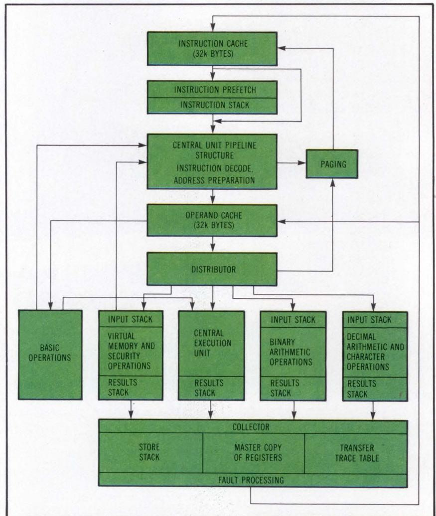
Microprogrammed central processor in Honeywell's DPS 88 uses 5-stage pipeline architecture to increase system performance. Responsible for program execution and all computation, CPU components include two 32k-byte cache memories, instruction unit, and five specialized units for executing instructions.
