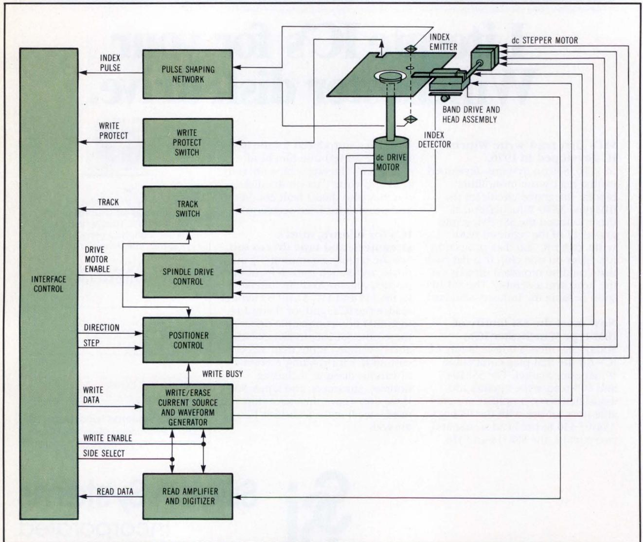
**Fig 3** Tandon TM35 microfloppy disk drive interface lines. The 34-pin edge connector used in interface provides compatibility with 5 1/4" disk drives.
