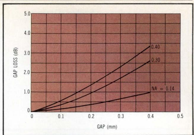
**Fig 5 Gap loss increases as function of fiber's NA and size of gap. By holding gap to 0.05 mm, energy loss from LED to fiber is only 0.30 dB.**
