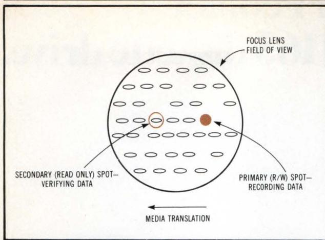
**Fig 3 The principle of DRAW data verification. Focus lens is used to form two spots at surface of storage medium. Primary high power modulated beam records data. Secondary low power CW read beam trails recording beam and verifies accuracy of recorded data.**
