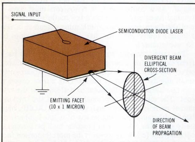
**Fig 2** Output beam from semiconductor diode laser is strongly divergent due to diffraction that occurs at extremely small region of emitting facet. Slot-shaped geometry of emitting facet gives rise to divergent beam with an elliptical cross-section.
