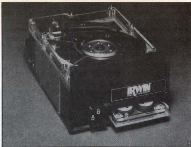
The Irwin 516 subsystem includes a 16M-byte Winchester drive and cartridge tape backup. Fitting a standard 5¼" configuration, the unit claims high storage capacity on a single platter. Average access time is under 35 ms including move and settling times.
