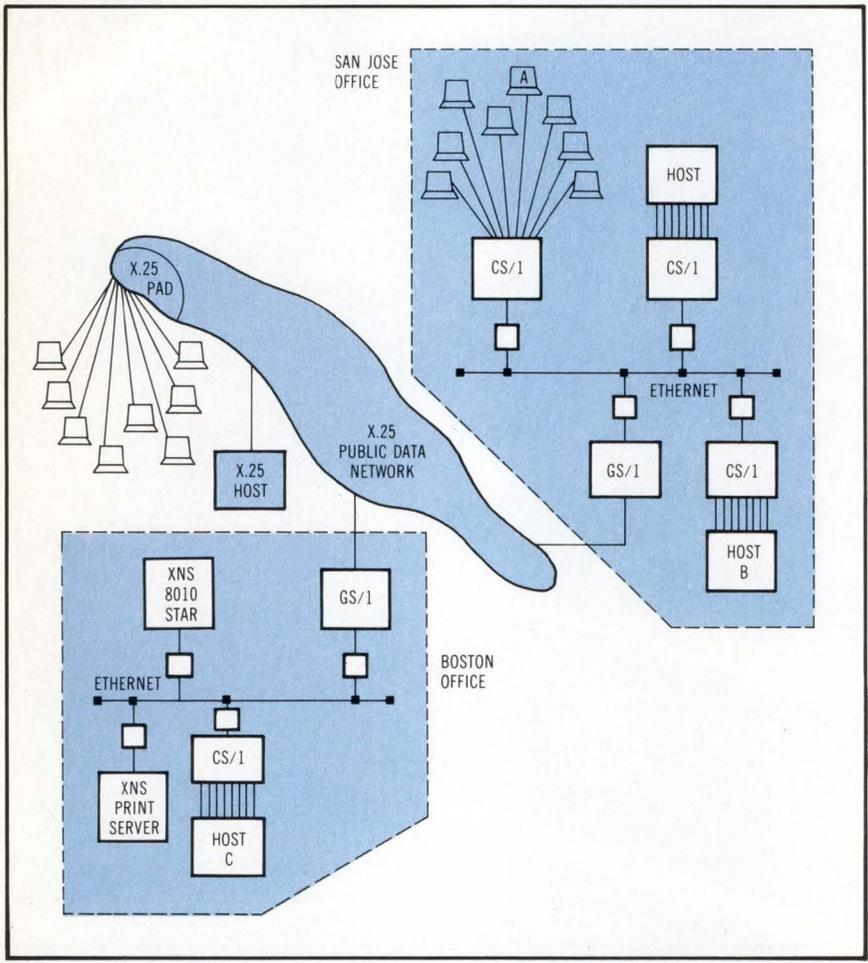
**Integrated Ethernet systems. Virtual connection can be established between terminal A and host B or C. Virtual connection supports logical name to physical address name mapping.**
