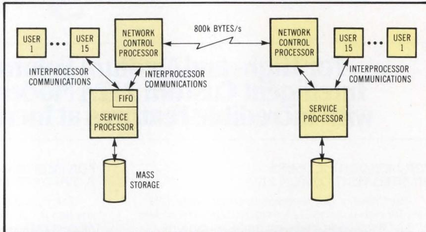
**DPC/NET takes advantage of dedicated FIFO buffers for interprocessor communications. Information passes between local user processors, network processors, and other nodes in the network via 800k-byte lines with RS-422 interfaces.**
