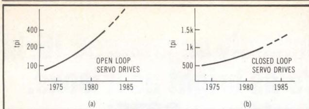
Track densities for both open loop and closed loop servo disk drives are increasing. The latter type of control system can provide higher track densities (b) than open loop types (a) since it provides greater read/write head positioning accuracy. Source: Seagate Technology.
