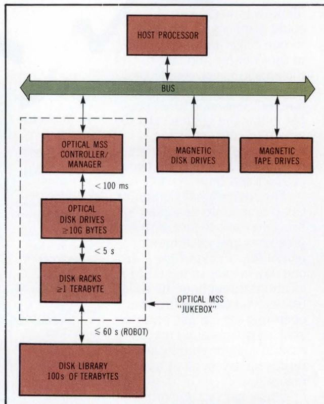
**Fig 8 Possible configuration for an optical MSS and disk library with application to extremely large data bases. Library access could be manual (offline), or automated (similar in principle to current automated tape library design).**
