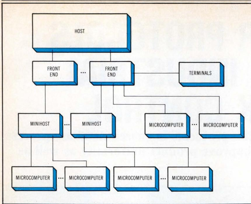
**Fig 1 Hierarchical network for manufacturing environment. Host and minihosts administer technical data that drive the microcomputer controlled manufacturing equipment.**
