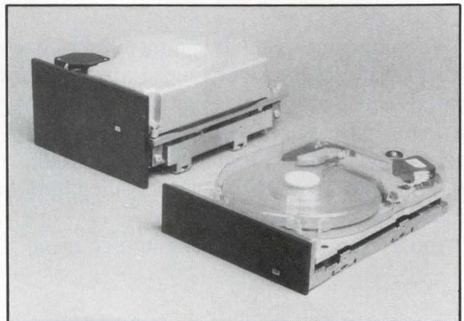
System designers can place two 5 1/4" hard disk drives in the space of one by using half-height units, as shown in this comparison from Shugart Associates. The SA706 has a single platter and stores 6.67M bytes (unformatted), while the SA712 stores 133M bytes on two disks.
