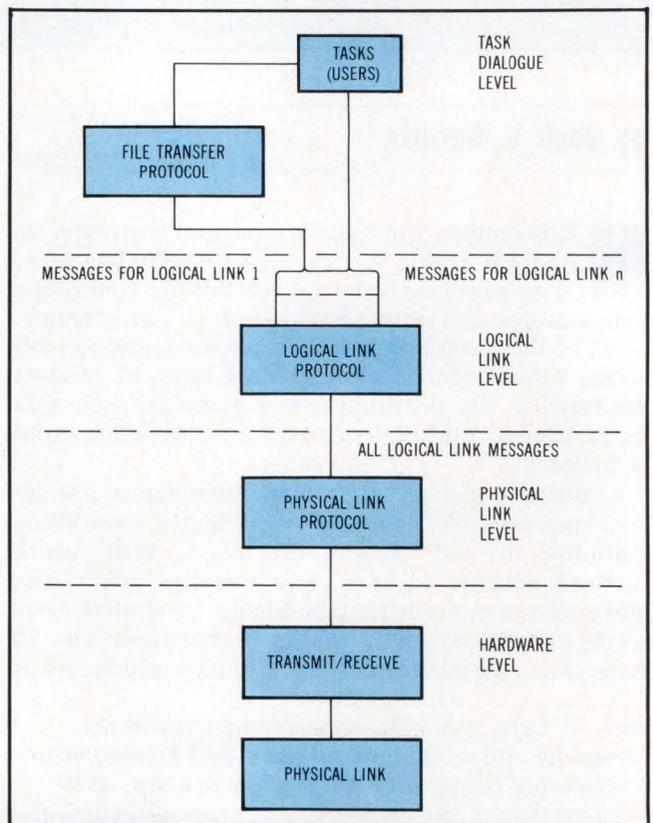
**Fig 2 Layered structure of network protocols. User application tasks access network through logical link level or through dialogue level protocol such as a file transfer.**
