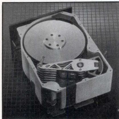
An innovative Winchester design gives the XT-1000 series of 5¼" drives 140M-byte max capacity and an average access time of 30 ms. The proprietary integral hub/dc motor design, with the spindle motor inside the disk hub, provides a deeper base casting and thus allows eight minifloppy sized disks to be stacked inside the enclosure.
