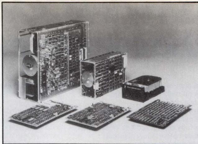
A family of Winchester drives from Priam includes 5 1/4", 8", and 14" drives, plus intelligent interface boards. The boards allow system designers to connect any combination of four Winchester drives—plus either tape or floppy disk backup—to a host processor.
