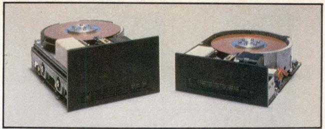
Both standard- and half-height 5¼" Winchesters are offered by MiniScribe. Standard-size versions have storage capacities from 6.4M bytes to 20M bytes, while the half-height versions store 6.4M bytes or 12.8M bytes. Average access times range from 85 ms to 120 ms.
