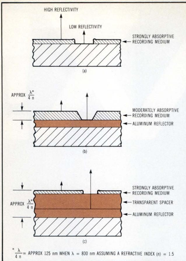
**Fig 6 Proposed configurations for optical data storage medium. Single layer (a) offers simplicity; antireflection bilayer (b) and trilayer (c) structures broaden range of useful materials and recording mechanisms.**
