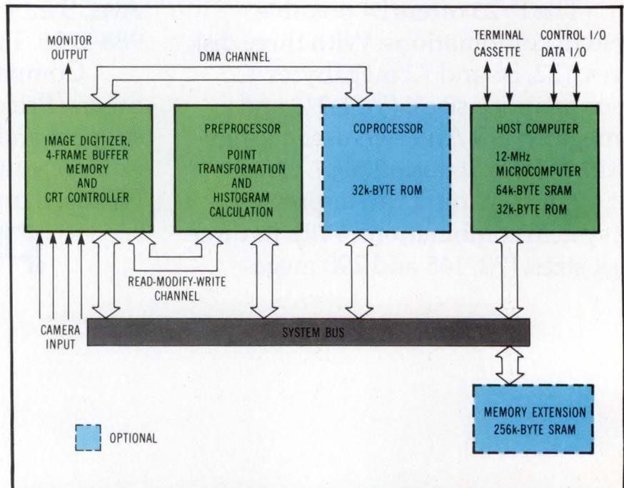
Optional coprocessor processes pixel arrays 10x faster than software routines executed in the 68000 host computer. Digitizer and preprocessor are also implemented in bipolar logic to gain realtime performance.
