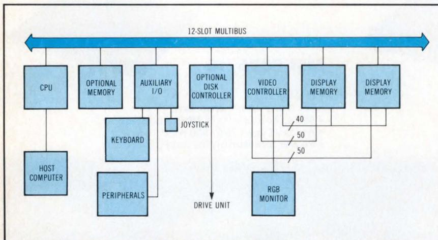
**Cubic System CS-3 block diagram. A total of 718k bytes of display memory are organized as two 512- x 512-pixel image planes with 12 bits/pixel. To upgrade the system from a graphics workstation to a standalone computer, the optional memory, disk controller, and CP/M-86 operating system may be added.**
