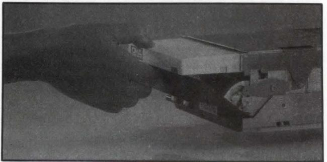
New 5¼" fixed/removable disk drives from DMA Systems provide higher storage capacities than earlier versions in the Micro Magnum family. Total unformatted storage capacities are 19.5M bytes and 26M bytes, respectively, for models 5/10 and 5/15. Of the total capacity, 6.5M bytes are on the removable cartridge for each drive version.
