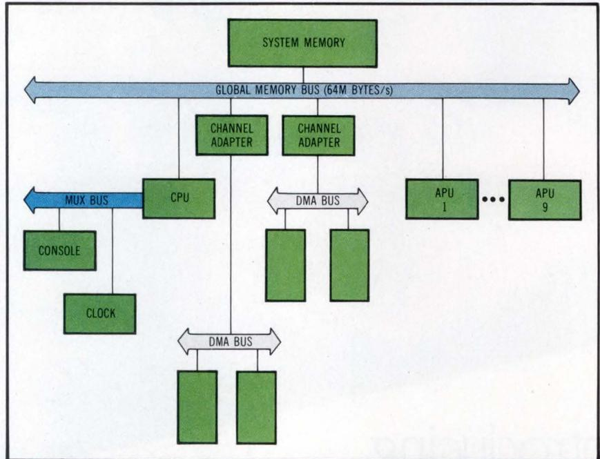
Growing from 2 to 10 processors, Perkin-Elmer's tightly coupled multiprocessor system 3200MPS handles communications between processors through a 16M-byte global memory over a full 64-bit bus. I/O transfers occur over four independent buses with 40M-byte/s bandwidth.
