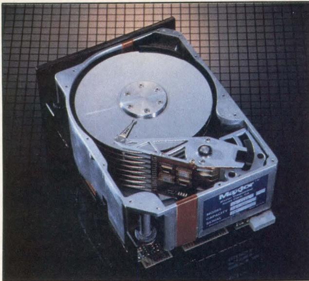
A new 5 1/4" Winchester from Maxtor packs 140M bytes of storage on eight stacked disks. The XT-1140 is the latest in a family of 5 1/4" drives that have the motor inside the spindle, thus allowing more disks to be stacked within standard physical dimensions. Access time is a low 30 ms.
