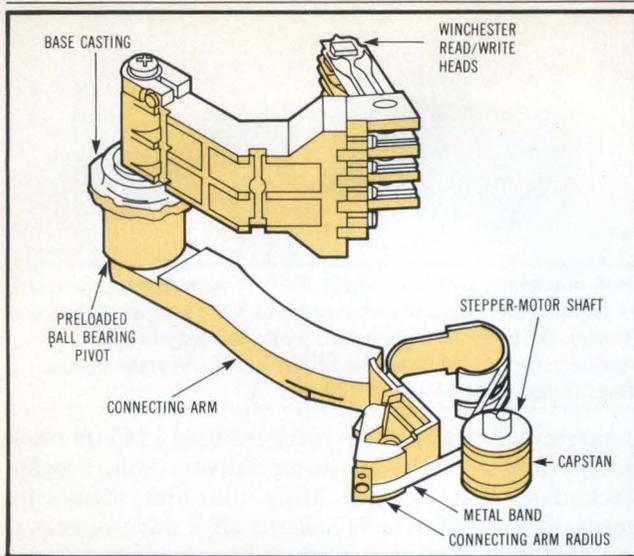
With this split-band capstan head positioner, Computer Memories solves the shock and vibration problems that affect open loop disk drive systems. The positioner assembly is used in the firm's CM5000 series of 5¼" Winchester drives. The read/write head assembly is at the end of an arm that pivots around a setpoint, allowing the assembly to more easily absorb shock without moving the head.
