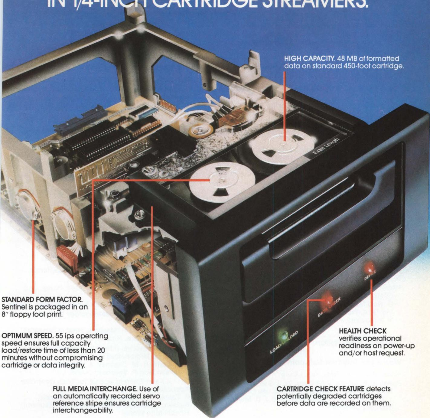
**HIGH CAPACITY.** 48 MB of formatted data on standard 450-foot cartridge.
