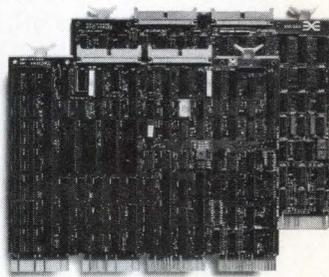
Q-bus embedded dual-density tape controller.
