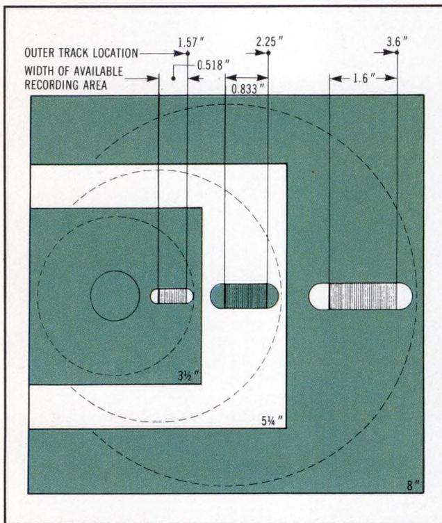
**Fig 1 Radial positions of disk areas available for recording. Comparison reveals that density can be increased on smaller disks due to reduced thermal and hygroscopic properties of Mylar media.**
