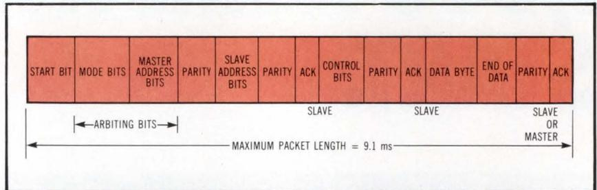
Each address, control, and data field in D<sup>2</sup>B is followed by a parity bit. The amount of information contained in data field depends on transfer mode selected. Information must fall within 9.1-ms limit for message duration.
