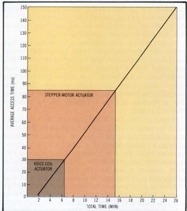
So-called voice-coil actuators for Winchester recording heads are much faster than conventional stepper motors, as shown in data prepared by Vertex. The graph compares the two techniques in terms of average access time and the total time to perform 10,000 random seeks while transferring one 256-byte sector per seek.
