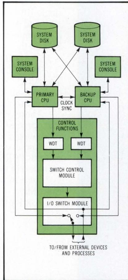
**Systemsafe/1000 uses dual HP 1000 Series F computers sharing serial input from external devices. Serial I/O control is switched within 200 ms of error detection. Data redundancy is maintained with mirrored disk storage.**
