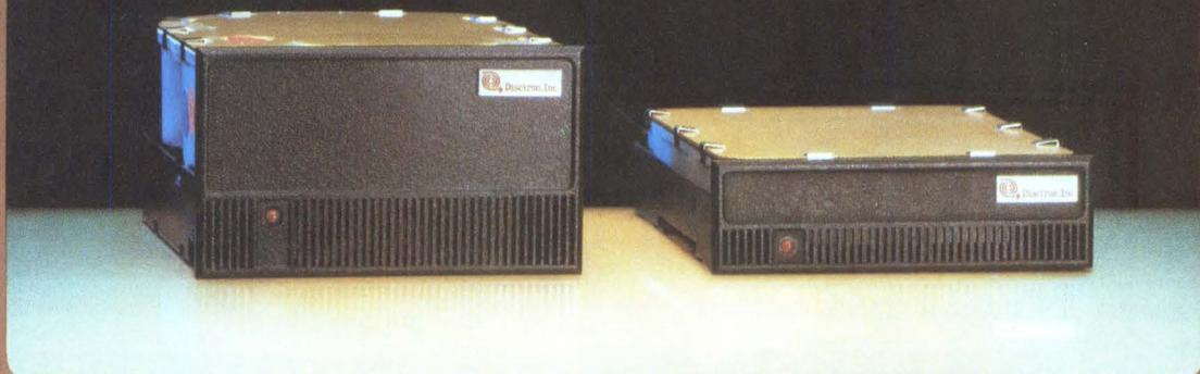
Disctron offers you more capacity, higher performance, and easier integration in 5 1/4-inch Winchester. With capacities to 40 megabytes. With average access times as low as 35 ms. And with special features—electronically dampened actuator, buffered step mode, electrical spindle brake, integral microprocessor control and built-in AGC.
