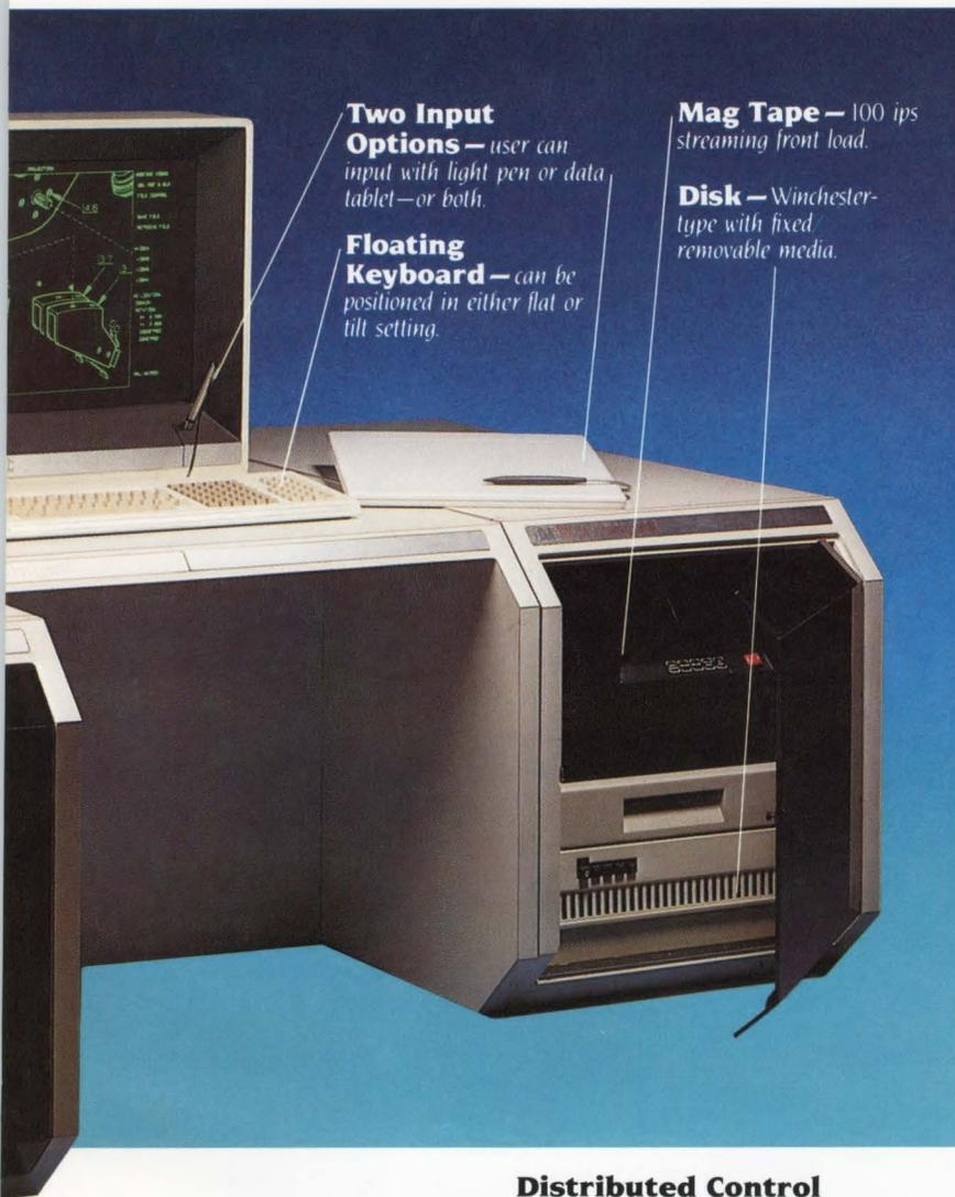
**Two Input Options** — user can input with light pen or data tablet — or both.
