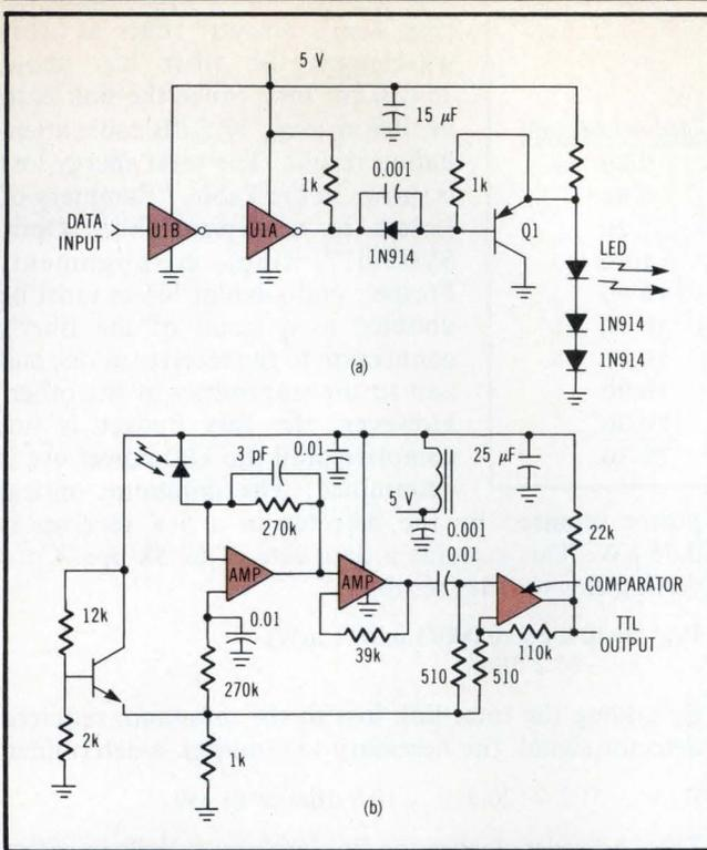
**Fig 3 Optical transmitter with LED (a). Circuit can drive LED at a 1M-bps data rate, far in excess of 62.5k-bps link illustrated. Receiver is p-i-n photodiode, requiring shielding from emi (b).**
