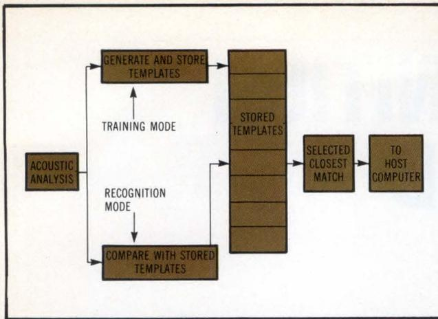
**Fig 1** Speech recognition through comparison of detected and stored voice templates. Computer detects closest match between spoken and stored templates but falls prey to time distortion errors and memory limitations.
