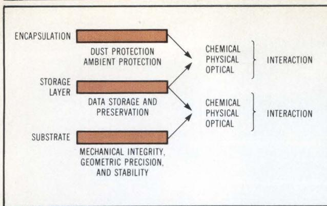
**Fig 4** Materials system of optical disk includes encapsulation, data storage layer, and disk substrate.
