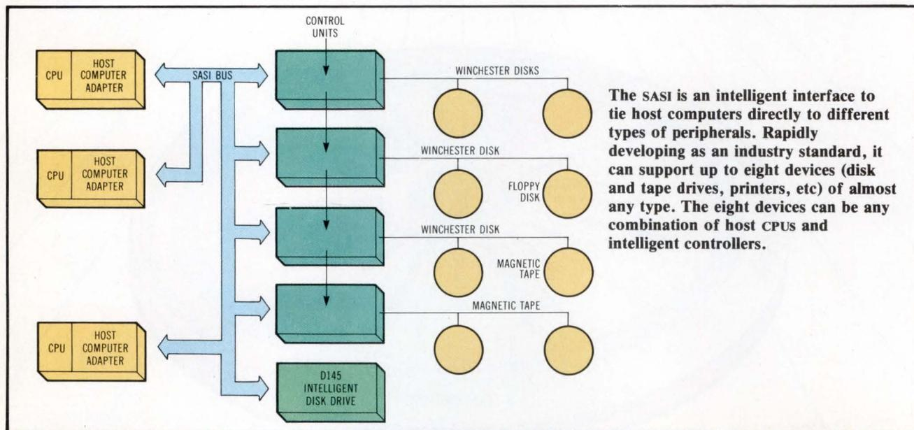
The SASI is an intelligent interface to tie host computers directly to different types of peripherals. Rapidly developing as an industry standard, it can support up to eight devices (disk and tape drives, printers, etc) of almost any type. The eight devices can be any combination of host CPUs and intelligent controllers.
