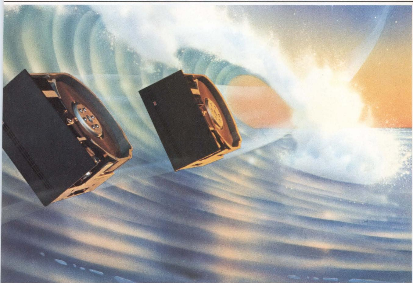
removable cartridge drive. Need a more compact drive? Pack more data in less room with our new ST206 half-high Winchester. Both new drives store 6.38 megabytes (unformatted) with reliable bit and track densities.
