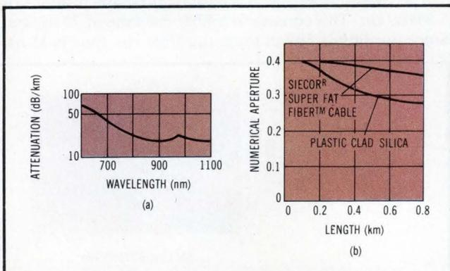
**Fig 4 Attenuation of optical fiber accounts for greatest decibel loss to network. Loss associated with wavelength of emitting diode is shown in (a). Loss due to length of cable is shown in (b).**
