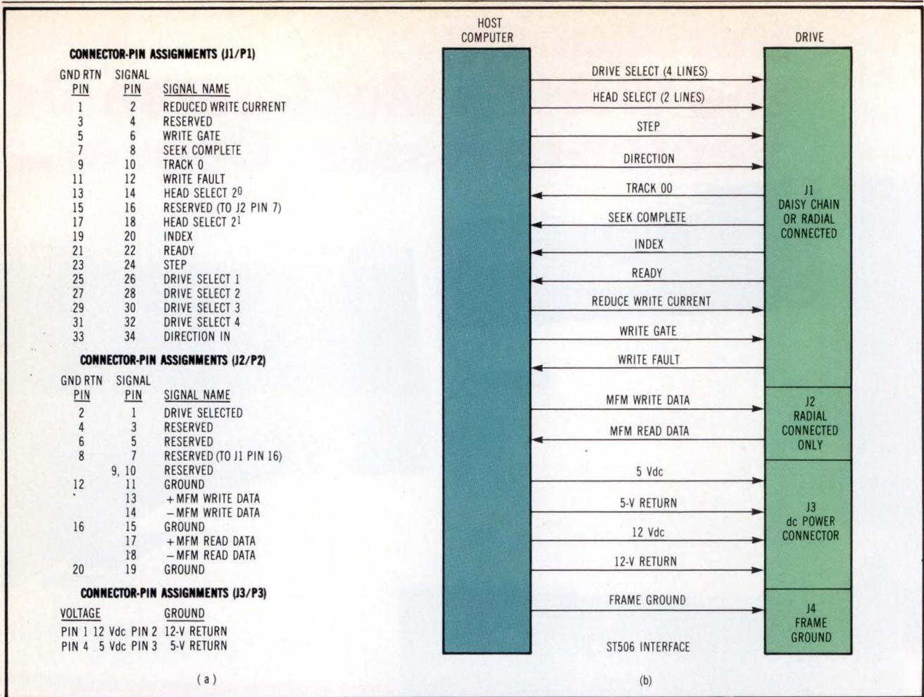
The Seagate Technology interface connector pinout for 5¼" Winchester disk drives (a), is based on Seagate Technology's ST506 5¼" Winchester disk drive. Interface lines to the host computer are shown in (b).
