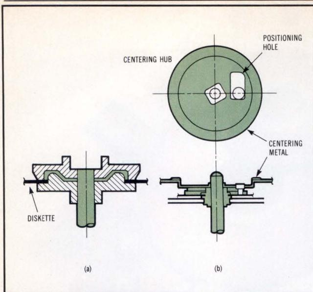
**Fig 2** Disk centering techniques used on conventional (a) and Sony (b) hubs. Surrounding disk centering hole with rugged metal ring prolongs disk life, improves centering accuracy, and ultimately reduces inner track errors.
