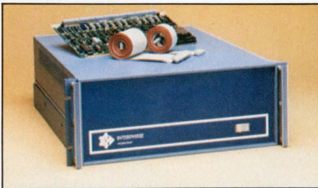
Interphase Corp, a manufacturer of bus-compatible controller boards, also sells complete Winchester disk systems. The subsystem shown includes an 8" Winchester drive, plus a power supply and fan. Various drive types and storage capacities are available.
