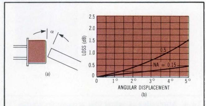
Fig 7 When fiber is not parallel to its emitting source or its receiver (a), some power loss occurs. Loss depends on angle of junction (b).
