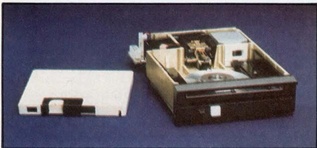
The SQ306 from SyQuest is the smallest removable-cartridge Winchester drive available. Fitting the standard half-height 5¼" space requirements, the unit has a 3.9" platter in its removable pack and provides 6.38M bytes of unformatted data storage.
