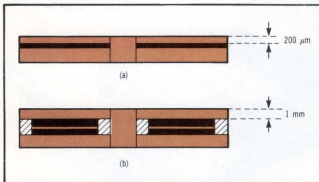
**Fig 5** Direct encapsulation (a) and air-sandwich (b) schemes have been proposed for optical disk.
