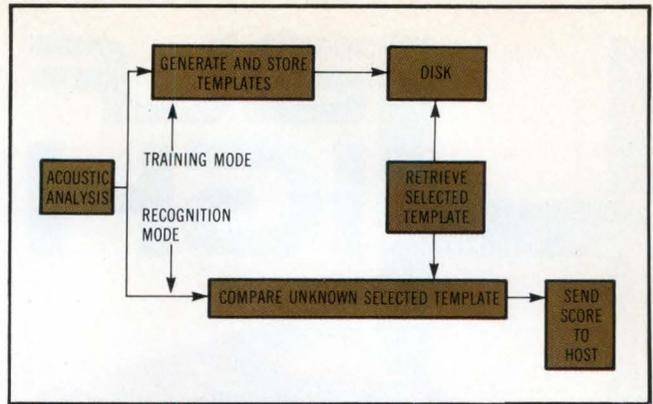
**Fig 3 Word verification method of speech recognition. Computer drives interaction with its user by selecting word from its vocabulary and then verifying user's response to it. Memory and processing demands are reduced since only one word is under analysis at a time.**
