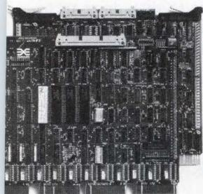
big SMD drives on your -11. Links Q-bus with 1-2 SMD drives. Software transparent media compatible with DEC 02, RM05, RP06. Features 3-sector data buffer, 32-bit ECC, to half a billion bytes capacity. Over 1500 units in service!
