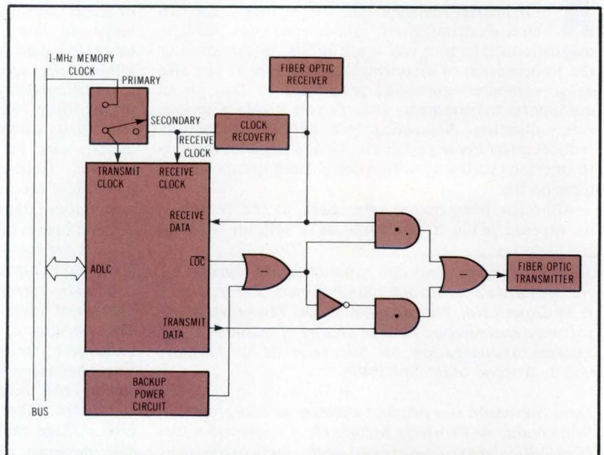
**Fig 2 Clock recovery and loop-through circuit. ADLC interfaces to fiber optic transmitter and fiber optic receiver in clock recovery circuit. Power backup on board prevents network crash, should one terminal fail.**
