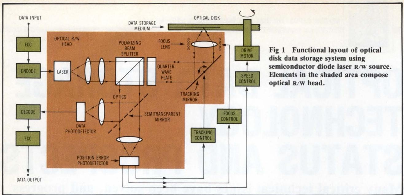
**Fig 1 Functional layout of optical disk data storage system using semiconductor diode laser R/W source. Elements in the shaded area compose optical R/W head.**
