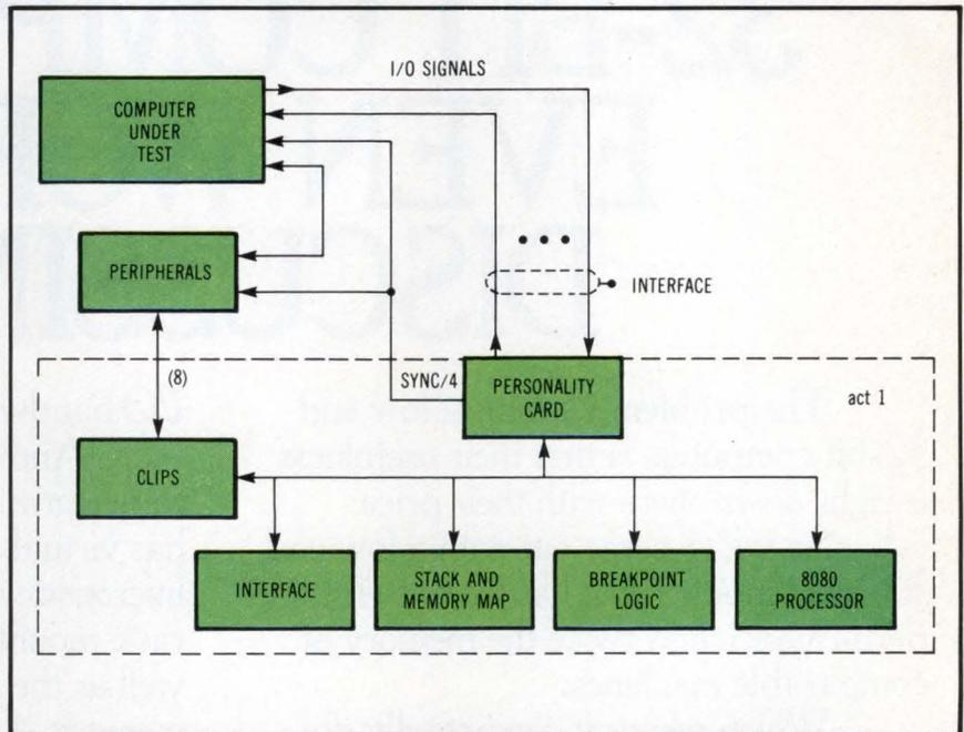
**Unique personality module for each target computer supported is key to realtime operation of act 1. Personality module generates necessary control and I/O signals needed for act 1 to interface independently with target processor. Module also aids disassembly of programs.**
