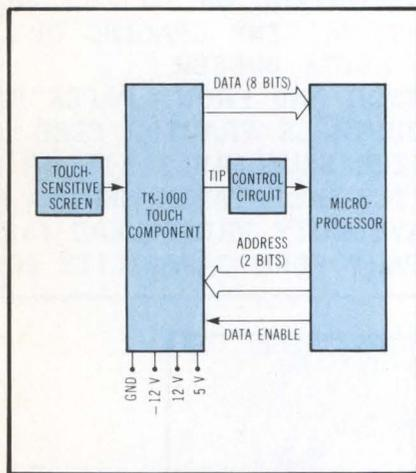
Interaction Systems has improved the resolution of its capacitive-sensing technology with TK-1000, a touch sensor that allows unrestricted definition of touch-sensitive areas on one surface. Proprietary technology, which deposits indium tin oxide over an unpatterned glass faceplate, provides continuous X-Y coordinates of the touch point in 8-bit (0 to 255) numeric output for both dimensions. The unpatterned, temper-coated
