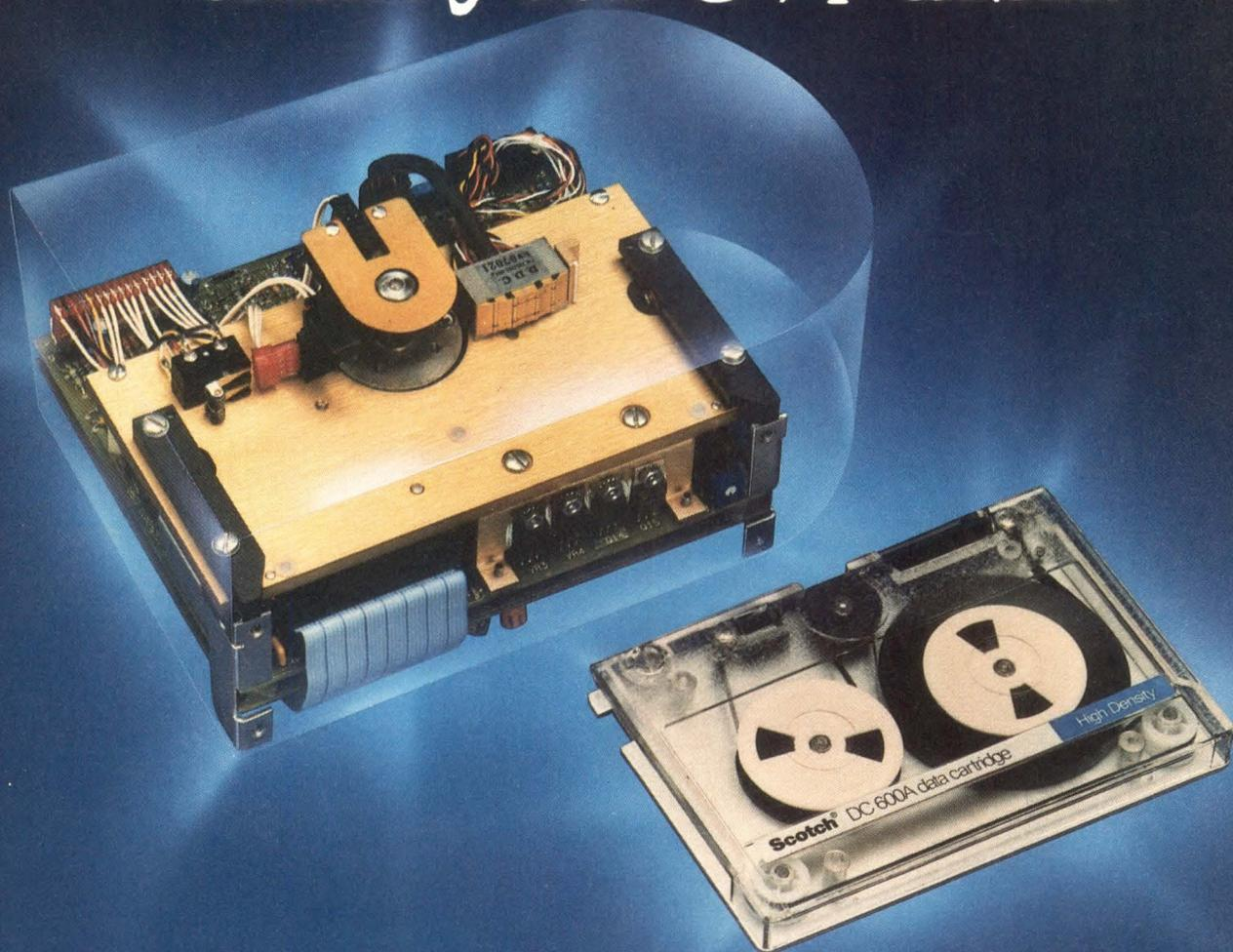
Digi-Data Corporation proudly introduces the industry's first full-function  $\frac{1}{4}$ " cartridge tape drives to fit within a 5 $\frac{1}{4}$ " disk footprint. Small in size (3.25 × 5.75 × 6.90"), but large in performance, these drives provide up to 300% more storage capacity than other available start/stop or streaming drives. Their 30 Mbytes of unformatted capacity will handle the backup requirements for most 5 $\frac{1}{4}$ " and 8" Winchester using a single cartridge.
