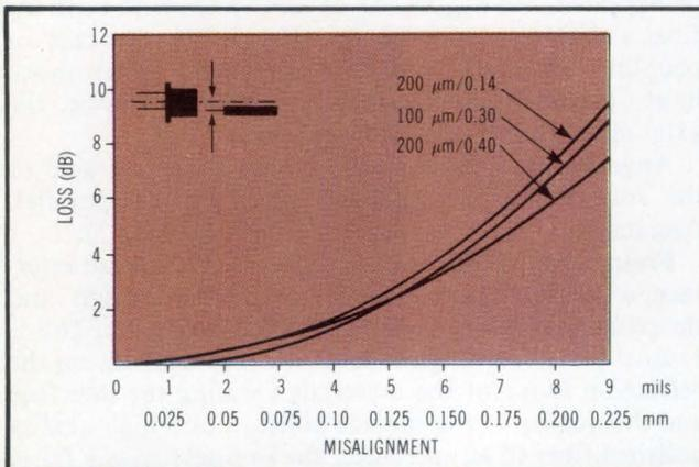
Fig 6 Axial misalignment is generally insignificant when optical fiber's core is much greater, or much smaller, than emitting device.
