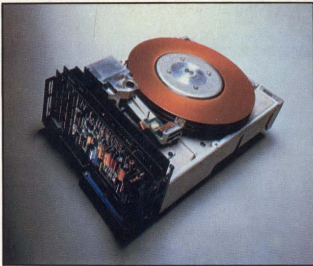
Using a voice-coil servo rotary actuator, compact hard disk drives in the 8500 series from 3M provide a storage capacity of 60M bytes and a random average seek time of 29 ms. The package is the same size as a standard 8" floppy disk drive.
