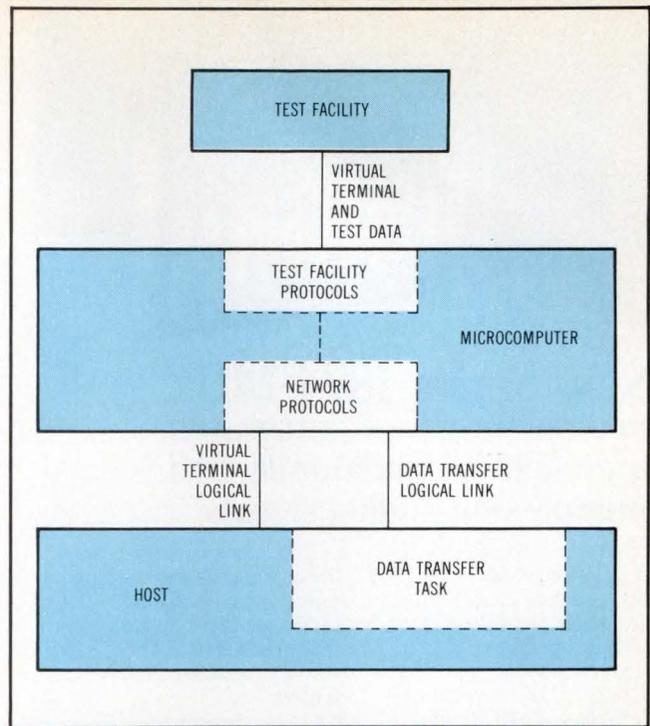
**Fig 3 Test computer/host interface scheme. Microcomputer acts as protocol converter, exchanging messages between test computer and host. Multiple logical links allow one link to be used to make test computer's terminal into virtual terminal of host, while another link transfers test data.**
