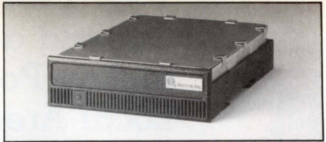
Half-height 5¼" drives from Dicom store 25.5M bytes (model 620) or 42.5M bytes (model 640). Both versions have a 40-ms average access time. Head positioning employs voice-coil and closed loop servo technology.
