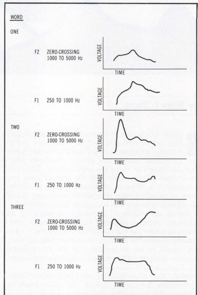
**Fig 2** Zero-crossing analysis of words "one," "two," and "three" provides estimate of major resonant frequencies of speech. Signals are derived by first dividing speech into frequency regions F1 and F2.
