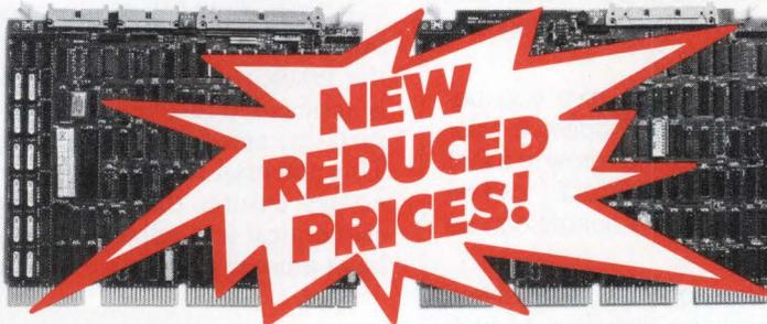
Low cost for smaller-sized disks. Single quad-board interfaces LSI-11s to 8" & 14" SMD hard disk drives. Same great SC01-level performance in most applications. Software transparent. Full 32-bit ECC, self-test, 512-word bootstrap, real-time clock control, and bus terminators. Mix and match drives on one controller. 72,000 hours MTBF!
