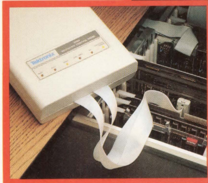
6809 Prototype Control Probe tip fits easily in hard to reach locations. Probe status lights monitor key processor signals.
