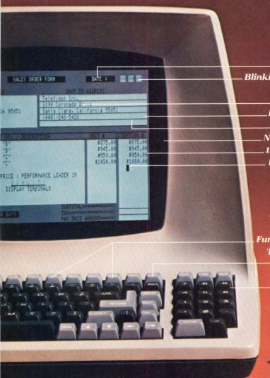
> Upper/lower \_\_\_\_\_ case char, \_Protected fields \_\_\_\_ Underlining Non-glare screen \_12 x 10 char, res, \_ Blinking cursor
