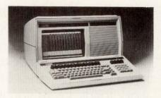
Low profile, and foldup keyboard of Direct's VP 800/A video display terminal adapt it to laboratory or office environments. Unit can display 28 lines of 132 characters with an additional programmable status line
