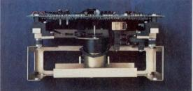
20 MByte Streaming Cartridge Tape Drive.
