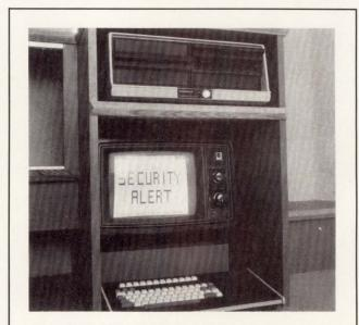
Fig 3 Keyboard and display device. User inputs and programming are entered into system through ASCII keyboard. Unused channel of standard TV receiver displays information. Floppy disc unit at top stores all information for homeowner
