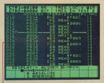
By using the proper personality module, software flow can be displayed using the mnemonics of the chip under test, here the Motorola MC6802.
