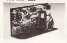
Single-output switching regulated dc power supply series SWS 150 comes in 5 models rated at 150 W that provide 5 V at 30 A, 12 V at 12.5 A, 15 V at 10 A, 24 V at 6.5 A, and 28 V at 5.5 A. Open frame series offers continuous operation, 115/230-Vac single phase input, and 75% efficiency. Features include overvoltage protection, logic shutdown and/or inhibit, power fail alarms, and factory burnin. **Standard Power, Inc**, 1400 S Village Way, Santa Ana, CA 92705.
