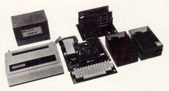
FLAIM/65 is a complete, professional quality development system for the 6500 microprocessor family. FLAIM/65 includes a ROCKWELL AIM 65 (with 20 character display and thermal printer plus full size keyboard), five slot motherboard, 16 K static RAM memory, dual drive 5½ inch disk system with full operating system in EPROM, CENTRONICS 730 dot matrix printer (100 CPS), assembler, PL/65 compiler and full system power supply. Best of all — the system pictured is priced well under \$4000 (U.S. only).
