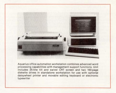
cations functions. Word processing capability includes display of justified text, single- and double-underlines, footnote references, bold print, horizontal and vertical lines, and even forms. Screen information can be scrolled both vertically and horizontally.
