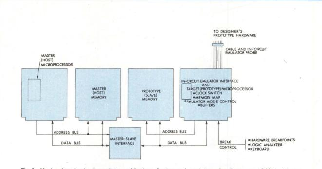
Fig 3 Master-slave in-circuit emulator architecture. System and prototype functions are divided between master (host) and slave (target) microprocessors, respectively. System development functions, such as file management, text editing, host I/O, and debugging, are performed by master microprocessor. Prototype related functions, such as prototype program execution, prototype I/O, and in-prototype testing, are done by slave microprocessor
