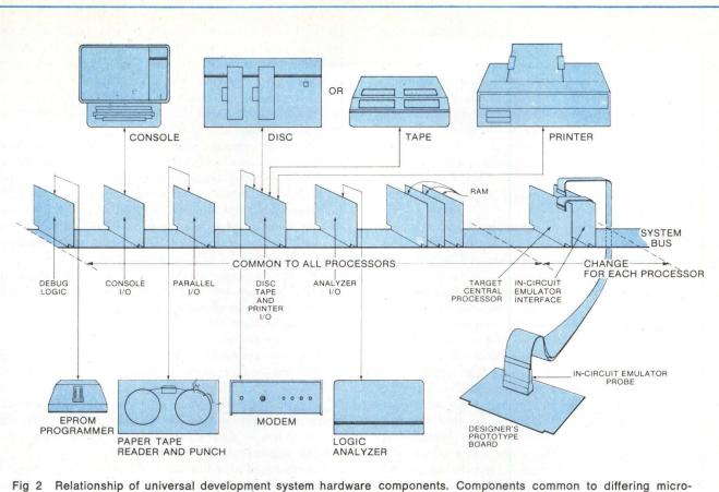
Fig 2 Relationship of universal development system hardware components. Components common to differing microprocessors include all I/O and memory devices. Only target central processor and in-circuit emulator interface are changed to accommodate specific microprocessor
