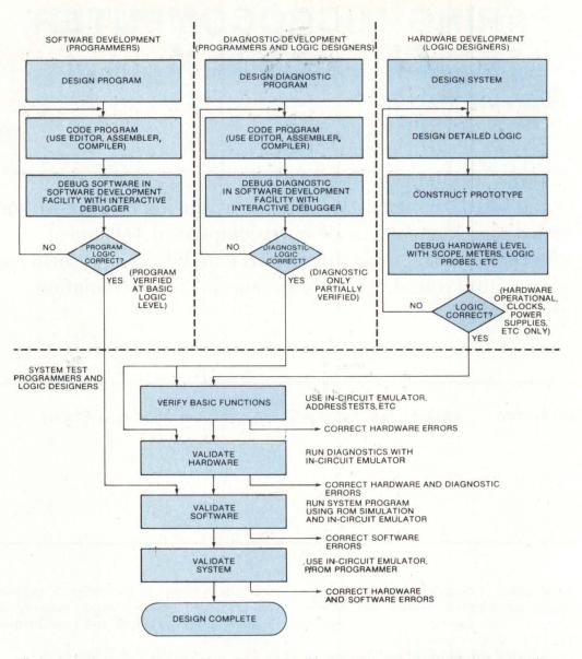
Fig 1 Microprocessor based system design with development system. Development of microcomputer based design involves preparation of application program, hardware design, diagnostic programming, and system test phase. Capability of development system is especially critical in latter, when it is necessary to sort out hardware versus software problems
