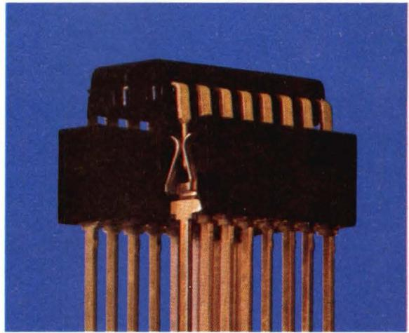
Get the high reliability that eliminates trouble. RN "side-wipe" DIP sockets make contact with the wide, flat sides of your IC leads. You get 100% greater surface contact for positive, trouble-free electrical connection.
