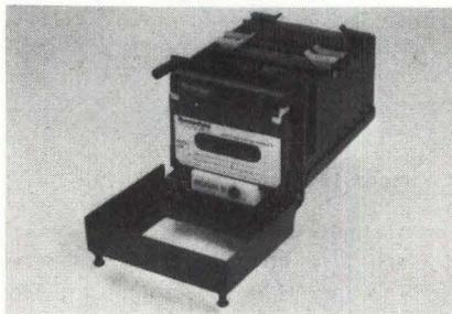
analog information at a 0- to 10-V level may be multiplexed, converted to digital data, buffered, and clocked onto a cassette tape at rates up to 100 bits/s. Recording format is complementary NRZ and recording density is 615 bits/in. Unit is CMOS throughout, and requires only 85 mA when recording. **Memodyne Corp.**, 385 Elliot St, Newton Upper Falls, MA 02164.
