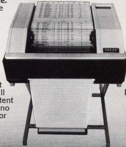
The Tally technique minimizes moving parts. The one-piece Tally print comb prints one horizontal dot row at a time. The paper advance assembly progressively steps the paper vertically one dot row to complete the matrix character. It's simple. It's reliable.
