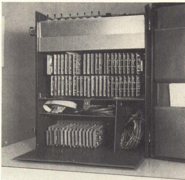
codes compatible with a six-bit-plus-parity (BCD) code. This includes the NAND, SMAL (Small-Level), SMS and SLT (Solid Logic Technology) logic families, with voltages ranging from +12 volts to -12 volts. Switches, indicators and counters are easily accessible by lifting the cover of the carrying case (Fig. 4).
