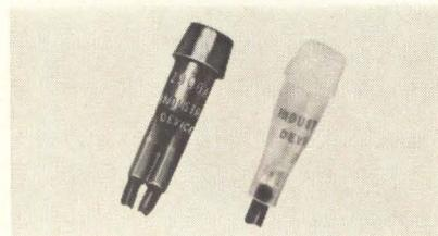
One-piece, lens/body GLO-DOT Series 6- and 12-V indicator lights are available in five lens colors: red, white, green, blue, and yellow. The economical lights have built-in incandescent lamps and 4½" long 24 AWG insulated leads, pre-stripped one-half inch for rapid connection. Lights are designed for easy mounting in 5/16" diameter holes, with push-on mounting nuts supplied. Industrial Devices, Inc.
