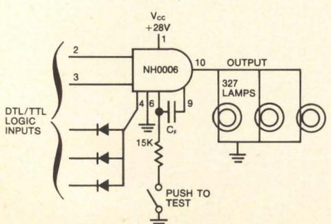
LAMP DRIVER WITH EXPANDED INPUTS
