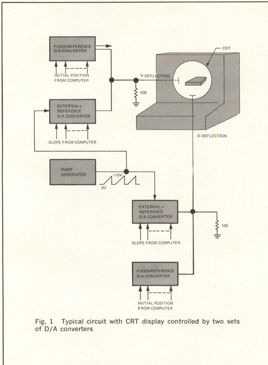
Fig. 1 Typical circuit with CRT display controlled by two sets of D/A converters
