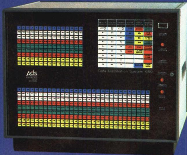
**FULL CONTENTION** is the big feature of the compact ADS-630, the new **economical** bit type time-division multiplexer. With it, you can expand your real-time telephone/computer network — pyramid data terminals and utilize **all** low speed computer ports on a first-come/first-served dial-up basis. ADS-630 will increase system efficiency; reduce costs dramatically.
