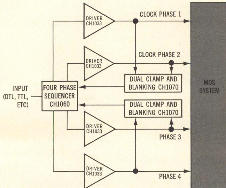
The four phase system shown uses a CH1060 FOUR PHASE SEQUENCER, four CH1033 HIGH SPEED CLOCK DRIVERS and two CH1070 DUAL CLAMP AND BLANKING CIRCUITS.
