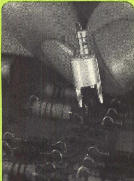
**NEW PLUG-IN HOLDER . . .** for Littelfuse subminiature fast acting picofuse, is designed for P. C. board installation. Accepts regular or high reliability picofuses with ratings from 1/16 to 10 amps. Picofuse . . . the world's smallest fuse . . . weighs only 1/5 gram. Ideal for computers, sophisticated airborne instruments and other sub-miniature circuits.
