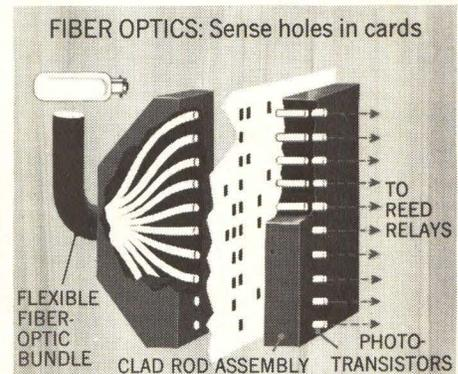
Electro-optical systems incorporating fiber optics are operating at up to four times the speed of electro-mechanical systems. When a combination of fiber optics, phototransistors, and reed relays is used, reading of basic data is not controlled by mechanical limitations. The use of fiber optics allows wide design freedom to increase system operating speed.
