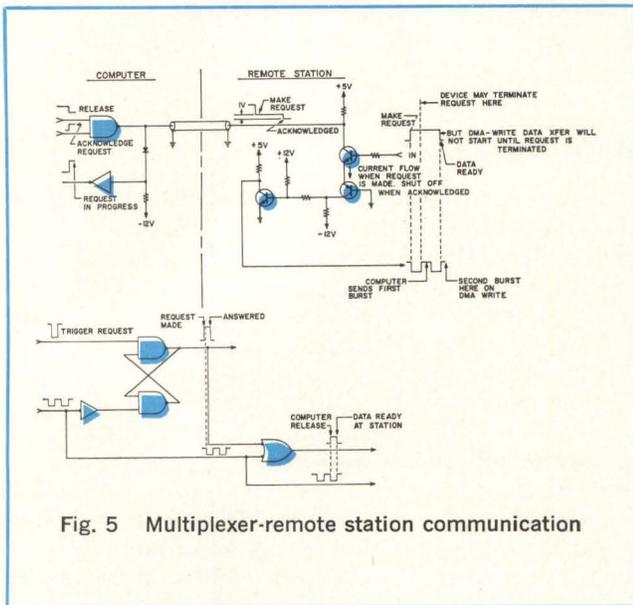
Fig. 5 Multiplexer-remote station communication
