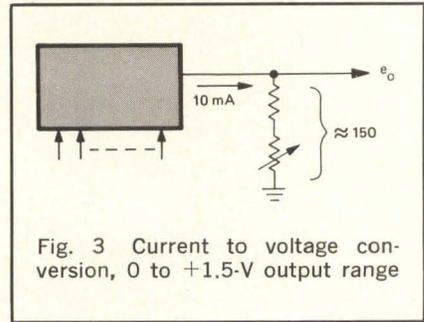
Fig. 3 Current to voltage conversion, 0 to +1.5-V output range
