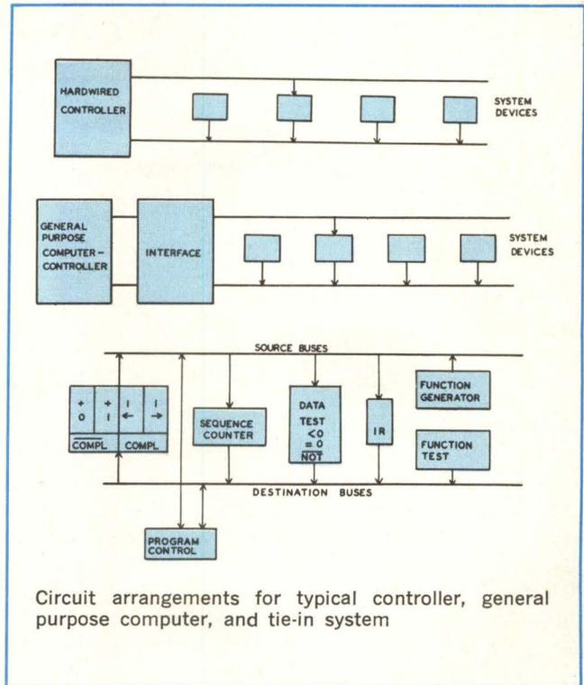
Circuit arrangements for typical system controller, general purpose computer, and tie-in system
