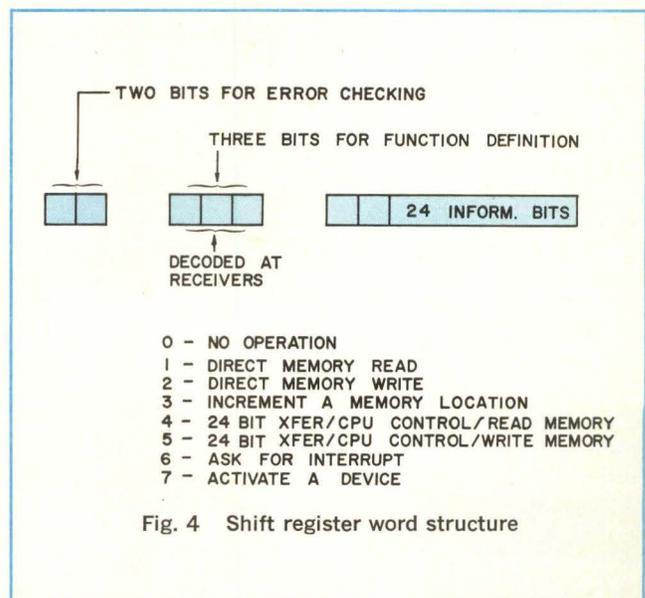
Fig. 4 Shift register word structure
