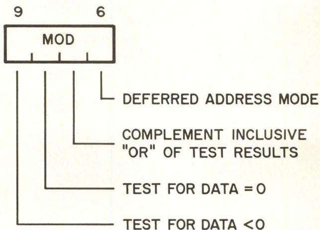
If a jump is performed, the current value of the sequence counter is automatically stored in a trap register associated with the data test. If the jump is to a subroutine, the trap register provides the link back to the calling program.
