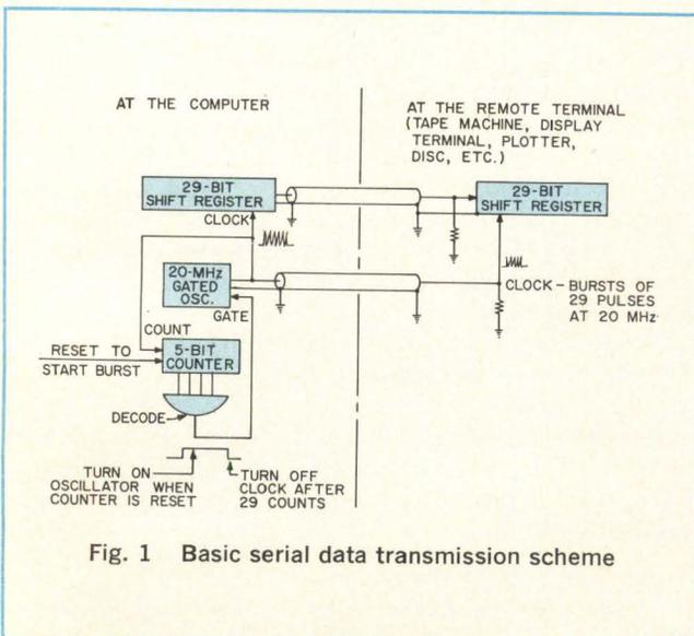
Fig. 1 Basic serial data transmission scheme
