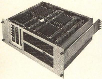
High speed commercial memory system — **NANOMEMORY 2600**. Full cycle time of 600 nanoseconds, and word capacities of 16K by 18 or 8K by 36. It's all done with a second-generation 2-1/2D drive system with efficient circuit and logic design, for reduced component count and high MTBF, and wide operating margins—the real feature of the 2-1/2D configuration. It is easily expandable in the field, and comes in a standard 19" rack.
