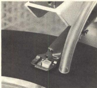
Typical head testing (shown above) using the Royco sensing tube for the pick-up of abnormal amounts of particles generated by an aerodynamically unstable head.
