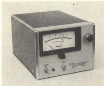
The particle generation is sensed and displayed in analog fashion (shown above) for immediate indication. When a pre-set limit is exceeded, the head retraction mechanism actuates automatically or an alarm notifies the operator of an aerodynamically unstable head.
