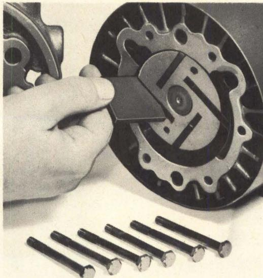
Normal service is occasional flushing of chamber and replacement of vanes. Just remove the six end plate bolts and you're inside . . . it's really that simple.
