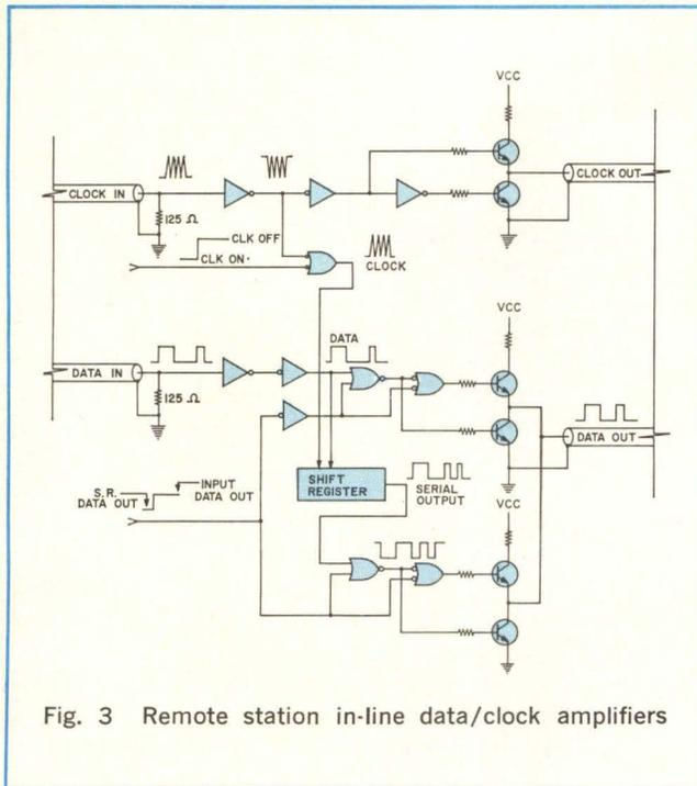
Fig. 3 Remote station in-line data/clock amplifiers
