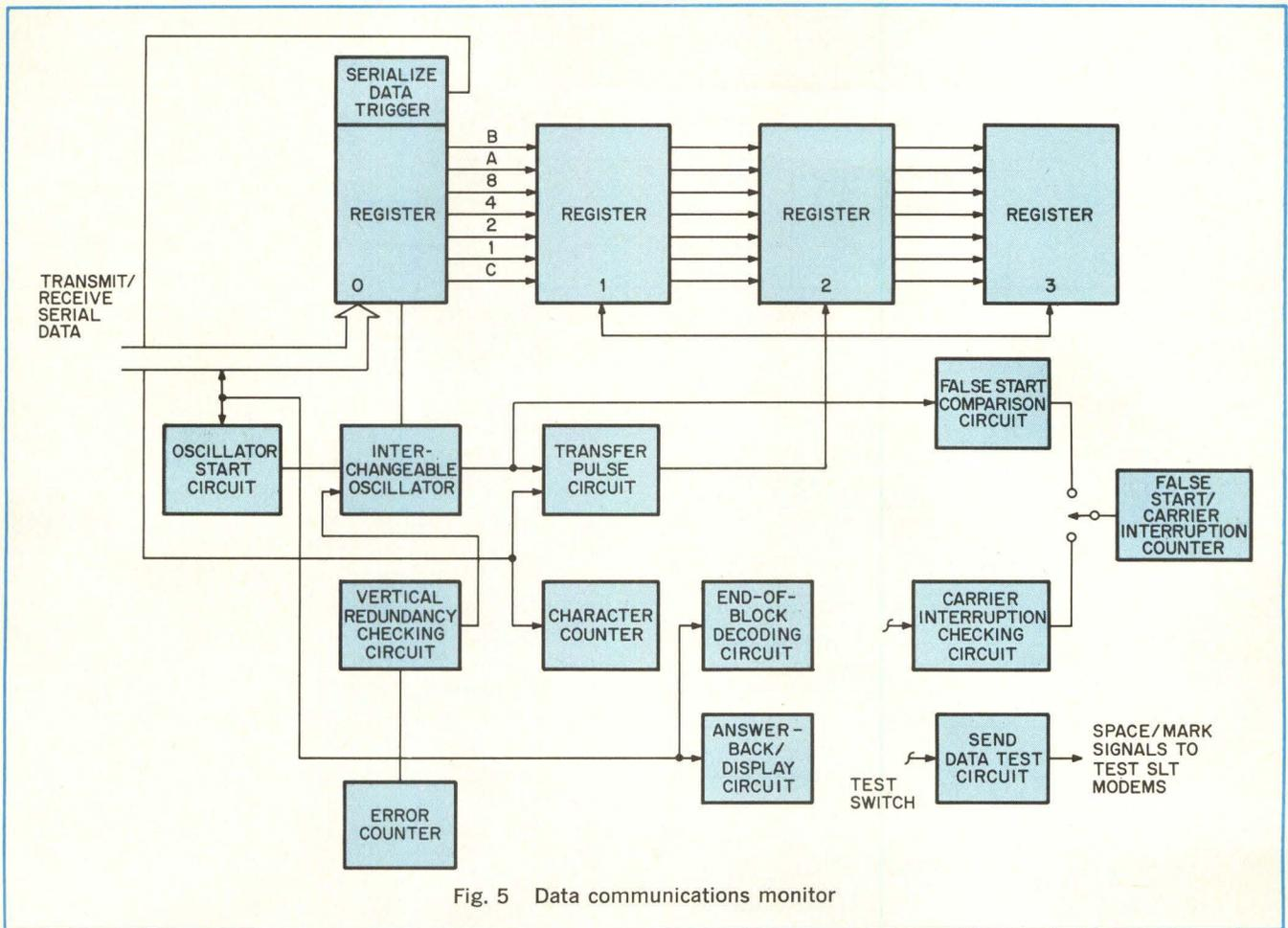
Fig. 5 Data communications monitor
