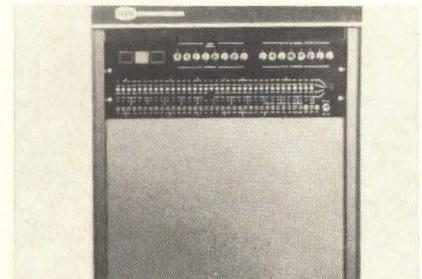
The DC-16 interfaces with all available mini-computers and from one to eight IBM 2311 or 2312 type disc drives. The controller avoids the former requirement for the processor to drive the disc and, in addition, simplifies programming, increases subsystem efficiency, and takes over several software functions. The system requires only seven commands for easy programming and has 10 records containing 2,560 bytes per track. KDI Interactive Data Systems, Inc.
