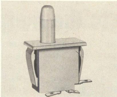
Momentary action switch E69-00A is specifically engineered for use as a door interlock and office machine "start" switch. It is housed in a long-life white molded nylon case, featuring a "snap-in" design for easy panel mounting and features coil spring snap-action mechanism and rock-wipe contact action. The switch is available in spdt or spst, either normally open or normally closed. Maximum operating force is 15 oz. A free sample is available upon request. Cherry Electrical Products Corp.
