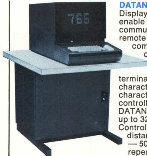
**DATANET765\*** Terminal Display Controller Units enable interactive communications with a remote or co-located computer. Each controller will operate one or two keyboard/display terminals with up to 1012 characters (22 lines of 46 characters each). Other controllers, such as the DATANET 760, will serve up to 32 remote terminals. Controller-to-terminal distances up to 1000 feet — 5000 feet with repeater units.
