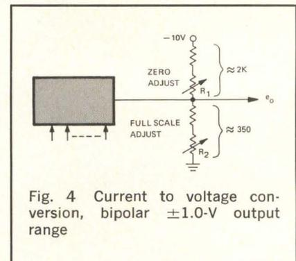
Fig. 4 Current to voltage conversion, bipolar  $\pm 1.0$ -V output range
