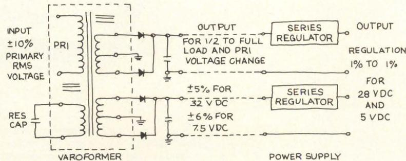
Starting with our basic Varoformer™ (constant voltage transformer) we can design power supplies to perform simple or complex functions by the addition of series regs. From 4% regulating Varoformers to custom-designed power supplies with multiple outputs, on-off sequencing, and remote sensing. If you're a computer/peripheral designer, all you have to do is tell us what goes in and what comes out. We'll take care of the rest.
