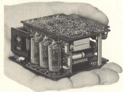
1. That's an average-sized hand in the illustration. Even when not removed from its attractive dustproof case, the Analogic AN2510 is half the size of competitive units, and requires only half the power . . . yet standard features are true differential input, 0.05% accuracy, BCD output, and  $-10^{\circ}\text{C}$  to  $+60^{\circ}\text{C}$  temperature range. No DPM at any price (or size) offers more features or better specs.
