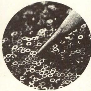
Five new memory cores for your next stack or system. All are medium or high drive, all coincident current, and all are fast switching for your high speed applications. Four new cores available in 18 mil, 20 mil, and two types of 30 mil sizes for use from 0° to 70°C. Also, a new wide temperature range 18 mil core for severe environments of -55° to +100°C.
