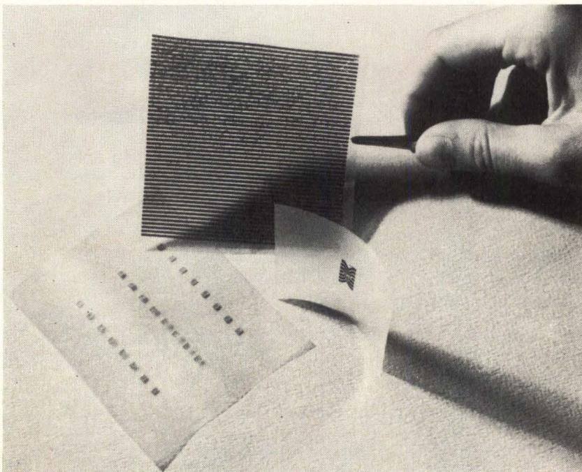
A wide variety of patterns may be produced with the TDS, including a strip pattern composed of a ferrite material for a computer memory stack
