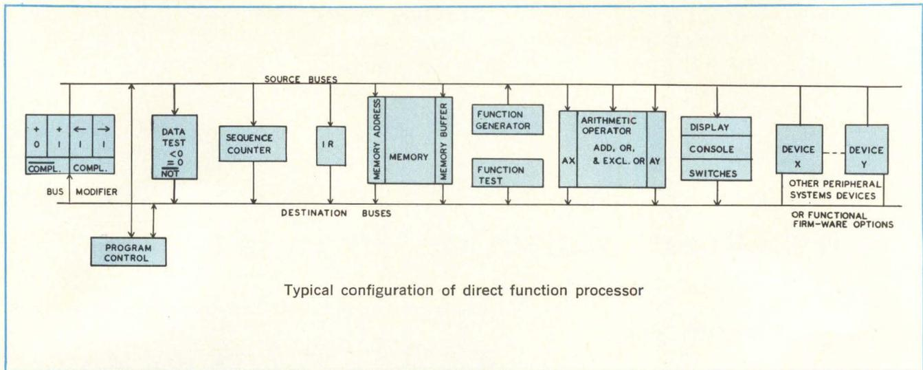
Typical configuration of direct function processor
