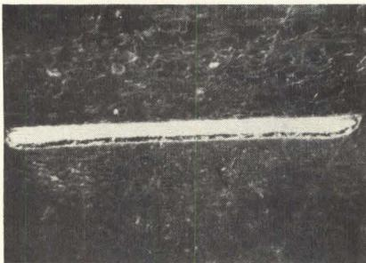
Cross section of a line 1 mil thick and 20 mils wide, illustrating the minimal undercut achieved with RICO PC+
