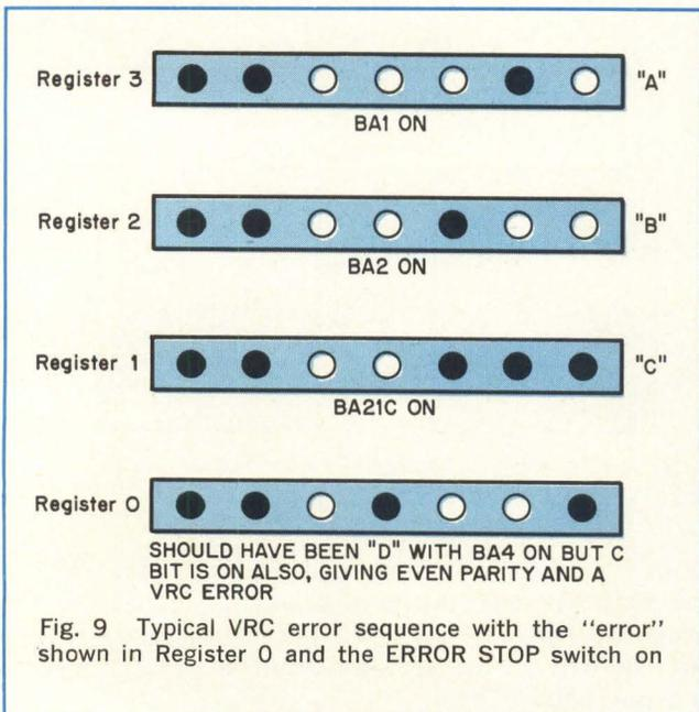
If the data line is at a space level on the first transition of the line-sampling oscillator, a "0" space is set into the "C"-bit position of the deserializer/display register (Register 0), and the register contents are simultaneously shifted. Since all the register-bit positions are set on at the start of each character, the first sample and shift pulse turns the "C" bit trigger off and all other bit triggers on.
