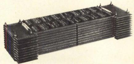
Perfect for high speed, large capacity mainframe memory systems... **NANOSTAK 3020**...technology breakthrough in 3W, 2-1/2D stacks. Stackable, compact size is an amazing 25% of competitive planar stacks and offers a significant advantage in form factor for system packaging. Extremely fast 650 nanosecond cycle time for 8K or 16K by 40, or 32K by 20 word memories.
