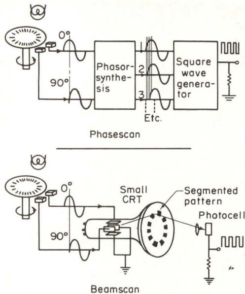
Fig. 15. Phasescan and beamscan techniques.
