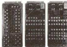
boards offer you an electrical output accuracy of  $\pm 0.5$  degrees at 250 ma output current. Data input is 11 bit Binary angular data in parallel format.
