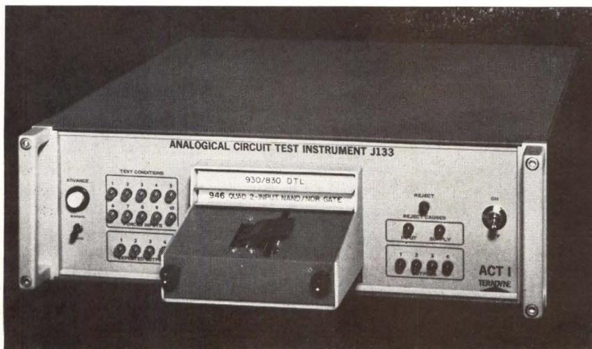
Fig. 2. This new test instrument makes 15,000 analog and logical tests on digital integrated circuits in 1/100 of a second.
