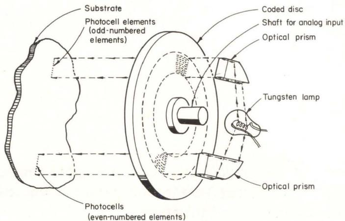
Fig. 16. Basic digital encoder system showing optical encoding scan techniques.
