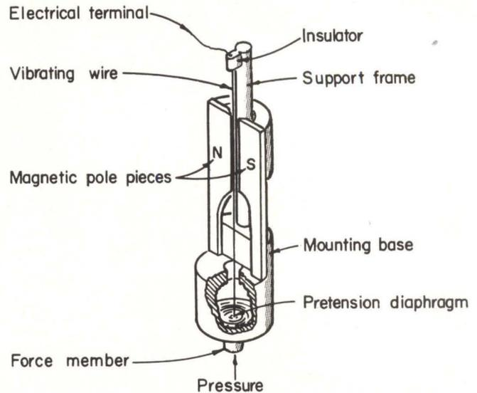
Fig. 1. Sectional view of a vibrating-wire transducer.
