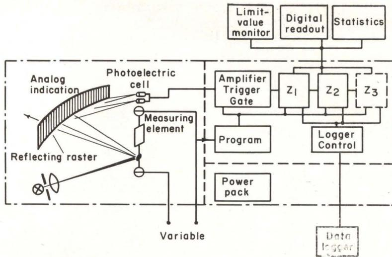
Fig. 9. Mode of operation and lay-out of the Digizet.
