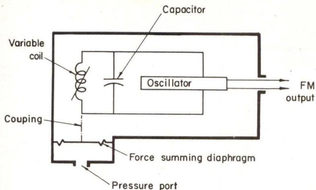
Fig. 2. Variable-reluctance digital transducer with internal oscillator.
