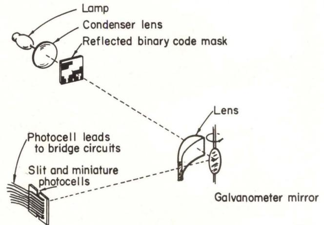
Fig. 8. Modified digitizer optical arrangement for obtaining seismic measurements.
