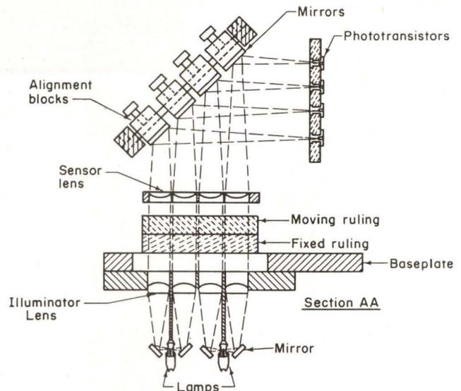
Fig. 21. Arrangement of optical parts.
