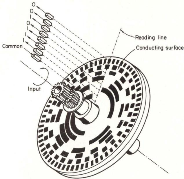
Fig. 13. Brush-type digital shaft encoder.
