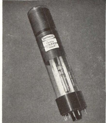
**New Symbolray\* CRT.** This new tube provides alphanumeric inputs for computer readout devices. The tube's 2" target can be scanned electronically to select symbols, characters, and punctuation marks in sequence to form readout on a display tube. Designated type CK1414, this tube provides an economical method of generating characters for hard copy print-out or for cathode-ray display. Designs with 64 or 100 characters are available.
