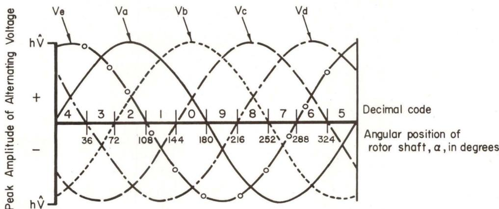
Fig. 4. Output voltages of interconnected mixing transformer secondaries.
