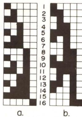
Fig. 17. Binary-coded scales.
