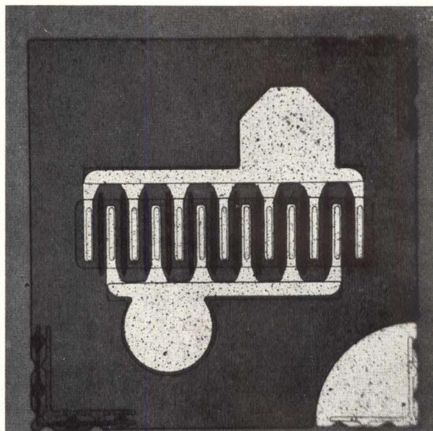
TIS88 is well-suited for RF amplifier and mixer applications because of its high-frequency capability, and also because of its square-law transfer characteristic which minimizes cross-modulation.
