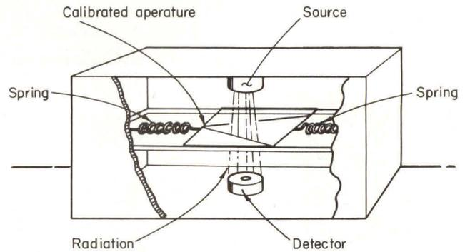
Fig. 5. Nuclear techniques applied to acceleration measurement.
