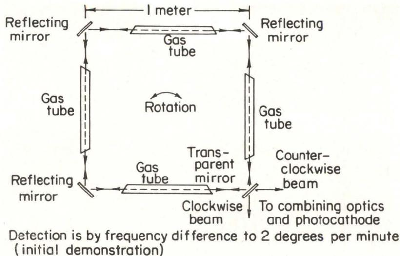
Fig. 22. Application of lasers in measurement of rotation.
