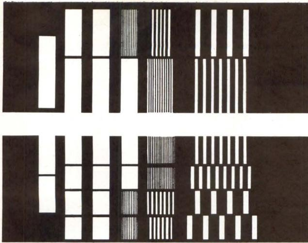
Fig. 20. Eleven-bit Gray-coded optical rulings folded against each other to form the ruling pair.
