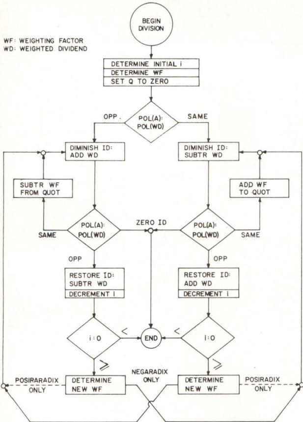
Fig. 2. Flow chart for division using the mechanical restoring algorithm. The paths designated for negaradix and posiradix systems are for constant  $K$  in weighting factor  $(-1)^K (r^i)$ . If the sign of  $(r^i)$  alternates, the designation of the paths would be reversed. In the general case, for any new weighting factor, each pass must begin with the first polarity test (not shown).
