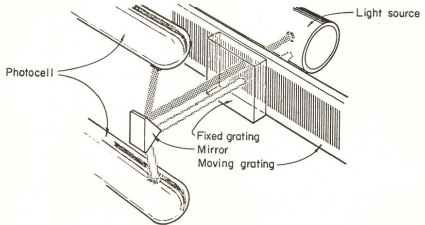
Fig. 12. Measuring displacement by Moiré fringes.
