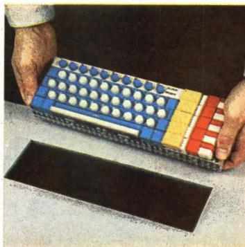
**KB allows bench assembly.** Assemble a complete keyboard matrix at the bench where the job is easier, faster. Even the wiring is done before the matrix is set into the console.
