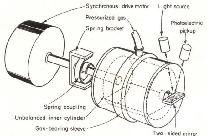
Fig. 10. A feasibility model of the synchronous rotating-pendulum accelerometer.
