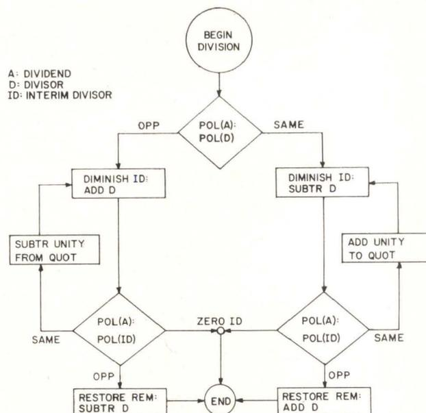
Fig. 1. Flow chart for division using the counting algorithm.
