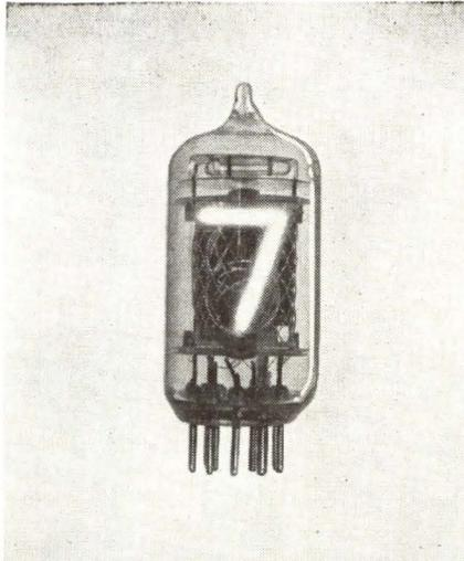
**Datavue\* Side-View Tubes.** New type CK8650, with numerals close to front, permits wide-angle viewing. These side-view, in-line visual readout tubes display singly numerals 0 through 9 or preselected symbols such as + and - signs. Their  $\frac{5}{8}$ " high characters are easily read from a distance of 30 feet. Less than \$5 in 500 lots, they also cost less to use because the bezel and filter assembly can be eliminated and because their mating sockets are inexpensive.
