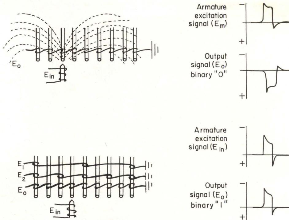
Fig. 19. Principles in the development of magnetic-reluctance digital transducer.
