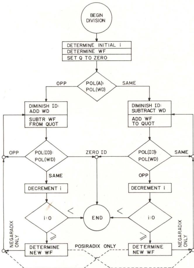
Fig. 3. Flow chart for division using the mechanical non-restoring algorithm.
