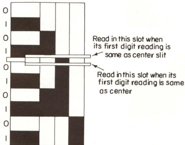
Fig. 18. Two-slit switching system.
