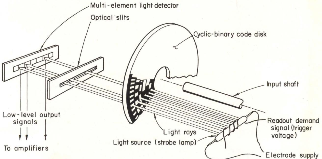
Fig. 14. Brushless-type digital shaft encoder.
