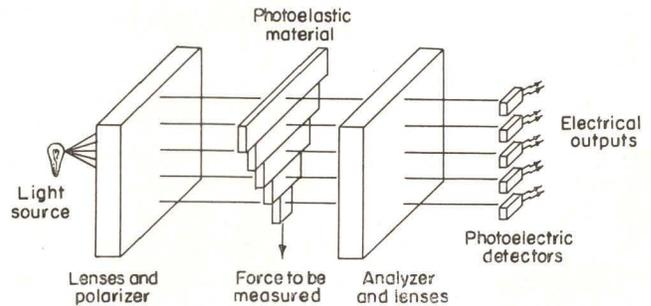
Fig. 6. Digital techniques for measuring force by the photoelastic method.
