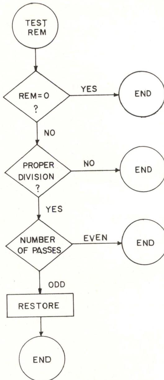
Fig. 4. Flow chart for testing remainder in the mechanical non-restoring negadecimal division algorithm.
