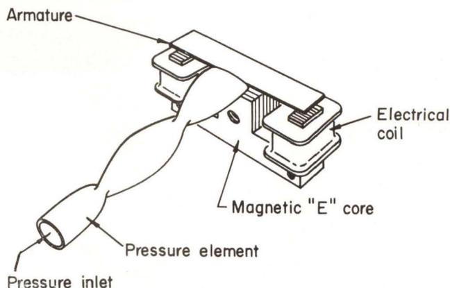
Fig. 3. The twisted-tube variable-reluctance transducer.
