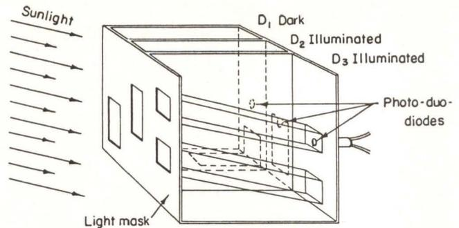
Fig. 7. Digital solar aspect sensor with Gray code light mask.
