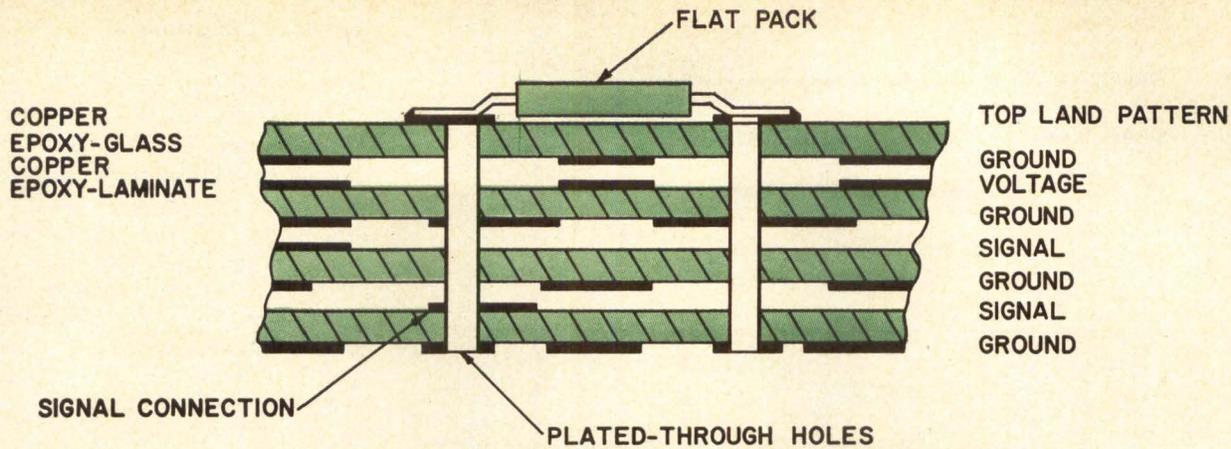
Fig. 2 Cross-sectional view of multilayer PC board
