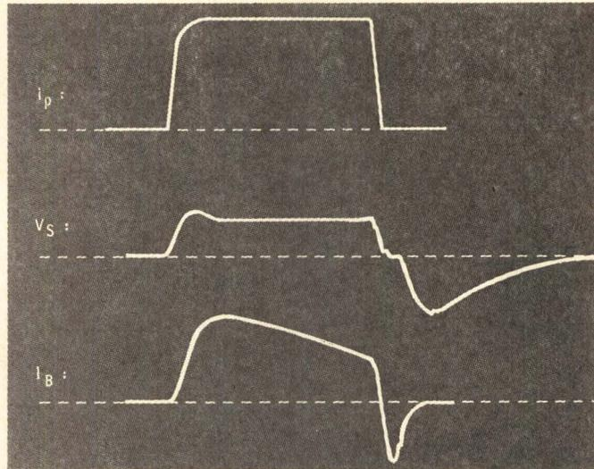
Fig. 16 Current-driven switch secondary response.
