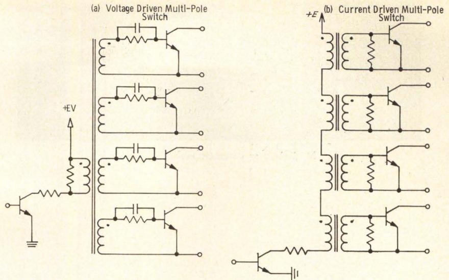
Fig. 20 Multi-pole switch configurations.
