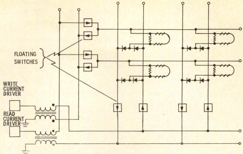
Fig. 26 Balun or common mode transformer used in current source and return circuit.
