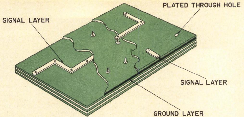
Fig. 1 Sectional view of multilayer PC board
