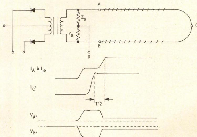
Fig. 22 Parallel line termination.
