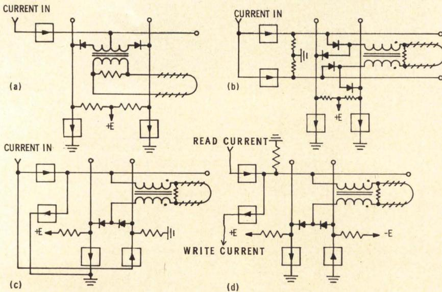
Fig. 25 Examples of transformer-diode matrices.
