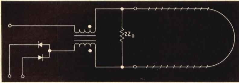
Fig. 23 Balun or common mode line coupling.
