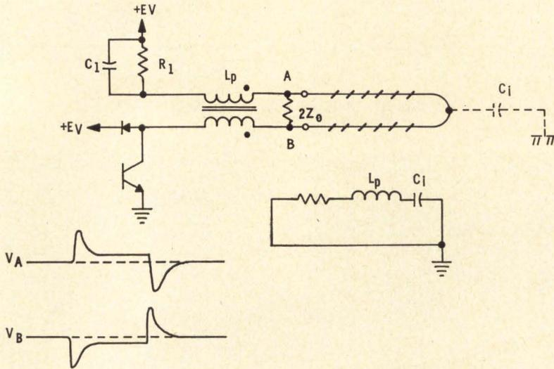
Fig. 24 Inhibit line coupling.
