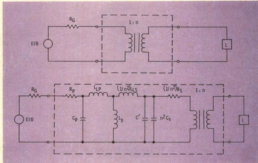
Fig. 1 Pulse transformer and general equivalent circuit.
