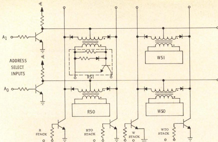
Fig. 18 Current-driven switch with turn-off drive.
