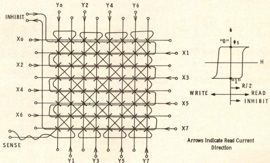
Fig. 8 Coincident-current plane wiring configuration.
