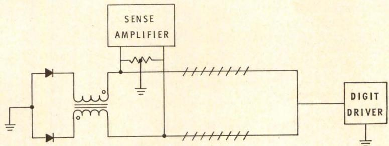
Fig. 28 Common sense-digit line with current splitting transformer.
