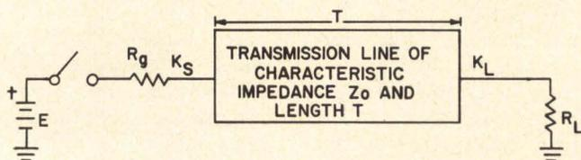
Fig. 5 Equivalent circuit
