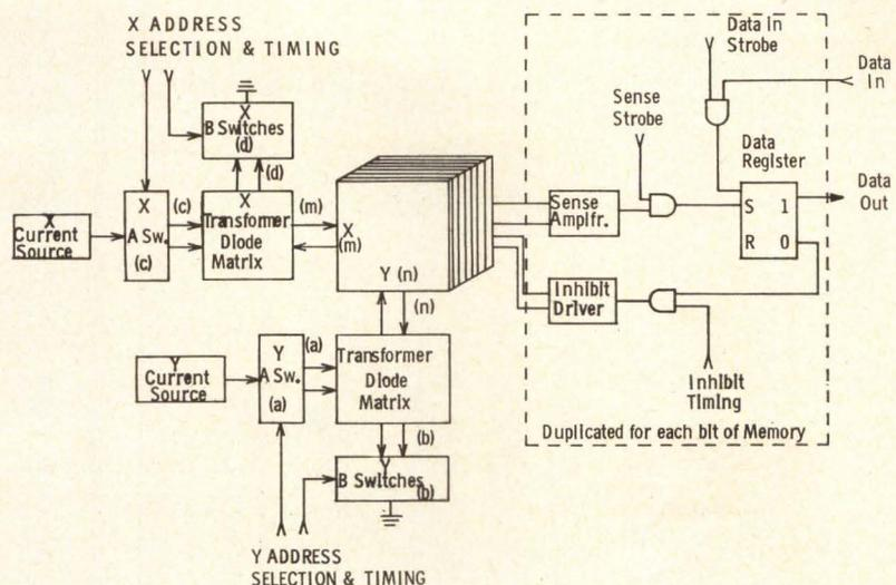
Fig. 10 Coincident-current memory system.
