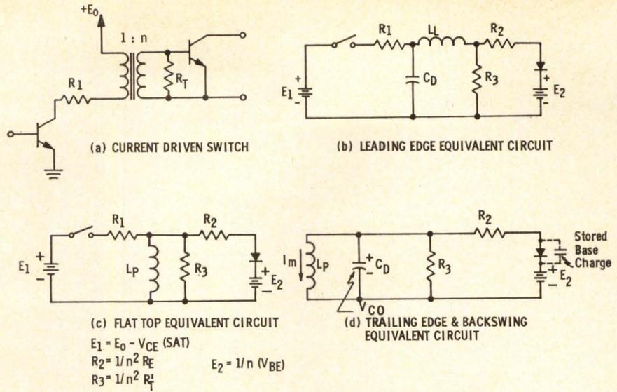
Fig. 15 Current-driven switch analysis.
