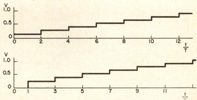
Fig. 9 Step-function generator with source impedance of 500 ohms driving an unterminated line
