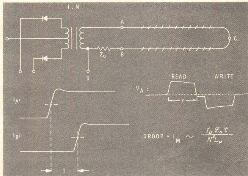
Fig. 21 Series line termination.
