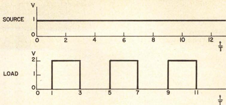
Fig. 6 Zero-impedance step-function generator driving an unterminated line
