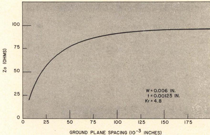
Fig. 4 Z<sub>0</sub> vs. ground plane spacing
