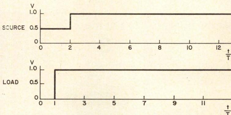
Fig. 8 Step-function generator of impedance  $Z_0$  driving an unterminated line
