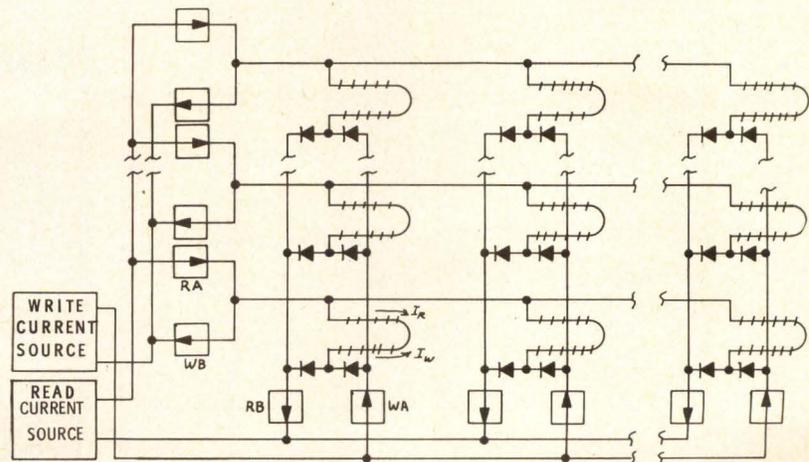
Fig. 11 Diode matrix with floating switches.
