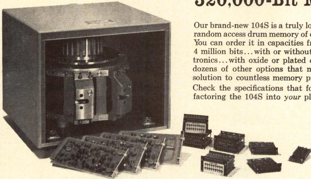
Our brand-new 104S is a truly low-cost, universal, random access drum memory of computer quality. You can order it in capacities from  $\frac{1}{4}$  million to 4 million bits...with or without read/write electronics...with oxide or plated drum...and with dozens of other options that make it the ideal solution to countless memory problems.
