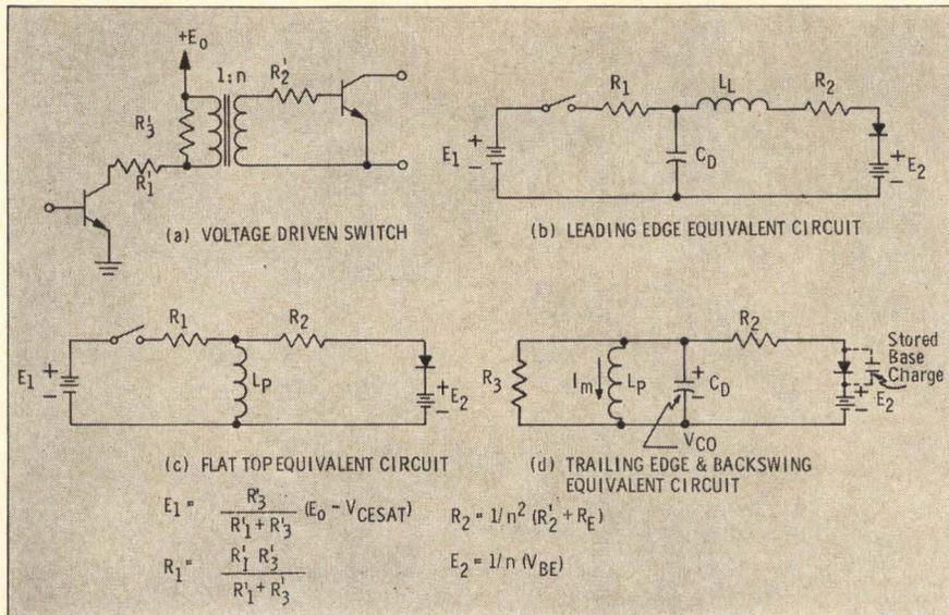
Fig. 13 Voltage-driven switch analysis.
