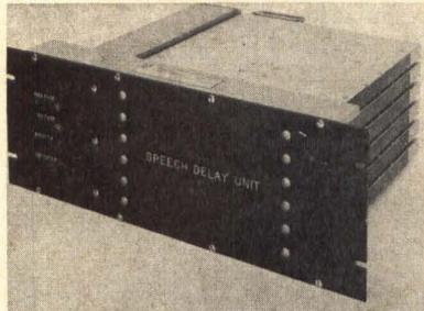
The DDI Analog Delay System imposes precise time delay of analog information using combined analog and digital techniques. System illustrated delays speech 60 msec. Longer delays are achieved by using additional digital delay lines. Applications include sonar data processing, speech and analog data transmission and autocorrelation.
