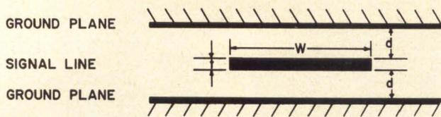
Fig. 3 Tri-plate construction
