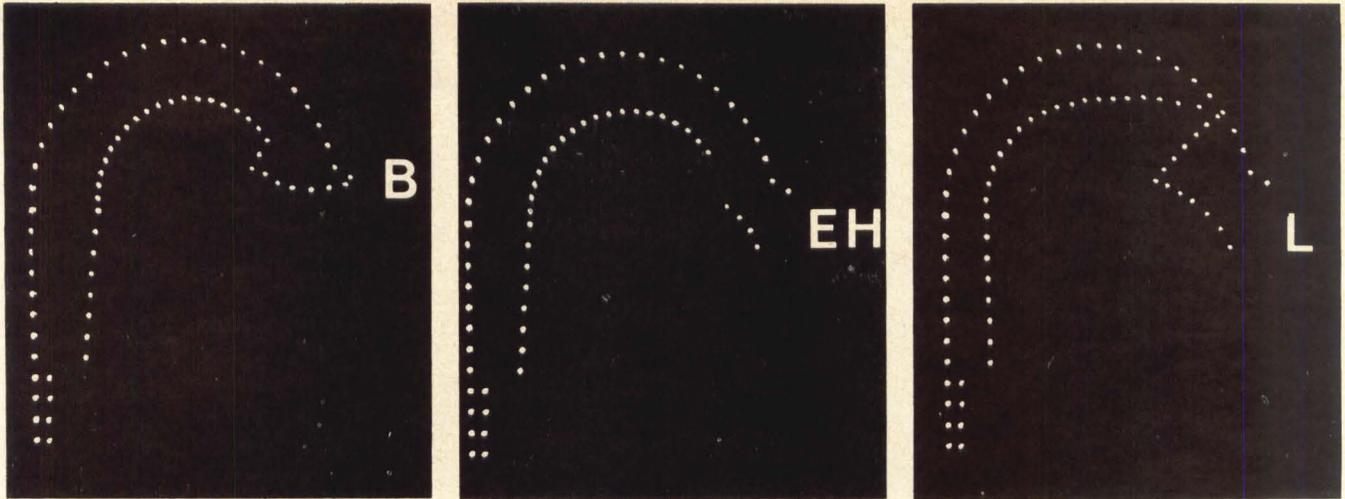
A computer-generated display of the vocal tract shows the changes in the position of the tongue, lips, and pharynx on an oscilloscope as the word "Bell" is spoken.
