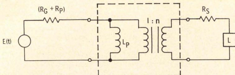
Fig. 5 Low-frequency equivalent circuit (flat-top period).
