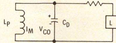
Fig. 6 Fall and backswing equivalent circuit (primary open-circuit).
