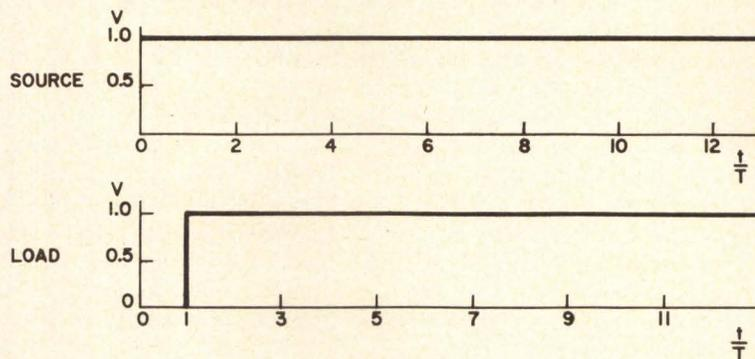
Fig. 7 Zero-impedance step-function generator driving a line terminated in  $Z_0$
