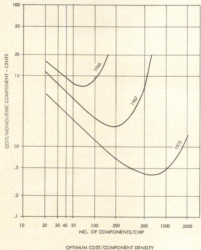
polar transistor NAND gates. At the existing rate of improvement in fabrication technology, optimum chip complexity will double in 1967 and is expected
