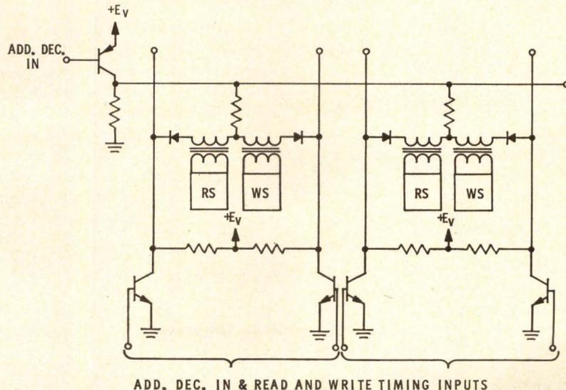
Fig. 17 Example of voltage-driven switch, driven from matrix.
