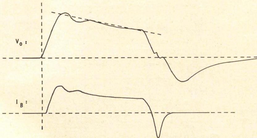
Fig. 14 Voltage-driven switch secondary response.
