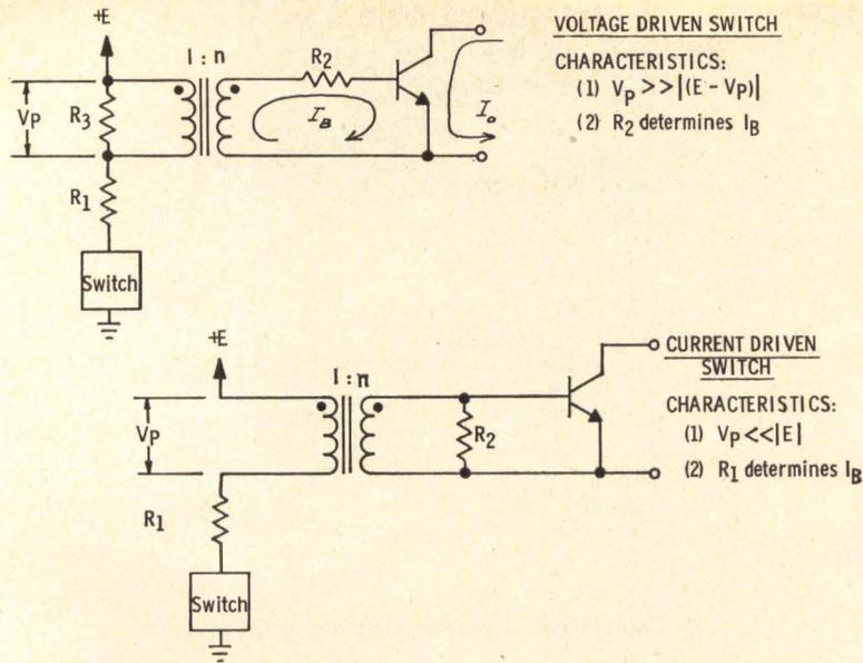
Fig. 12 Voltage- and current-driven switches.
