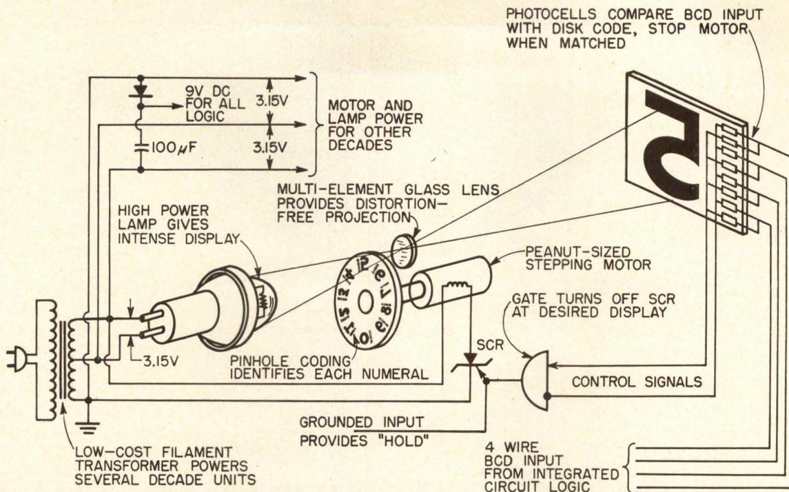
further pulses to the stepping motor are shut off. The stepping motor then stops with its detent holding the desired numeral in view until a further updating is required.
