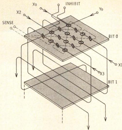
Fig. 9 Coincident-current stack wiring configuration.
