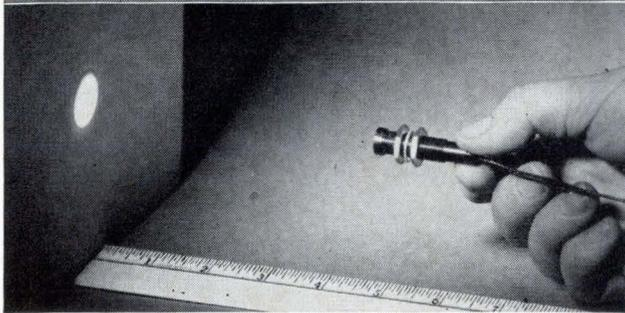
This new family of beam emitters, designed to activate photosensors, projects a narrow, intense and uniform cone of energy to an area approximately  $\frac{3}{4}$ " in diameter at a distance of 12".
