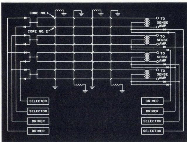
Fig. 4 The Y drive line selection is similar to that for the X lines except that the Y current drivers and the selector switches must handle twice the current, since they provide current for two lines. The Y selection matrix requires four diodes for each pair of lines because current must be driven in both directions. For the purpose of illustration, a 2 x 2 matrix is shown, but the same scheme is used for the 8 x 4 matrix of the actual system.
