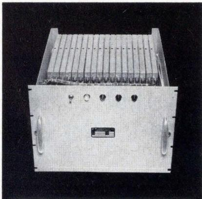
Microsonics has proven capabilities and facilities to design and build reliable ultrasonic storage systems at high information rates (up to 100 mc) which gives long term service in difficult environments of shock, vibration, and temperature. These systems have the capability of handling digital signals for computer storage or analog information as in radar signal processing.
