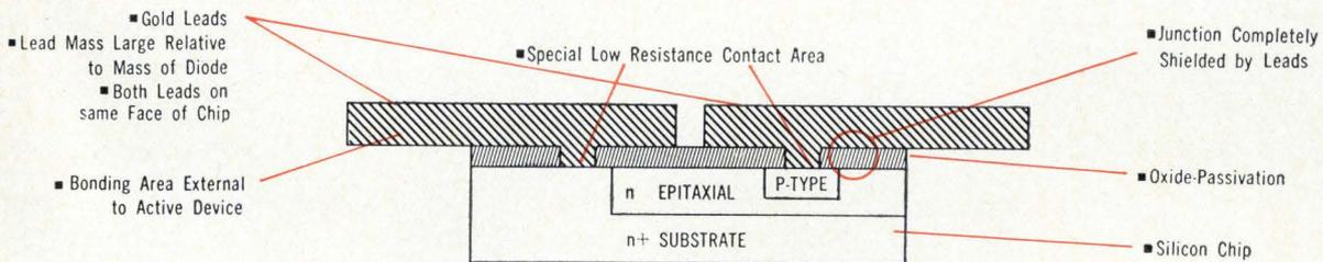
General Instrument's **HERCULEADS** beam-lead diode is a self-contained diode package with total environmental immunity—the smallest discrete diode available—and it is virtually indestructible.
