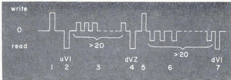
Fig. 3 Core test pulse pattern.
