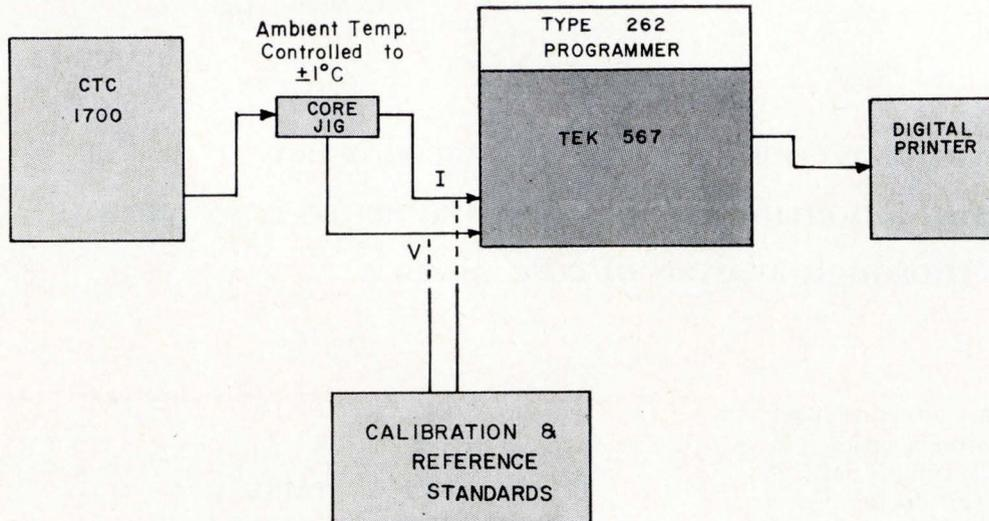
Fig. 2 Block diagram of automatic core tester. The basic parts are a Computer Test Corp. (CTC) Model 1700 programmed pulse generator, a Tektronix 567 oscilloscope with a Type 262 Programmer, a digital printer, and calibration and reference standard equipment that typically consists of a Computer Test Corp. Model 1085 Calibrator, a time mark generator, and a signal generator.
