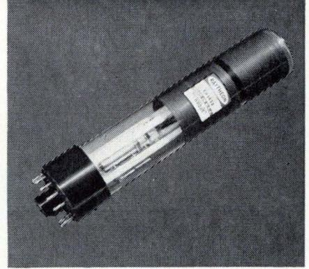
**Symbolray\* CRT Tube.** The new Raytheon CK1414 Symbolray tube provides alphanumeric inputs for computer readout devices. The tube's 2" target can be scanned electronically to select symbols, characters, and punctuation marks in sequence to form the readout on a display tube. This type has applications with data processing equipment as an economical method for generating characters for hard copy print-out or for cathode ray display. Design with 64 and 100 characters are available.
