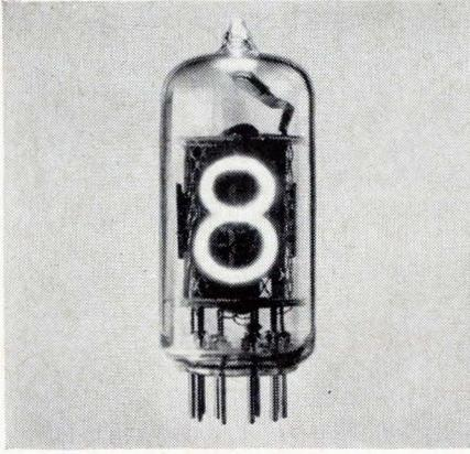
**Datavue\* Numerical Indicator Tubes in side-view configurations.** These side-view in-line visual readout tubes display singly numerals 0 through 9 or pre-selected symbols such as + and - signs. Gas-filled cold-cathode tubes, they employ the principle of the neon-glow lamp. And their life expectancies range upward of 200,000 hours in dynamic operation.
