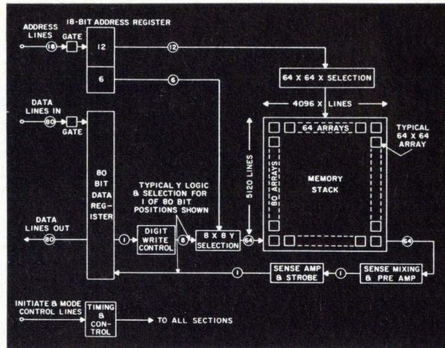
Fig. 1 Block diagram of Fabri-Tek's 2 $\frac{1}{2}$ D mass memory.
