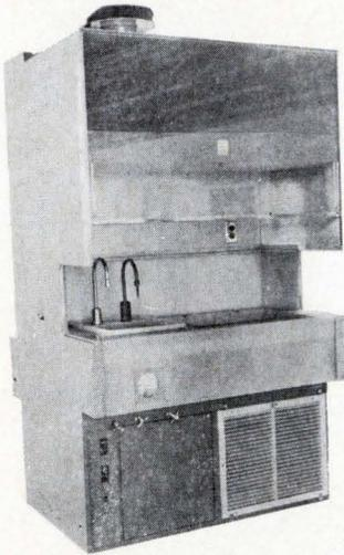
The vertical laminar flow hood having a top mounted HEPA filter and a perforated work surface through which the clean air flows is one of the most versatile of any of the existing types of clean hoods.
