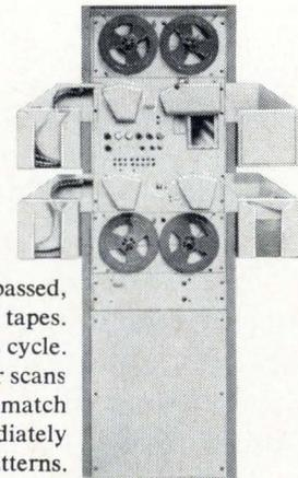
The Roytron 8001 Verify-Duplicate System. An unsurpassed, low cost, one-pass system for producing *verified* duplicate punched tapes. Three readers and one punch duplicate and verify in one continuous cycle.
