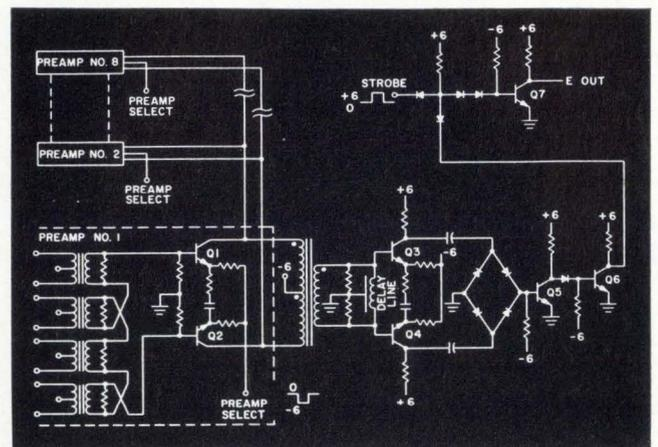
Fig. 5 Sense amplifier used in new memory system.
