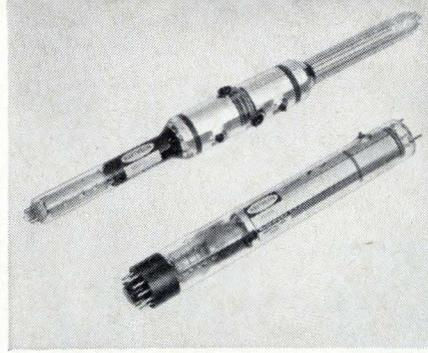
**Recording Storage Tubes.** Raytheon recording storage tubes are electronic input/output cathode ray storage devices. Applications include radar scan-conversion, slow-down video, signal processing, signal enhancement, time delay, and stop motion. Types include single gun and dual gun—standard and miniature sizes. Shown above are miniature single-gun (CK1516) and dual-gun (CK1519) storage tubes, which provide high resolution and erase capability of 1.2 seconds.
