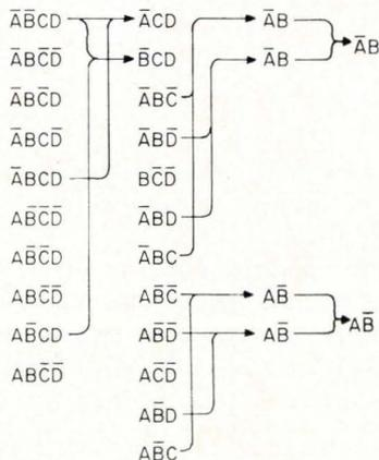
Now continue with the new list as shown in the right-hand column of figure above. When the process can be carried no further, the unchecked terms are prime implicants:  $\bar{A} C D$ ,  $B C D$ ,  $B \bar{C} \bar{D}$ ,  $A \bar{C} \bar{D}$ ,  $\bar{A} B$ ,  $A \bar{B}$ .
