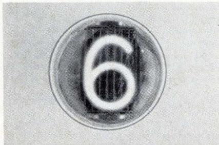
**Datavue\*End-View Tubes.** Raytheon end-view Datavue tubes have essentially the same characteristics as side-view types. They fit into standard-size receptacles and conform to EIA ratings. Models include round (CK8421) and rectangular (CK8422). Both models are designed for ultra-long life, with an expectancy of 200,000 hours or more in dynamic operation.
