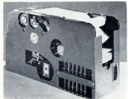
Fig. 12 Potter Instruments' Model HSP-3604 military printer.
