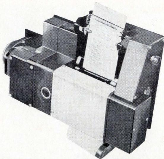
Fig. 15 Soroban Engineering's Model CT-1 printer.
