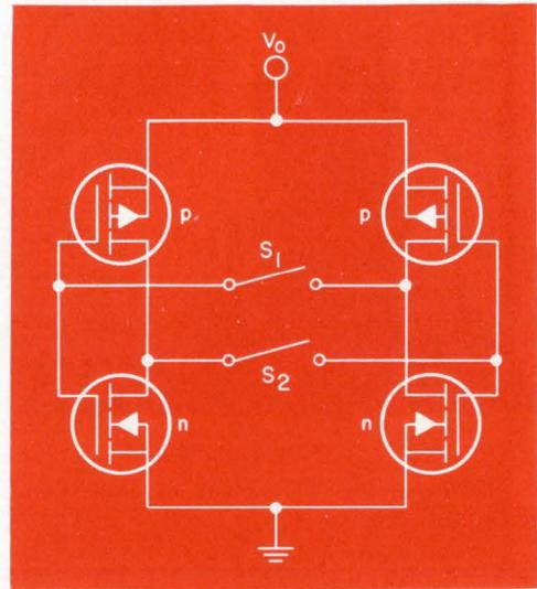
Fig. 14 Shift register stage.
