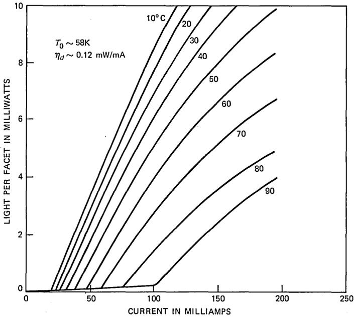
Fig. 14—Light-current characteristics of a CSBH laser emitting at 1.55  $\mu\text{m}$ .
