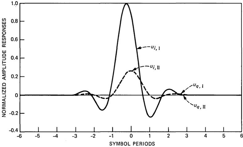
Fig. 3—16-QAM signal, time-domain impulse responses for a notch-centered fade.
