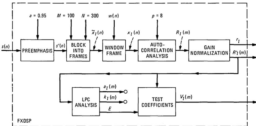
Fig. 1—Signal processing for extracting LPC features for recognition.
