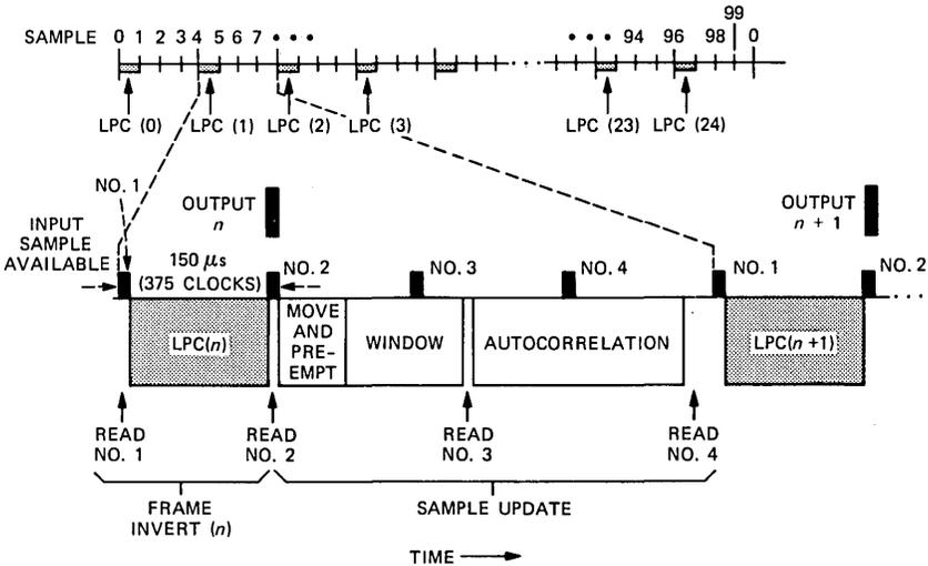
Fig. 5—Timing of input, output, and program sections.
