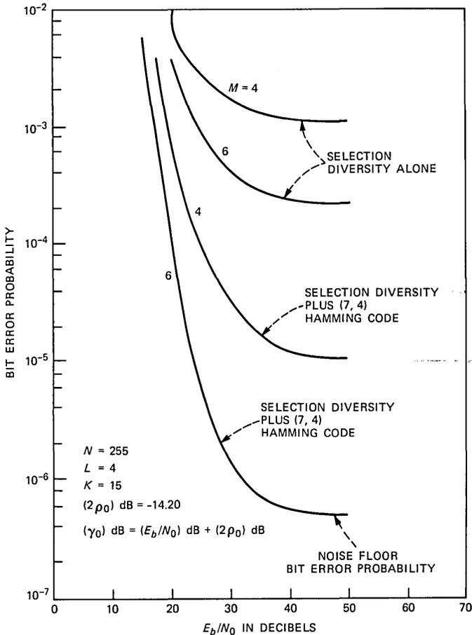
Fig. 9—Bit error probability as a function of  $E_b/N_0$  for  $M = 4$  and  $M = 6$ .
