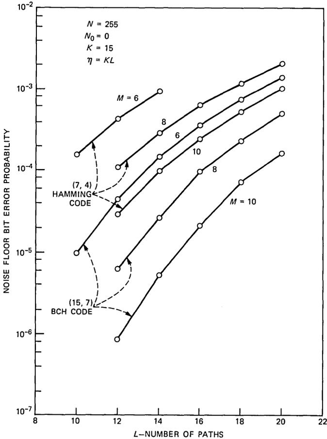
Fig. 8—Noise floor error probability for the (7, 4) Hamming code and (15, 7) BCH code for various orders of diversity.
