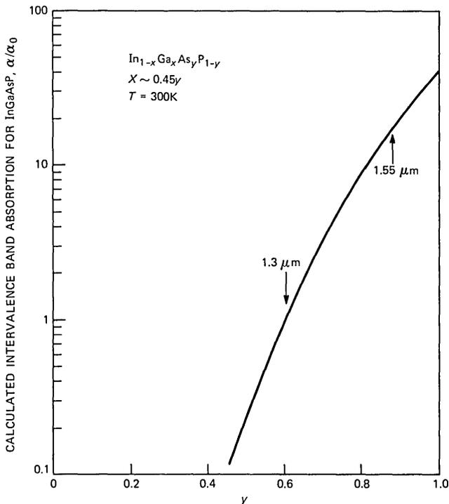
Fig. 7—The calculated intervalence band absorption from Ref. 8 normalized to its value for 1.3  $\mu\text{m}$ .
