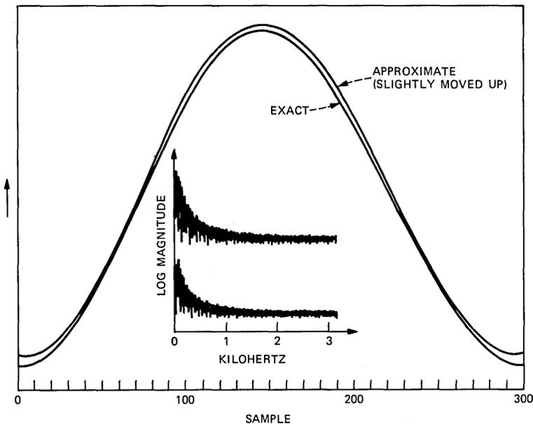
Fig. 6—Comparison of exact and Taylor series approximation of Hamming window.
