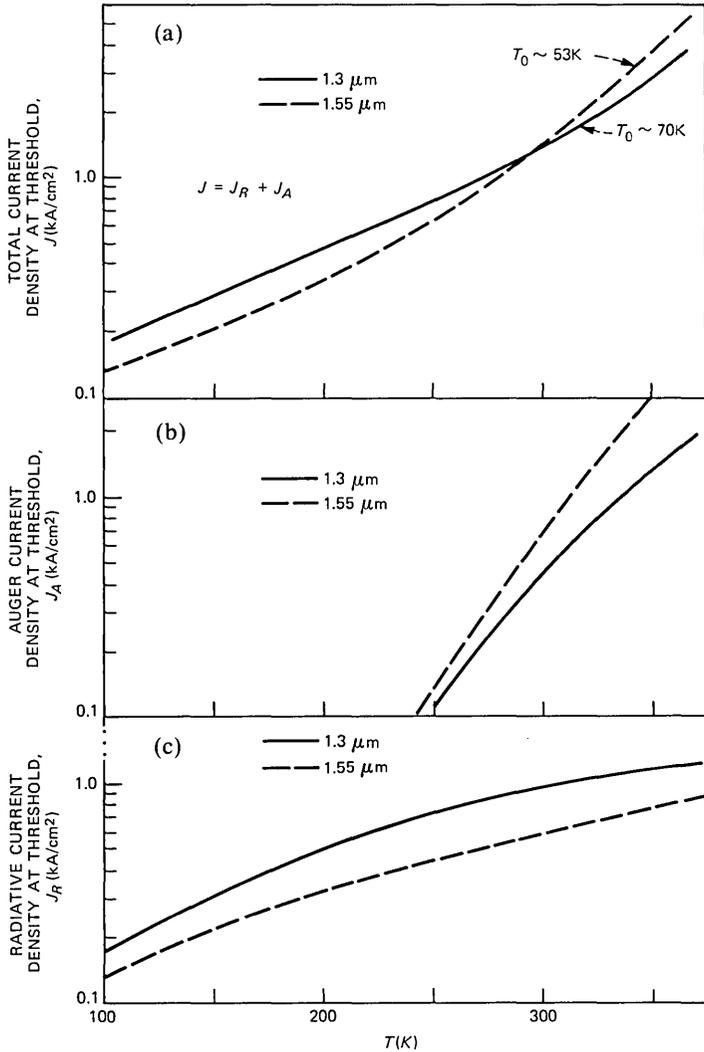
Fig. 4—The calculated radiative and Auger component of the current for lasers emitting at 1.3 and 1.55  $\mu\text{m}$ . (a) Radiative. (b) Auger component. (c) Total.
