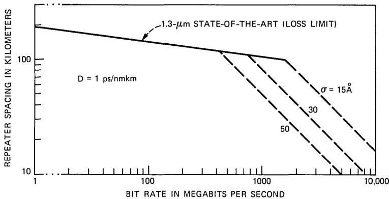
Fig. 15—Bit rate versus repeater spacing for lightwave systems operating near 1.3  $\mu\text{m}$ .
