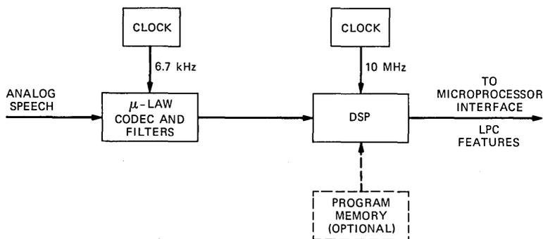
Fig. 2—LPC feature measurement hardware.
