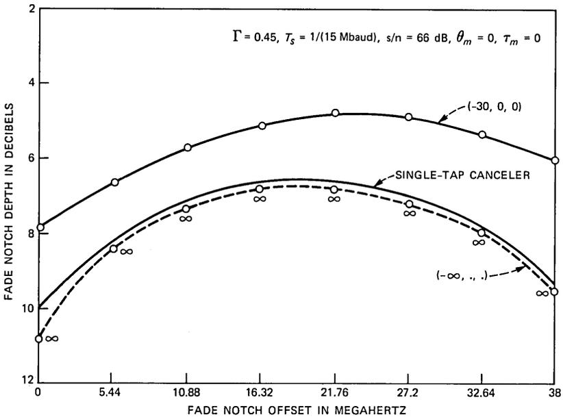
Fig. 10—Canceler performance in dual-polarized 64-QAM radio for a 30-dB flat fade on cross-coupled interfering path.
