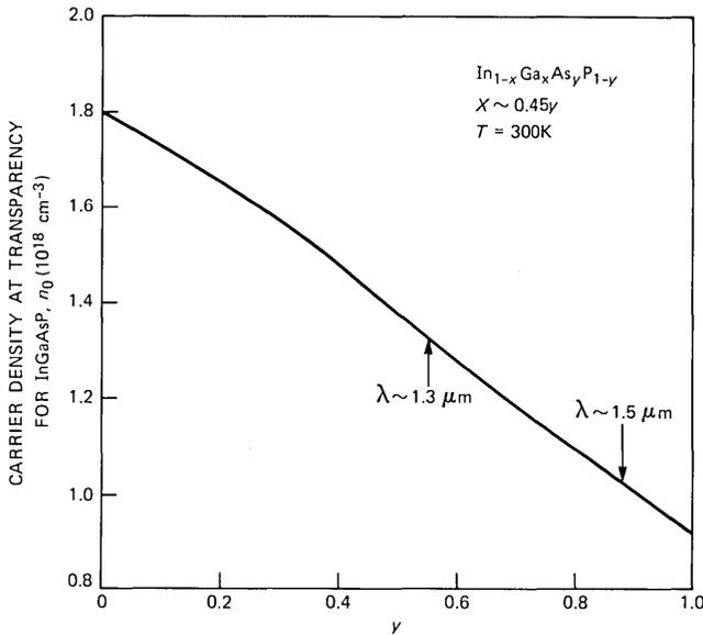
Fig. 3—The injected carrier density at transparency for undoped InGaAsP.
