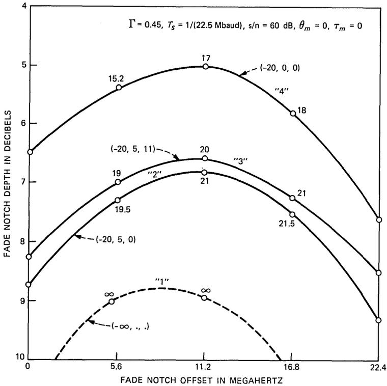
Fig. 5—Performance signature curves for dual-polarized 16-QAM radio.
