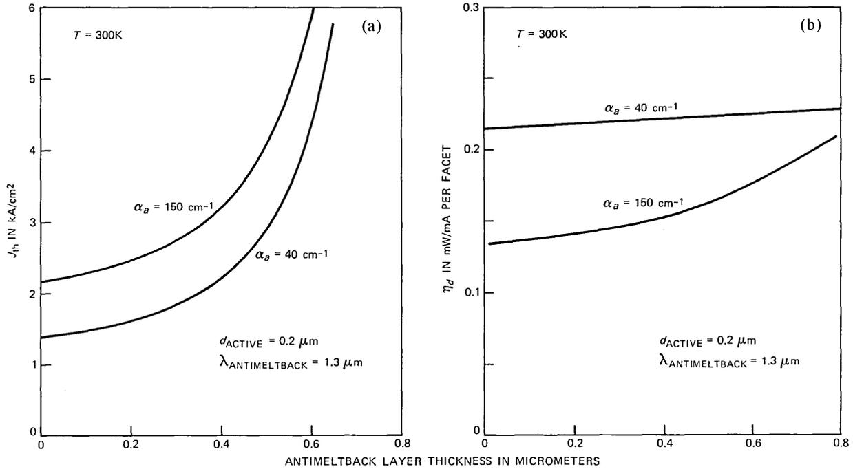
Fig. 8—The (a) threshold current and (b) external differential quantum efficiency as a function of the thickness of the antireflection layer.
