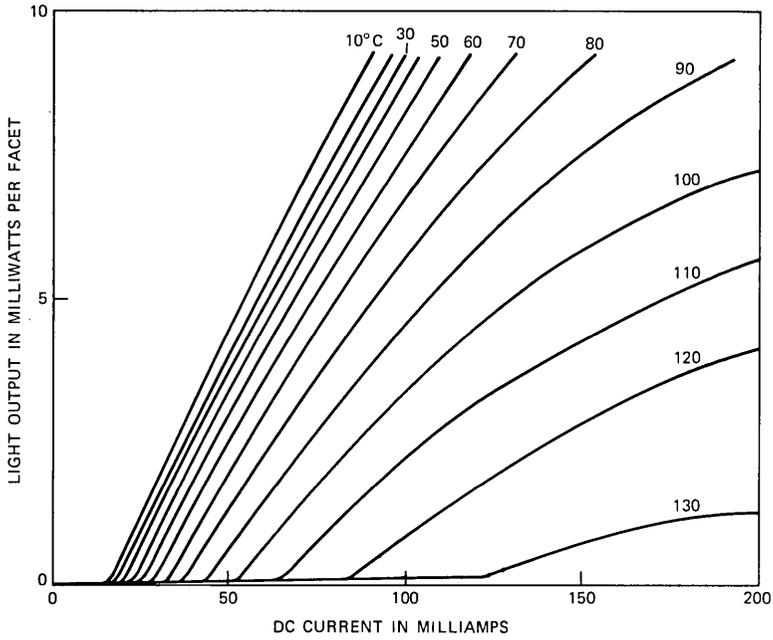
Fig. 10—Light-current characteristics of a DCPBH laser emitting at 1.3 μm.
