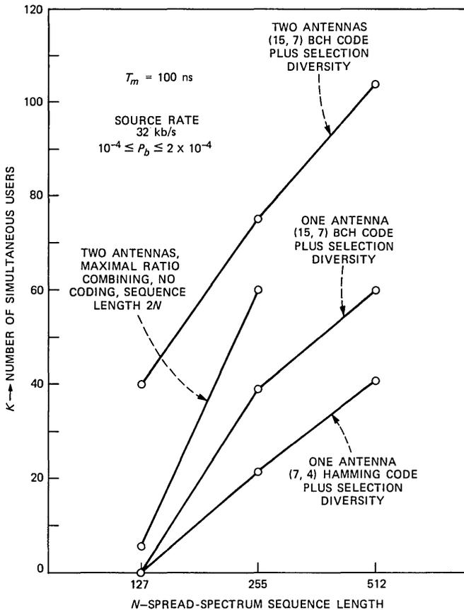
Fig. 12—Number of simultaneous users versus spread-spectrum sequence length when  $T_m = 100$  ns.
