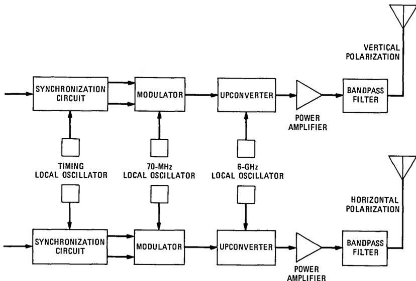
Fig. 2—A dual-polarized system transmitter.
