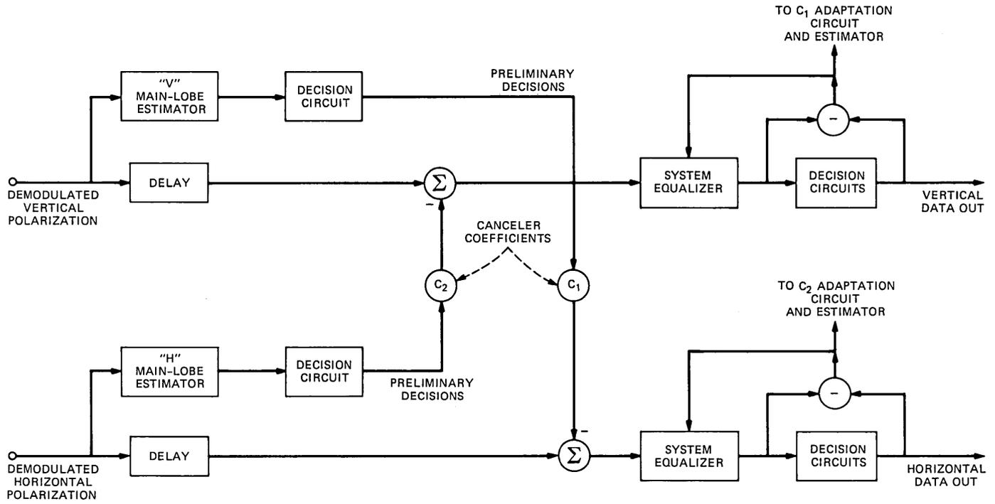
Fig. 6—Cross-polarized canceler/equalizer structure.
