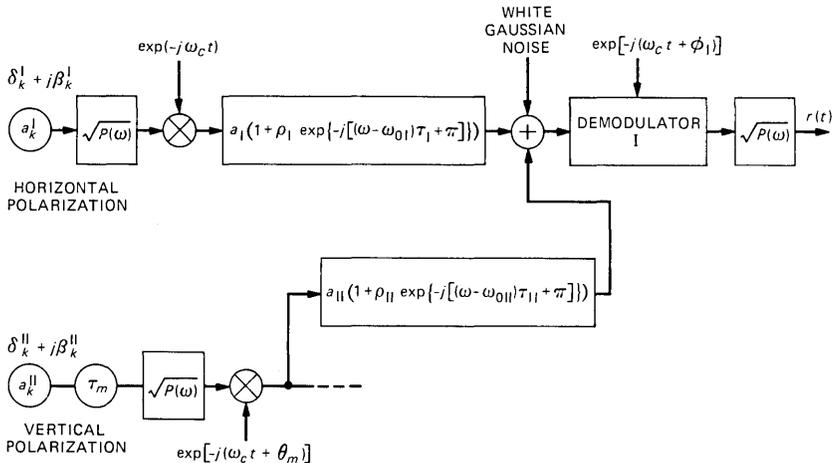
Fig. 1—Channel model for a dual-polarized system.
