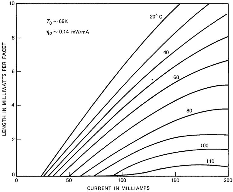
Fig. 11—Light-current characteristics of a DCPBH laser emitting at 1.55 μm.
