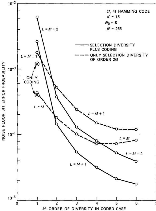
Fig. 5—Comparison of selection diversity plus coding versus selection diversity alone.
