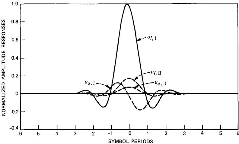
Fig. 4—16-QAM signal, time-domain impulse responses for an offset fade.
