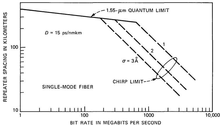
Fig. 16—Bit rate versus repeater spacing for lightwave systems operating near 1.55  $\mu\text{m}$ .
