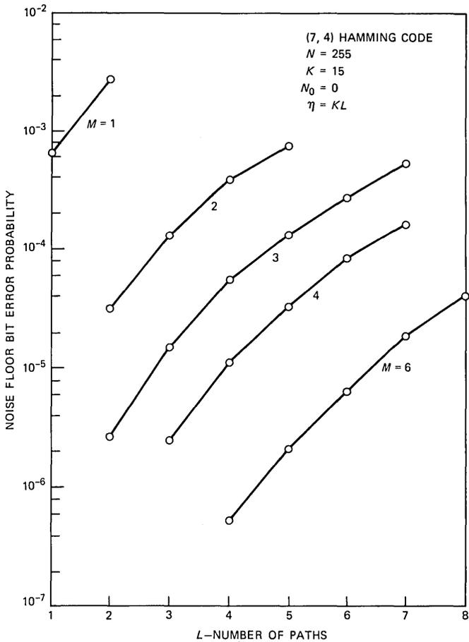
Fig. 7—Noise floor error probability for the (7, 4) Hamming code and various orders of diversity.
