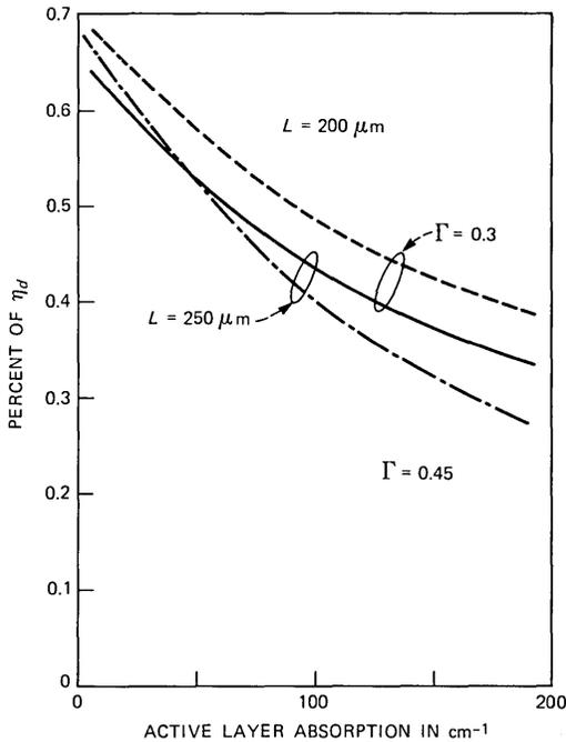
Fig. 6—The calculated external differential quantum efficiency as a function of optical loss in the active.
