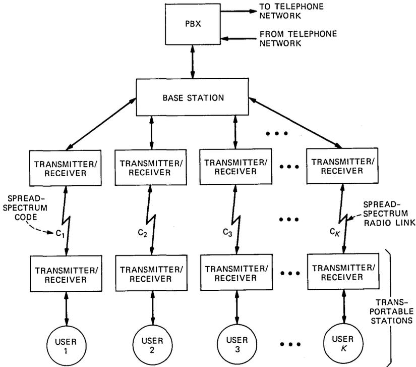
Fig. 1—A star-connected, indoor, wireless, local area network. Each user has a unique spread-spectrum code.
