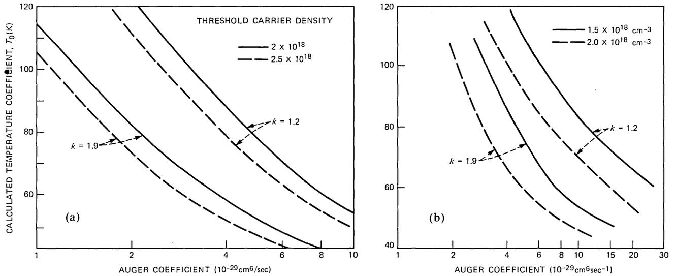
Fig. 5—The calculated  $T_0$  values as a function of Auger coefficient. (a)  $\lambda = 1.3\text{-}\mu\text{m}$  InGaAsP. (b)  $\lambda = 1.55\text{-}\mu\text{m}$  InGaAsP.
