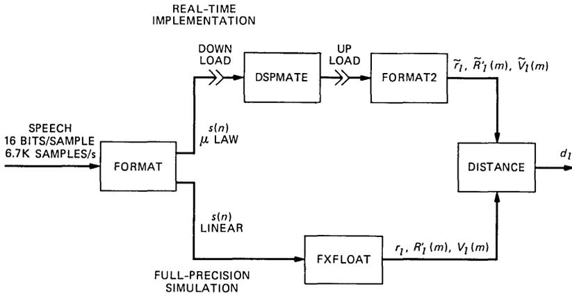
Fig. 7—Program module architecture for FXDSP verification.
