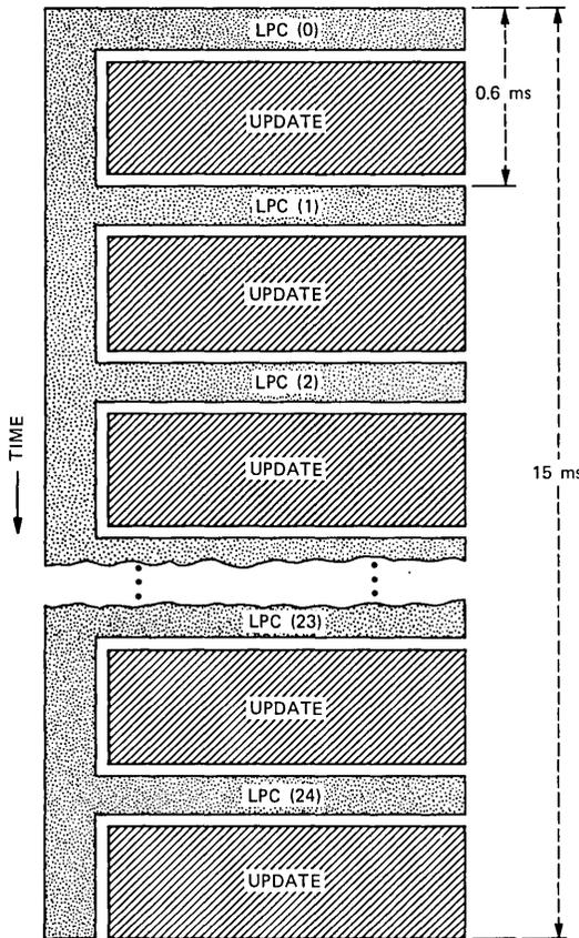
Fig. 4—Interleaving of sample update and frame-inversion programs.
