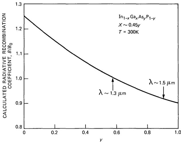
Fig. 2—The relative radiative recombination coefficient  $B/B_0$  is plotted as a function of band gap of InGaAsP.
