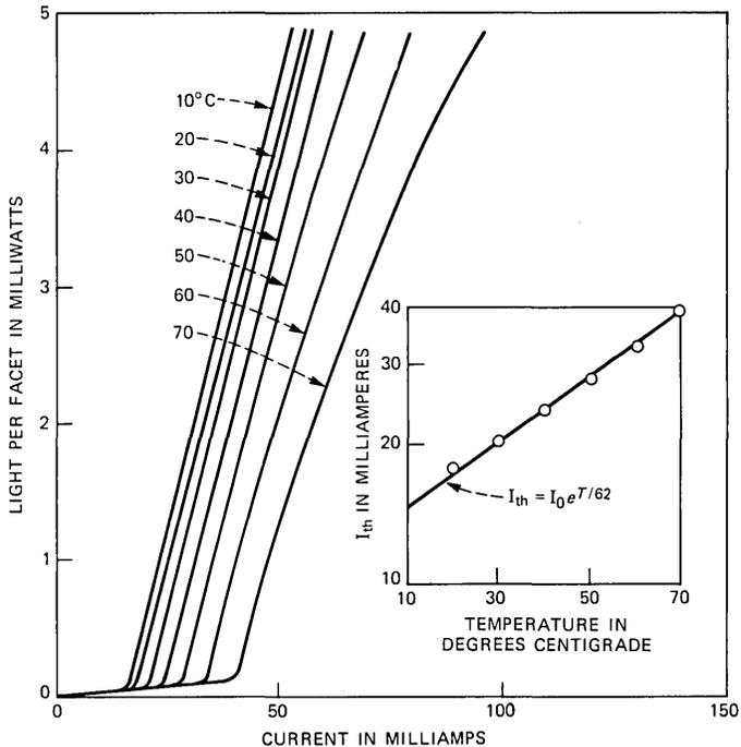
Fig. 12—Light-current characteristics of a EMBH laser emitting at 1.3  $\mu\text{m}$ .
