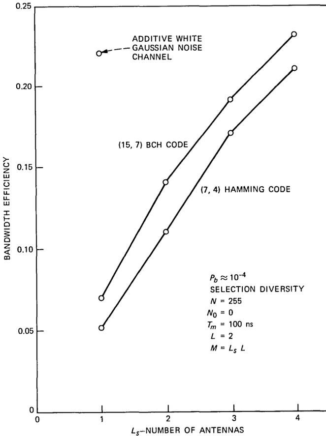
Fig. 11—Bandwidth efficiency of error-correction-coded spread-spectrum systems. For  $N = 255$ , selection diversity alone requires  $L_s = 8$  to get an efficiency of 0.11.
