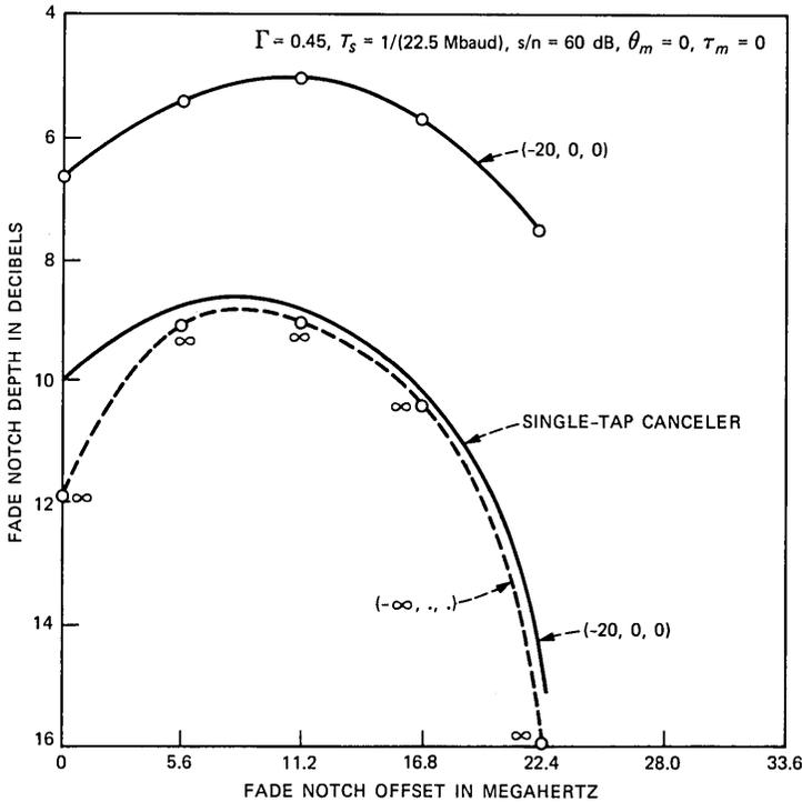
Fig. 7—Canceler performance in dual-polarized 16-QAM radio for a flat fade on cross-coupled interfering path.
