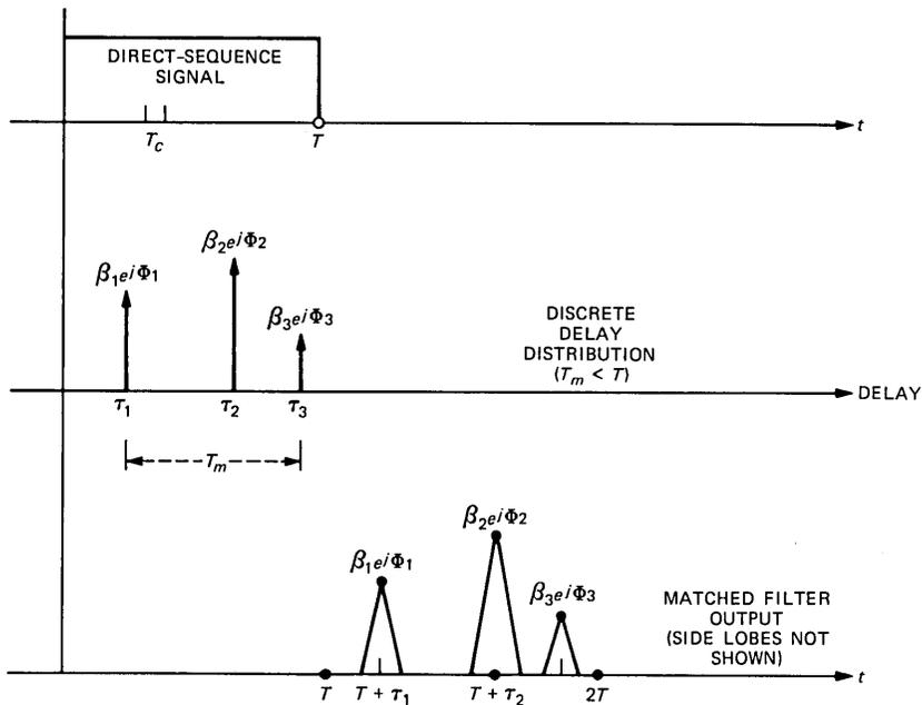
Fig. 4—Signal transmission model for a direct-sequence, spread-spectrum system and a discrete multipath model.
