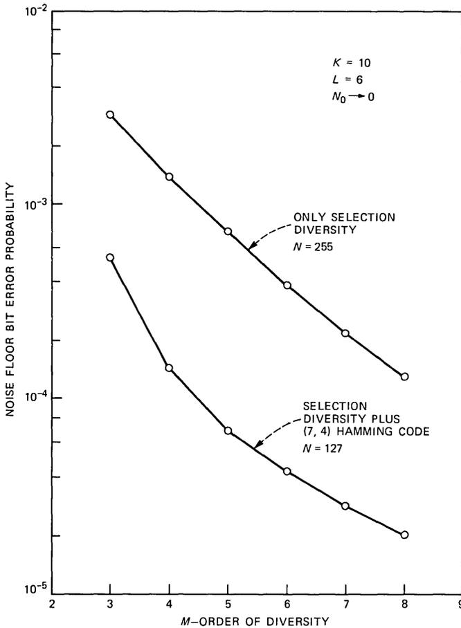
Fig. 6—Comparison of coding versus no coding in the same spread-spectrum bandwidth.
