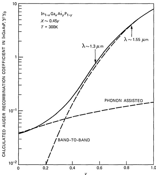
Fig. 1—The relative Auger coefficient  $\gamma/\gamma_0$  is plotted as a function of band gap of InGaAsP.
