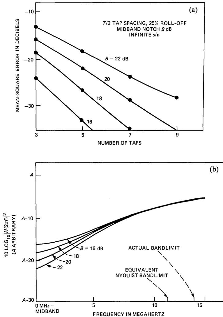
Fig. 3—(a) Steady-state mean-square error versus number of taps for quartic criterion. (b) Power transfer characteristics of channels used in computation of mean-square error<sub>1 $\infty$</sub>  for quartic algorithm.
