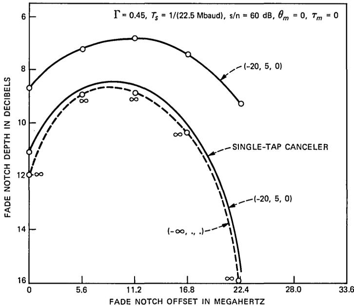
Fig. 8—Canceler performance in dual-polarized 16-QAM radio for a dispersive fade on cross-coupled interfering path.
