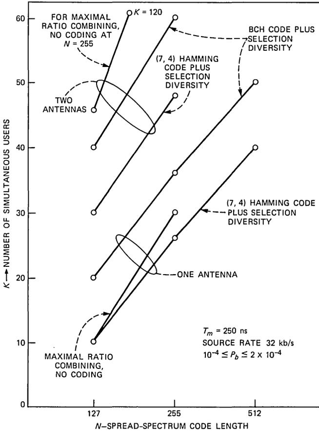
Fig. 13—Number of simultaneous users versus spread-spectrum sequence length when  $T_m = 250$  ns.
