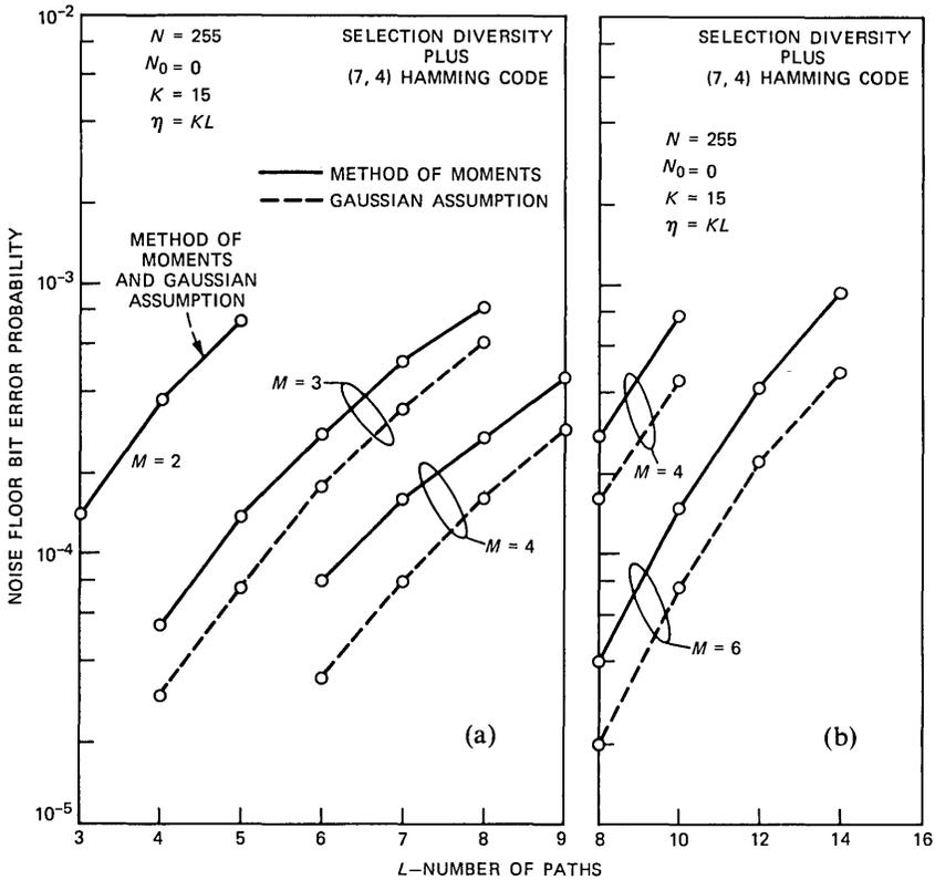
Fig. 10—The Gaussian assumption for (a) low orders of diversity and (b) high orders of diversity.
