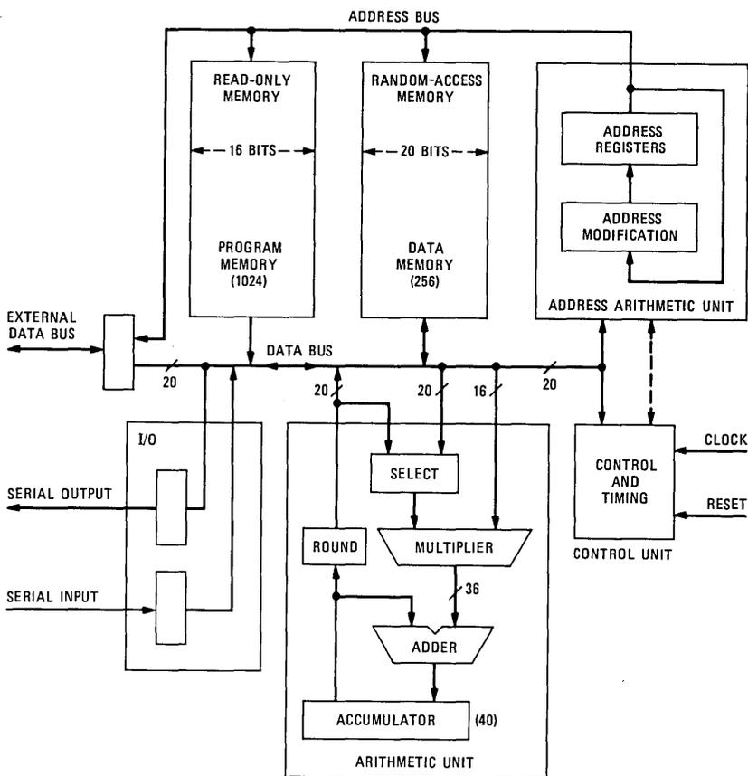
Fig. 3—Block diagram of DSP.
