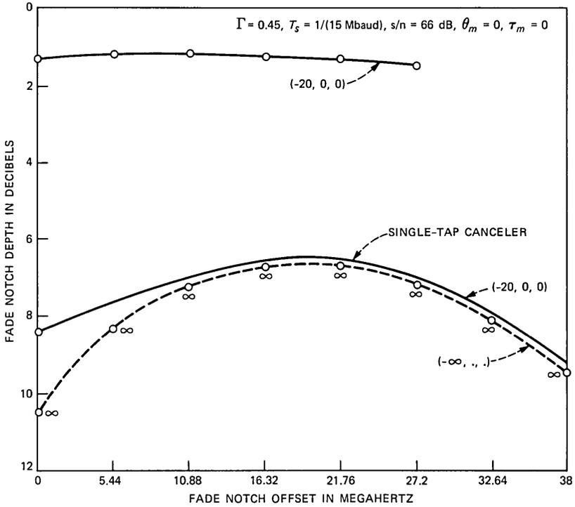
Fig. 9—Canceler performance in dual-polarized 64-QAM radio for a 20-dB flat fade on cross-coupled interfering path.
