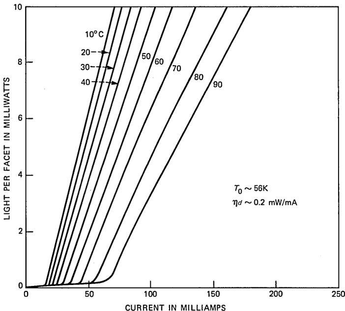
Fig. 13—Light-current characteristics of a CSBH laser emitting at  $1.3 \mu\text{m}$ .
