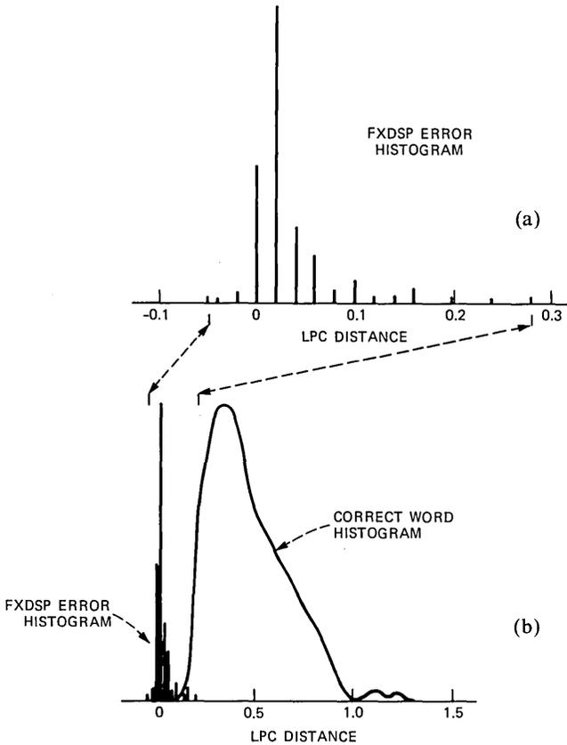
Fig. 8—Comparison of LPC distance from FXDSP to distance of correct word matches.
