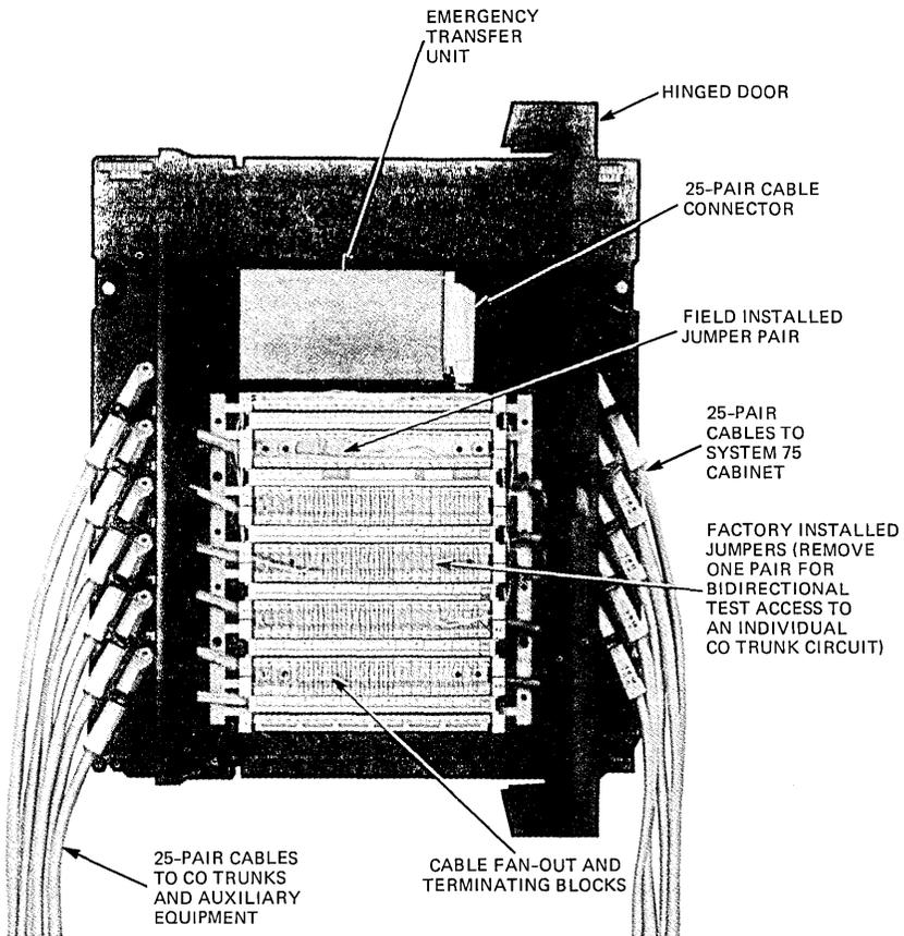
Fig. 14—Cable access panel.
