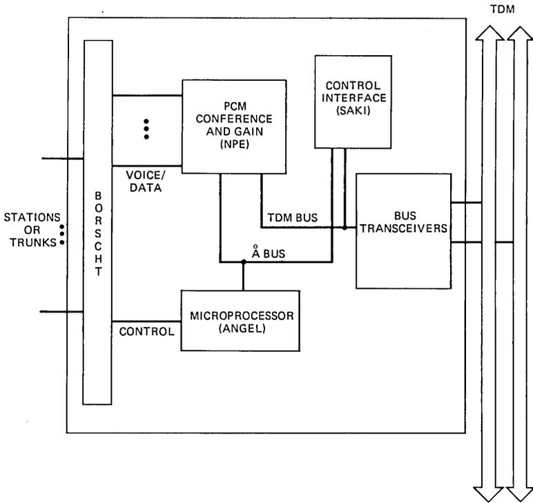
Fig. 6—Architecture of a System 75 generic port board.
