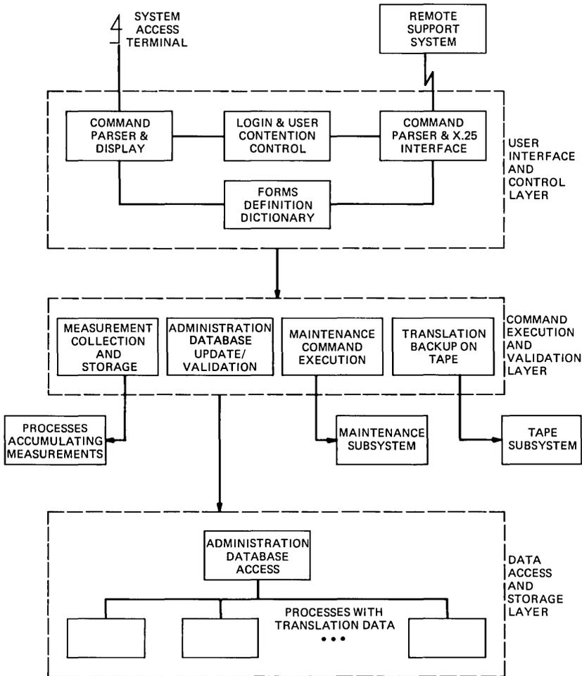
Fig. 4—System management layered software.
