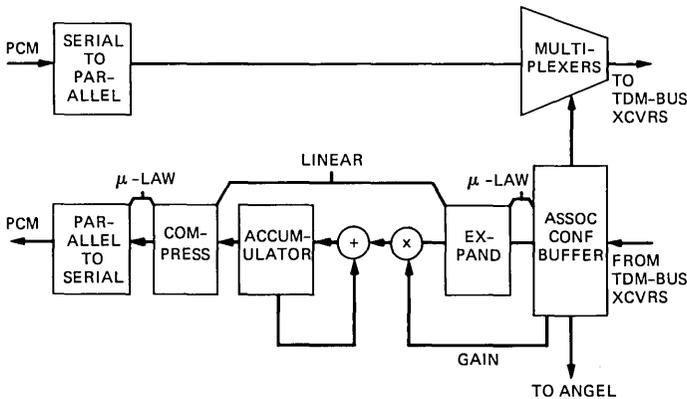
Fig. 3—Architecture of one of the network processing element's four channels.
