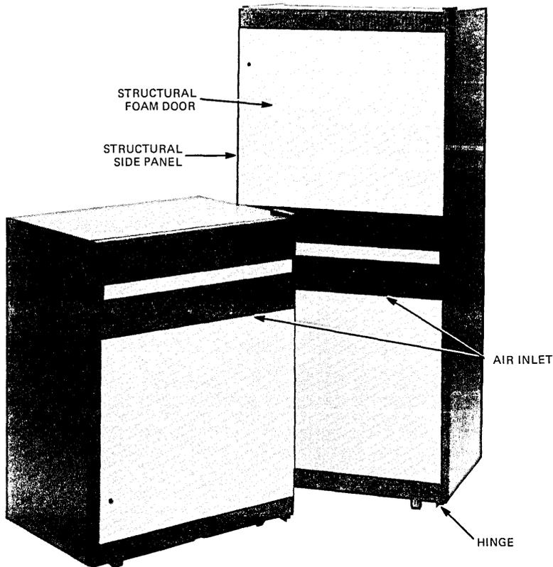
Fig. 4—Small and medium cabinet configurations.
