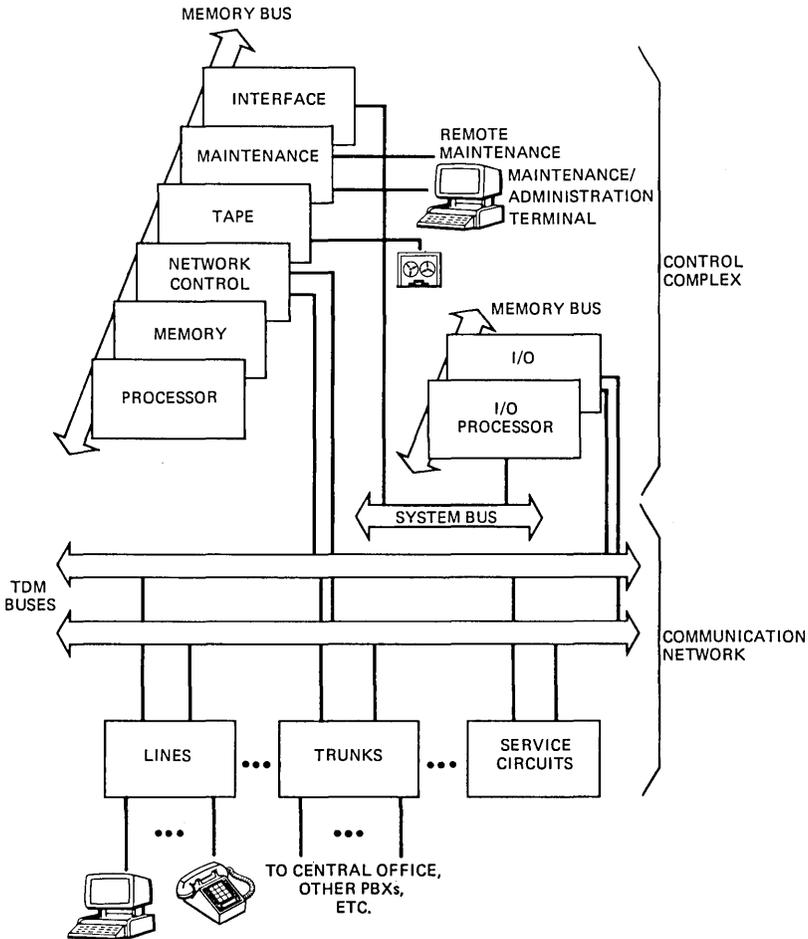
Fig. 8—System 75 communication and control architecture with I/O processor.
