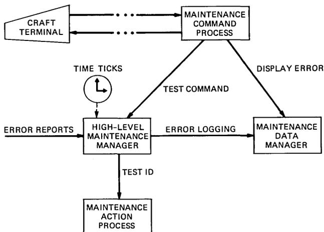
Fig. 3—Maintenance software architecture.
