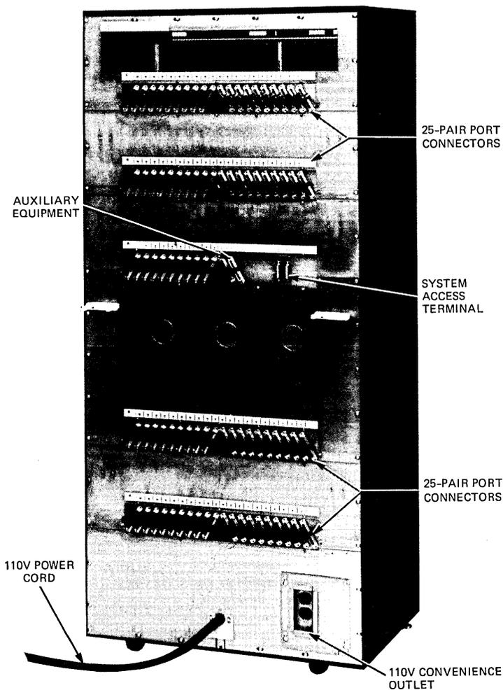
Fig. 10—Equipment cabinet external interfaces.
