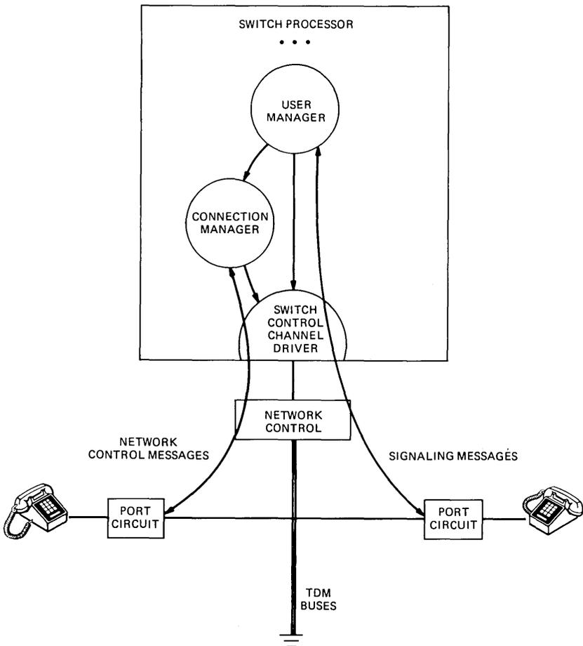
Fig. 5—Communications network control.
