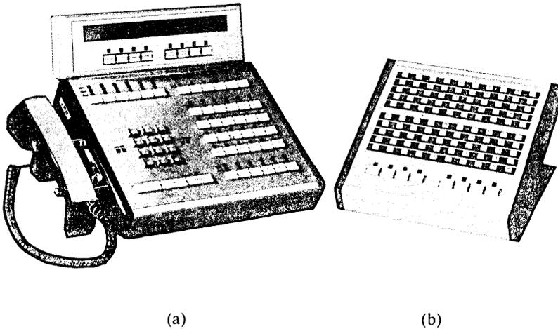
Fig. 3—(a) Basic service attendant position console. (b) Direct extension selection console.
