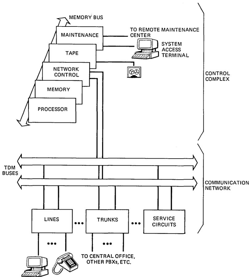
Fig. 1—System 75 communication and control architecture.
