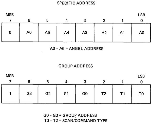
Fig. 2—Addressing modes of TDM bus control channel.
