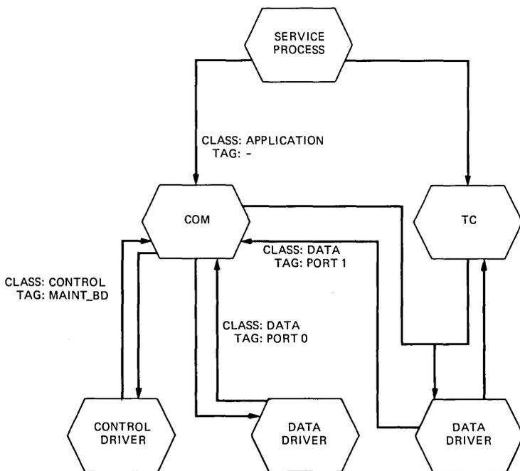
Fig. 7—Communications subsystem processes and paths for a service process with access to port 1 of the maintenance board.
