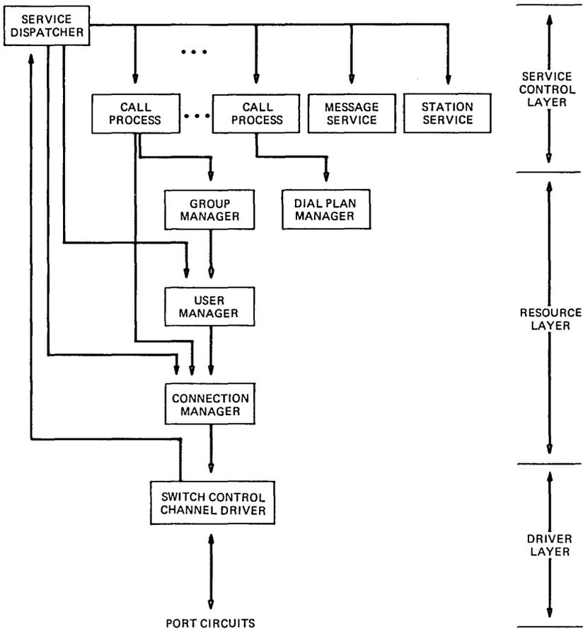
Fig. 3—Switch services software structure.
