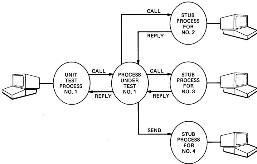
Fig. 6—Process test environment.
