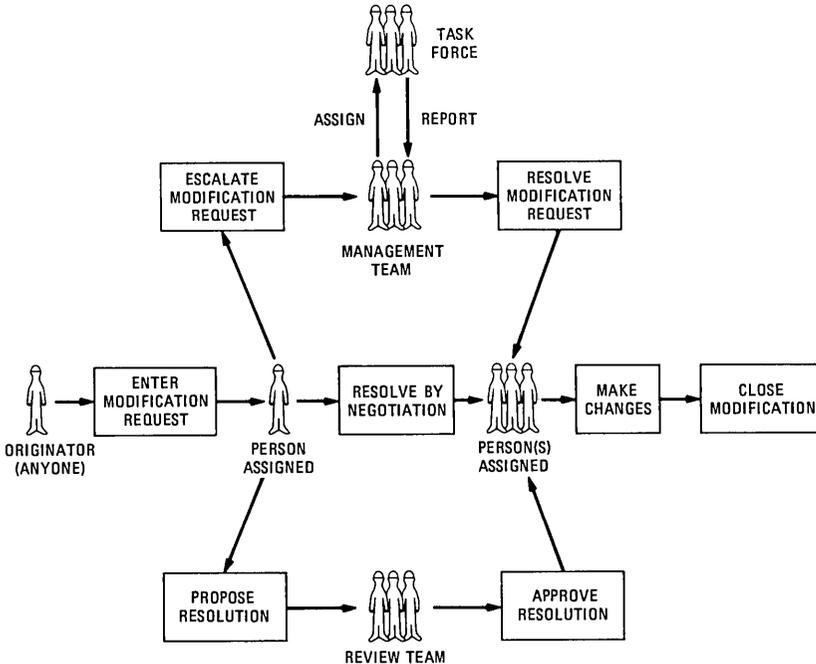
Fig. 5—Resolution process for modification requests.
