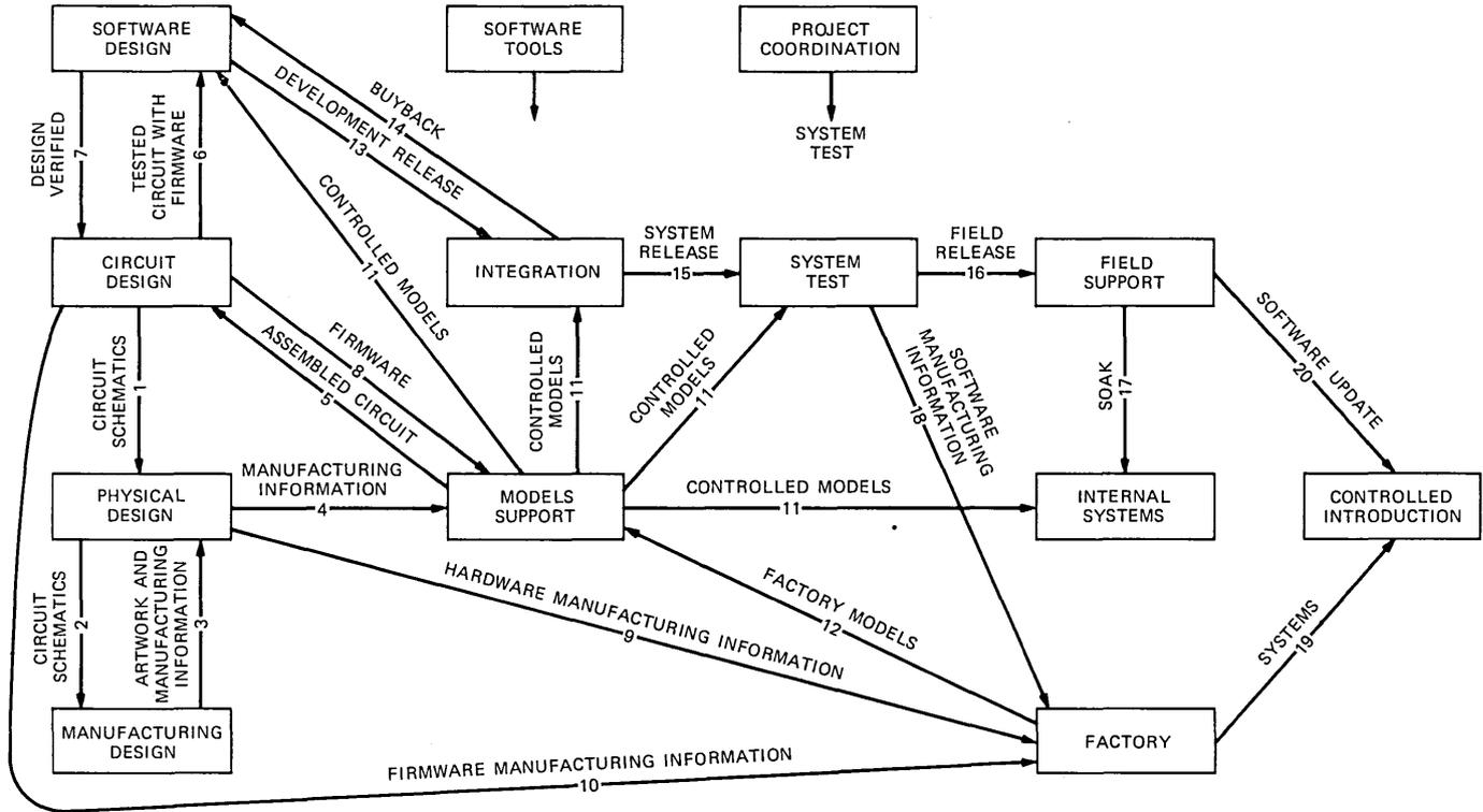
Fig. 3—Information flow for circuit pack design.
