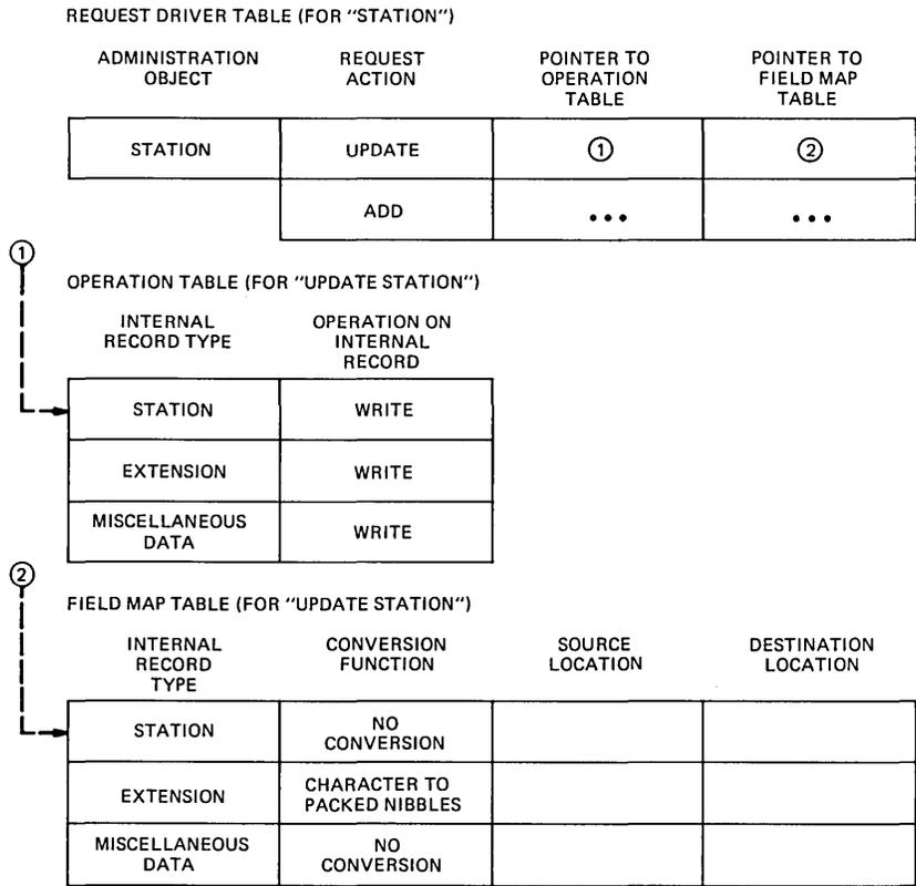
Fig. 8—Example of table-driven software.
