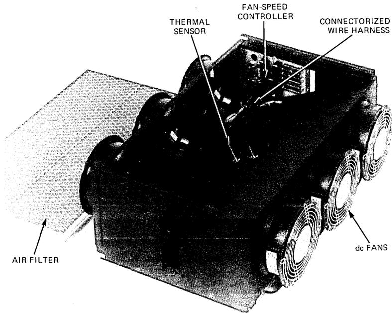
troller; and connectorized wiring to mate with power and alarm leads in the cabinet wiring harness.
