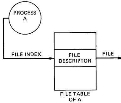
Fig. 4—The *UNIX* system implementation of files.
