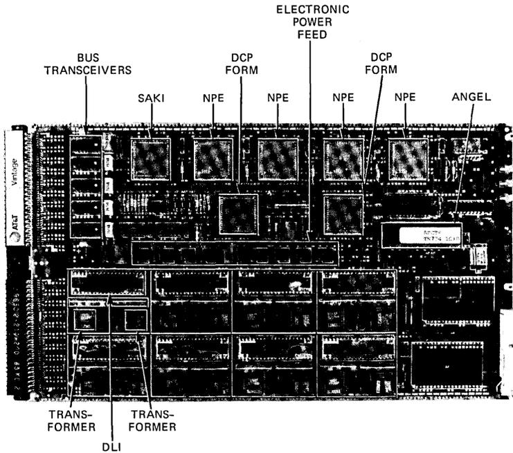
Fig. 7—Photograph of System 75 digital line circuit with major functional blocks indicated.
