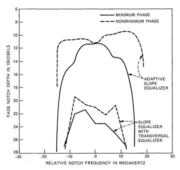
Fig. 6—DR 6 measured equipment signatures for 16-QAM digital radio. Performance for radio with adaptive slope equalization and adaptive slope and transversal equalization for 6.3-ns path delay. (Adapted from Ref. 20.)
