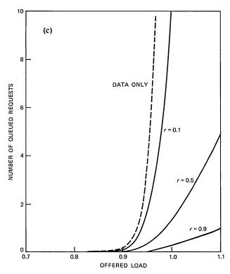
Fig. 5(c)—Mean data message queue length versus offered load for integrated systems and a single traffic system with 500 slots.
