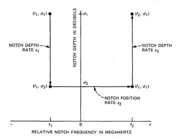
Fig. 7—Test sequence for dynamic simulation of multipath propagation.
