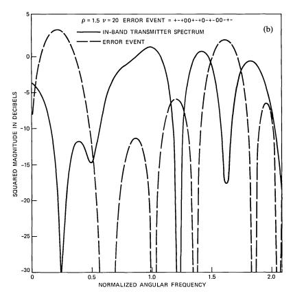
Fig. 10b—The in-band transmitter spectrum is optimized for a limited set of error events, one of which is shown. The extraordinary flexibility afforded by over one million states allows the optimum spectrum to have some peaks and valleys in opposition to those of the minimizing error event.
