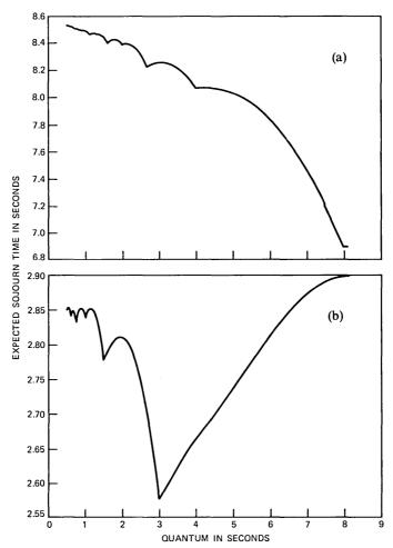
Fig. 1—Expected sojourn times as a function of the quantum for (a) type II jobs and (b) type I jobs.
