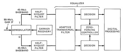
Fig. 2—Baseband receiver with adaptive transversal equalizer.
