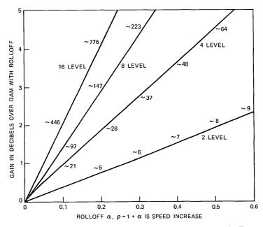
Fig. 11—Gain versus rolloff characteristics for partial response  $2^{-1/2}$  ( $\overline{0}$ , 1, 1,  $\overline{0}$ ), where the approximate number of constellation points are shown for competing QAM system, and the number of levels equals the number of states per rail.
