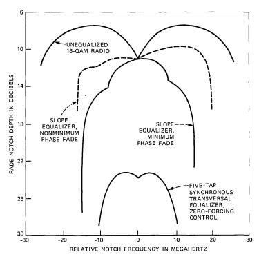
Fig. 5—DR 6 theoretical equipment signatures for 16-QAM digital radio. Performance for radio without equalization, with an adaptive slope equalizer, and with a five-tap synchronous transversal equalizer using zero-forcing control.
