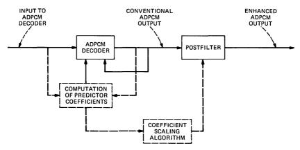
Fig. 2—Adaptive postfiltering of the output of an ADPCM decoder. The coefficients of the postfilter are scaled versions of the coefficients of the adaptive predictor in DPCM. In DPCM-APB, the predictor coefficients are obtained on the basis of observations of a recent history of decoder input and decoder output. The parts of the circuit that determine coefficient values are shown by broken lines.
