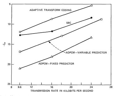
Fig. 6—Objective noise-to-signal measure,  $\ell_m,$  averaged over 16 articulation bands for the 12 coders in Fig. 6.
