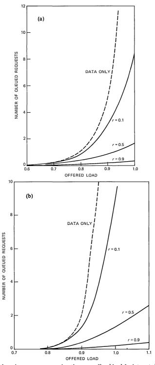
Fig. 5—Mean data message queue length versus offered load for integrated systems and a single traffic system with: (a) 20 slots, and (b) 100 slots.
