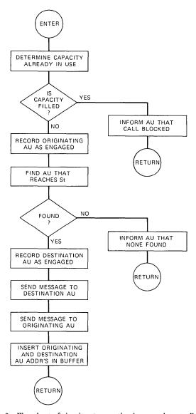
Fig. 9—Flowchart of circuit setup routine in central controller.
