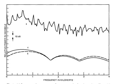
Fig. 4—(a) Input speech spectrum; and power transfer functions of postfilter with scaling coefficients for (b)  $\alpha = 0.2$ ,  $\beta = 1.0$ , and for (c)  $\alpha = 1.0$ ,  $\beta = 1.0$ . The plot (c) is merely the transfer function of the inverse predictor in the DPCM-APB system. [The 0-dB line is the same for (b) and (c) but different for (a)].
