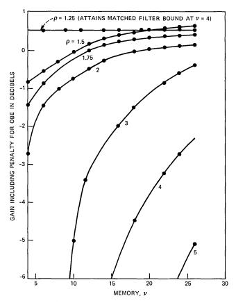
Fig. 9—Gain limit versus memory under spectral confinement constraint for  $P_e = 10^{-3}$ .
