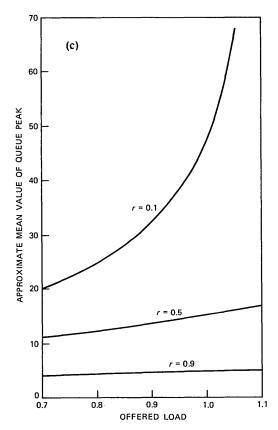
Fig. 6(c)—Approximate mean value of queue peaks versus offered load from eq. (23) for integrated systems with 500 slots.
