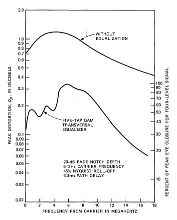
Fig. 4—Theoretical reduction in peak distortion,  $D_p$ , with a five-tap QAM transversal equalizer arrangement. Peak eye closure is noted for four-level transmission, that is, one rail of a 16-QAM system.
