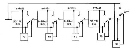
Fig. 13—Fault detection and isolation in super sections.
