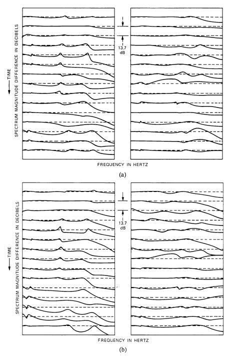
Fig. 7—Log spectral difference between the original and reconstructed signals: (a) with a fixed, unquantized predictor; (b) with an adaptive, quantized predictor.
