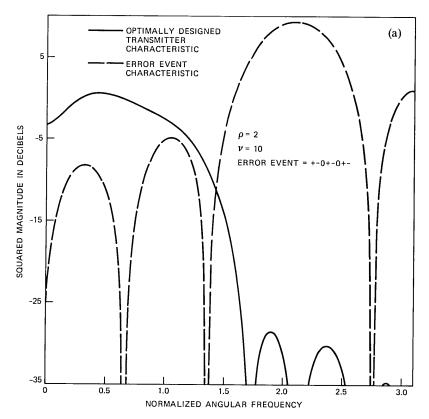
Fig. 10a—Example of an optimally designed transmitter characteristic and an error event characteristic. Vertical dotted line delineates the band edge.
