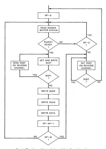
Fig. 6—Flowchart of forward channel data dispatch routine.
