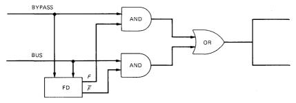
Fig. 12—Realization of two-way switch for fault isolation. FD outputs F and  $\overline{F}$  are complementary, signifying FAULT and NO FAULT.
