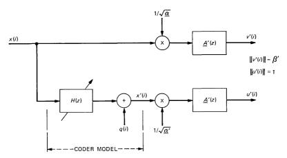
Fig. 3-Measuring coder performance with the likelihood ratio in a forward manner.
