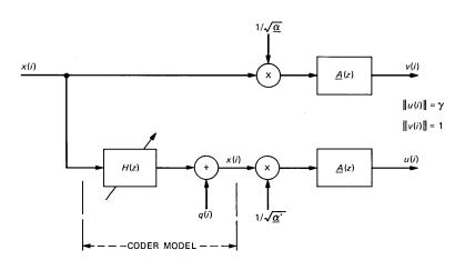
Fig. 4—Measuring coder performance with the likelihood ratio in a backward manner.
