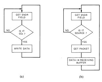
Fig. 10—Flowchart of (a) real-time signal dispatch, and (b) real-time signal reception.
