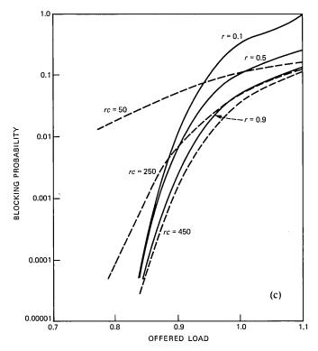
Fig. 4(c)—Voice message blocking probability versus offered load for integrated systems with 500 slots and single traffic systems with 50, 250, and 450 slots.
