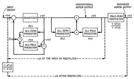
Fig. 3—Complete block diagram of an ADPCM system with a pole-zero predictor [defined by all-zero and all-pole components A(z) and B(z)] and a pole-zero postfilter [defined by components A'(z) and B'(z) that are derived from A(z) and B(z)]. The extreme case of A'(z) = B'(z) = 0 results in conventional ADPCM without postfiltering. The case of A'(z) = A(z) and B'(z) = B(z) results in a postfilter transfer function that is identical to the input signal spectrum, as in Fig. 1b.
