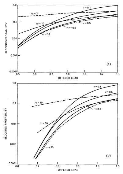
Fig. 4—Voice message blocking probability versus offered load for integrated systems with: (a) 20 slots and single traffic systems with 2, 10, and 18 slots; (b) 100 slots and single traffic systems with 10, 50, and 90 slots.
