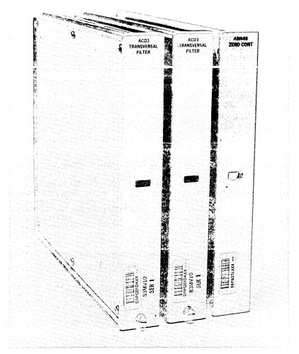
Fig. 3-Adaptive transversal equalizer consisting of two transversal filter circuit packs and one zero-forcing control circuit pack.
