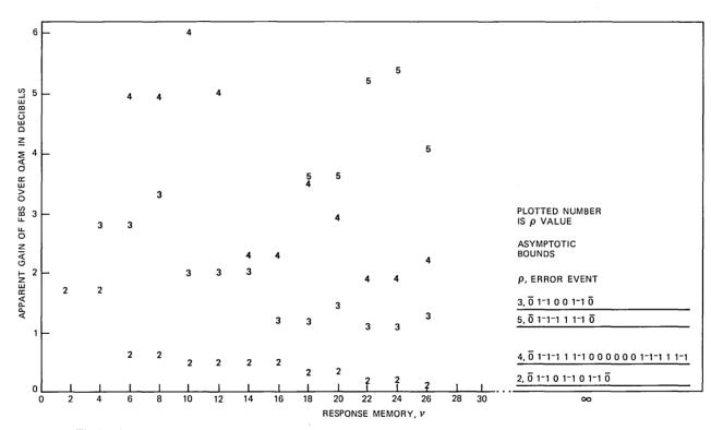
Fig. 5—Apparent gain of FBS over QAM (gains unachievable because of interference from adjacent bands).
