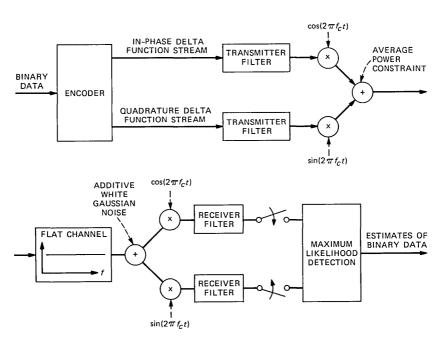
Fig. 2—Generic system structure. For QAM the transmit and receive filters are low-pass filters. For the FBS case they are a matched pair with finite memory in the sampled data domain. The nominal cutoff frequency of the low-pass filters is  $W=\mathscr{W}/2$ .
