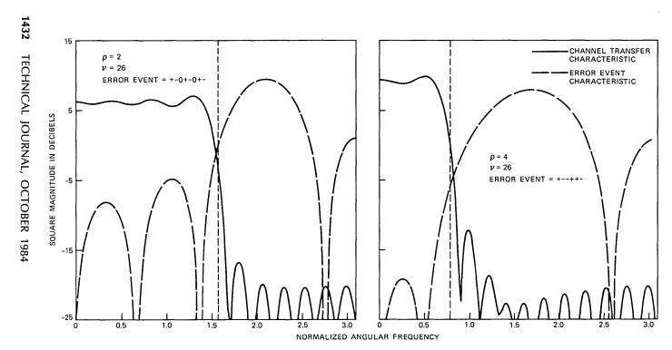
Fig. 7—Examples of  $|H_{\nu,\rho}^{NY}|^2$  and extremal error event (+ and – mean +1 and –1). Vertical dotted line marks transition from in-band to out-of-band.
