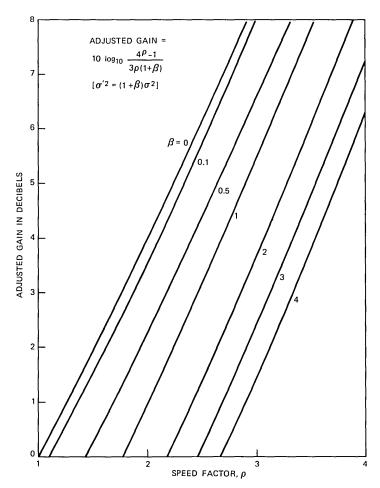
Fig. 3—Adjusted gain versus speed factor when matched filter bound is attained. Adjusted gain =  $10 \log_{10} \frac{4^{\rho} - 1}{3\rho(1 + \beta)}$ .
