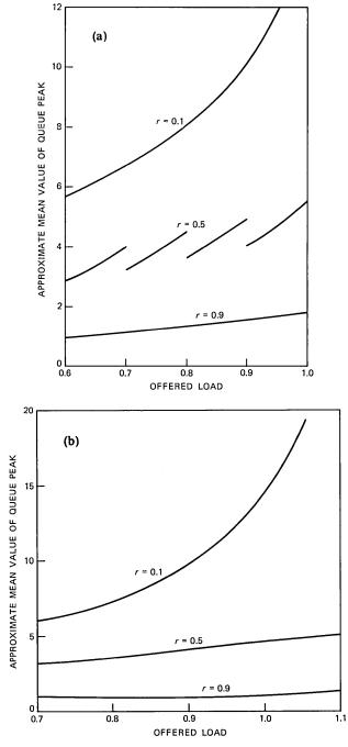
Fig. 6—Approximate mean value of queue peaks versus offered load from eq. (23) for integrated systems with: (a) 20 slots and (b) 100 slots.
