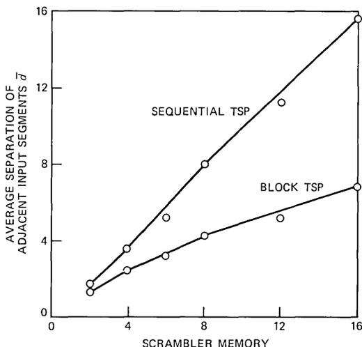
Fig. 4—Average temporal distance  $\bar{d}$  as a function of scrambler memory in (i) block TSP and (ii) sequential TSP with  $t = 2b$ . Minimum specified distances are the  $\min(d)$  values in Table II.
