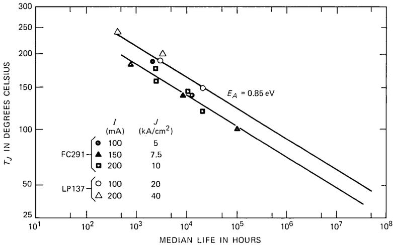
Fig. 16—Arrhenius plot of median life under various aging conditions. The activation energy is 0.85 eV.
