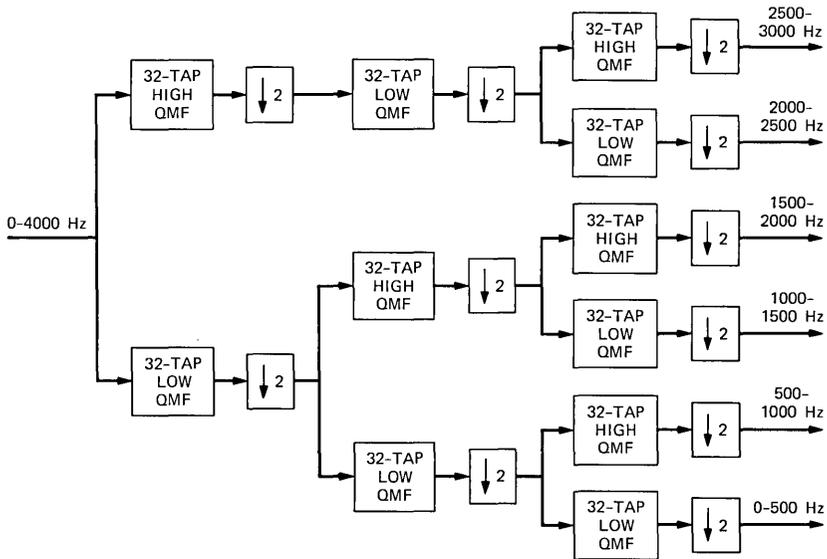
Fig. 6—Analysis filter bank for the half-duplex system.
