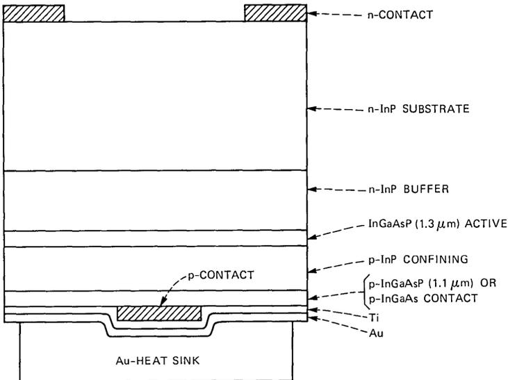
Fig. 9—Schematic structure of a Schottky-barrier isolated LED.
