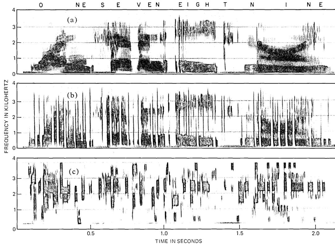
Fig. 7—Speech spectrograms: (i) unscrambled speech (female speaker, digit sequence “1789”), (ii) output of sequential TSP scrambler with communication delay of 128 ms, and (iii) output of sequential TFSP scrambler with the same communication delay of 128 ms.
