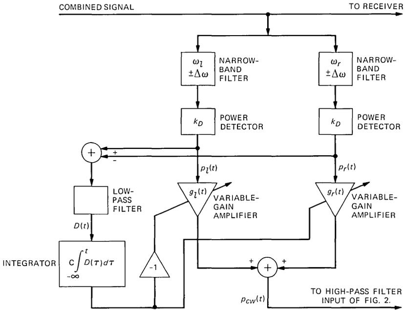
Fig. 3—Power detector portion of equalizing-combiner phase-control loop.
