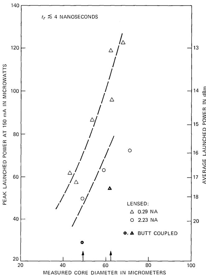
Fig. 12—Optical power launched into fiber as a function of NA and core radius. Two common fibers (0.23 NA, 50- $\mu\text{m}$  core; 0.29 NA, 62.5- $\mu\text{m}$  core) are indicated by arrows.
