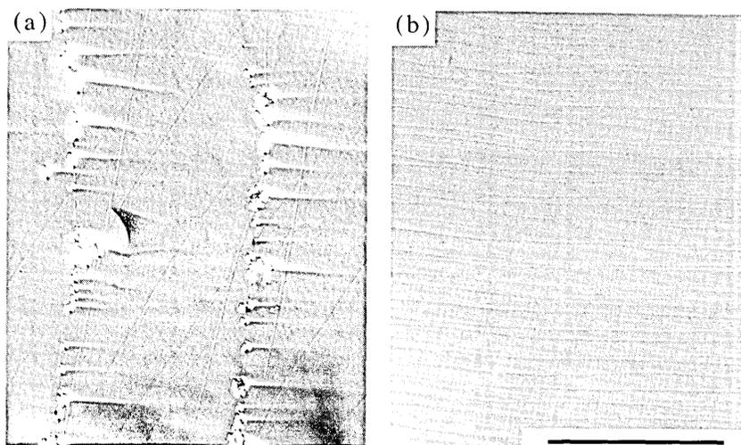
Fig. 5—A Nomarski micrograph (black bar = 100  $\mu\text{m}$ ) of the exposed InGaAsP active layer showing: (a) In inclusions owing to an incomplete wipe-off, and (b) inclusion-free surface of properly wiped-off layer.
