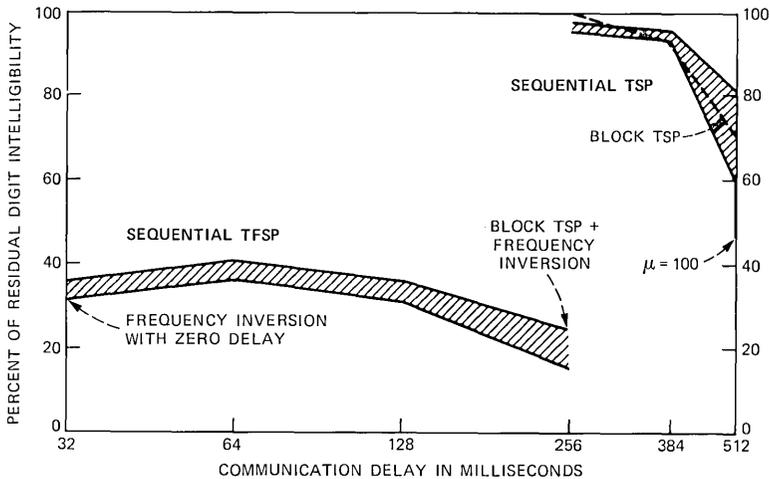
Fig. 5—Mean intelligibility of digits as a function of delay for sequential TSP sequential TFSP scramblers. Upper curves refer to averages over all four digit positions and over both male and female speakers. Lower curves refer to scores for the third digit position for the male speaker. The dashed lines refer to block TSP, digit position three, and male speaker.
