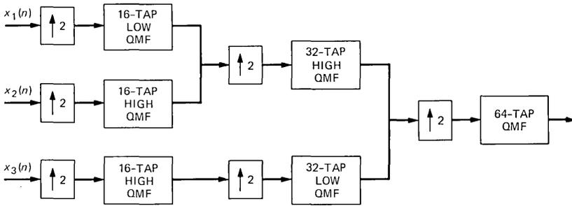
Fig. 4—Structure of filter bank #2 for the full-duplex system.
