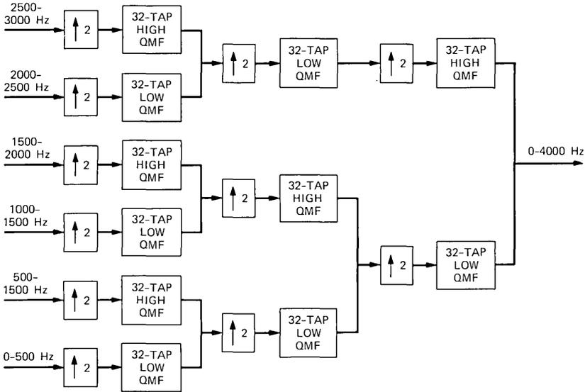
Fig. 7—Synthesis filter bank for the half-duplex system.
