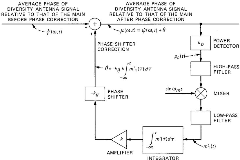
Fig. 2—Block diagram of maximum-power combiner phase-control loop.
