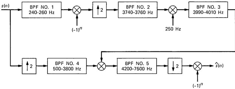
Fig. 11—Phase-roll compensation network.
