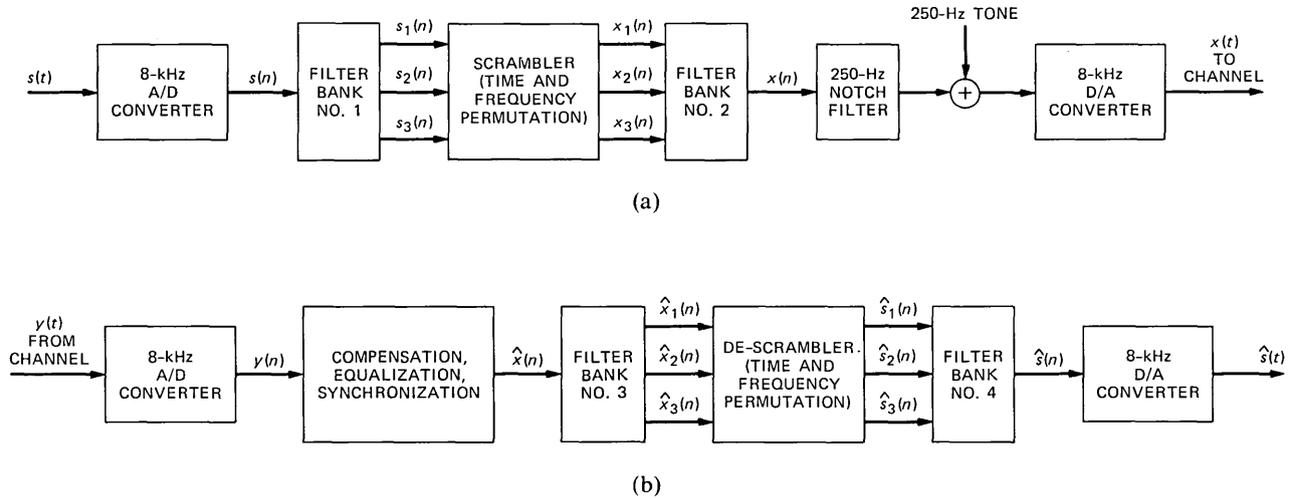
Fig. 1—Block diagram of the proposed full-duplex system. (a) Transmitter. (b) Receiver.
