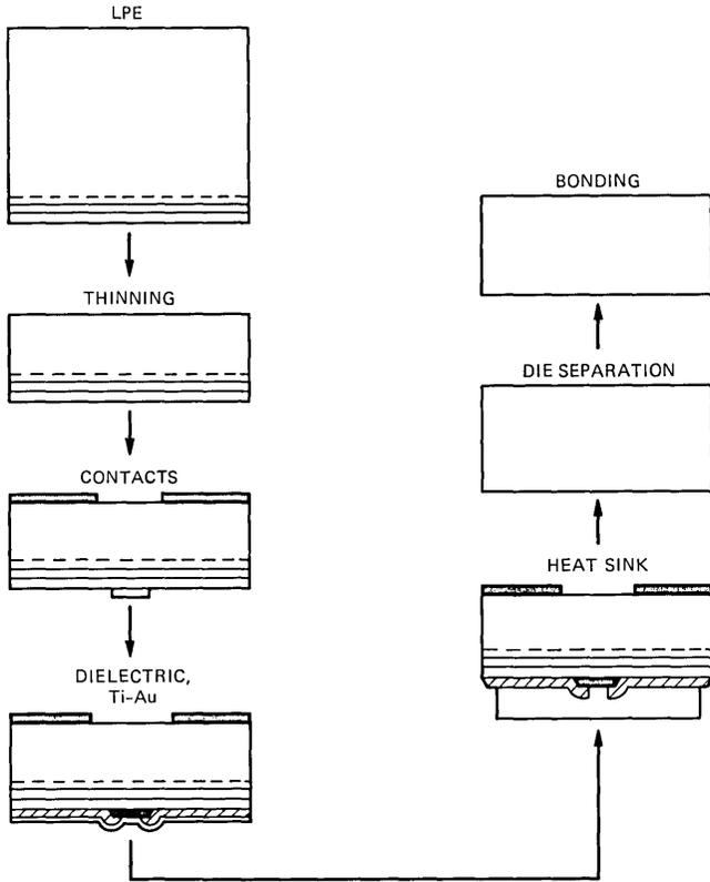
Fig. 7—Schematic processing diagram for a dielectric-isolated LED.
