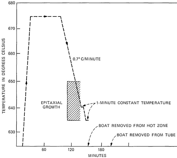
Fig. 1—Schematic diagram of melt homogenization and LPE growth cycle.
