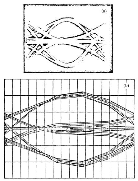
Fig. 10—Experimentally (a) and computationally (b) generated eye diagrams by transmitting bidirectional data over 18 kft of No. 22 Awg cable. The echo cancellation is 35 dB.
