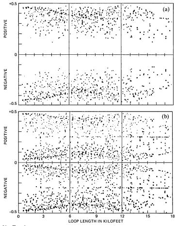
Fig. 29—Eye data scatter plots for 144-kb/s тСм-mode transmission (actual line rate is 324 kb/s). Bridged taps are left intact. Subscriber side data are given. (a) Eye opening. (b) Eye thickness.
