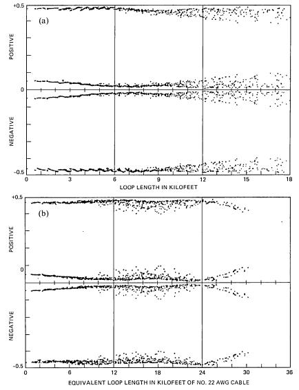
Fig. 21—Eye thickness scatter plots for 80-kb/s data transmission in the TCM mode. In the set of six figures (a through f) the data at the s end of the loops are given. (a) Eye thickness (Y-axis) versus loop length in kft (X-axis). (b) Eye thickness versus equivalent loop length (expressed in kft of No. 22 AWG cable).
