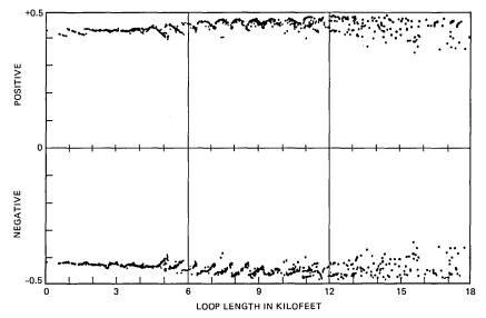
Fig. 46—Eye opening scatter plot for the 1973 survey loops at 162 kb/s TCM mode. (Effective rate is 72 kb/s.)
