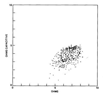
Fig. 5—Scatter plot of loop resistance plotted against its impedance (subscriber side). Temperature =  $60^{\circ}$ F, Frequency = 32 kHz, X- and Y-scale = 20 ohms/division.
