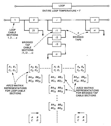
Fig. 50-Loop with bridged taps.
