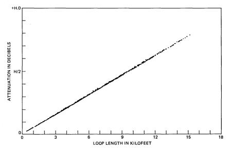
Fig. 3—Scatter plot of loop attenuations plotted against the equivalent loop length of No. 22 AWG cable. The frequency is 32 kHz and the temperature is  $60^{\circ}$ F. The X-scale is 2 kft/division and Y-scale is 5.0 dB/division.
