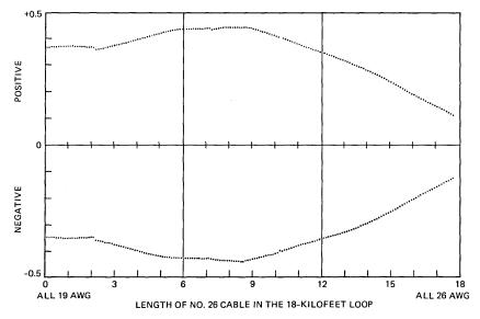
Fig. 31—Eye openings with Nos. 19 and 26  $_{\rm AWG}$  composite cable loops having a total length of 18 kft (144 kb/s).
