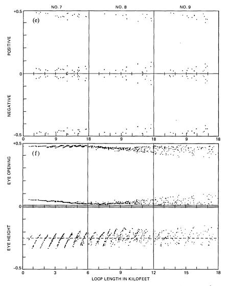
Fig. 21—(e) Eye thickness for loops with 7-, 8-, or  $\geq$ 9-cable sections versus loop length in kft (numbers indicate number of sections). (f) Eye thickness and eye height for all loops versus loop length in kft.
