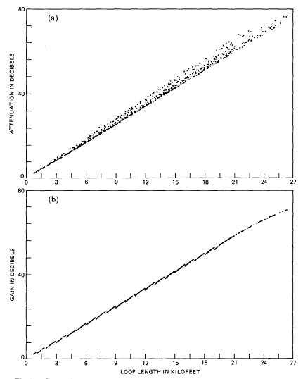
Fig. 35—Comparison of loop attenuations and equalizer gains for various loops at 324 kHz. The Y-axis scale is 8 dB/division. (a) Loop attenuation. (b) Equalizer gain.
