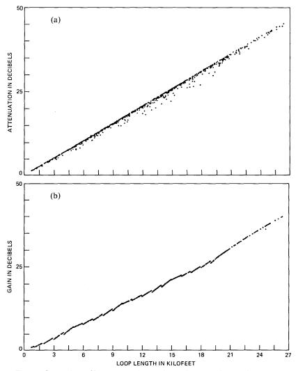
Fig. 33—Comparison of loop attenuations and equalizer gains for 1973 loop survey at 56 kHz plotted against the loop length expressed in equivalent kft of No. 22 AWG cable. Scale on the Y-axis is 5 dB/division, and on the X-axis it is 1.5 kft/division. (a) Loop attenuation. (b) Equalizer gain.
