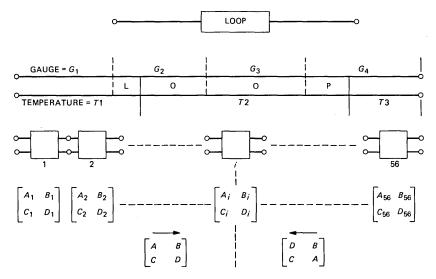
Fig. 49-Loop without bridged taps.
