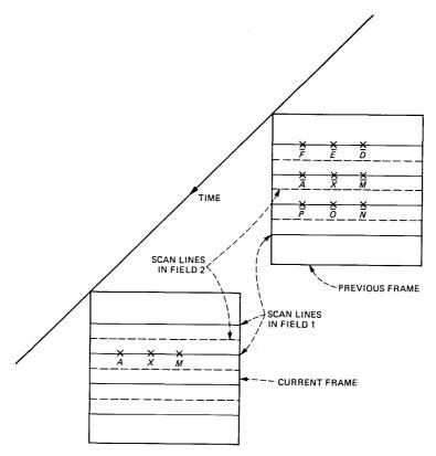
Fig. 2-Pel configuration for interframe processing.
