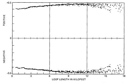
Fig. 45—Eye opening scatter plot for the 1973 survey loops at 126 kb/s TCM mode. (Effective rate is 56 kb/s.)
