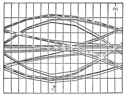
Fig. 17—Experimentally (a) and computationally (b) generated eye diagrams over a four-section (3.46 kft, 19 AWG; 8.7 kft, 24 AWG; 9.8 kft, 22 AWG; 3.46 kft, 19 AWG) loop at 324 kb/s in the TCM mode. The loop attenuation at half-bit rate is approximately 48 dB.
