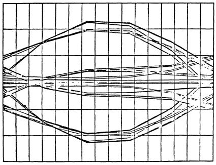
Fig. 12—Eye diagram obtained by transmission of data at 324 kb/s (for an effective bidirectional rate of 144 kb/s) in the  $\tau$ CM mode. The loop configuration is the same as that for the simulations in Fig. 11.
