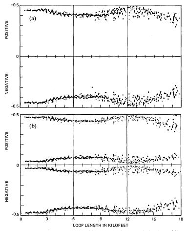
Fig. 28—Eye data scatter plots for 144-kb/s тСм-mode transmission (actual line rate is 324 kb/s). Bridged taps are stripped from the loops. Subscriber side data are given. (a) Eye opening. (b) Eye thickness.
