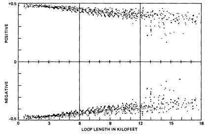
Fig. 36—Eye opening scatter plot at 324 kb/s with 20,000-ft, four-section equalizer in the  $\tau_{CM}$  mode of transmission. Subscriber side data are given.
