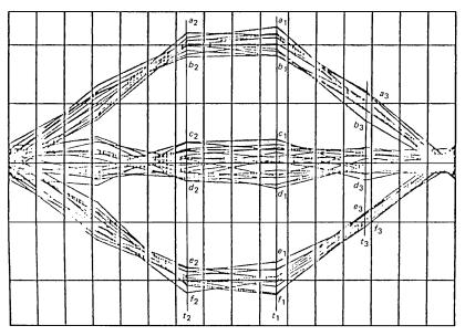
Fig. 20-Extraction of eye statistics from the eye diagram.
