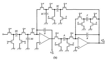
Fig. 4b—Switched-capacitor all-pole biquad—parasitic-compensated equivalent to Fig. 4a.
