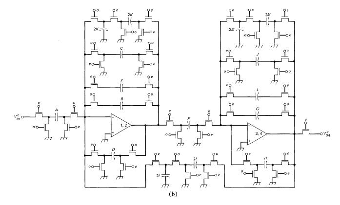
Fig. 12b—Fourth-order low-pass sc leapfrog filter—two-amplifier realization.
