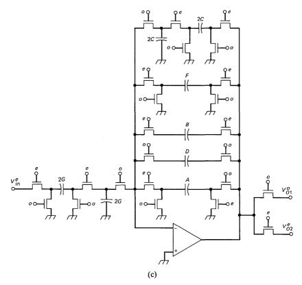
Fig. 4c-Switched-capacitor all-pole biquad-single-amplifier equivalent to Fig. 4b.
