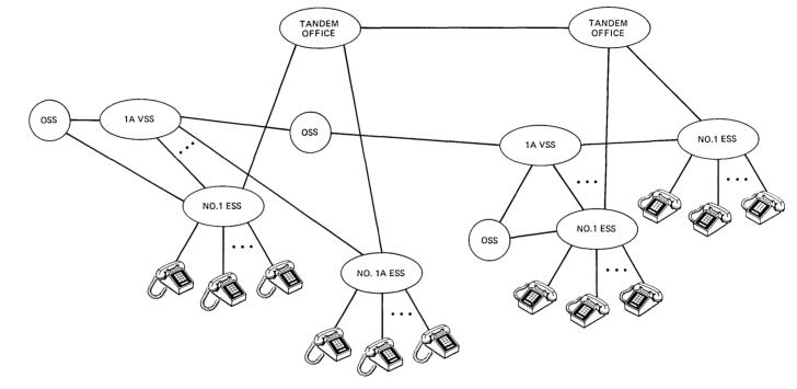
Fig. 1—1A vss: a new node in the SPC network.
