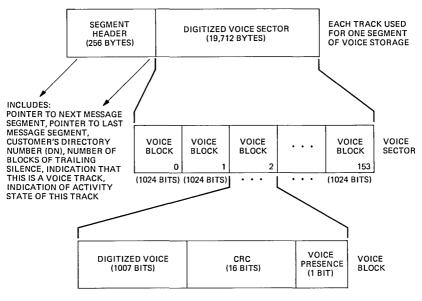
VOICE IS PARTITIONED INTO SEGMENTS, EACH CONTAINING 155,078 BITS (4.85 SECONDS) OF THE TOTAL MESSAGE. EACH SEGMENT IS STORED SEPARATELY ON THE DISK MEDIUM ALONG WITH A DATA HEADER CONSISTING OF A DESCRIPTION OF THE MESSAGE'S SEGMENT POSITION, THE MESSAGE OWNER, THE TYPE OF MESSAGE, AND THE STATUS OF THE MESSAGE.
