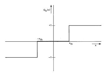
Fig. 3-Three-level quantizer for gradient quantization.
