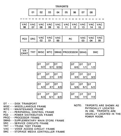
Fig. 9-Voice storage system floor plan.
