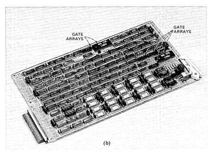
Fig. 6b-ML PWB buffer.
