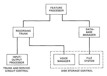
Fig. 7—Basic structure of call processing software.
