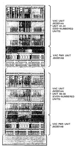
Fig. 8-Voice access circuit frame.
