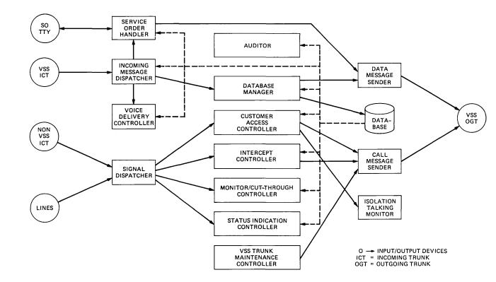
Fig. 3—Host Ess conceptual design.
