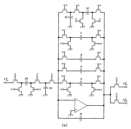
Fig. 6a—Single-amplifier biquad stabilization via continuous feedback—circuit schematic.
