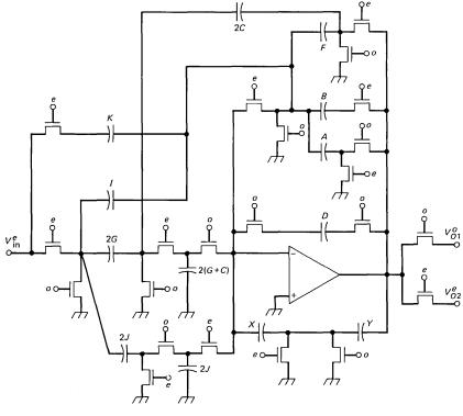
Fig. 11a—Switch sharing in single-amplifier biquads—switched shared equivalent to the circuit in Fig. 8a.
