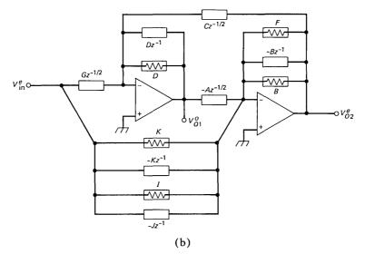
Fig. 8b—Single-amplifier biquad which realizes the transfer functions in eq. (10)—equivalent circuit.
