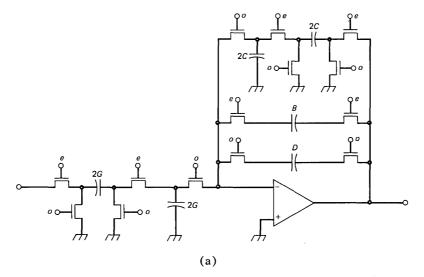
Fig. 10a-Switch sharing among parasitic-compensated toggles-original circuit.
