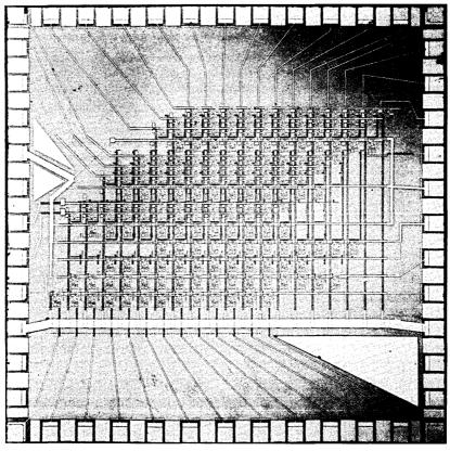
Fig. 1-A photomicrograph of the multiplier chip.
