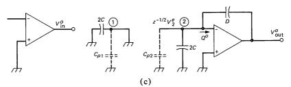
Fig. 1—Parasitic-compensated inverting integrator. (a) Complete circuit with parasitic capacitances. (b) *e*-phase connectivity. (c) *o*-phase connectivity.
