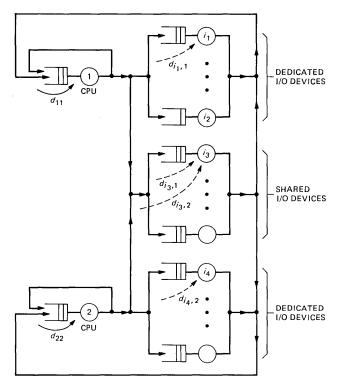
Fig. 9-Two systems sharing mass storage devices.
