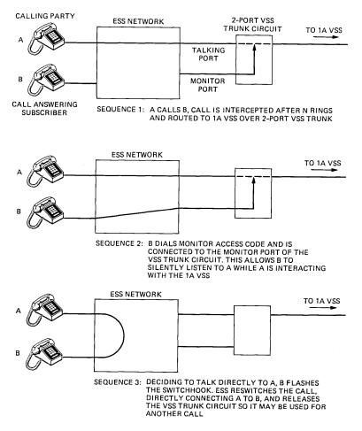
Fig. 4-Monitor/Cut-Through capability.
