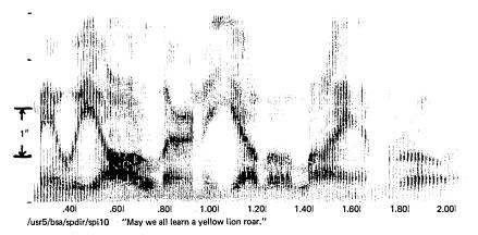
Fig. 4—Digital spectrogram in traditional format.
