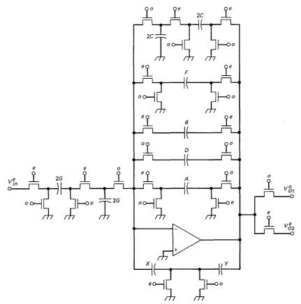
Fig. 7-Single-amplifier biquad stabilization via XY sc feedback.
