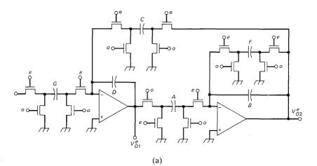
Fig. 4a-Switched-capacitor all-pole biquad-parasitic-insensitive realization.
