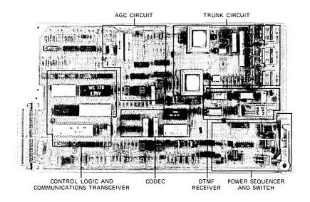
Fig. 5-Trunk access circuit.
