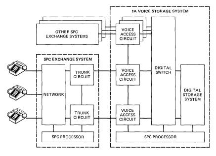
Fig. 1—The 1A vss in the spc network.
