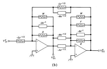
Fig. 6b—Single-amplifier biquad stabilization via continuous feedback—equivalent circuit.
