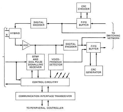
Fig. 2-No. 1A vss voice access circuit.
