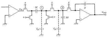
Fig. 3-Parasitic-compensated noninverting integrator.
