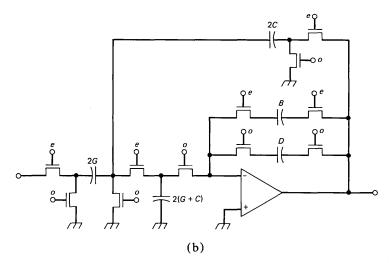
Fig. 10b—Switch sharing among parasitic-compensated toggles—switch-reduced equivalent of Fig. 10a.
