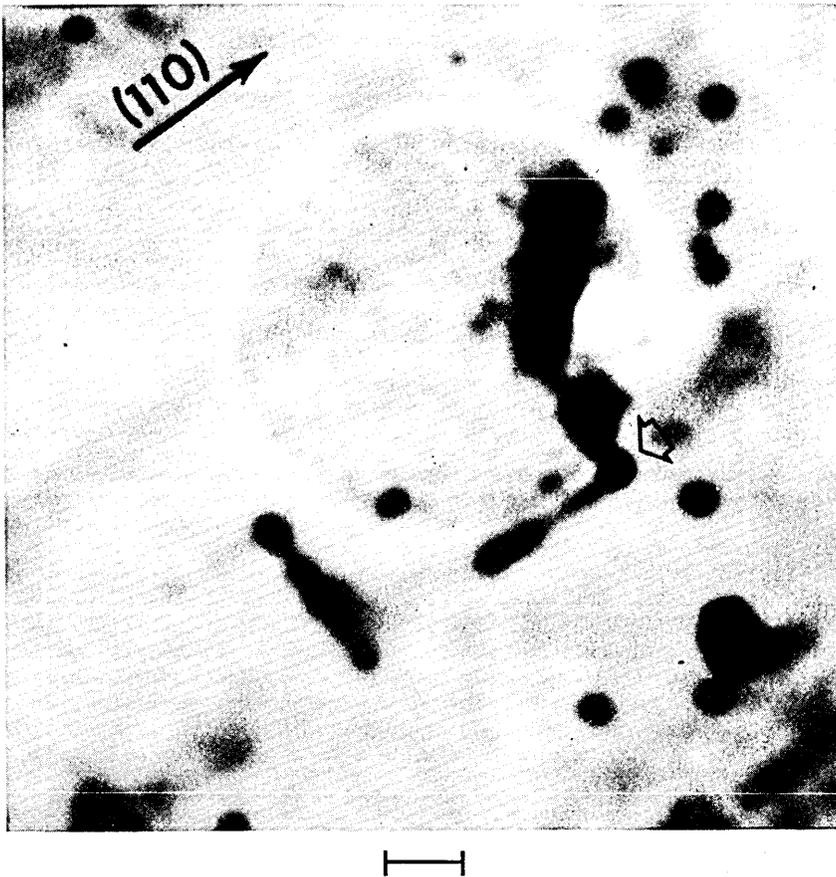
Fig. 21—Dark line defects oriented along  $\langle 100 \rangle$  and  $\langle 110 \rangle$  directions in a planar DH LED induced by current injection during burn-in. The circular region defines the 50- $\mu\text{m}$ -diameter back surface contact.
