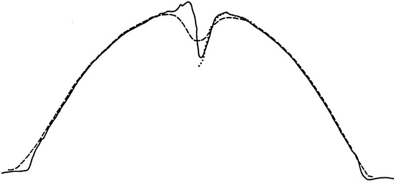
Fig. 18—Profiles of fiber no. 5 as measured by RNF (solid), FOCUS (dotted), and TRANS (broken) techniques.
