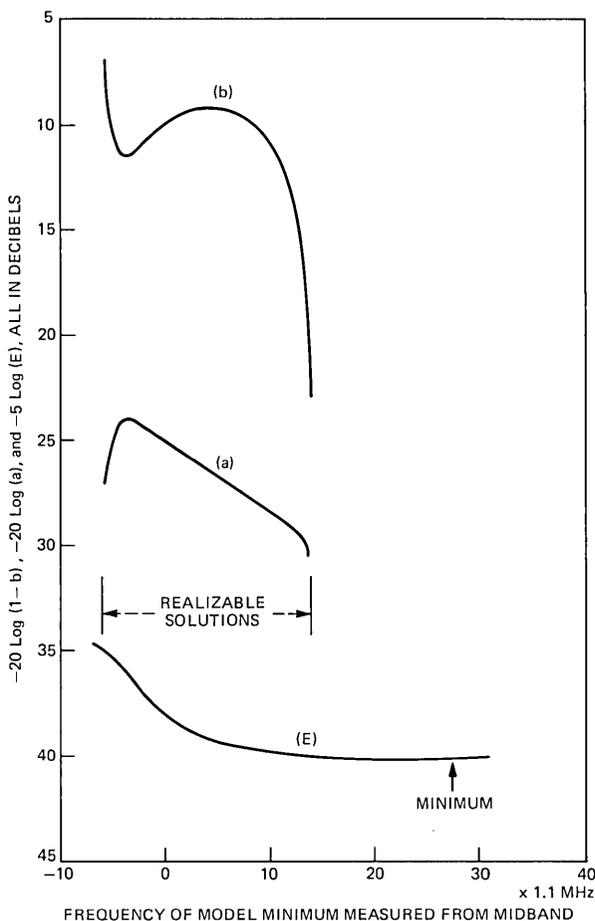
Fig. 6—Locus of weighted fit error and model parameters with  $f_o$  as a free variable for typical scan in Fig. 4.
