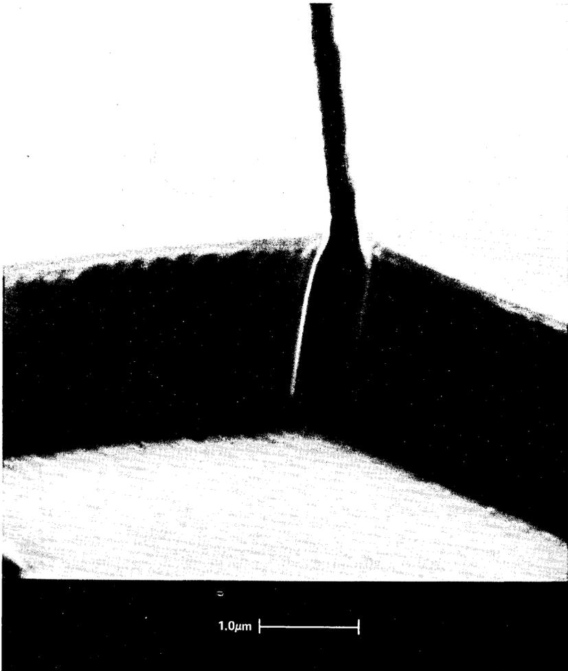
Fig. 7—A  $0.45\text{-}\mu\text{m}$  trench RF etched into a  $2.0\text{-}\mu\text{m}$  thick layer of organic material (resist). Initial patterning was done with projection photolithography.
