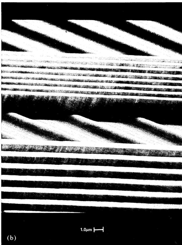
Fig. 5b—Profile of Fig. 5a showing step coverage and flat top surface. Thick resist varies from 2.8- $\mu\text{m}$  high in valley to 2.1  $\mu\text{m}$  on top of a step. Resist width is 1  $\mu\text{m}$ .
