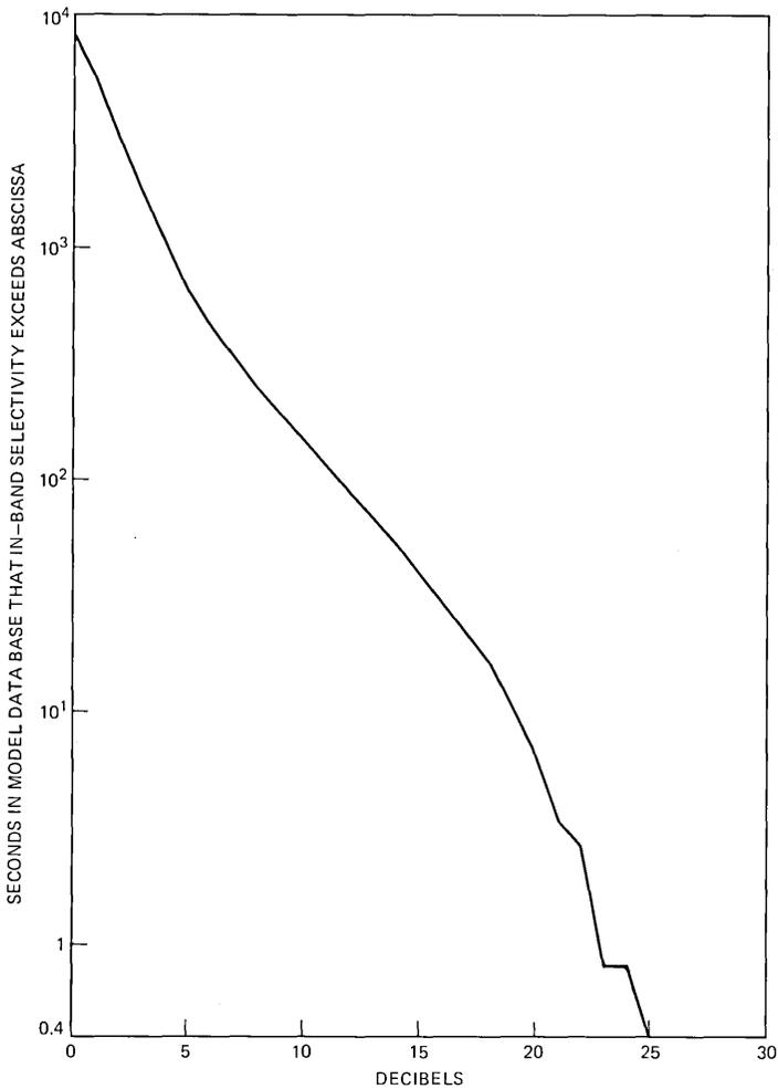
Fig. 20—Distribution of in-band selectivity (25.3-MHz bandwidth) for model data base.
