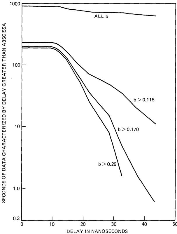
Fig. 13—Distribution of optimum delay for simple three-path model, as qualified by realizability, the sharpness of minimum, and by several values of the model parameter  $b$ .
