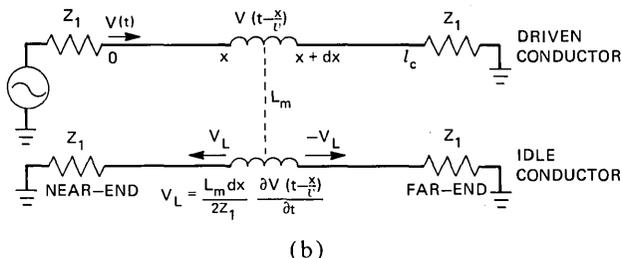
Fig. 3—A simplified model of crosstalk for a pair of lossless, uniformly, and loosely coupled conductors terminated with matched loads.  $Z_1$ ,  $v$ , and  $l_c$  denote characteristic impedance, propagation velocity, and coupled length, respectively. (a) Capacitive crosstalk,  $V_c$ , resulting from the mutual capacitance per unit length,  $C_m$ . (b) Inductive crosstalk,  $V_L$ , resulting from the mutual inductance per unit length,  $L_m$ .
