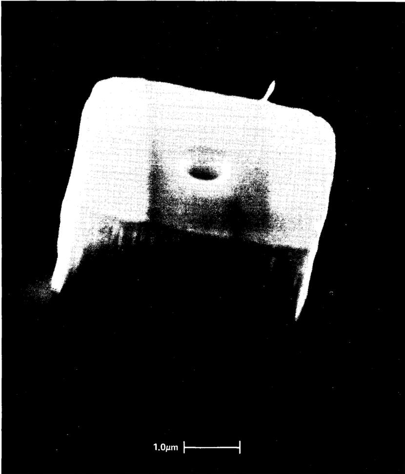
Fig. 6—A 0.5- $\mu\text{m}$  trench in 2.3- $\mu\text{m}$  thick resist.
