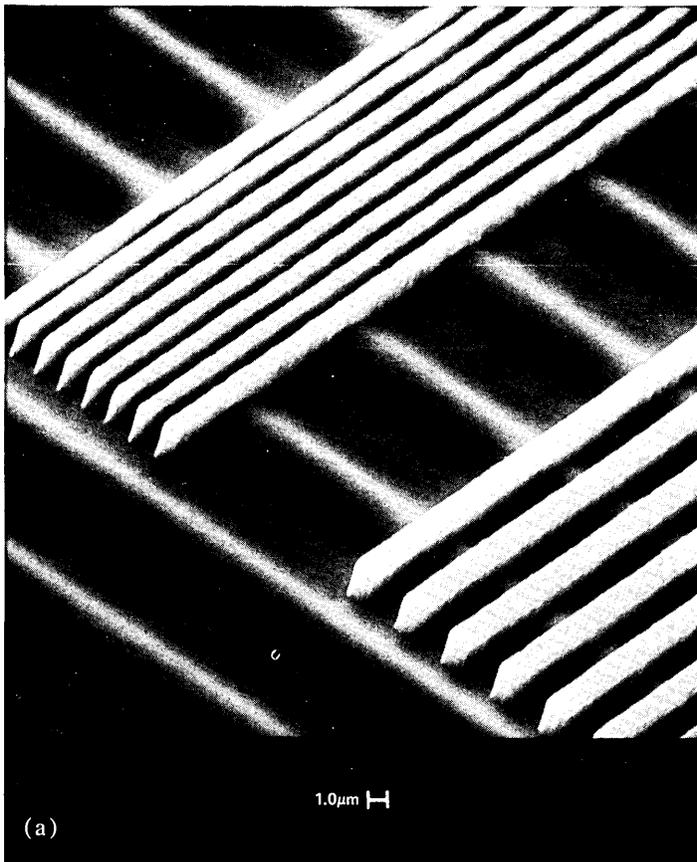
Fig. 5a—1- $\mu\text{m}$  lines and spaces on top of phosphosilicate glass steps. Note uniformity in line width.
