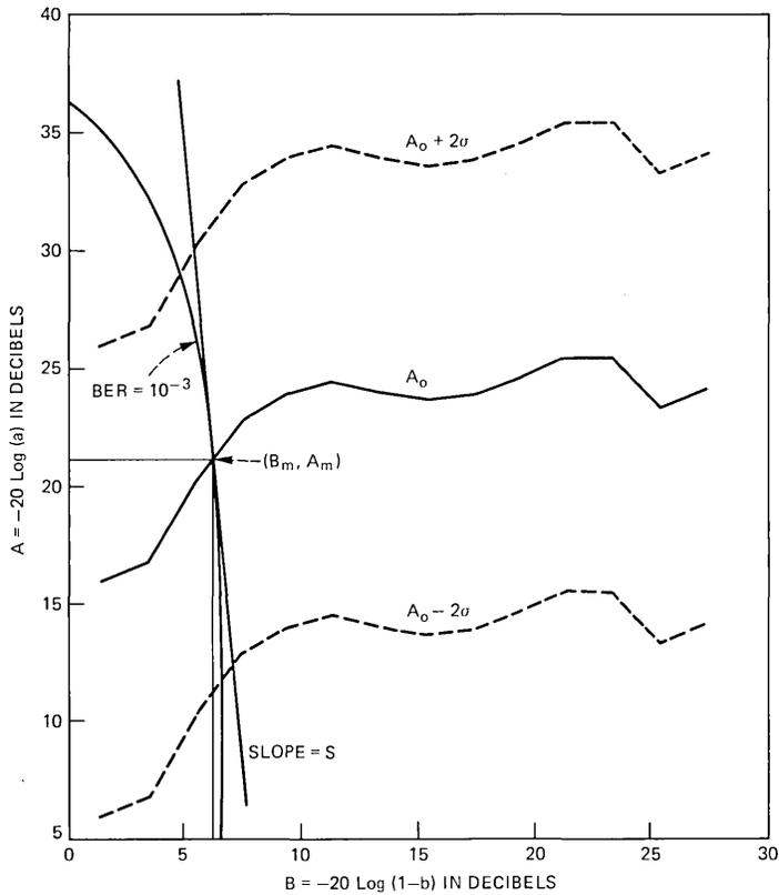
Fig. 14—Approximate outage calculation for 10 dB less transmitted signal.
