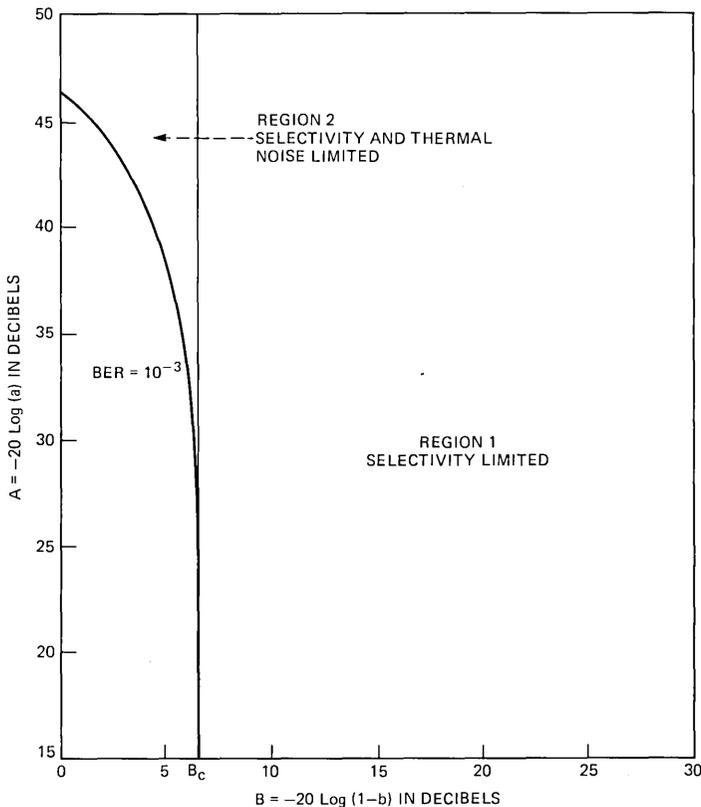
Fig. 11—Classification of outage with respect to critical curve for  $\text{BER} = 10^{-3}$ ,  $f_0 = 19.8$  MHz.
