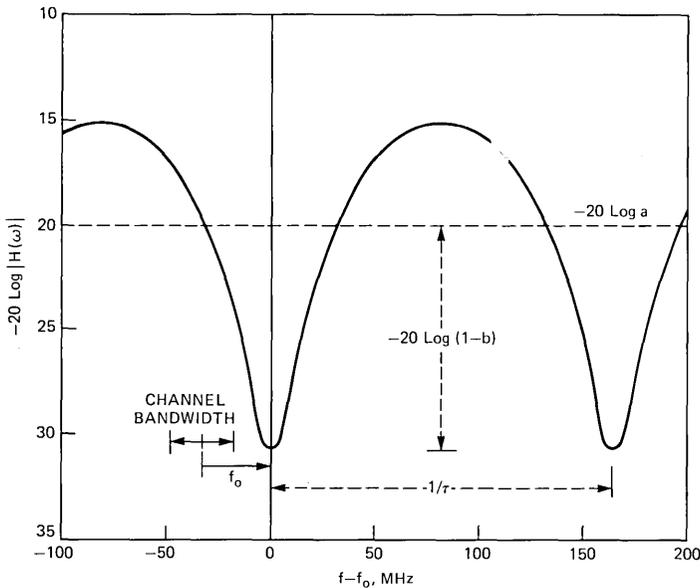
Fig. 1—Attenuation of channel model function,  $H(\omega) = a[1 - b \exp(-j(\omega - \omega_0)\tau)]$ , for  $\tau = 6.3 \text{ ns}$ ,  $a = 0.1$ ,  $b = 0.7$ .
