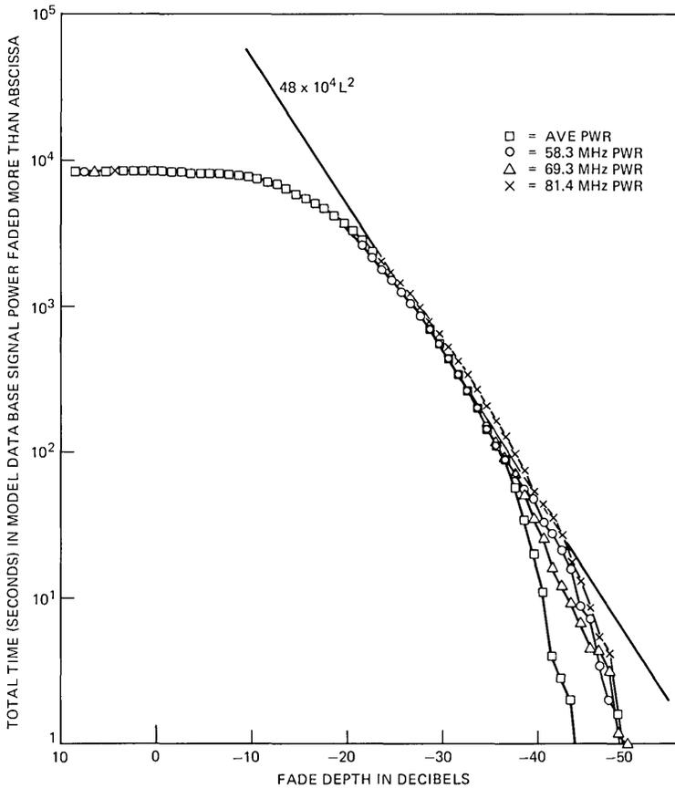
Fig. 5—Amplitude distributions for model data base period.
