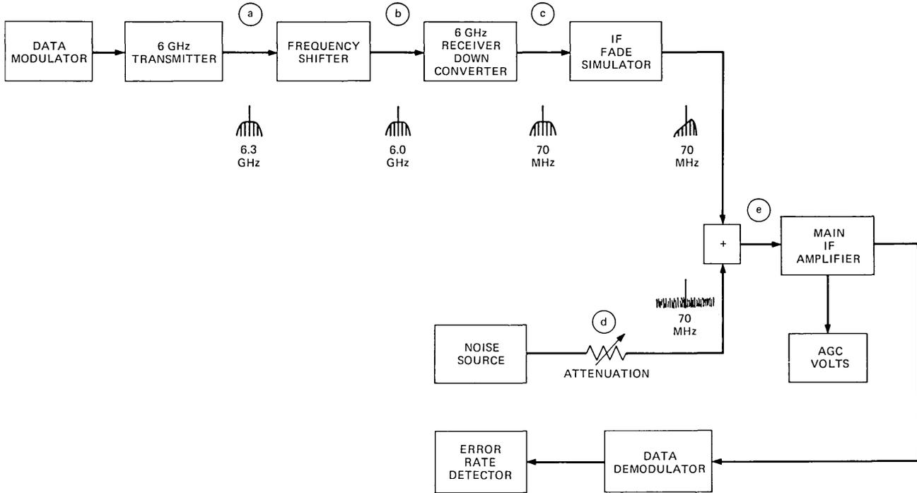
Fig. 7—Laboratory test arrangement.
