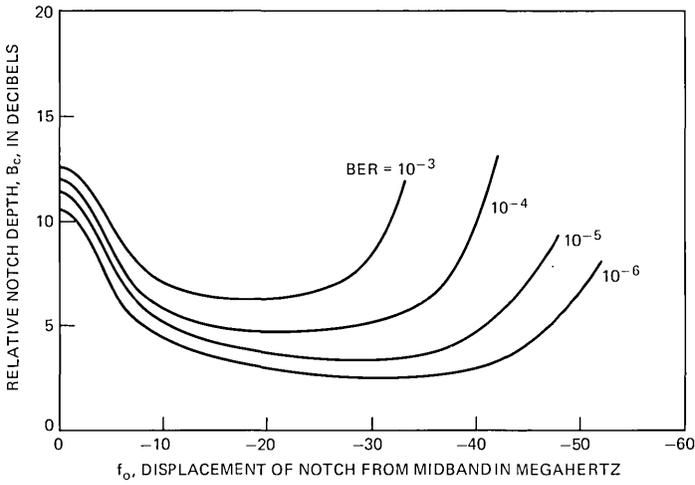
Fig. 13—Asymptotic performance curves. Locus of values of  $f_o$  and  $B$  that produce a fixed BER at high carrier-to-noise ratio.
