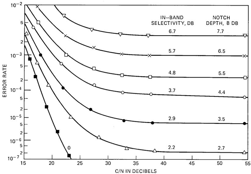
Fig. 9—High-speed digital radio IF dispersive fade simulations,  $\tau = 6.3 \text{ ns}$ ,  $f_0 = -19.8 \text{ MHz}$ .
