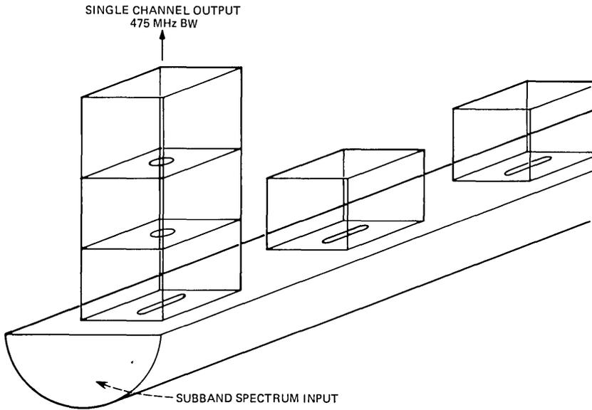
Fig. 4—Channel-dropping filter.
