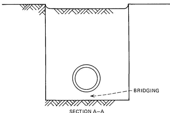
Fig. 4—Sheath-soil interaction model.
