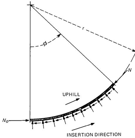
Fig. 12—Plan view of forces on a segment of waveguide in a curve.
