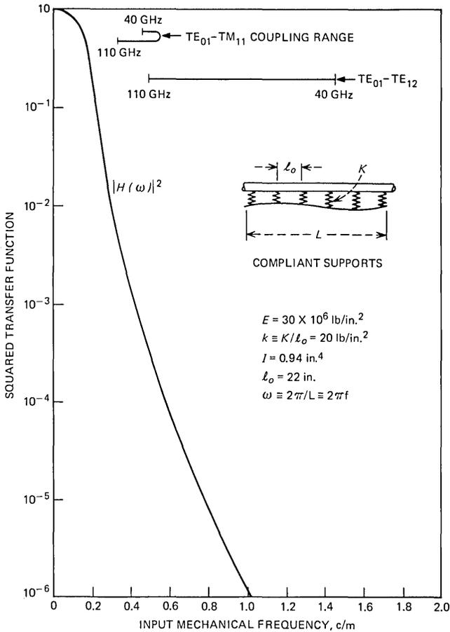
Fig. 7—Response of waveguide-support system.
