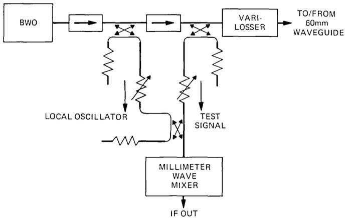
Fig. 3—RF millimeter-wave circuit arrangement.
