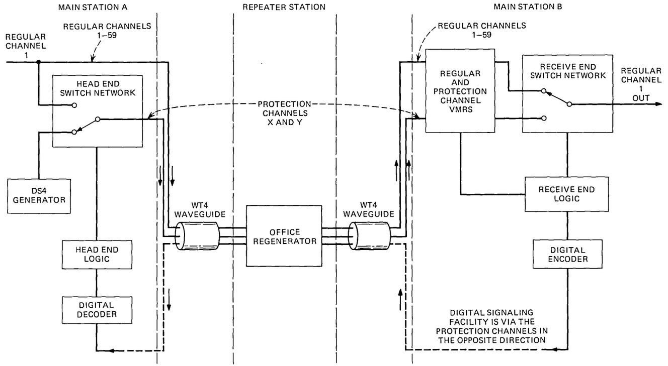
Fig. 4—Switching section—simplified block diagram.
