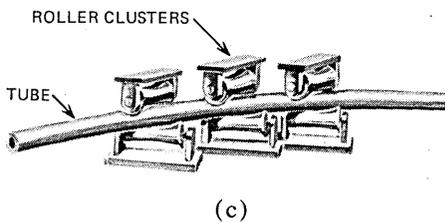
Fig. 6—Manufacturing process for steel tube. (a) Tube forming and welding. (b) Cold drawing. (c) Roller straightening.
