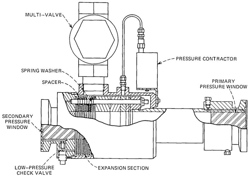
Fig. 6—Multifunction waveguide.
