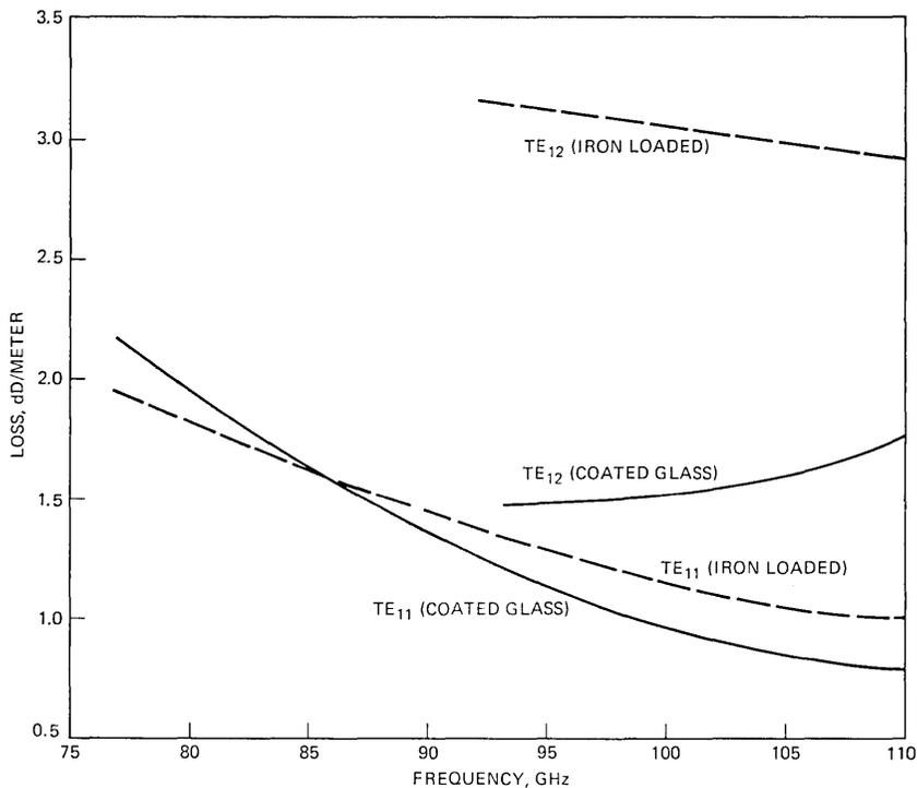
Fig. 14—Measured loss of TE<sub>11</sub> and TE<sub>12</sub> modes in helix waveguide.
