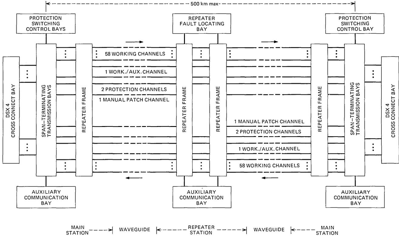
Fig. 1—Layout of protection span.
