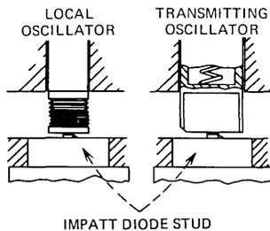
Fig. 18—Bias rods for WT4 oscillators.
