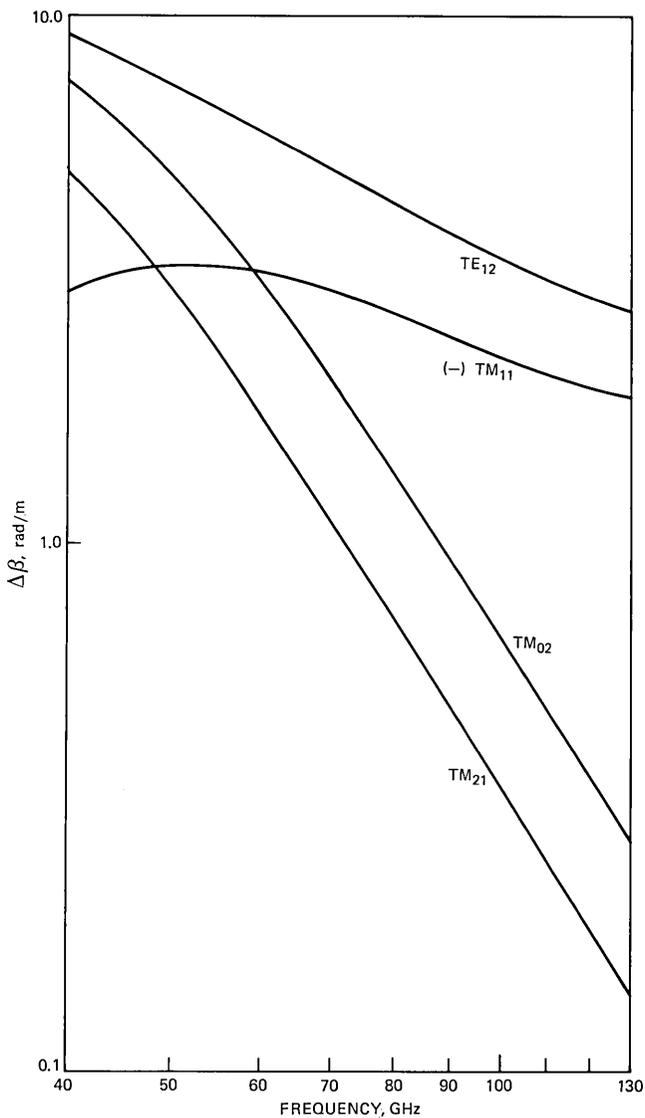
Fig. 3—Differential propagation constants in 60-mm lined waveguide.
