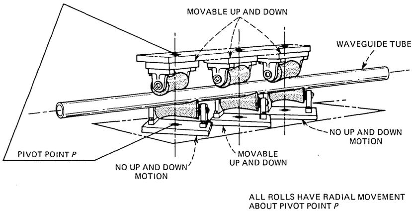
Fig. 4—Roller straightener.
