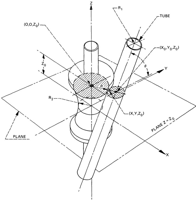
Fig. 5—Roller-tube interaction.
