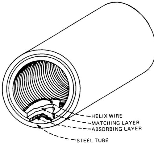
Fig. 5—Helix waveguide.
