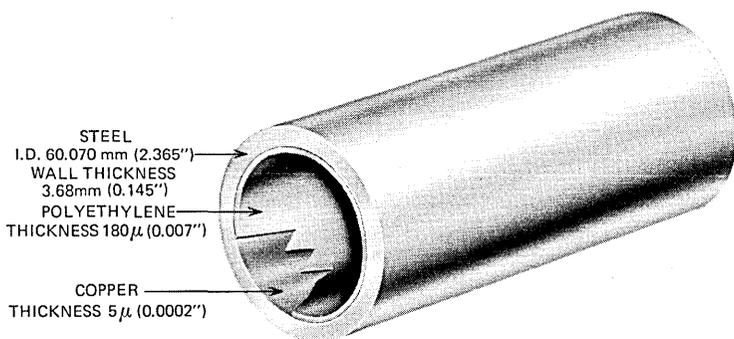
Fig. 2—Dielectric-lined waveguide configurations.
