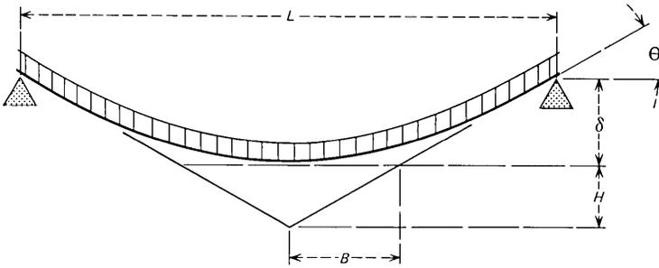
Fig. 9—WT4 sheath on simple supports.
