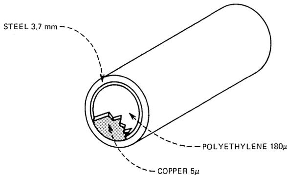
Fig. 4—Dielectric-lined waveguide.
