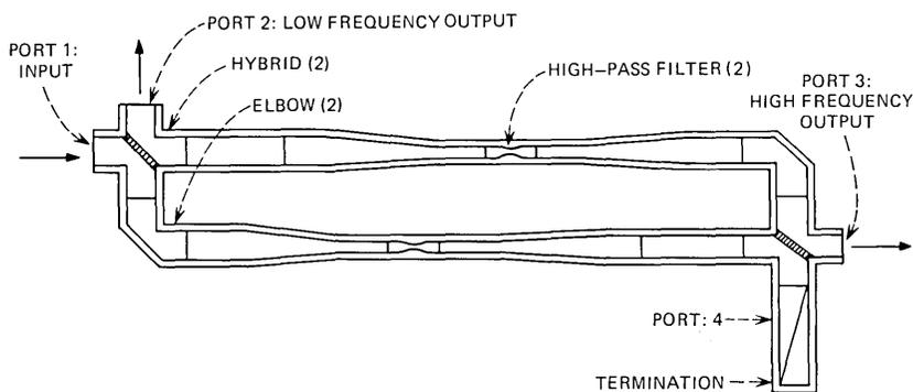
Fig. 3—Band-splitting filter.
