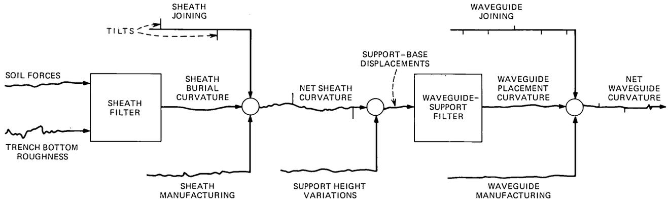
Fig. 2—Waveguide curvature inputs and filtering.
