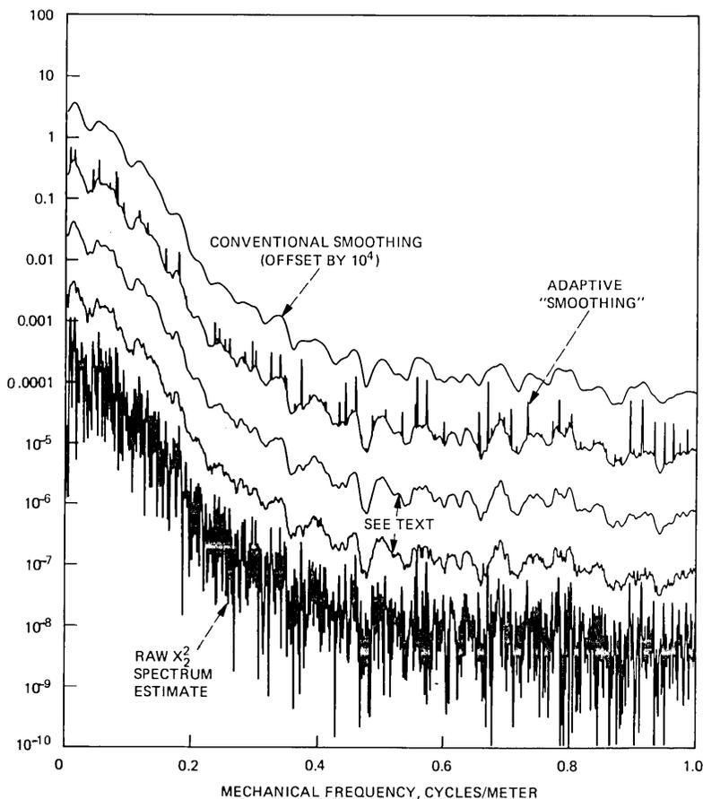
Fig. 11—Steps of a simple adaptive “smoothing” procedure applied to mode filter section 14 vertical curvature spectrum.
