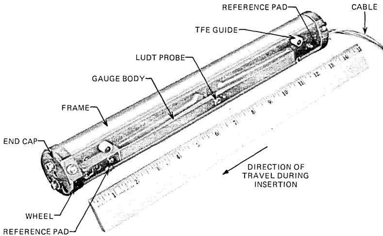
Fig. 7—Curvature gauge.
