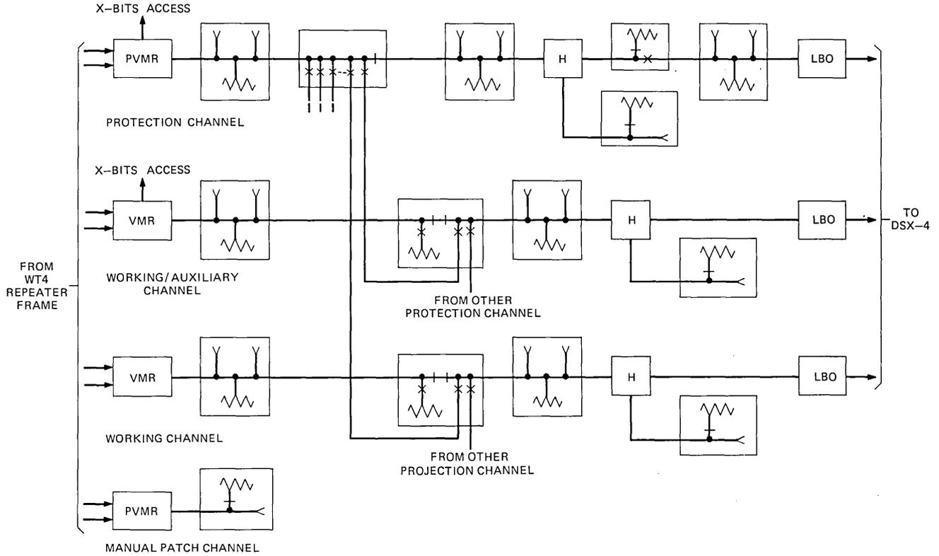
Fig. 3—Receive section.
