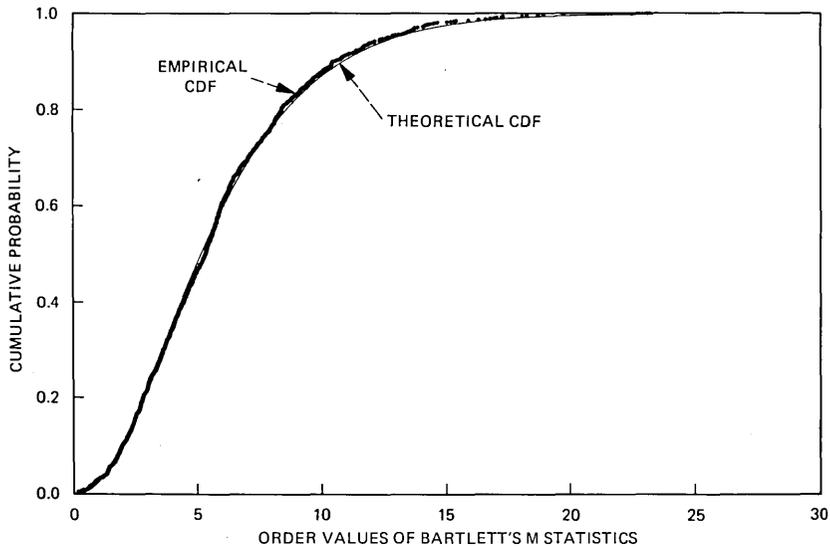
Fig. 10—Comparison of the empirical cumulative distribution function for the *unsmoothed* values of Bartlett's  $M$  statistic shown in Fig. 9 with the theoretical distribution. The points used in this test were spaced  $4/T$  in frequency. For this comparison the kolmogorov  $D^-$  statistic has a value of 0.0264 which is at the 35 percent point.
