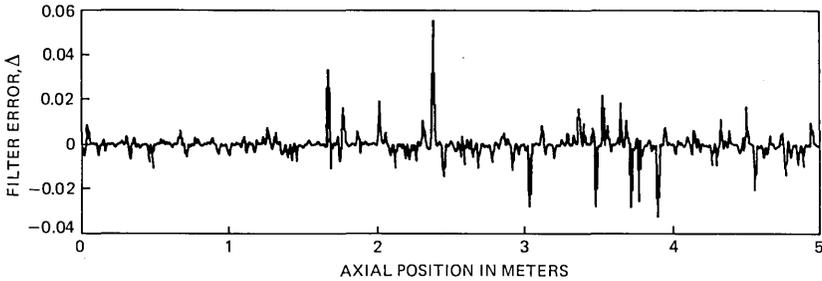
Fig. 15—Filtering error,  $\Delta$ , between the original uncontaminated data and robust-filtered version using the bisquare influence function with  $u_{bs} = 6$ . Note the extensive errors occurring in the uncontaminated part of the series.
