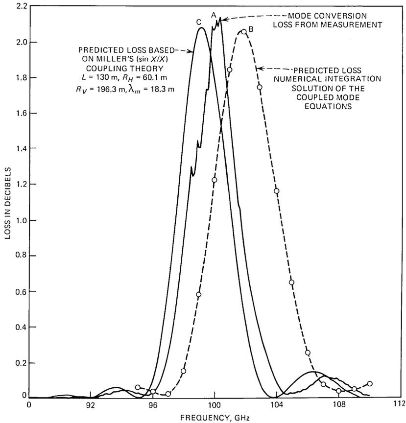
Fig. 7—TE<sub>01</sub> loss due to mode conversion in modulated bend at Chester.
