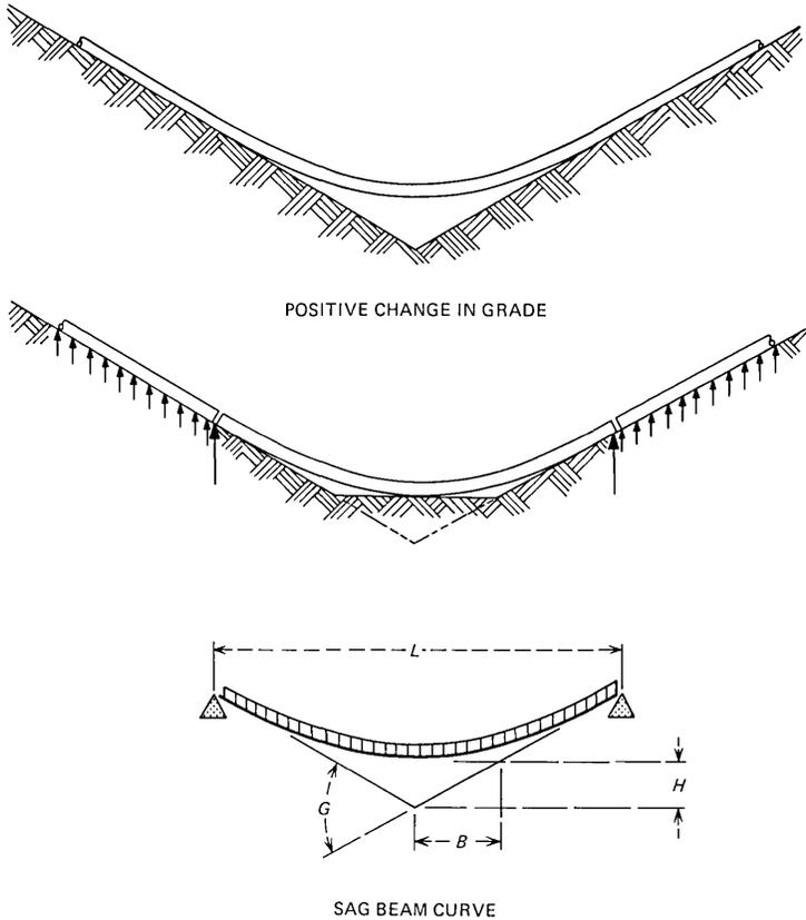
Fig. 4—WT4 sheath at positive change in grade.
