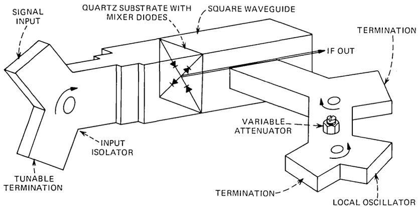
Fig. 2—Down-converter assembly.
