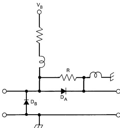
Fig. 10—Schematic of variable attenuator.
