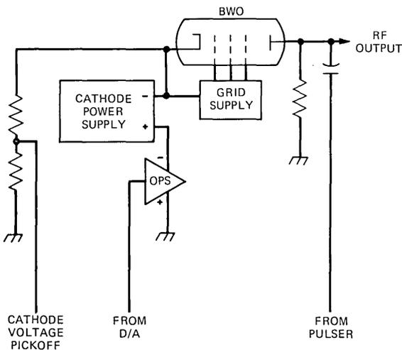
Fig. 4—BWO frequency-control circuit arrangement.
