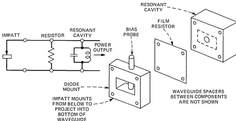
Fig. 3—Transmitting IMPATT oscillator.
