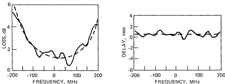
Fig. 2—Equalized loss and delay characteristics.
