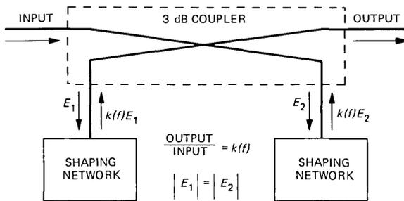
Fig. 3—Basic equalizer configuration.
