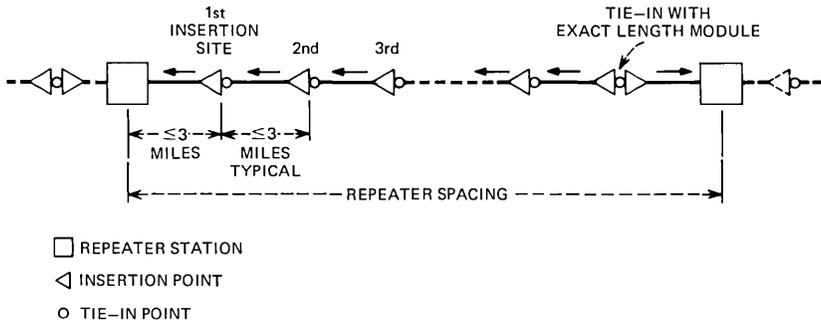
Fig. 1—Insertion segments within a waveguide repeater span.
