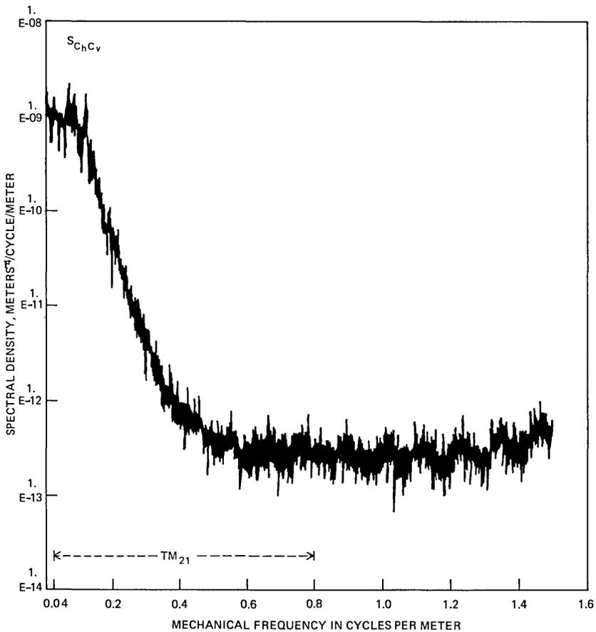
Fig. 7—Average field test  $C_h C_v$  product spectrum.
