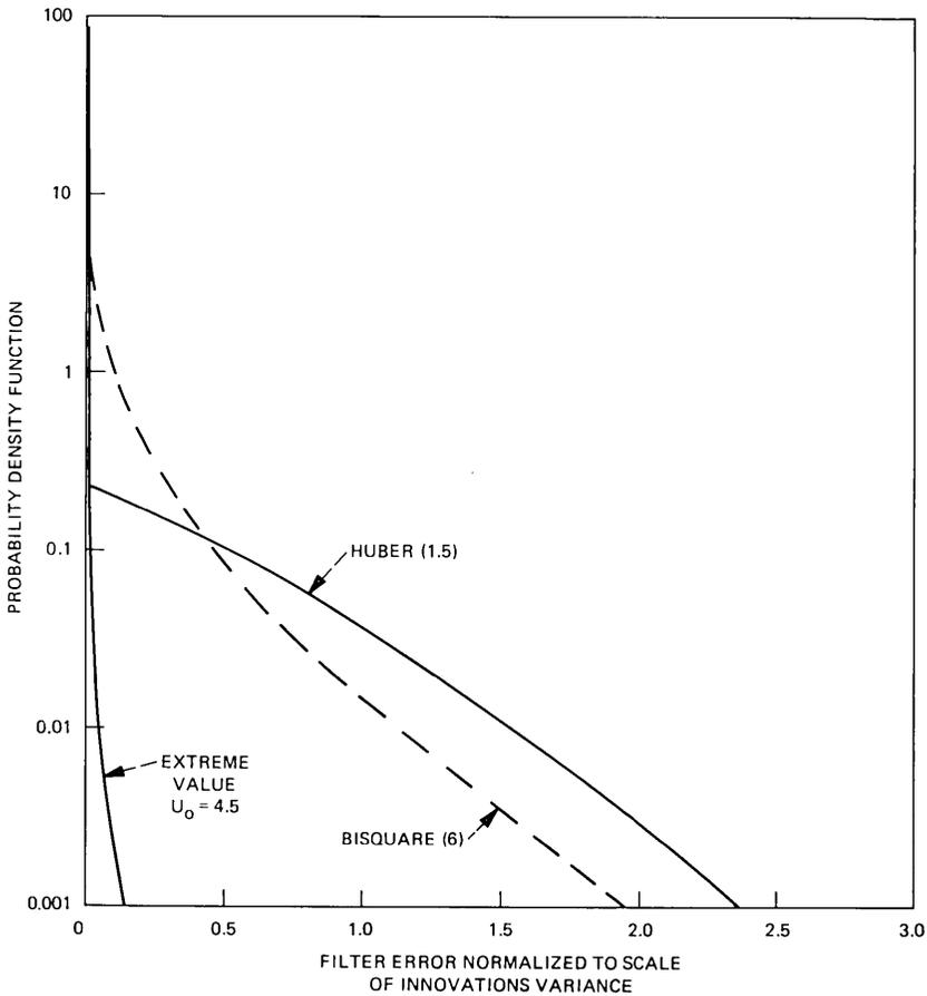
Fig. 16—Probability density functions for the error sequence of a robust filter operating on a first-order autoregressive process with  $\alpha = 0.9$ . For the extreme value case the density appears to be trimodal with the side modes at  $\pm 6.5$  and a level of about  $10^{-5}$ .
