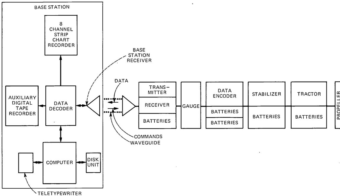
Fig. 8—Block diagram of field evaluation test mouse system.
