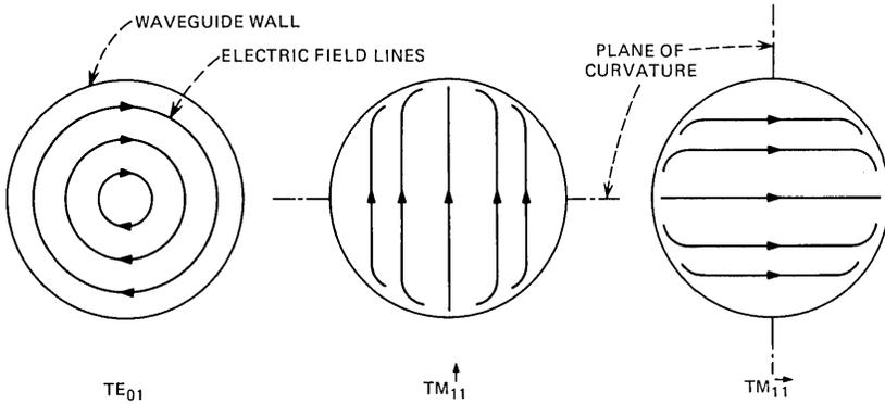
Fig. 1—Normal mode electric fields in dielectric-lined waveguide.
