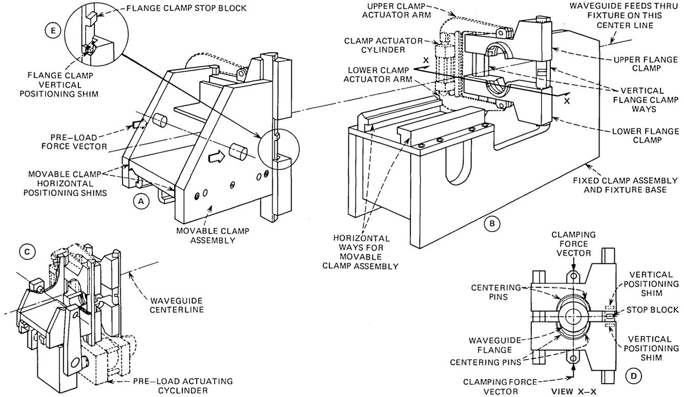
Fig. 5—The WSV aligning and preloading mechanisms.
