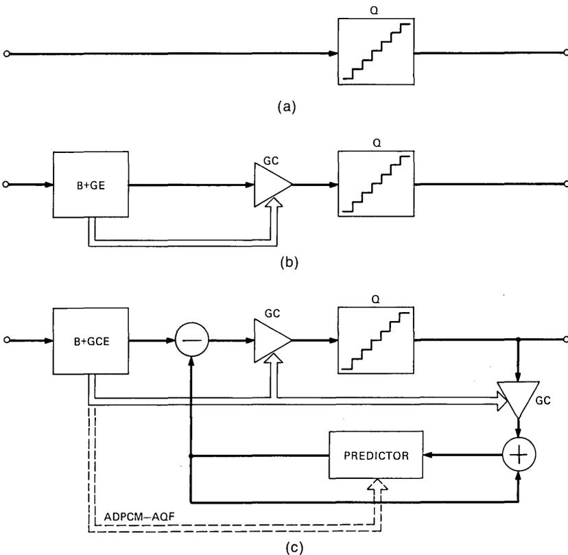
Fig. 6—Speech-encoding schemes. (a) Nonadaptive PCM. (b) PCM with adaptive quantization (PCM-AQF). (c) DPCM and adaptive DPCM (ADPCM) with adaptive quantization (DPCM-AQF, and ADPCM-AQF). Q = quantizer, GC = gain control, B + GCE = buffer and gain and coefficients estimation.
