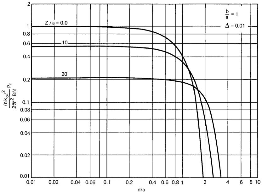
Fig. 5—Normalized total power injected into parabolic-index fiber as a function of the transverse source displacement  $d$  for several values of the distance  $z$  of the source from the fiber and for  $\Delta = 0.01$ .
