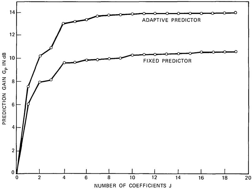
Fig. 11—Prediction gains vs number of predictor coefficients.
