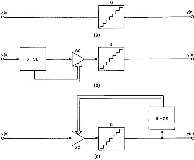
Fig. 1—PCM encoding schemes. (a) nonadaptive PCM. (b) Adaptive PCM with forward estimation (PCM-AQF). (c) Adaptive PCM with backward estimation (PCM-AQB).  $x(n)$  = input signal,  $y(n)$  = quantized signal, Q = quantizer, GC = gain control, B + GE = buffer and gain estimation.
