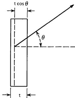
Fig. 1—Schematic of a partially opaque source disc. The effective width for waves emitted at a normal angle to the surface is  $t$ ; for waves emitted at an angle  $\theta$ , the effective width is  $t \cos \theta$ .
