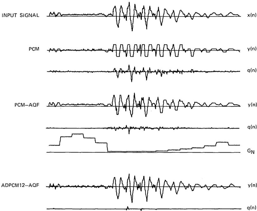
Fig. 8—Comparison of waveforms.  $x(n)$  = sequence of input samples (512 samples),  $y(n)$  = sequence of decoded samples,  $q(n)$  = sequence of quantization errors,  $G_N$  = sequence of amplifier gains.
