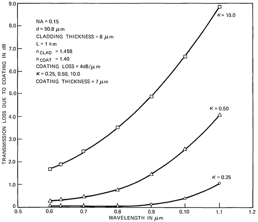
Fig. 12—Transmission loss due to coating vs wavelength.
