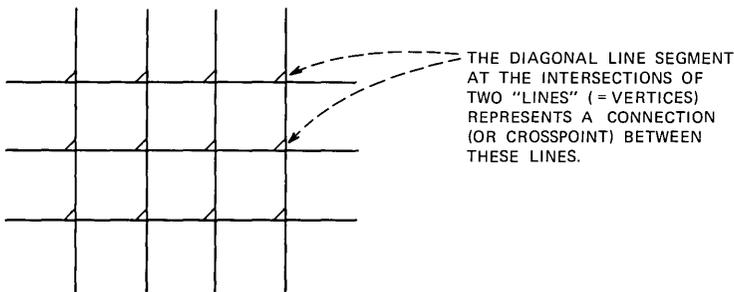
Fig. 8—Rectangle network of size  $3 \times 4$ .
