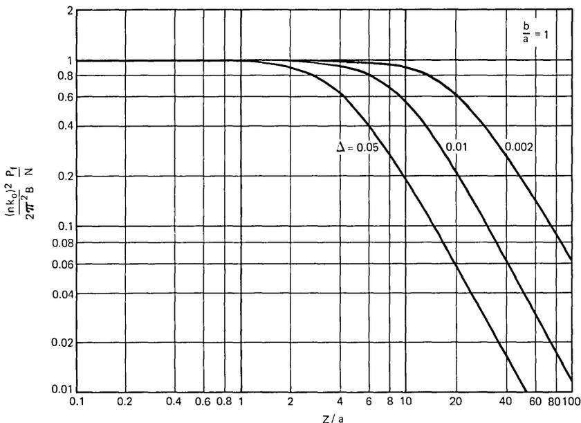
Fig. 4—Normalized total power  $P_i$  injected into the parabolic-index fiber as a function of the distance  $z$  between source and fiber.  $N$  is the total number of modes [see (28)];  $B$  is the source brightness. This figure holds for a source-to-fiber core radius ratio  $b/a = 1$ .
