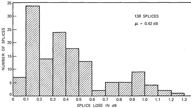
Fig. 8—Histogram of splice losses.
