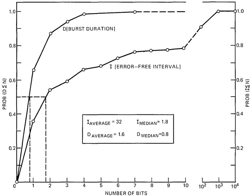
Fig. 1—Time statistics of burst errors [ $P(E) = 0.06$ ].
