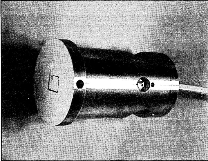
Fig. 4—Polishing fixture.
