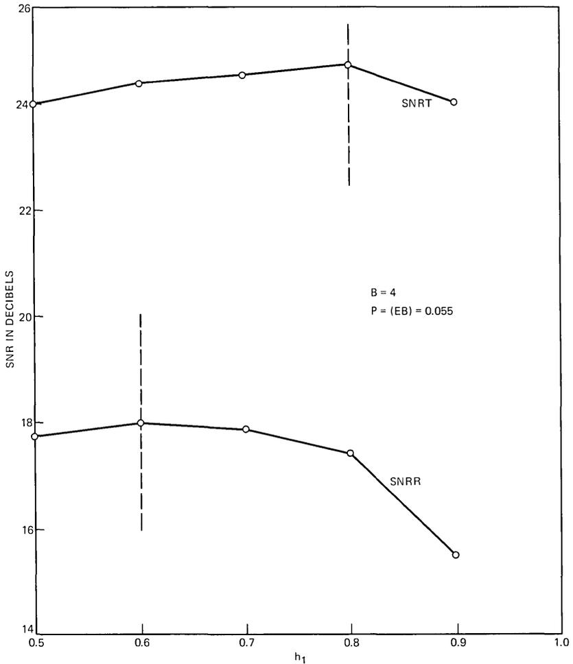
Fig. 13—Design of predictor coefficient  $h_1$  in DPCM-AQF.
