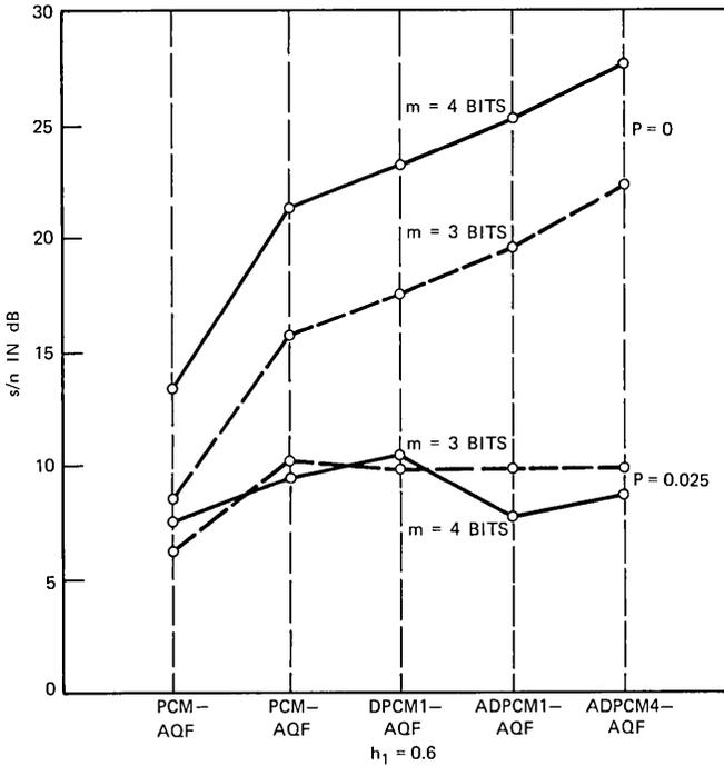
Fig. 16—Comparison of three- and four-bit encoding schemes.
