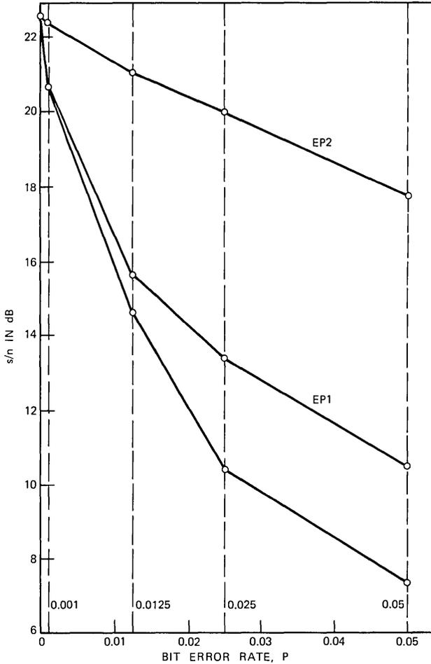
Fig. 11—Signal-to-noise ratio performance of a three-bit ADPCM4-AQF scheme in the presence of correlated errors.
