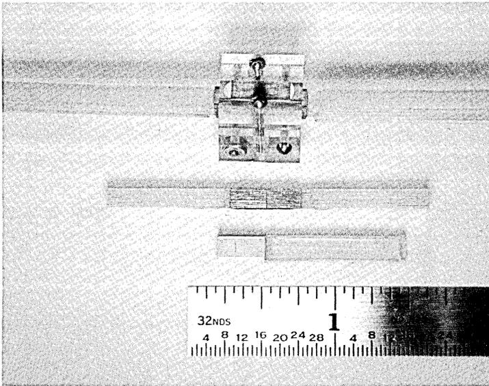
Fig. 6—Top: final alignment fixture; middle: epoxyed splice; bottom: single connector.
