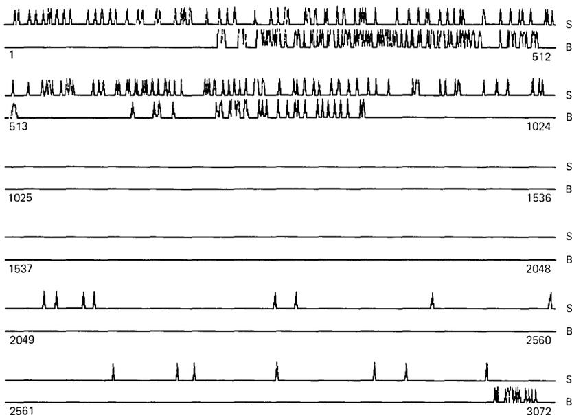
Fig. 4—Illustration of error scrambling [ $P(E) = 0.025$ ,  $V/\lambda = 36.2$  Hz].
