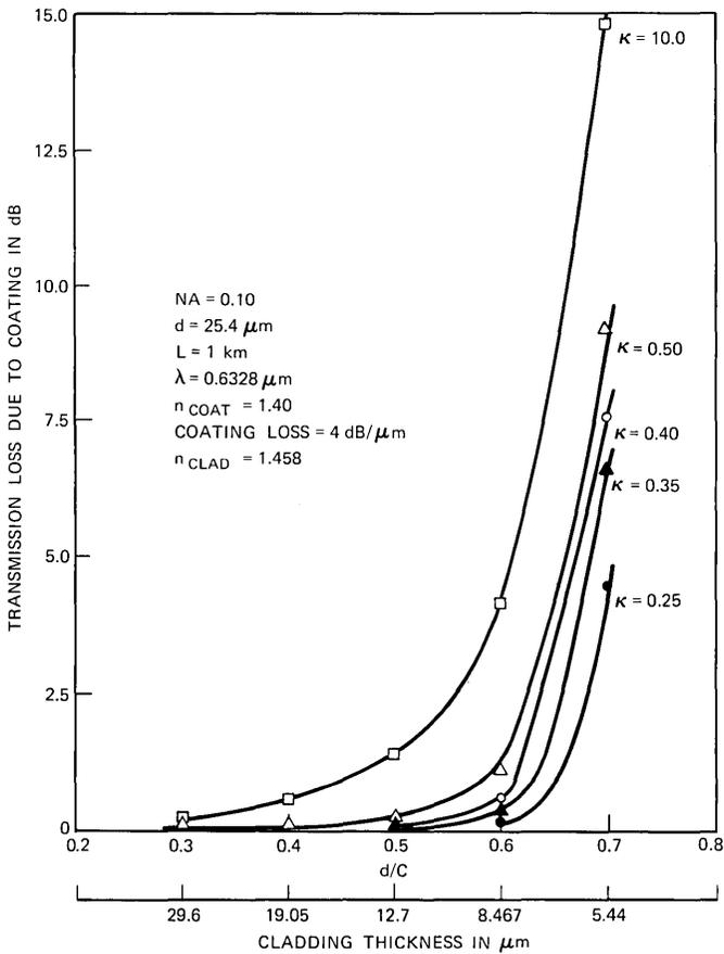
Fig. 3—Transmission loss due to coating vs  $d/C$  and vs cladding thickness; NA = 0.10,  $d = 25.4 \mu\text{m}$ .
