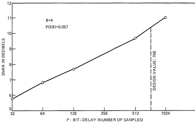
Fig. 15—Effect of time diversity on received-speech quality ( $V/\lambda = 36.2$  Hz).
