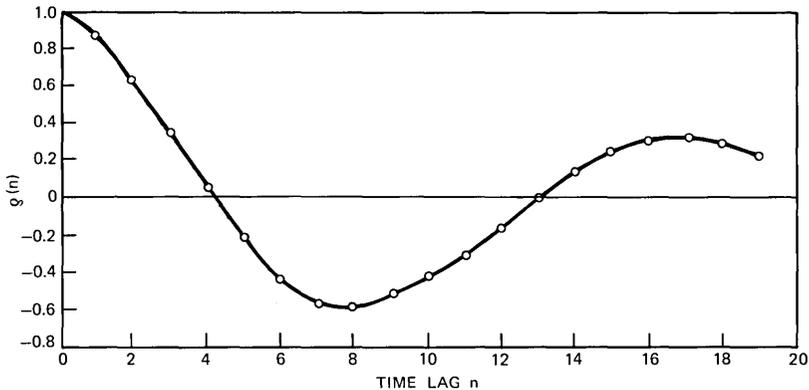
Fig. 10—Normalized autocorrelation function (female voice; 200 to 3200 Hz).
