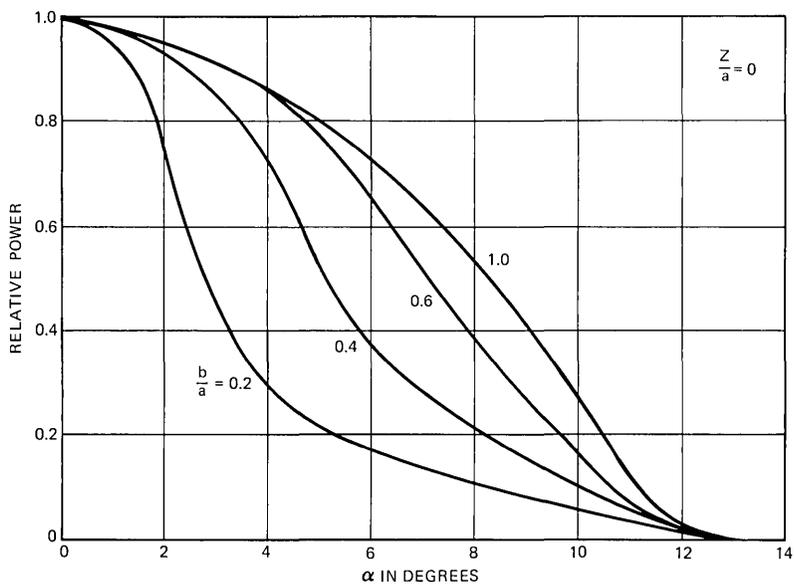
Fig. 11—Far-field radiation pattern from the end of the fiber for several values of the source-to-fiber core radius ratio  $b/a$ .
