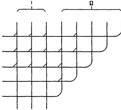
Fig. 9—Rearrangeable network corresponding to graph  $M(3, 5)$ .
