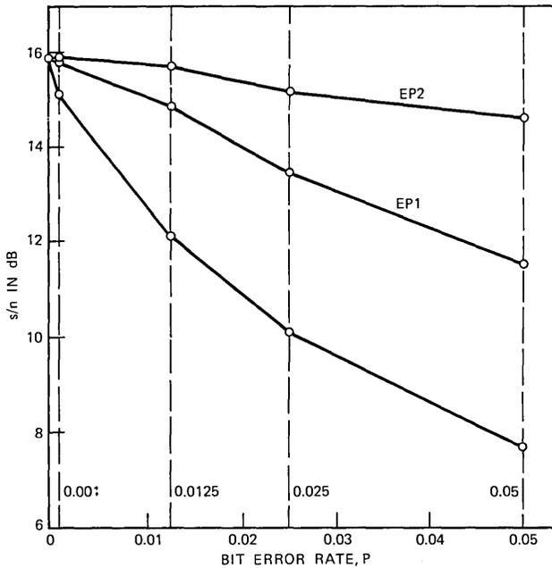
Fig. 8—Signal-to-noise ratio performance of a three-bit PCM-AQF scheme in the presence of correlated errors.
