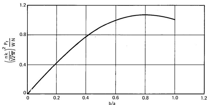
Fig. 13—Total power injected into the fiber with the high-brightness LEDs of Fig. 12 as a function of the (normalized) source radius  $b$ .
