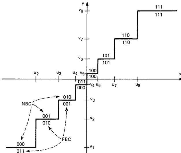
Fig. 2—Symmetric nonuniform quantizer.  $m = 3$  bits,  $M = 8$  steps, NBC = natural binary code, FBC = folded binary code.
