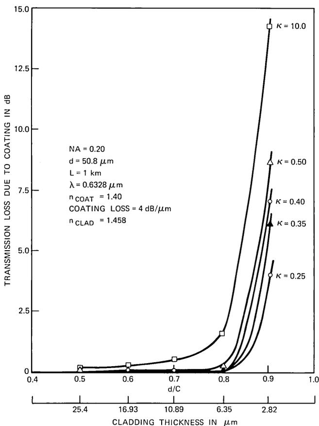
Fig. 8—Transmission loss due to coating vs  $d/C$  and vs cladding thickness; NA = 0.20,  $d = 50.8 \mu\text{m}$ .
