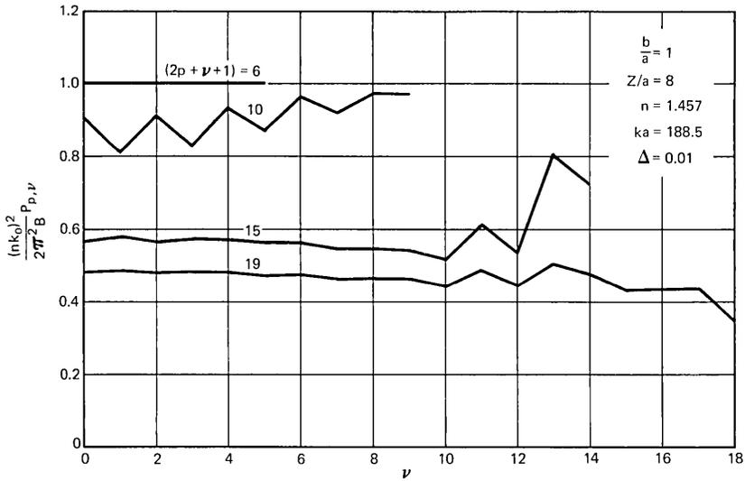
Fig. 8—Normalized power of individual modes belonging to the compound mode number  $2p + \nu + 1$  (whose values are given in the figure) as a function of the azimuthal mode number  $\nu$ . The source-to-fiber distance is  $z/a = 8$ , all other parameters are the same as in Fig. 7.
