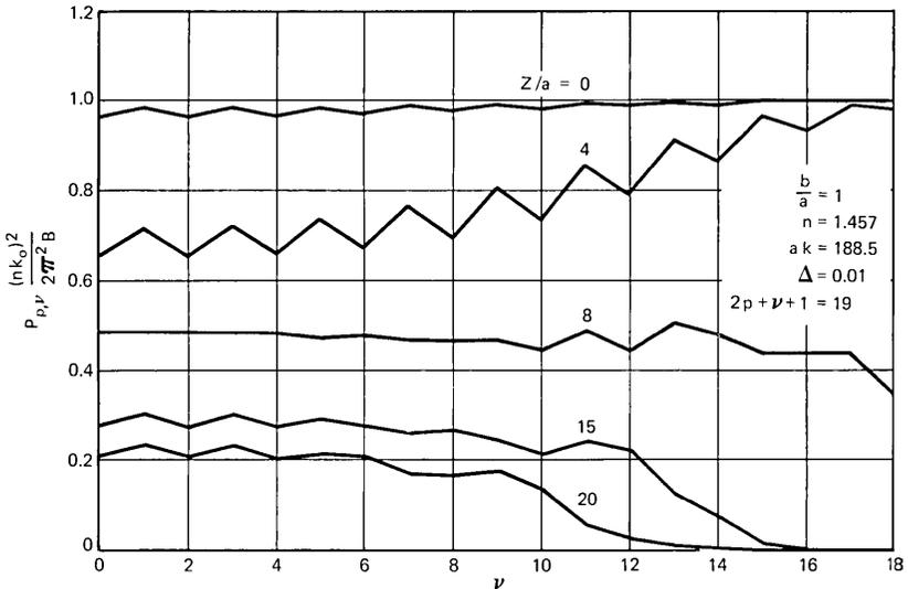
Fig. 7—Normalized power in a given mode belonging to the mode group with compound mode number  $2p + \nu + 1 = 19$  as a function of the azimuthal mode number  $\nu$  for several values of the distance  $z$  between source and fiber. These curves apply to the case  $b/a = 1$ ,  $ka = 188.5$ ,  $\Delta = 0.01$ ,  $n = 1.457$ .
