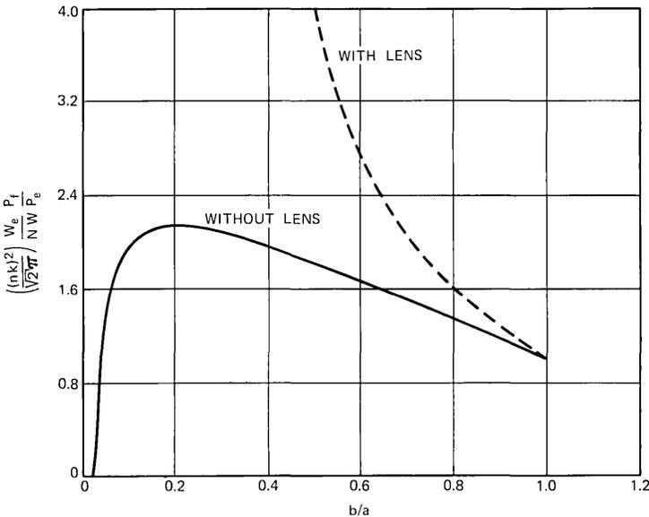
Fig. 15—Normalized ratio of total power injected into the fiber,  $P_f$ , relative to the electrical drive power  $P$  of the diode as a function of the (normalized) source radius. The solid curve applies for an LED in direct contact with the fiber; the dotted curve describes operation with a matching lens.
