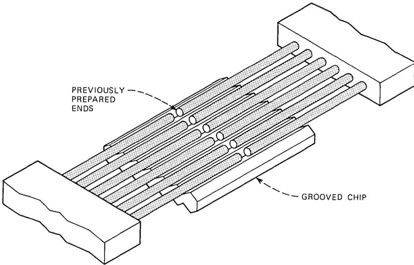
Fig. 9—Single layer of a permanent cable splice.
