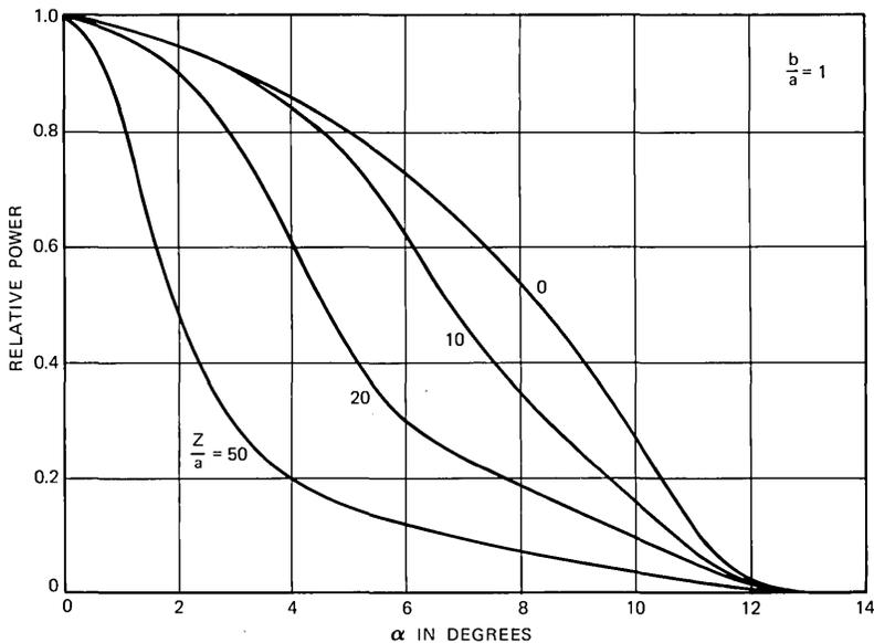
Fig. 6—Far-field radiation pattern.  $\alpha$  is the angle (in degrees) of the direction of the observation point with respect to the fiber axis. The curves are arbitrarily normalized to unity at  $\alpha = 0$ . The source-to-fiber core radius ratio is  $b/a = 1$ ,  $\Delta = 0.01$ .
