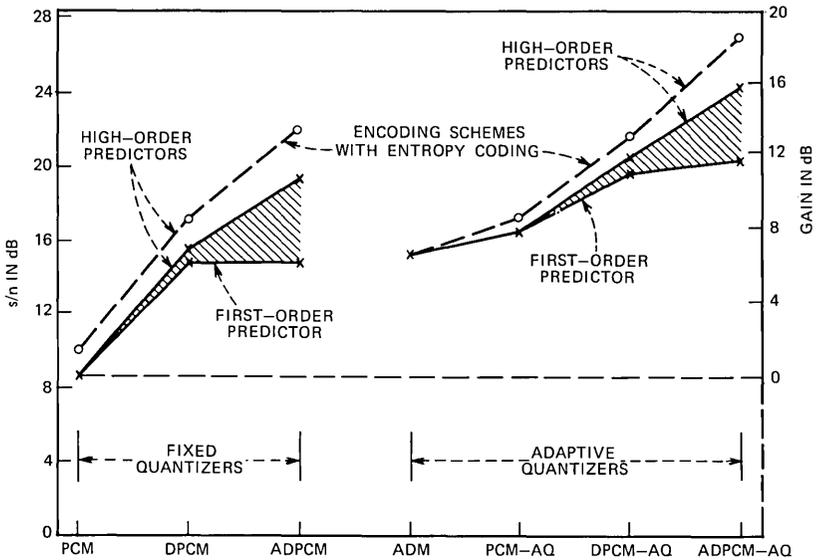
Fig. 7—Signal-to-noise ratio values and gains (over logarithmic PCM) for different three-bit speech-encoding systems.
