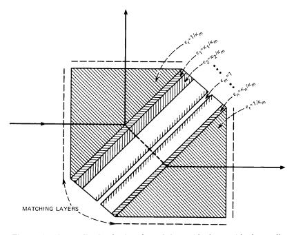
Fig. 2—A prism realization having the *m*th layer (the layer with the smallest dielectric constant) made of an air separation. Note that  $\kappa_m = \kappa_{\min} < 1$ . Matching layers are required at the external surfaces of the prisms.
