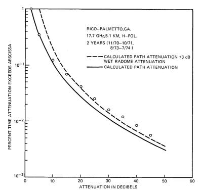
Fig. 6—Comparison of 17.7-GHz rain attenuation data at Palmetto, Georgia, with calculated result (solid line) using rain rate data in Fig. 12.
