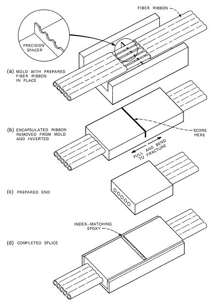
Fig. 1—The molded-plastic fiber-tape splicing technique.
