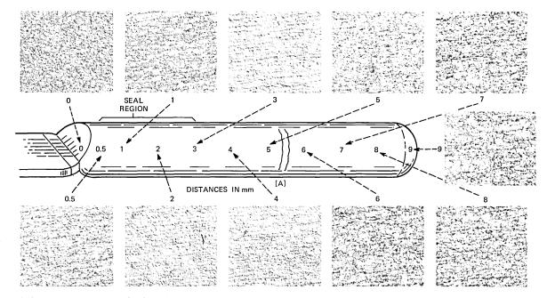
Fig. 5-Microstructures along the length of a typical sealed reed shank-etched 5-percent nital, DIC, 1500X. [A] represents the approximate end of the heat-affected zone.
