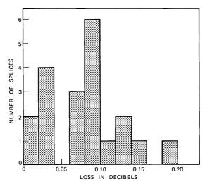
Fig. 8-Histogram of loss measurement data.
