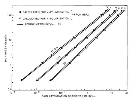
Fig. 2—Theoretical relationship between rain rate and rain attenuation gradient.
