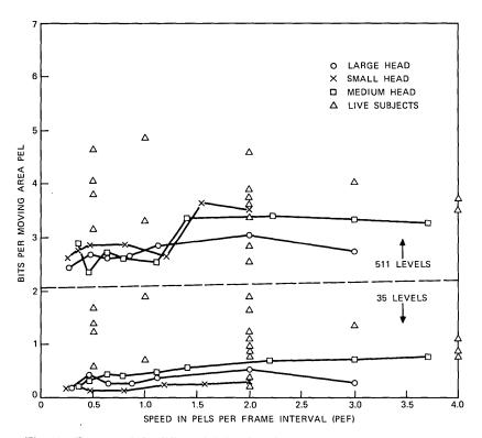
Fig. 10—Entropy of the differential signal in the moving area when minimum MSE linear prediction is carried out. In each field  $P_Z$  is the linear combination of the 22 pels shown in Fig. 2, which minimizes  $(Z - P_Z)^2$  averaged over the moving area. Entropies are significantly smaller than any of the previous results; however, live subject results are, in general, above the moving area results.
