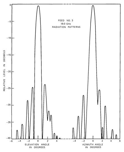
Fig. 9—Feed 3, 19.0-GHz radiation patterns.
