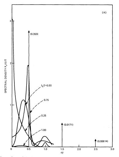
Fig. 2—Spectral density of binary FSK system with raised-cosine signaling and pulse duration T. K = 1.  $2f_d$  is the spacing between two adjacent *a priori* chosen frequencies.
