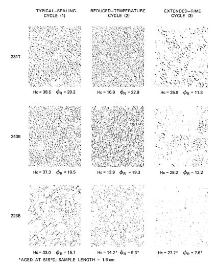
Fig. 7—Microstructures following various elevated-temperature exposures on samples shown in Fig. 6—etched 5-percent nital, DIC, 1500X.
