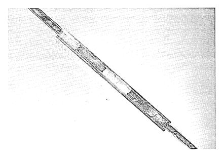
Fig. 10—Completed splice using brass alignment channel and epoxy cement both for index matching and for holding the assembly together.
