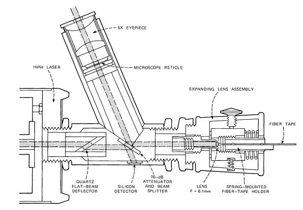
Fig. 6-Apparatus used for loss measurements.
