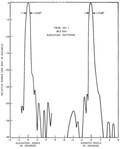
Fig. 12-Feed 1, 30.2-GHz radiation patterns.
