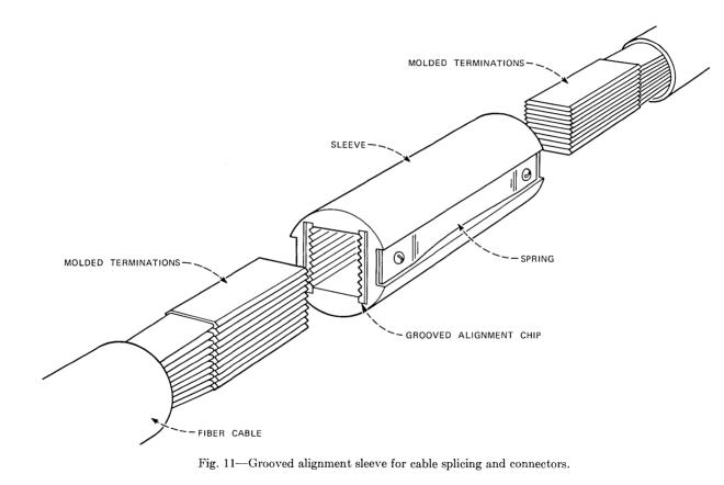
less than 0.1 dB. This technique involves no handling of individual fibers and alleviates some of the difficulties of fiber-end preparation and mechanical alignment of previously prepared ends that are encountered with other techniques.
