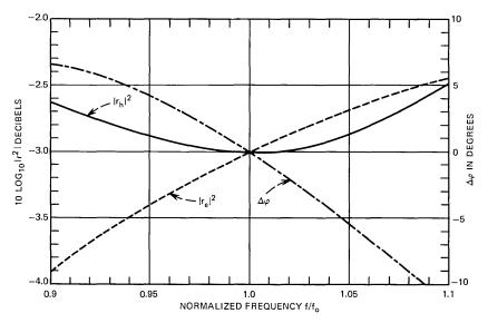
Fig. 5—Frequency response of the solution in 9.3 [five-layer, Type 1A solution with  $\theta = 46.91^{\circ}$ ,  $\epsilon_1 = \epsilon_3 = 2.1$  (Teflon),  $\epsilon_2 = 9.4$  (Kearfott Alumina),  $d_1/\lambda_o = 0.200$ ,  $d_2/\lambda_o = 0.084$ , and  $d_3/\lambda_o = 0.103$ ].
