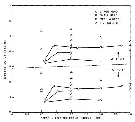
Fig. 13—Entropy of the differential signal in the moving area with minimum MSE linear prediction with subsampling, i.e.,  $P_Z$  is a linear combination only of pels B, D, F, G, J, M, P, R, T, U, and V.
