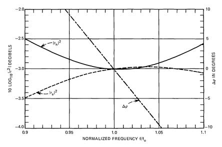
Fig. 4—Frequency response of the solution in 9.1 [three-layer, Type 1A solution with  $\theta = 73.43^{\circ}$ ,  $\epsilon_1 = 1.26$  (Buna S Rubber),  $\epsilon_2 = 9.4$  (Kearfott Alumina),  $d_1/\lambda_0 = 0.428$ , and  $d_2/\lambda_0 = 0.078$ ].
