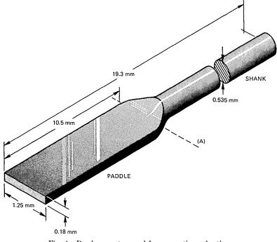
Fig. 4-Reed geometry used for magnetic evaluation.
