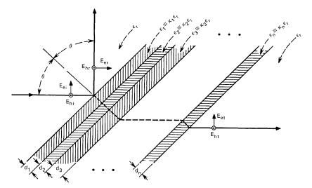
Fig. 1—*n*-layer dielectric inserted in a medium of a relative dielectric constant  $\epsilon_r$ . The subscript *h* refers to the *h*-mode (*E*-field perpendicular to plane of incidence), and *e* refers to the *e*-mode (*E*-field parallel to plane of incidence).
