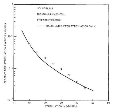
Fig. 8—Comparison of 18.5-GHz rain attenuation data in Holmdel, New Jersey, with calculated result (solid line) using rain rate data in Fig. 11.
