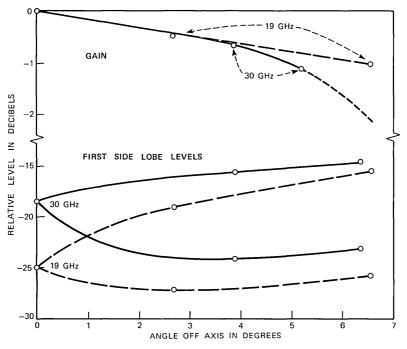
Fig. 6-Single-feed measurements of off-axis performance.
