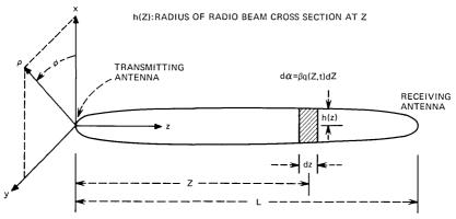
Fig. 1-Configuration of a radio path.
