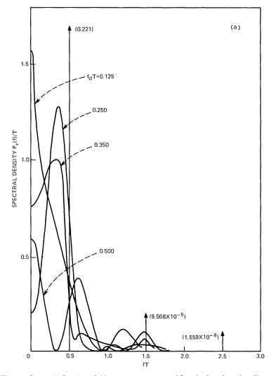
Fig. 5—Spectral density of binary FSK system with raised-cosine signaling and pulse duration 2T.  $K = 2.2f_d$  is the spacing between two adjacent *a priori* chosen frequencies.
