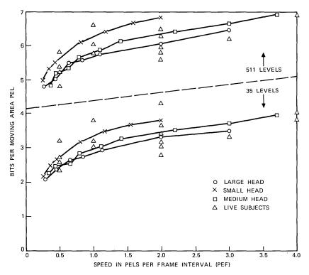
Fig. 3—Entropy of the frame difference signal in the moving area versus speed.  $P_Z = M$ . Starting with 8-bit PCM as was done in these simulations the differential signal could assume any of 511 levels. Results are also shown for coarser quantization to 35 levels which still gives very good picture quality. Solid curves are for the mannequin head at various distances from the camera. Unconnected points are for live subjects, such as in Figs. 1d and 1e.
