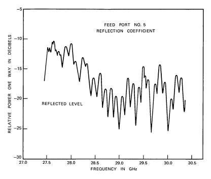
Fig. 15—Feed port 5, reflection coefficient.
