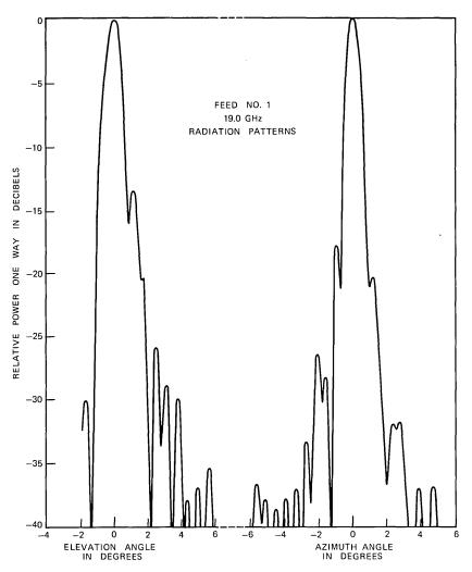
Fig. 10-Feed 1, 19.0-GHz radiation patterns.
