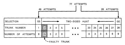
HOLDING TIME ESTIMATES FROM INDIVIDUAL CIRCUIT USAGE AND PEG COUNT DATA AVERAGE NORMAL HOLDING TIME = 246 s AVERAGE HOLDING TIME FOR TRUNK 2 = 19 s
