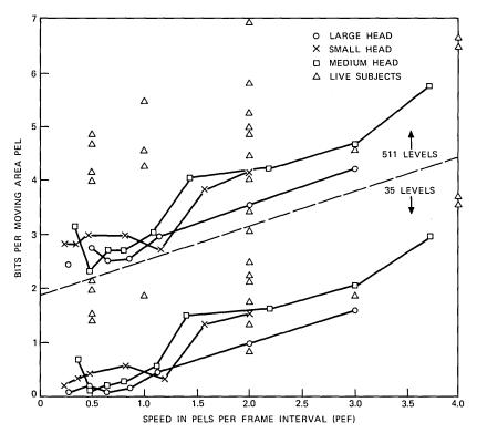
Fig. 12—Entropy of the differential signal in the moving area with minimum MSE linear prediction;  $P_Z$  is a linear combination only of the 11 pels in the previous frame. Results are about the same as those in Fig. 10 up to a speed of 1.3 PEF. Thus, in this range, the coder is removing mostly frame-to-frame redundancy.
