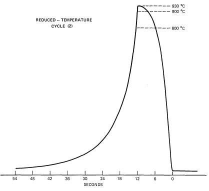
Fig. 2—Time/temperature thermocouple response for a 12-s insertion into a 1050  $^{\circ}\mathrm{C}$  furnace.
