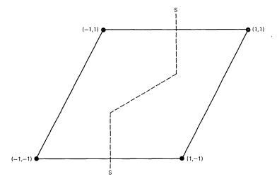
Fig. 2—Four signal points with intersymbol interference.
