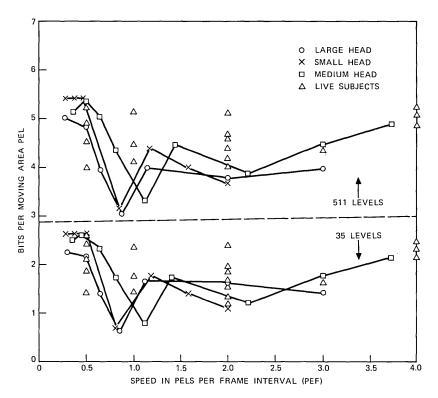
Fig. 9—Entropy of the differential signal in the moving area when movement compensation techniques are carried out. In this case,  $P_Z$  equals the pel in the previous field or frame that gives the smallest  $|Z - P_Z|$  averaged over the moving area. A sharp dip in the entropy occurs near 1 PEF.
