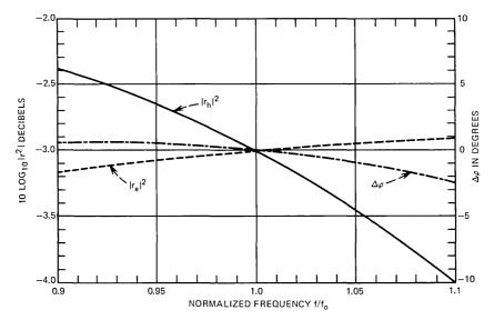
Fig. 6—Frequency response of the solution in 9.6 [three-layer, Type 2C prism solution with  $\theta = 45^{\circ}$ ,  $\epsilon_r = 2.54$  (polystyrene),  $\epsilon_1 = 1.59$  (Eccofoam PS),  $\epsilon_2 = 1$ ,  $d_1/\lambda_0 = 0.439$ , and  $d_2/\lambda_0 = 0.236$  ].
