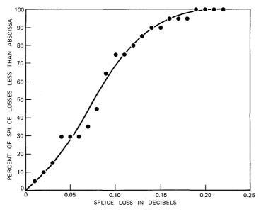
Fig. 9-Cumulative distribution of measured splice losses.
