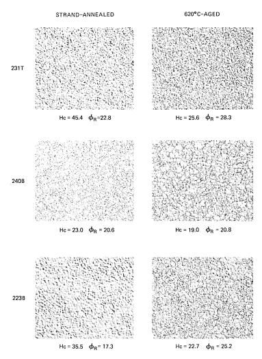
Fig. 6—Microstructures in strand-annealed and 620°C-aged conditions for two-phase (231T), primarily  $\alpha_1$ -phase (240B), and primarily  $\alpha_2$ -phase (223B) strand-annealed structures—etched 5-percent nital, DIC, 1500X.
