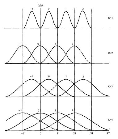
Fig. 1—Frequency modulation for different signal pulse durations. Index k is shown near peak of each pulse. Also, for simplicity, same signal pulse is shown for each k. T = time slot duration or signaling period. KT = maximum signal-pulse duration. Note different pulse center location for odd and even K.
