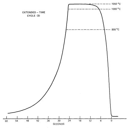
Fig. 3—Time/temperature thermocouple response for a 25-s insertion into a 1200  $^\circ\mathrm{C}$  furnace.
