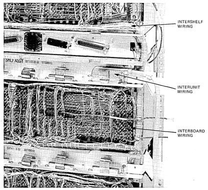
Fig. 2—Backplane wiring on DDs equipment.
