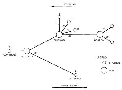
Fig. 4—A typical multipoint circuit.
