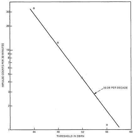
Fig. 6—Impulse noise on worst-case loop.
