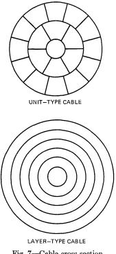
Fig. 7---Cable cross section.
