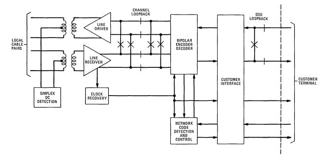
Fig. 10-DSU block diagram.
