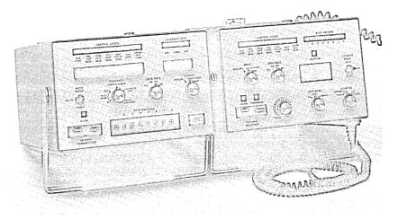
Fig. 6—Digital transmitter and receiver test sets.
