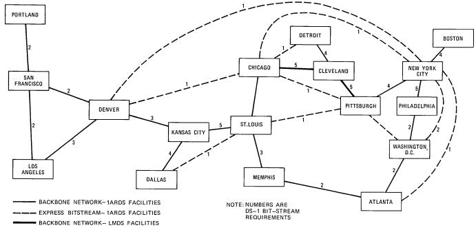
Fig. 5-Example network subset-backbone and express bit streams.
