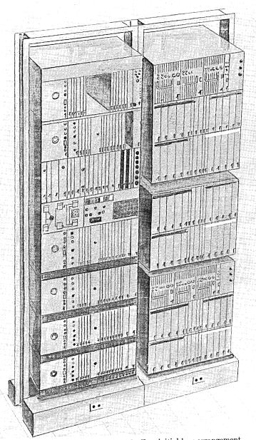
Fig. 4—Seven-foot, TIDM, local-office, initial-bay arrangement.
