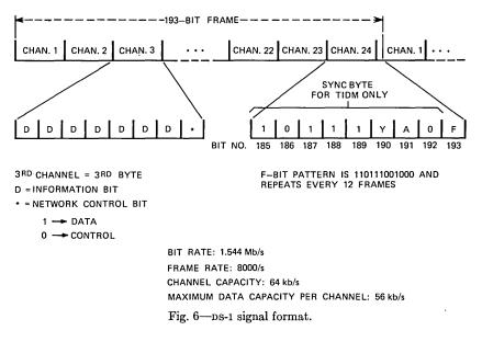
the 193rd or F-bit. As illustrated in Fig. 6, the former appear as a fixed pattern while the latter follows the 12-frame pattern employed in the D1D, D2, and D3 channel banks. Bits 190 and 191 are employed for housekeeping purposes by the T1DM. The remaining 23 bytes are assigned as data channels.
