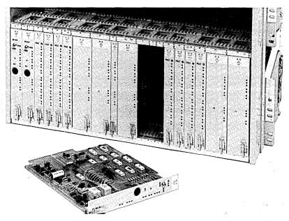
Fig. 1-Typical DDs circuit pack and equipment shelf.
