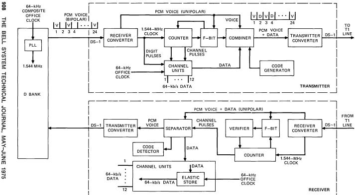
Fig. 9-T1WB4 data-voice multiplexer, simplified functional block diagram.
