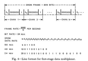
to form a framing channel. The length of the framing sequence is equal to the maximum number of channels of the SRDM. These sequences are shown in Fig. 4. The five-bit framing pattern used in the 9.6-kb/s SRDM is seen to be a subset of that employed in the 4.8-kb/s SRDM which, in turn, is a subset of that employed in the 2.4-kb/s SRDM. At the demultiplexer output, a 0 is inserted in bit position 1 of each channel.
