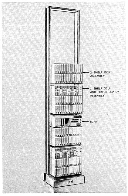
Fig. 3—Standard arrangement for office channel unit bay.
