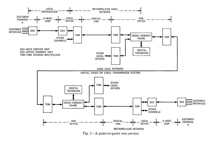
speed signal for long-haul transmission through the intercity network to the distant hub office. The high-speed signal may be carried over radio or cable systems of several types.
