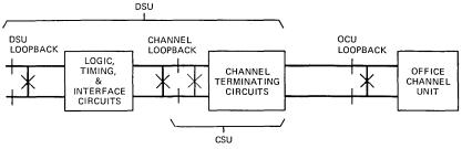
Fig. 8-Digital loopbacks.
