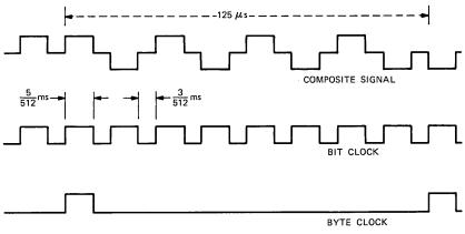
Fig. 4—Output clock waveforms.
