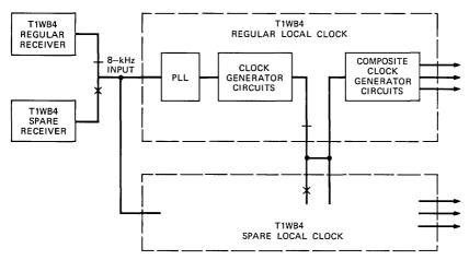
Fig. 10-General structure of integrated local timing supply.
