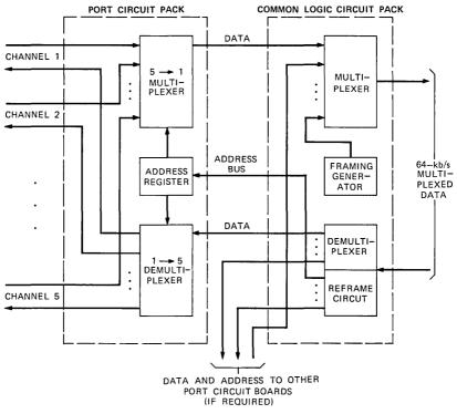
Fig. 5-Subrate data multiplexer, functional block diagram.
