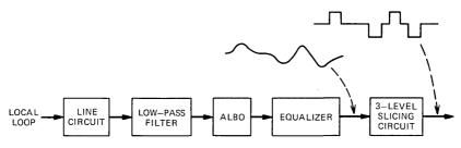
Fig. 2-Line receiver block diagram.
