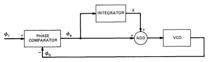
Fig. 3-Nodal timing supply phase-locked loop.
