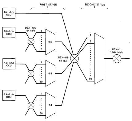
Fig. 1—Two-stage multiplex hierarchy.
