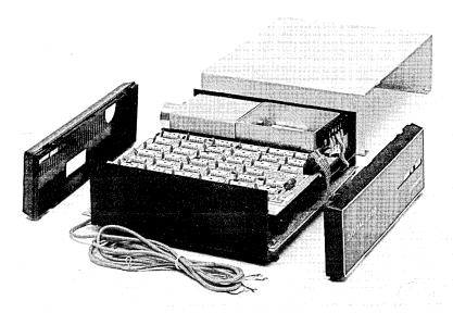
Fig. 10—Internal construction of DSU.
