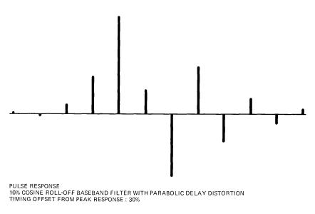
Fig. 3—Impulse response with peak distortion of 2.62.
