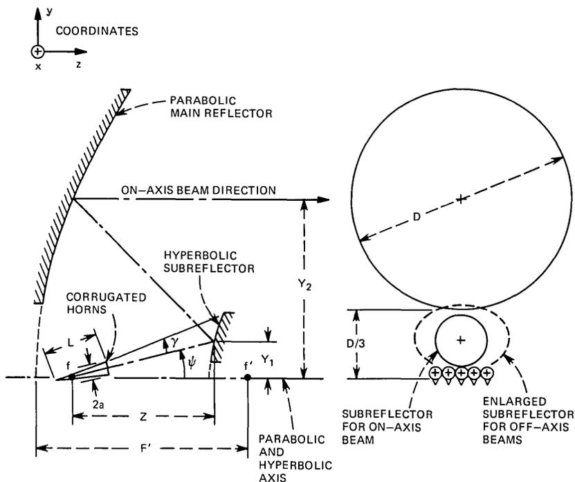
Fig. 1—Geometry of antenna and feed system. The feed horns are scaled for a 3m 20- and 30-GHz satellite antenna. For a 30m 4- and 6-GHz earth-station antenna,  $L$  and  $2a$  are half as large as shown.
