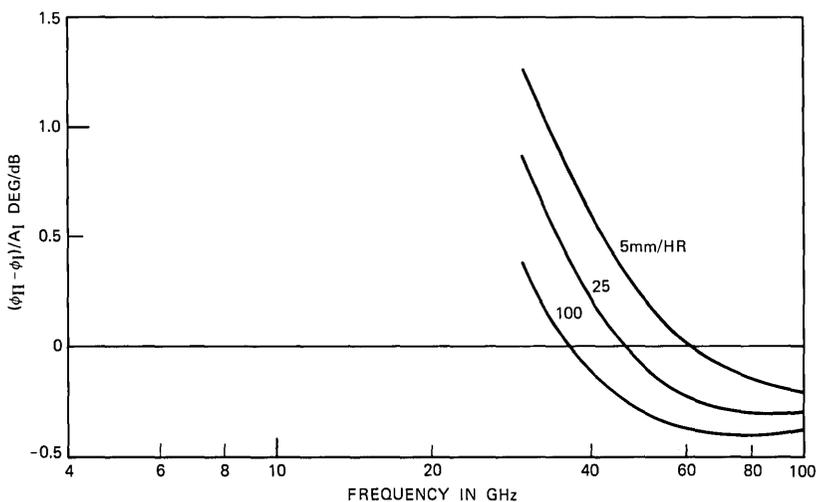
Fig. 4b—Normalized differential phase shift with respect to  $A_I$  (30 to 100 GHz).
