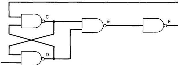
Fig. 10—Self-initializing circuit.
