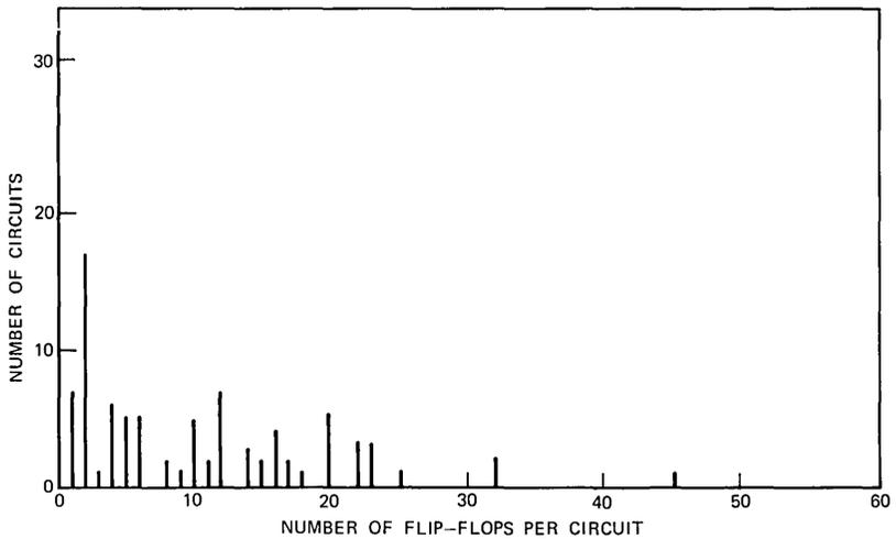
Fig. 14—Distribution of number of flip-flops per circuit.
