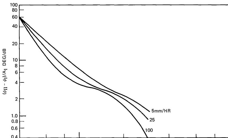
Fig. 4a—Normalized differential phase shift with respect to  $A_I$  (4 to 30 GHz).
