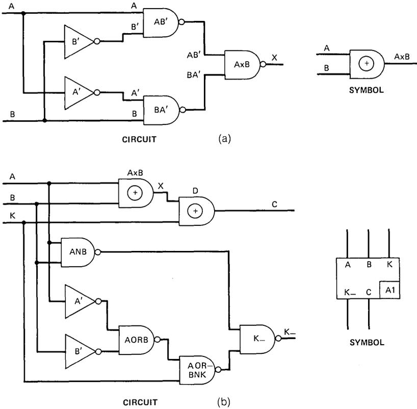
Fig. 2—(a) Exclusive-or circuit. (b) One-bit adder circuit.
