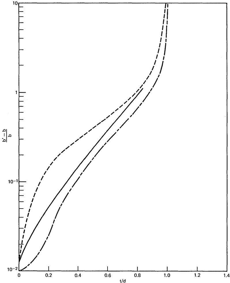
Fig. 10—Relative effective width of the core of the single-material fiber as a function of the relative thickness of its support slab  $t/d$  for the lowest-order mode. The solid line is the result of the numerical solution of the complete theory; the broken line was calculated from the solution of the approximate eigenvalue equation (34); and the dash-dot line is the result of Marcatili's theory.
