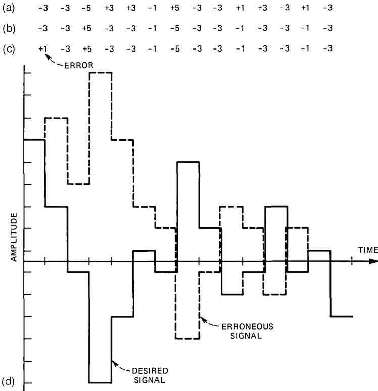
Fig. 6—Response of a multilevel differential code having step sizes  $\pm 1$ ,  $\pm 3$ ,  $\pm 5$ . (a) Ordinary differential code. (b) The code that signals changes of magnitude. (c) The code with an error. (d) The correct and erroneous responses.
