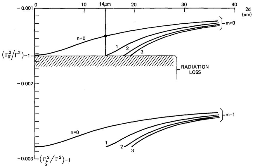
Fig. 3—Axial wave numbers  $\Gamma_{r,mn}$  for various  $m$  and  $n$  modes ( $r$  and  $\xi$  coordinates). Radiation loss is suffered whenever  $\Gamma_r < \Gamma_0$ . The radiation zone is shaded. This figure shows that single-mode propagation is possible if the ridge width  $2d$  is less than  $14 \mu\text{m}$  (for  $\lambda_0 = 1 \mu\text{m}$ ,  $n = 1.45$ ,  $t = 3.5 \mu\text{m}$ ,  $a = 50 \mu\text{m}$ , and  $\theta = 2.5^\circ$ ).
