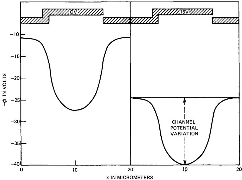
Fig. 6—Channel potential in a two-phase BCCD with all plates either at 0 or 15 volts. The parameters are  $d_1 = 0.6 \mu\text{m}$ ,  $d_2 = 0.12 \mu\text{m}$ ,  $Y_1 = 1.2 \mu\text{m}$ ,  $Q_n = 1.5 \times 10^{12} \text{cm}^{-2}$ ,  $N_A = 5 \times 10^{14} \text{cm}^{-3}$ .
