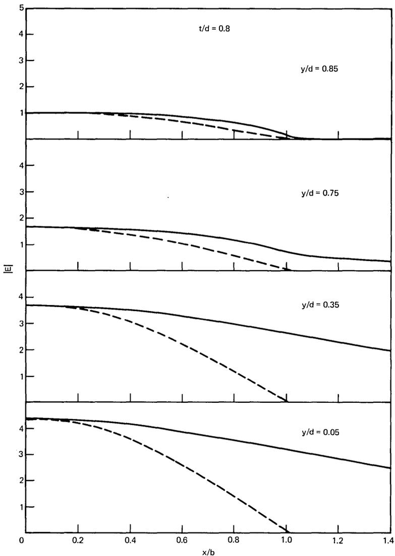
Fig. 5—Magnitude of the electric field vector shown as a function of the normalized horizontal dimension  $x/b$ . Solid curves describe the single-material fiber with  $t/d = 0.8$ , and the broken curves apply to the fiber with  $t/d = 0$ .
