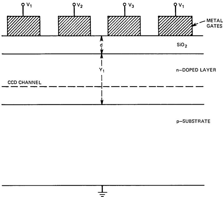
Fig. 1—Schematic diagram of a three-phase buried-channel CCD.
