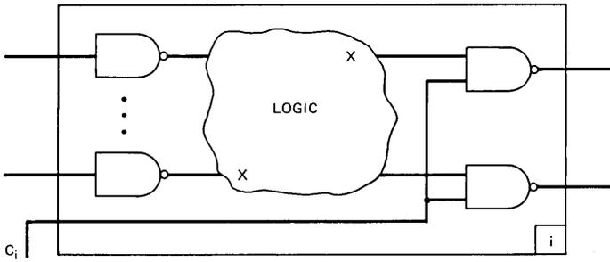
Fig. 4—Circuit-pack logic-disabling process.
