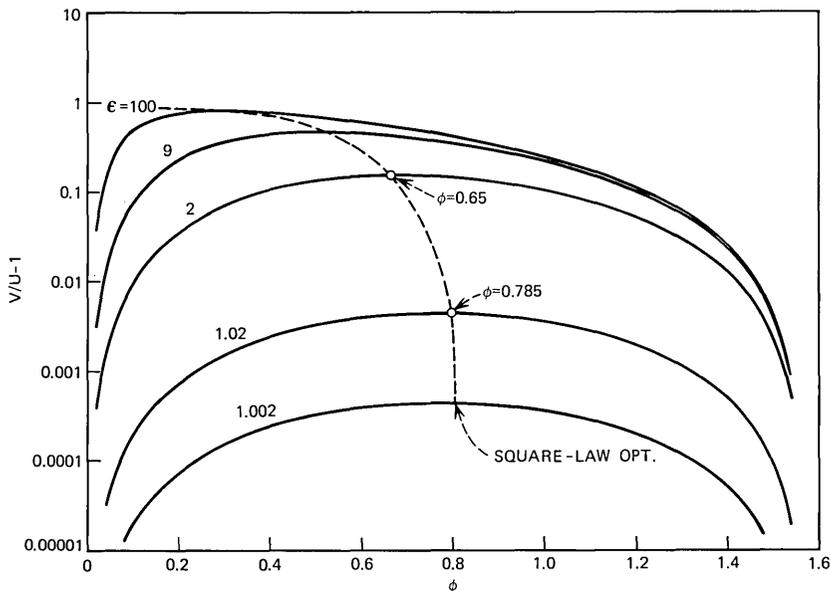
Fig. 2—Variation of the ratio of phase to group velocity in a dielectric slab for different relative permittivities, as a function of the characteristic angle  $\phi$ . The optimum points of operation for low pulse spreading in square-law tapered slabs are shown by a dashed line ( $\lambda = 1 \mu\text{m}$ ).
