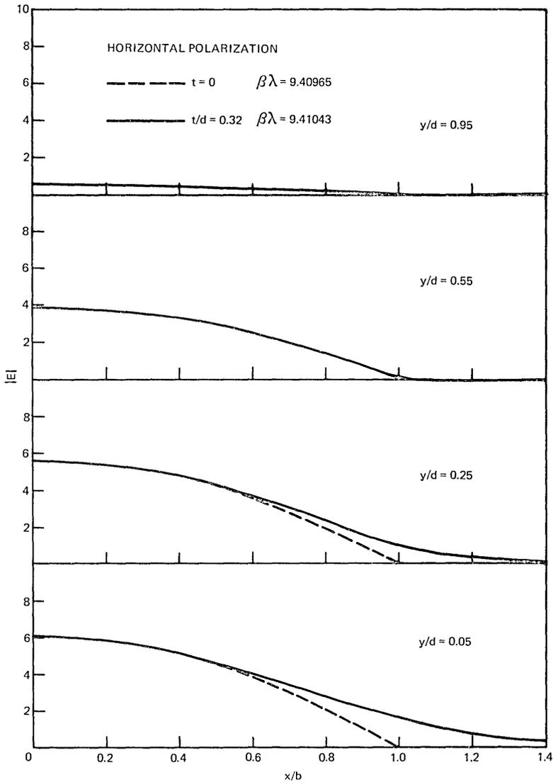
Fig. 3—Magnitude of the electric field vector shown as a function of the normalized horizontal dimension  $x/b$ . Solid curves describe the single-material fiber with  $t/d = 0.32$ , and broken curves apply to the fiber with  $t/d = 0$ .
