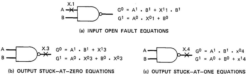
Fig. 8—Equations for handling faults in combinational circuits.
