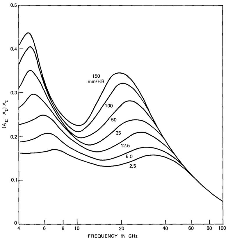
Fig. 3—Normalized differential attenuation with respect to  $A_I$ .
