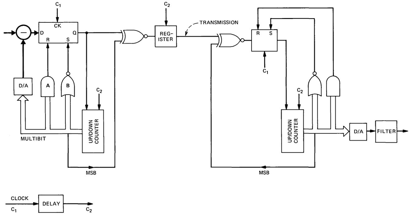
Fig. 2—Circuit that signals changes of magnitude.
