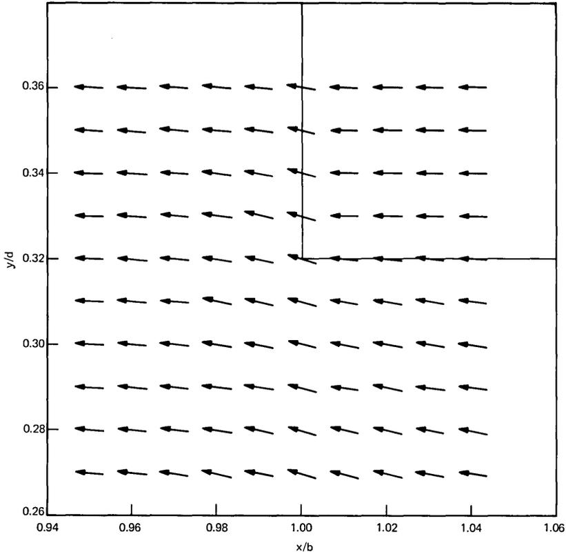
Fig. 9—Short arrows indicate the direction of the electric field vector of the lowest-order mode of the single-material fiber, with  $t/d = 0.32$  near the corner of the dielectric material where the support slab is attached to the core.
