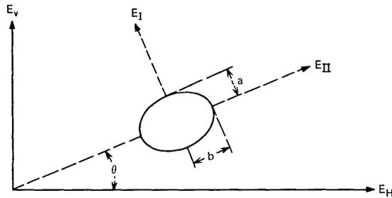
Fig. 1—Canted oblate spheroidal raindrop.
