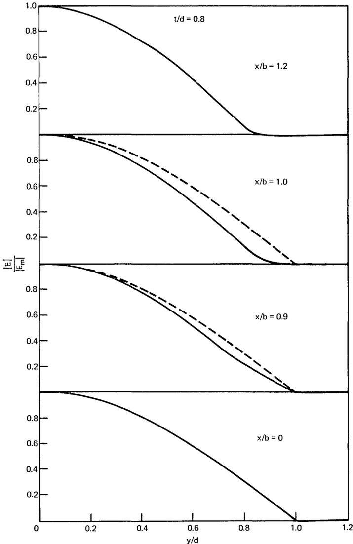
Fig. 6—Magnitude of the electric field vector relative to its maximum value at  $y = 0$  as a function of the normalized vertical dimension  $y/d$ . Solid and broken curves describe the single-material fiber with  $t/d = 0.8$  and  $t/d = 0$ .
