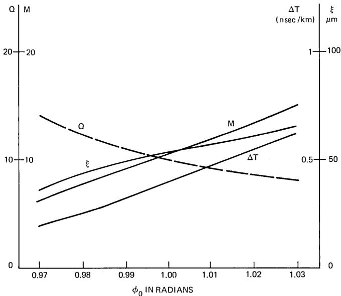
Fig. 5—Variation with the characteristic angle on axis  $\phi_0$  (or slab thickness on axis  $2d_0$ ) of the quality factor  $Q$  for  $\epsilon = 1.02$  ( $n = 1.01$ ) and  $\phi = \phi_0 - 5 \times 10^{-3}|y|$ . The variations of  $\xi$ ,  $M$ , and  $\Delta T$  are also given. The ray period is 5.6 mm and  $\theta_0$  is equal to  $4^\circ$  for  $\phi_0 = 1$ .
