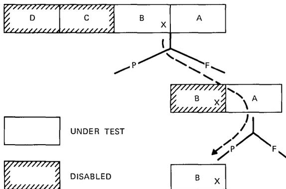
Fig. 2—Proposed method of fault location.
