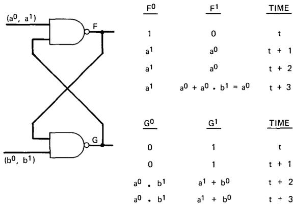
Fig. 4—Equations from  $F = 0, G = 1$  state.
