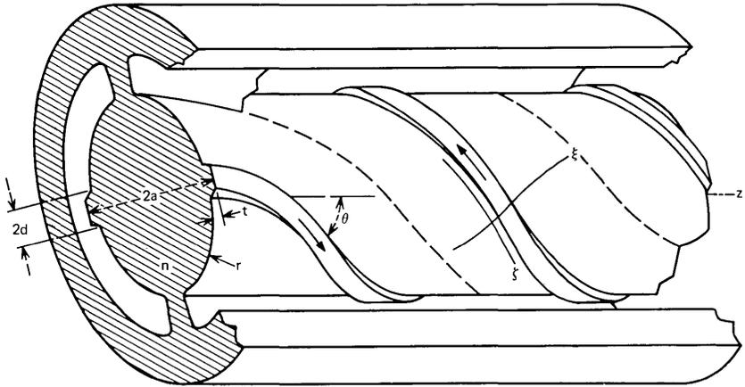
Fig. 1—Open view of the single-material, helicoidal fiber for two optical channels. The two optical beams propagate in the two ridges shown, with areas  $t \times 2d$ . The helicoidal motion is essential to maintain confinement. High-order modes are not confined. They radiate away to the envelope through the wings (only part of one is shown). The ratio period/diameter is much larger than that shown in the figure.
