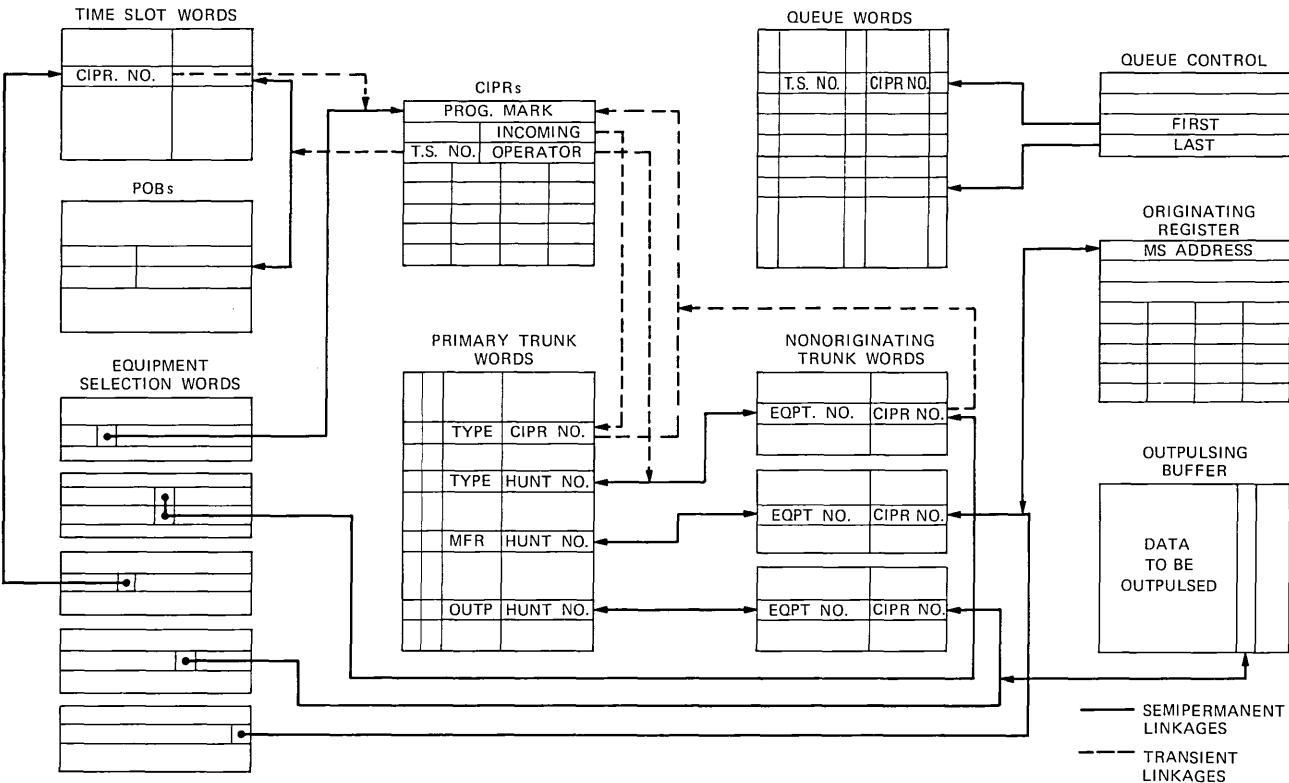
Fig. 12—Semipermanent call store linkage structure and transient linkage structure for connection between operator position and incoming intercept trunk.
