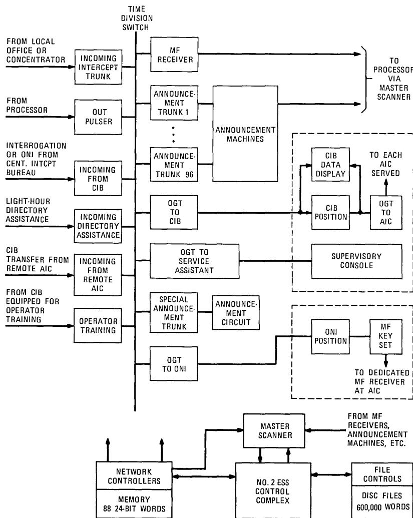
Fig. 3—Block diagram of an Automatic Intercept Center and operator positions.
