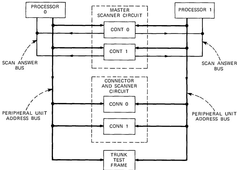
Fig. 15—Duplication or important network circuits.
