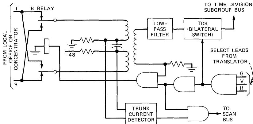
Fig. 2—Trunk circuit.
