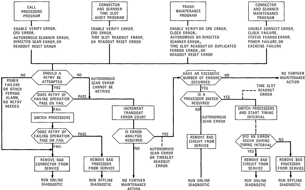
Fig. 16—Connector and scanner fault detection and recovery.
