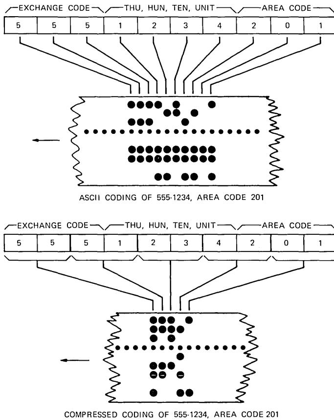
Fig. 5—Compressed code vs ASCII coding.
