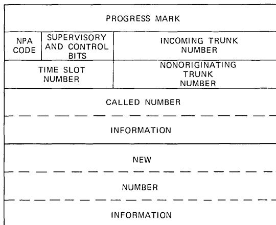
Fig. 3—Call-in-progress register (CIPR) format.
