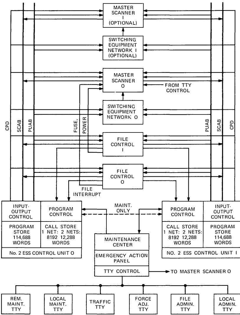
Fig. 4—Processor configuration and interfaces with peripheral equipment.
