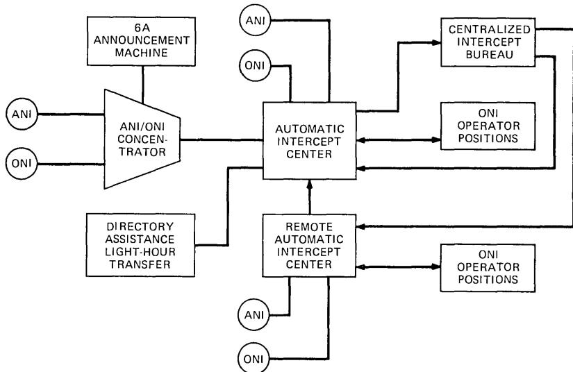
Fig. 2—Overall system configuration of an Automatic Intercept System.
