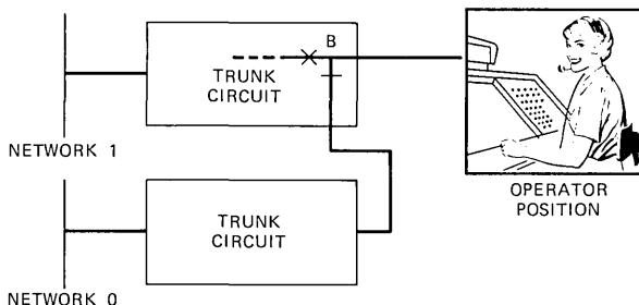
Fig. 3—Transfer arrangement for operator trunks.
