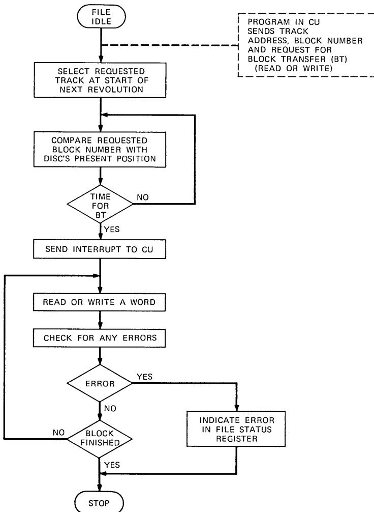
Fig. 6—Flowchart of block transfer.
